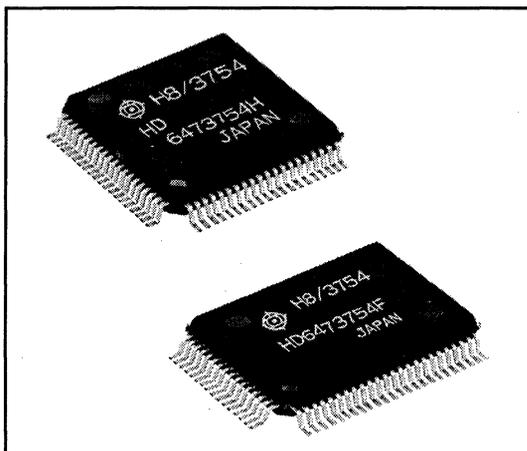
Additionally, the H8/3754 Series includes ZTAT™ (zero turn around time) versions of the H8/3726 that allow users to freely write programs to the on-chip PROM.
