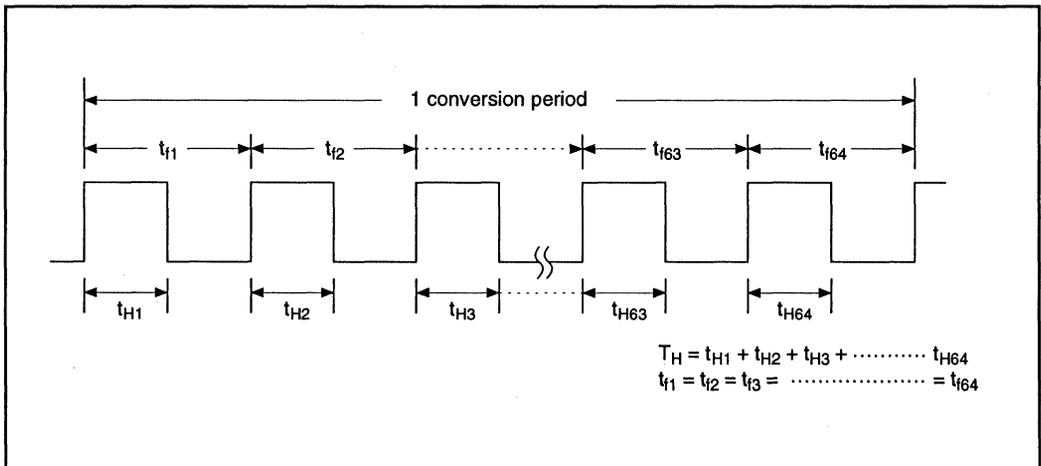
The output will be a high level output (100%) when the data value is between H'3FC0 and H'3FFF. The minimum conversion width pulse is output when the data value is H'0000.
