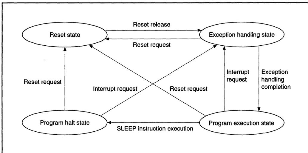
**Reset State:** The H8/300L CPU is reset in this state.
