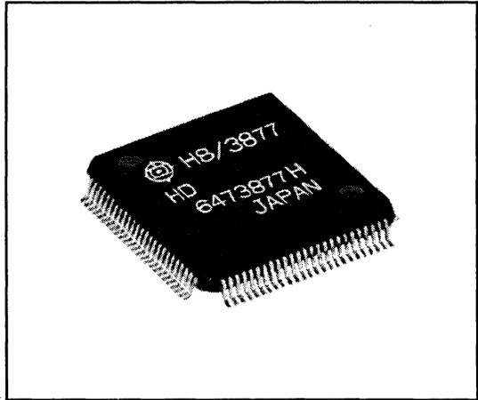
Additionally, the H8/3877 Series includes a ZTAT™ (zero turn around time) version of the H8/3877 that allows users to freely write programs to the on-chip PROM.
