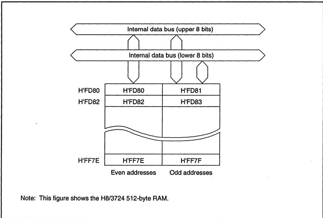
A short absolute addressing mode is provided by the H8/300L Series CPU MOV instruction for rapid access to locations from H'FF00 to H'FFFF. Furthermore, programs can be coded compactly due to the short instruction length. Since RAM locations H'FF00 to H'FF7F can be accessed by this short absolute addressing mode, programs can use this mode to implement high speed data handling.
