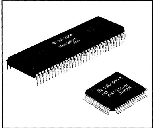
Additionally, the H8/3614 Series includes a ZTAT™ (zero turn around time) version of the H8/3614 that allows users to freely write programs to the on-chip PROM.
