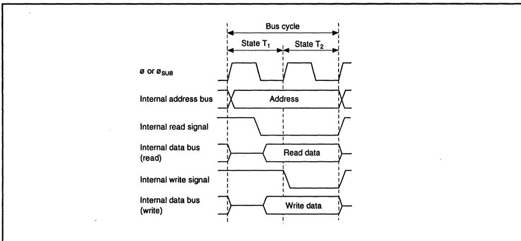
**On-Chip Peripheral Module Access Timing:** On-chip peripheral modules are accessed in two or three states. The data bus width in this case is 8 bits, so only byte access is possible.
