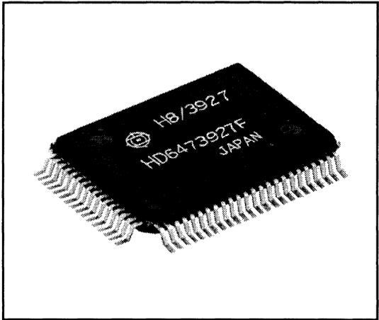
Additionally, the H8/3927 Series includes a ZTAT™ (zero turn around time) version of the H8/3927 that allows users to freely write programs to the on-chip PROM.
