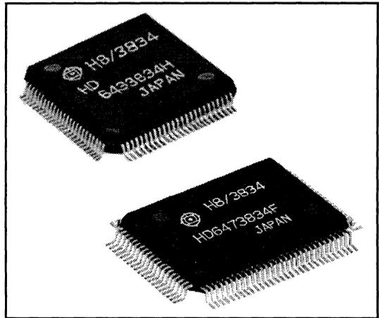
Additionally, the H8/3834 Series includes ZTAT™ (zero turn around time) versions of the H8/3834 and H8/3837 that allow users to freely write programs to the on-chip PROM.
