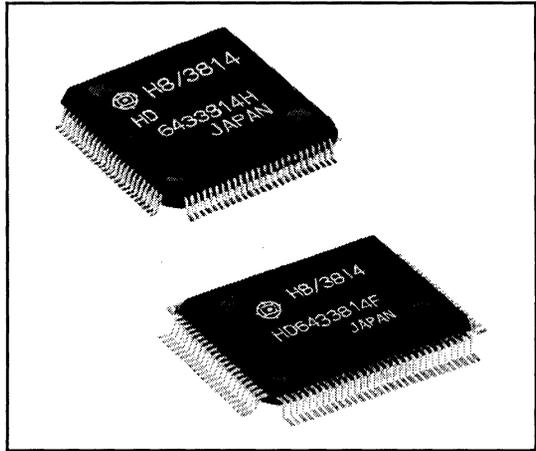
Additionally, the H8/3814 Series includes a ZTAT™ (zero turn around time) version of the H8/3834 that allows users to freely write programs to the on-chip PROM.
