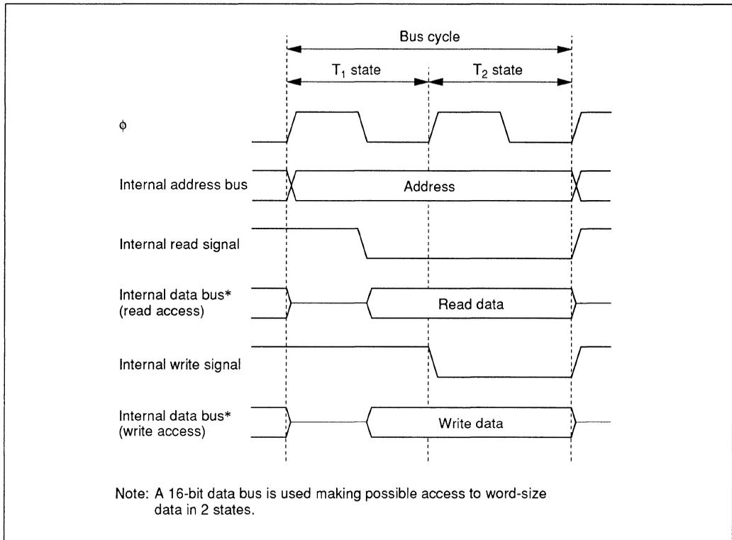
Figure 4-1. On-Chip Memory Access Cycle
