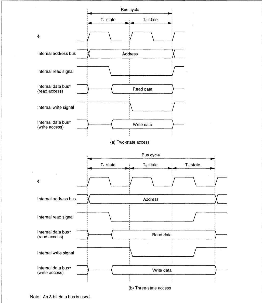
Figure 4-2. On-Chip Peripheral Module Access Cycle
