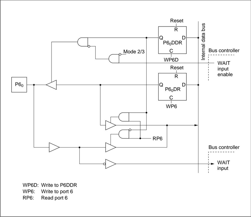
Figure C-5 (a) Port 6 Block Diagram (Pin P60)
