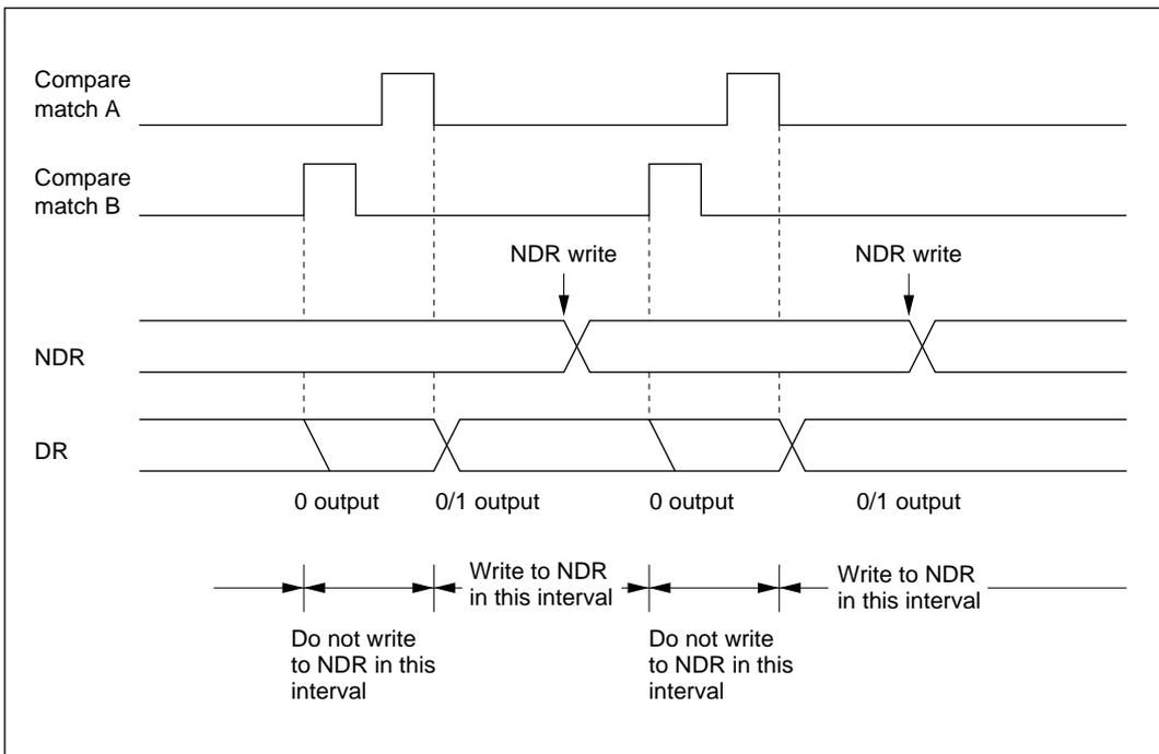
**Figure 9-10 Non-Overlapping Operation and NDR Write Timing**
