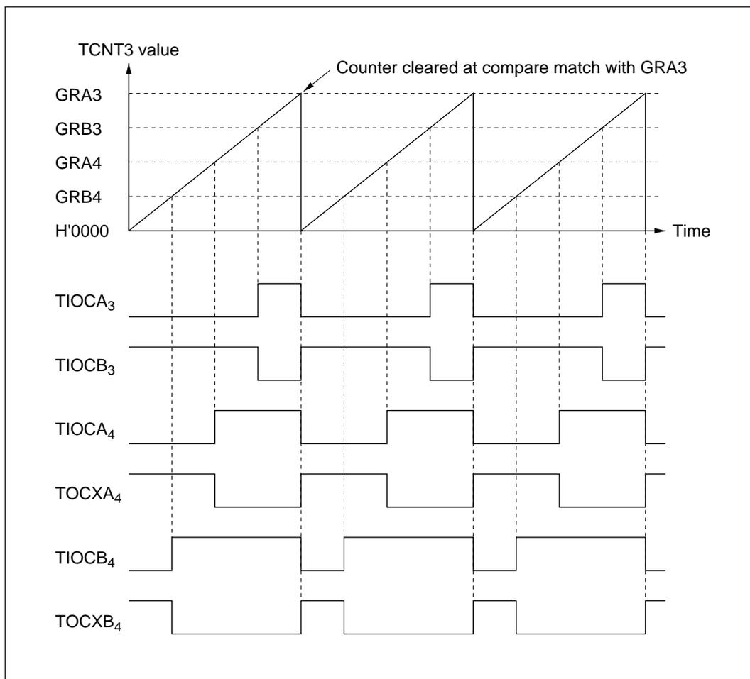
**Figure 8-32 Operation in Reset-Synchronized PWM Mode (Example)**
