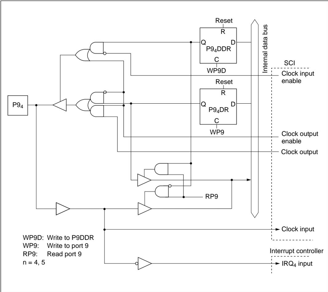
Figure C-8 (c) Port 9 Block Diagram (Pin P9<sub>4</sub>)
