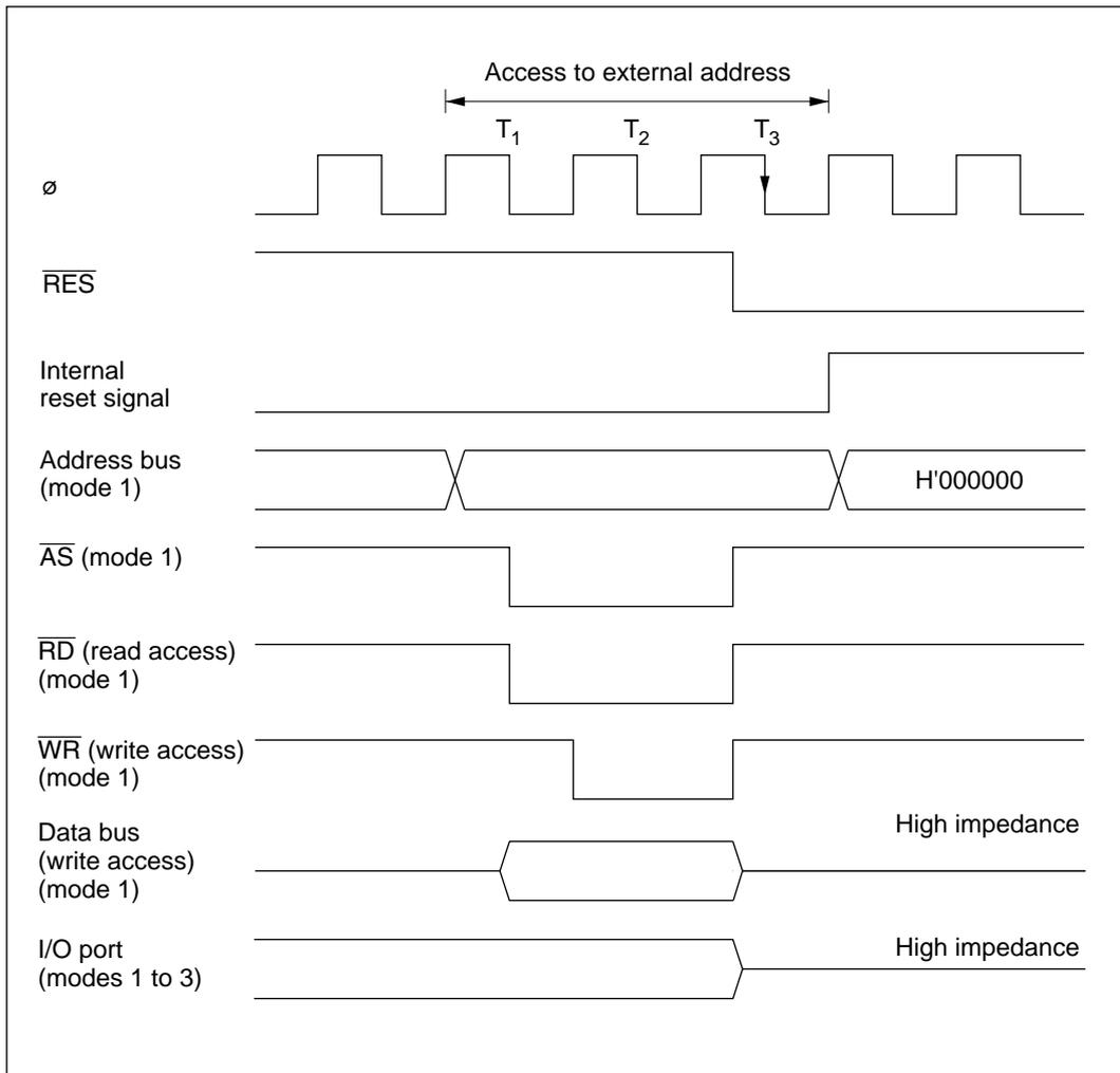
**Figure D-3 Reset during Memory Access (Reset during T<sub>3</sub> State)**
