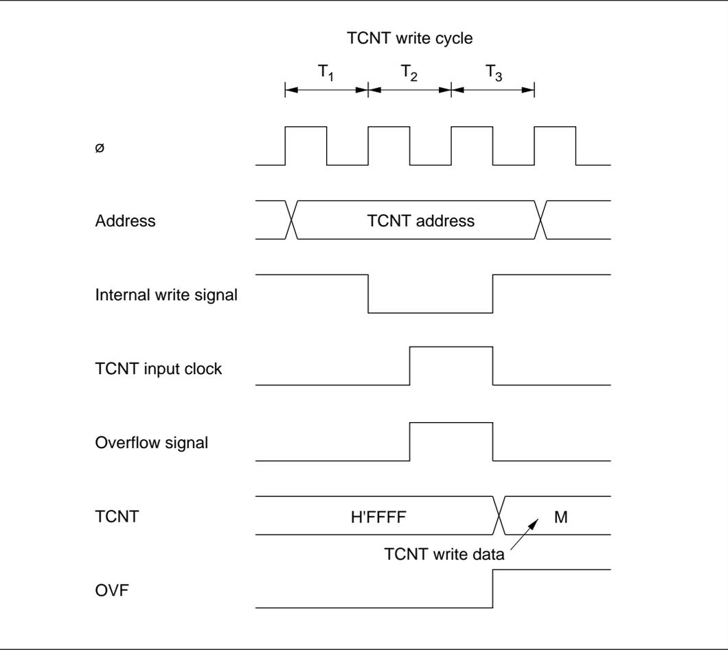
**Figure 8-65** Contention between TCNT Write and Overflow
