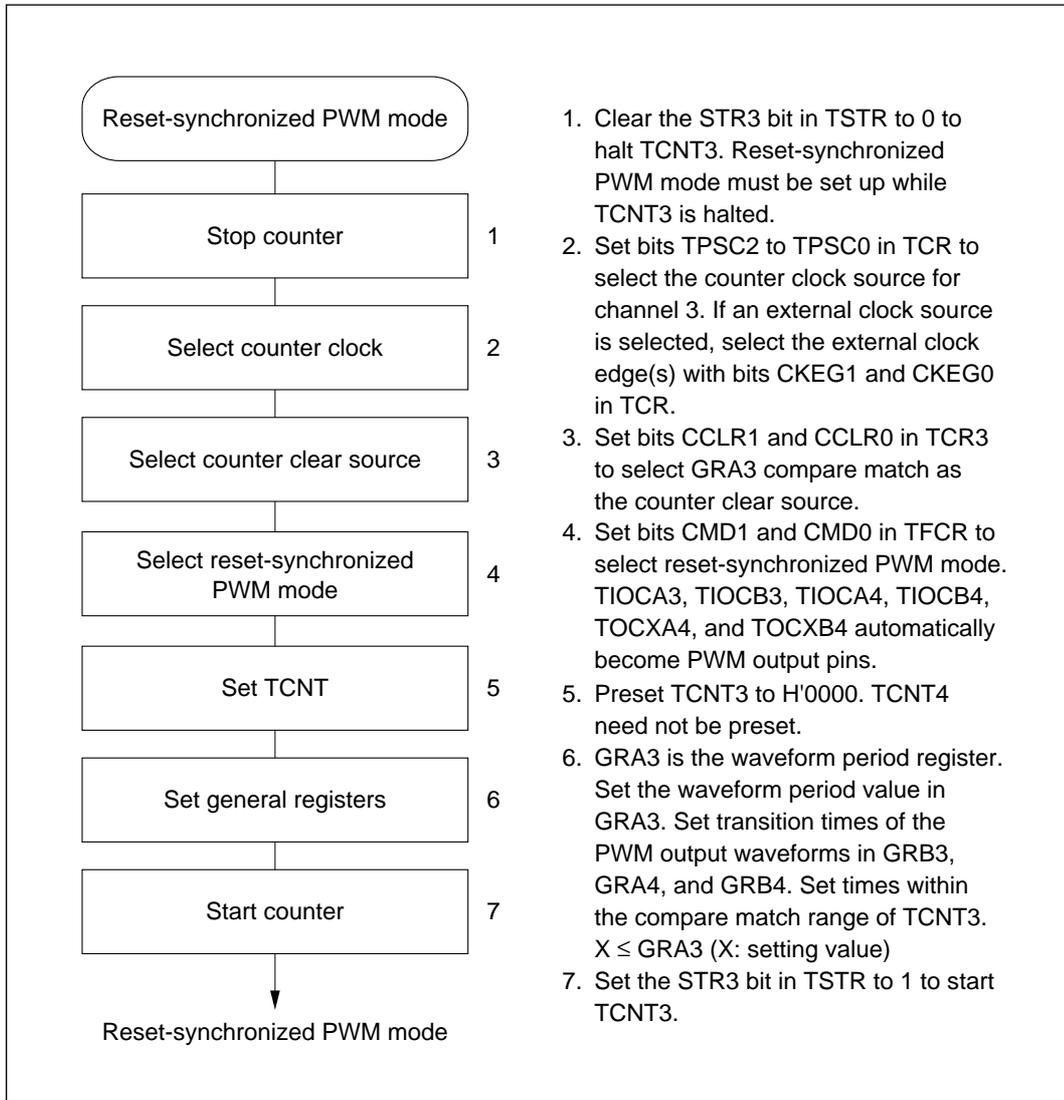
**Figure 8-31 Setup Procedure for Reset-Synchronized PWM Mode (Example)**
