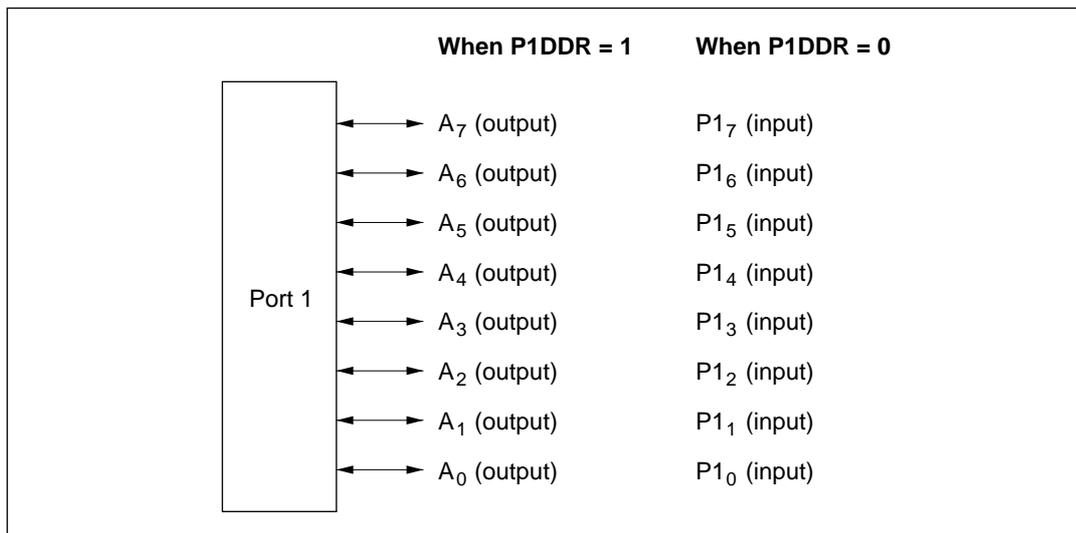
**Figure 7-2 Pin Functions in Mode 1 (Port 1)**
