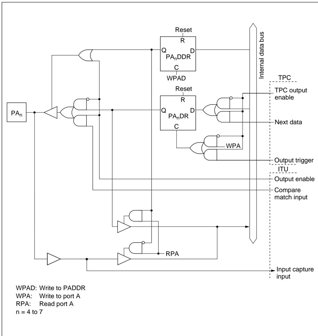
**Figure C-9 (c) Port A Block Diagram (Pins PA<sub>4</sub>, PA<sub>7</sub>)**
