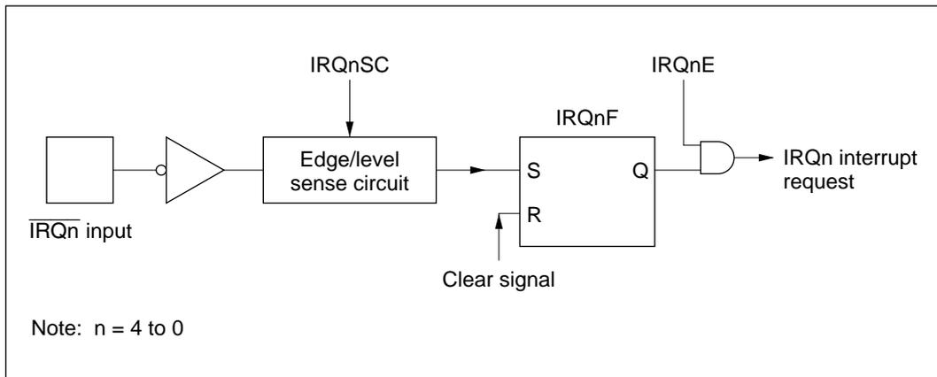
**Figure 5-2 Block Diagram of Interrupts IRQ<sub>0</sub> to IRQ<sub>4</sub>**
