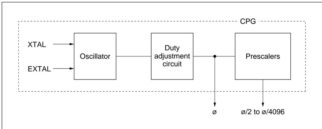
**Figure 15-1 Block Diagram of Clock Pulse Generator**
