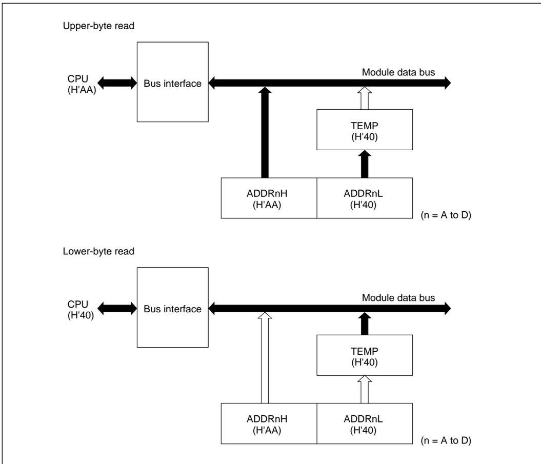
Figure 12-2 A/D Data Register Access Operation (Reading H'AA40)
