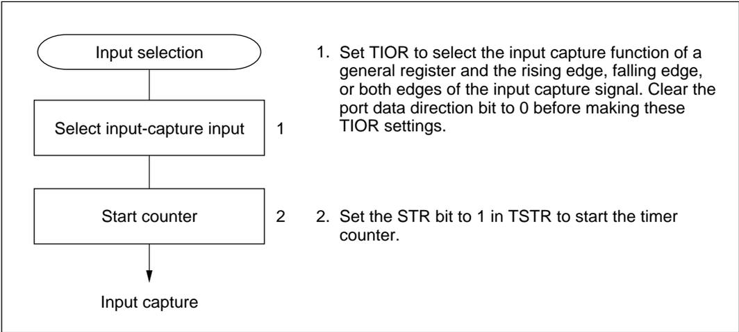
**Figure 8-23 Setup Procedure for Input Capture (Example)**
