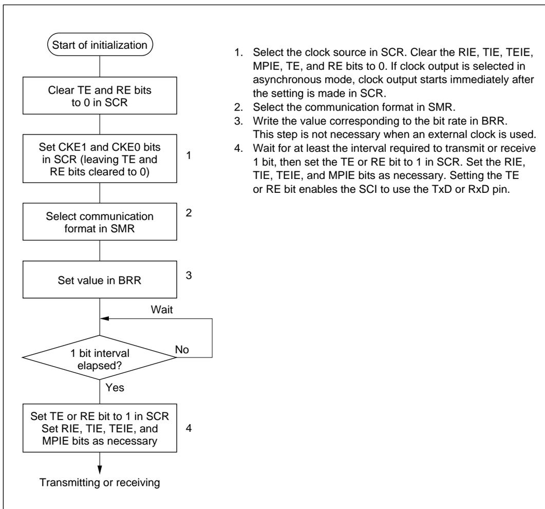
1. Select the clock source in SCR. Clear the RIE, TIE, TEIE, MPIE, TE, and RE bits to 0. If clock output is selected in asynchronous mode, clock output starts immediately after the setting is made in SCR.
