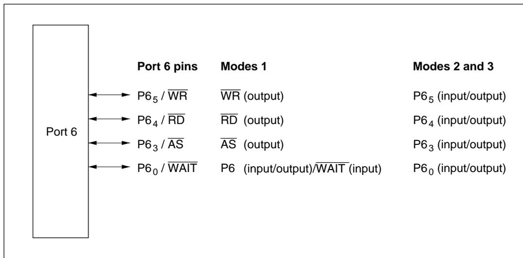
Figure 7-13 Port 6 Pin Configuration
