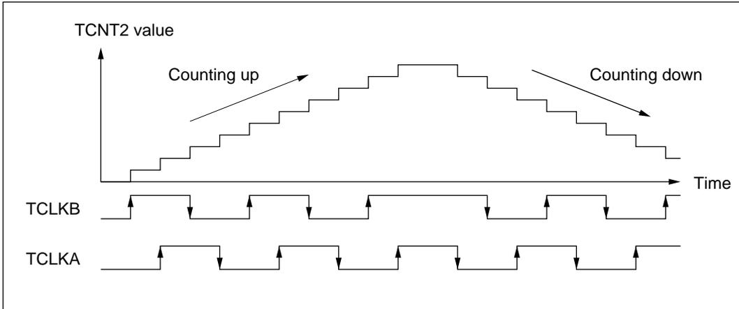
**Figure 8-44 Operation in Phase Counting Mode (Example)**
