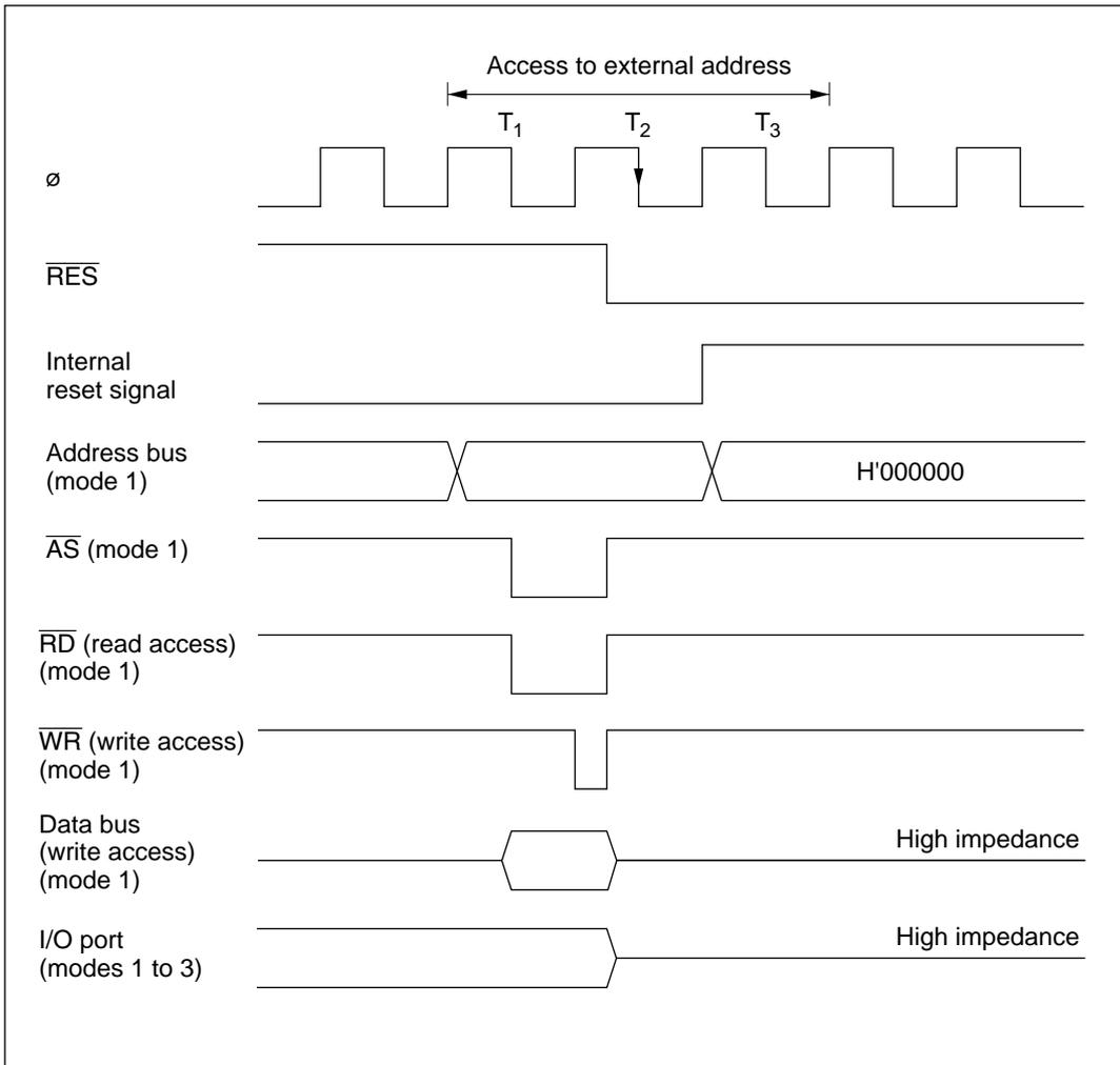
**Figure D-2 Reset during Memory Access (Reset during T<sub>2</sub> State)**
