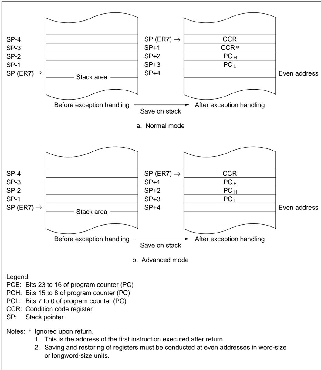
**Figure 4-5 Stack after Completion of Exception Handling**
