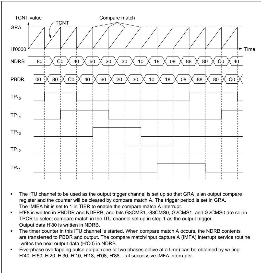
**Figure 9-5 Normal TPC Output Example (Five-Phase Pulse Output)**
