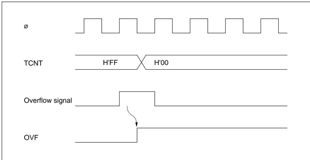
**Figure 10-6 Timing of Setting of OVF**
