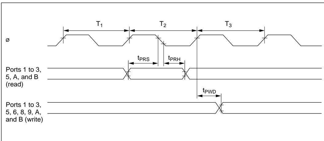
**Figure 17-11 TPC and I/O Port Input/Output Timing**
