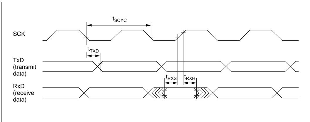
**Figure 17-15 SCI Input/Output Timing in Synchronous Mode**
