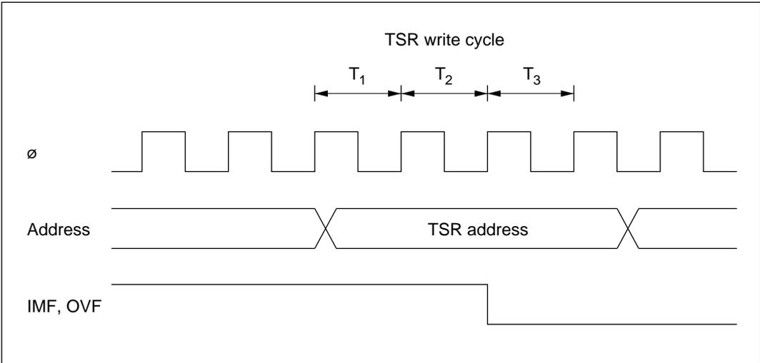
**Figure 8-60 Timing of Clearing of Status Flags**
