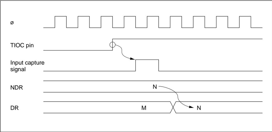
**Figure 9-8 TPC Output Triggering by Input Capture (Example)**
