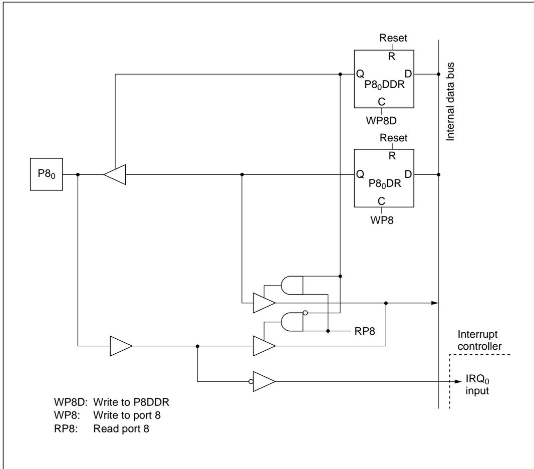
Figure C-7 Port 8 Block Diagram (Pin P80)
