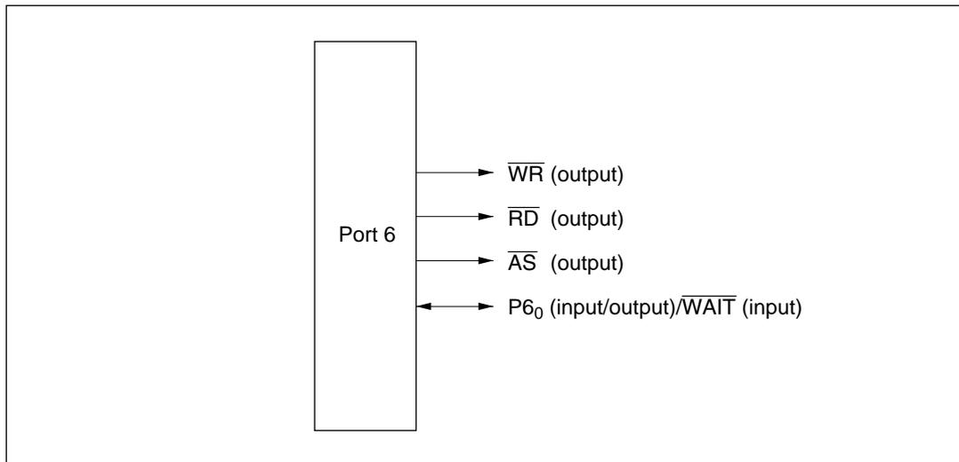
**Figure 7-14 Pin Functions in Mode 1 (Port 6)**
