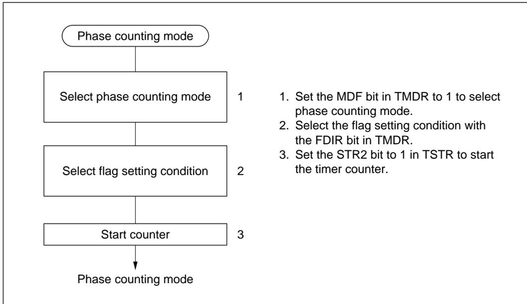
**Figure 8-43 Setup Procedure for Phase Counting Mode (Example)**
