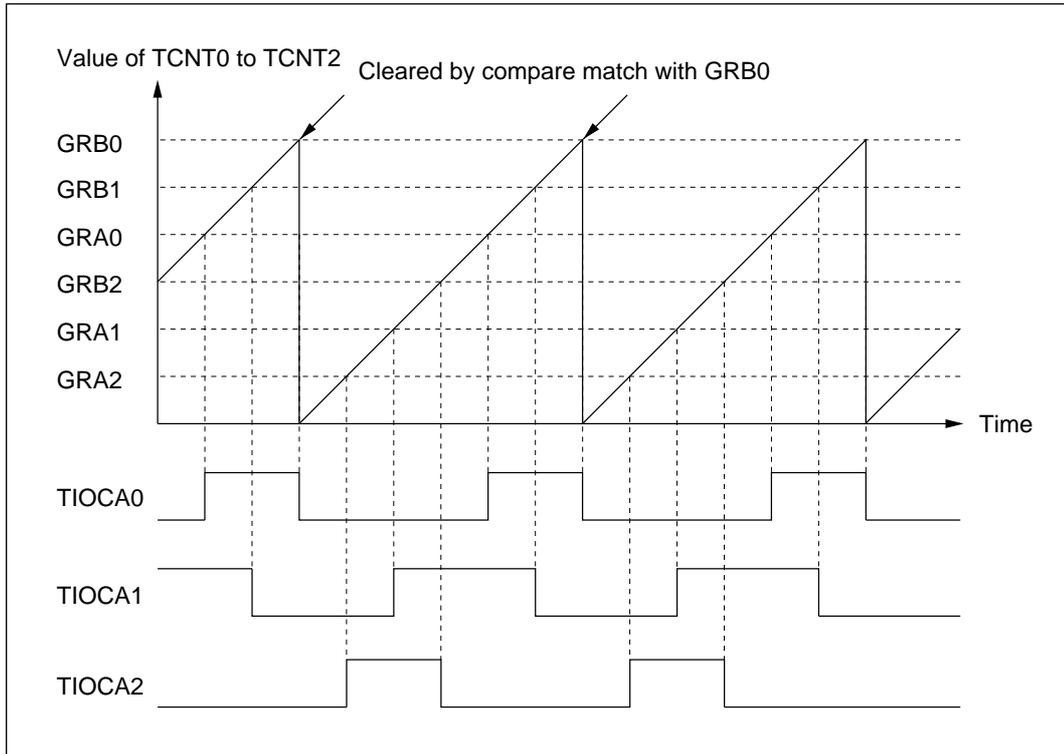
**Figure 8-27 Synchronization (Example)**
