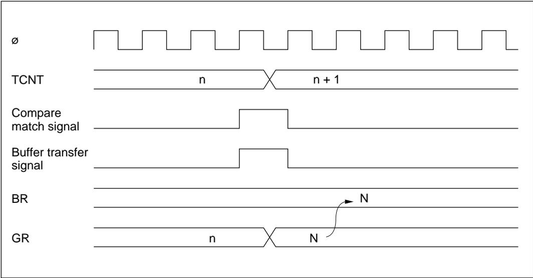
**Figure 8-50 Compare Match and Buffer Transfer Timing (Example)**
