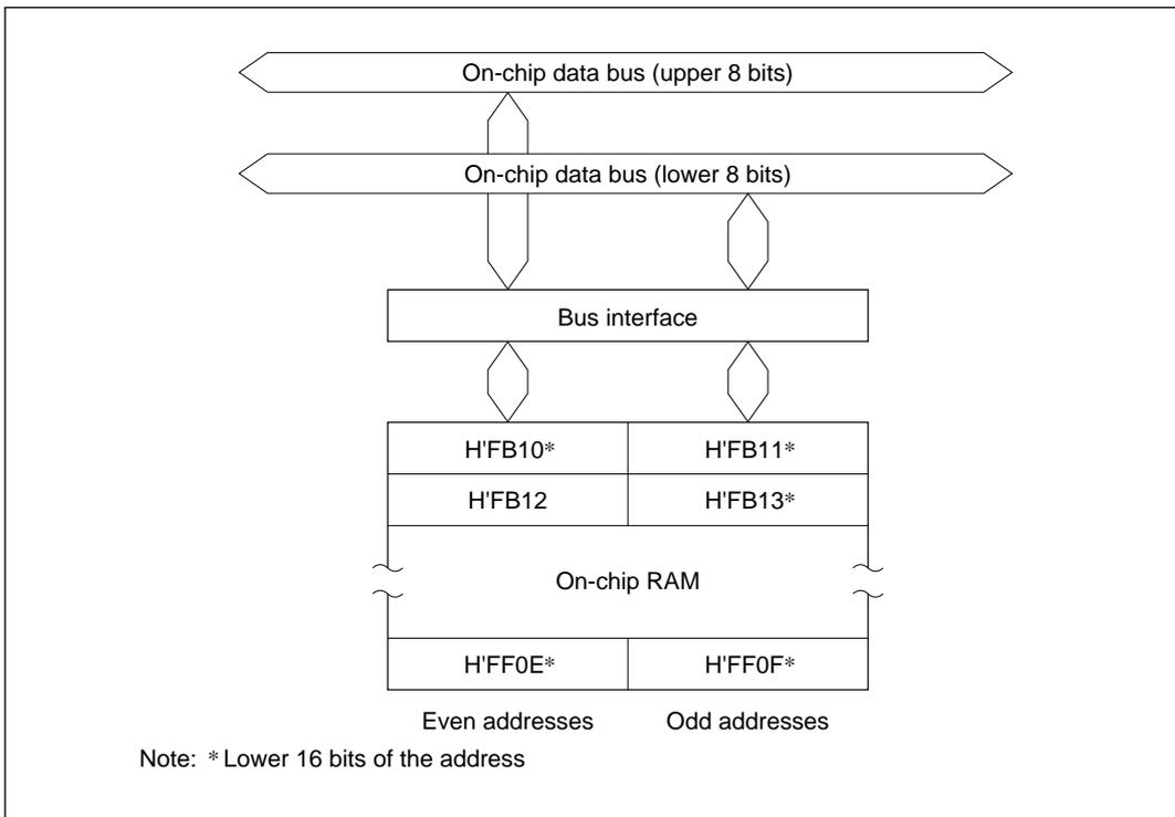
**Figure 13-1 RAM Block Diagram (H8/3031 in Mode 2)**
