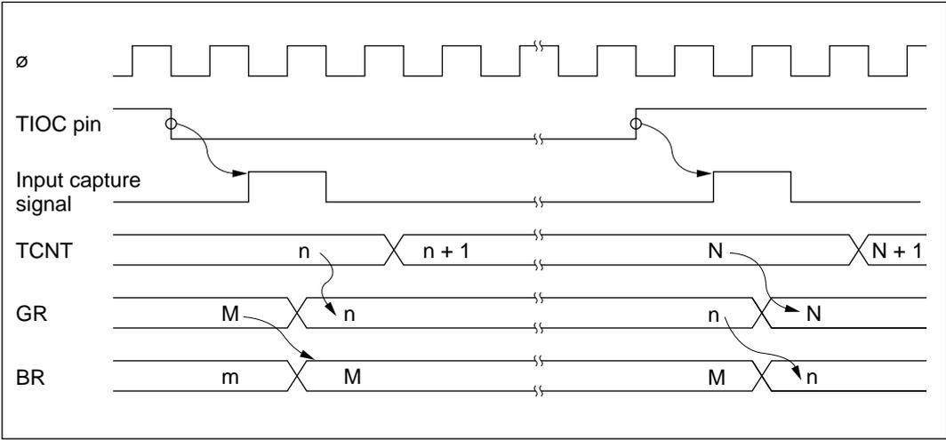
**Figure 8-52 Input Capture and Buffer Transfer Timing (Example)**
