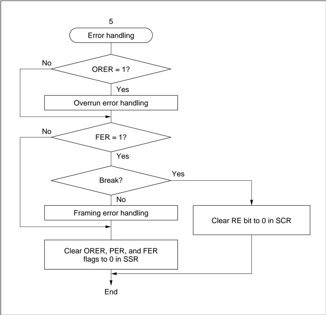
**Figure 11-12 Sample Flowchart for Receiving Multiprocessor Serial Data (2)**
