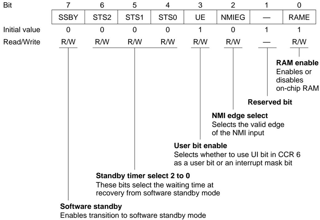
**Bit 7—Software Standby (SSBY):** Enables transition to software standby mode. (For further information about software standby mode see section 16, Power-Down State.)
