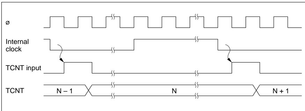
**Figure 8-17 Count Timing for Internal Clock Sources**
