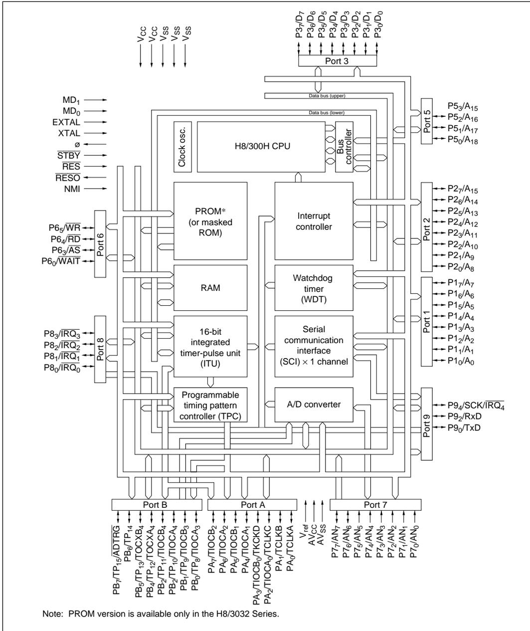
Figure 1-1 Block Diagram
