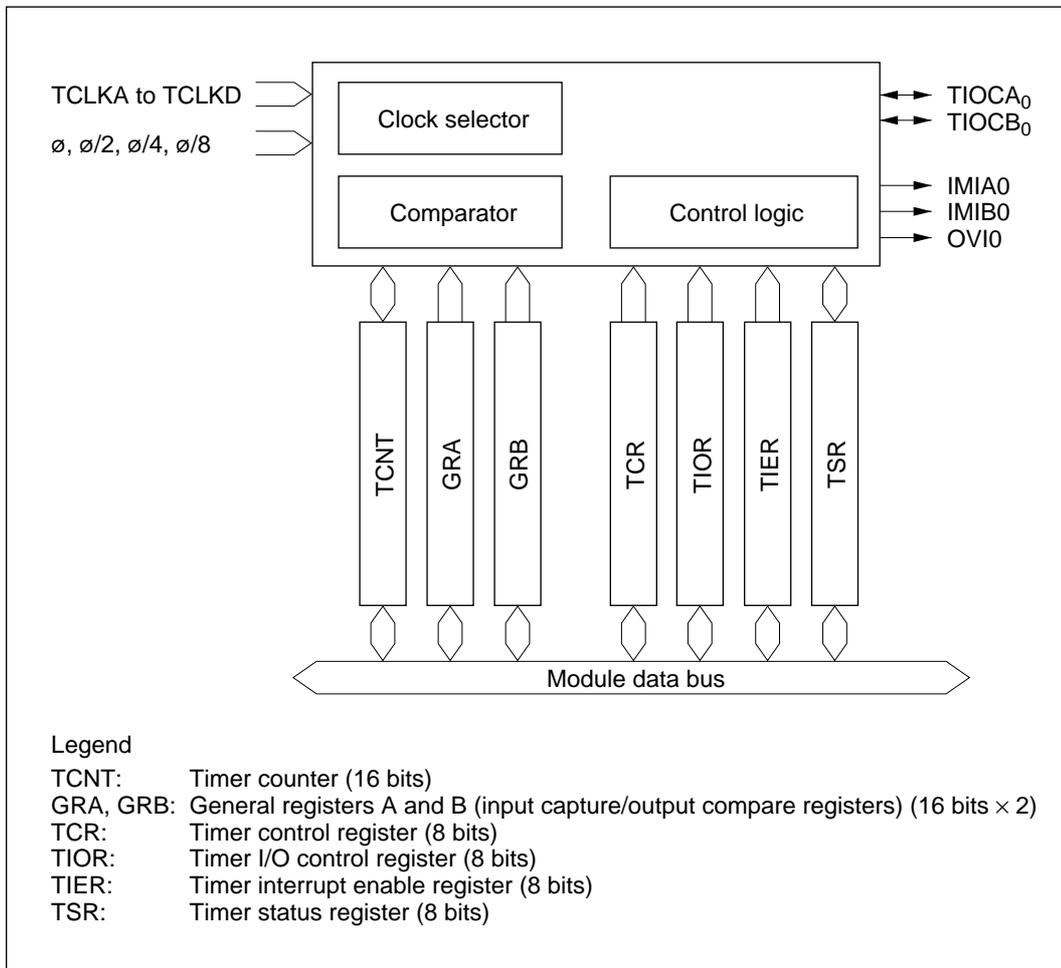
**Figure 8-2 Block Diagram of Channels 0 and 1 (for Channel 0)**
