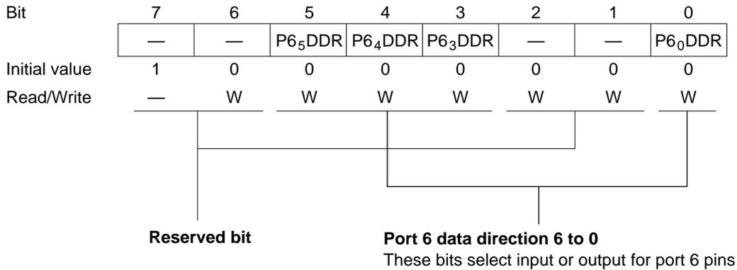
**Mode 1:** Pins P6<sub>5</sub> to P6<sub>3</sub> function as bus control output pins ( $\overline{WR}$ ,  $\overline{RD}$ ,  $\overline{AS}$ ). P6<sub>0</sub> functions as an input/output pin. When P6<sub>0</sub>DDR is set to 1, P6<sub>0</sub> is an output pin, and when P6<sub>0</sub>DDR is 0, P6<sub>0</sub> is an input pin. The P6<sub>5</sub>DDR to P6<sub>3</sub>DDR bit settings are ignored.
