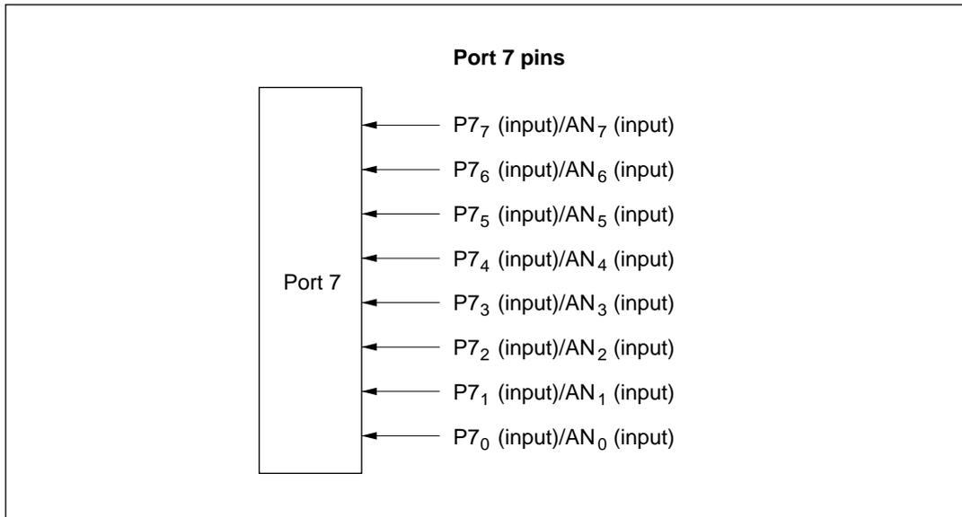
**Figure 7-16 Port 7 Pin Configuration**
