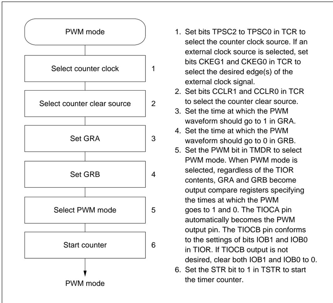
**Figure 8-28 Setup Procedure for PWM Mode (Example)**
