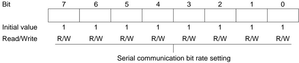
**SCR—Serial Control Register**
