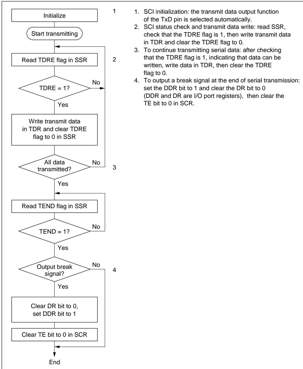
1. SCI initialization: the transmit data output function of the TxD pin is selected automatically.
