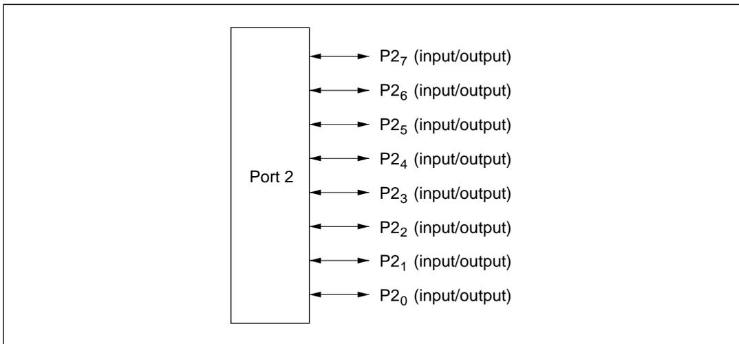
**Figure 7-6 Pin Functions in Modes 2 and 3 (Port 2)**
