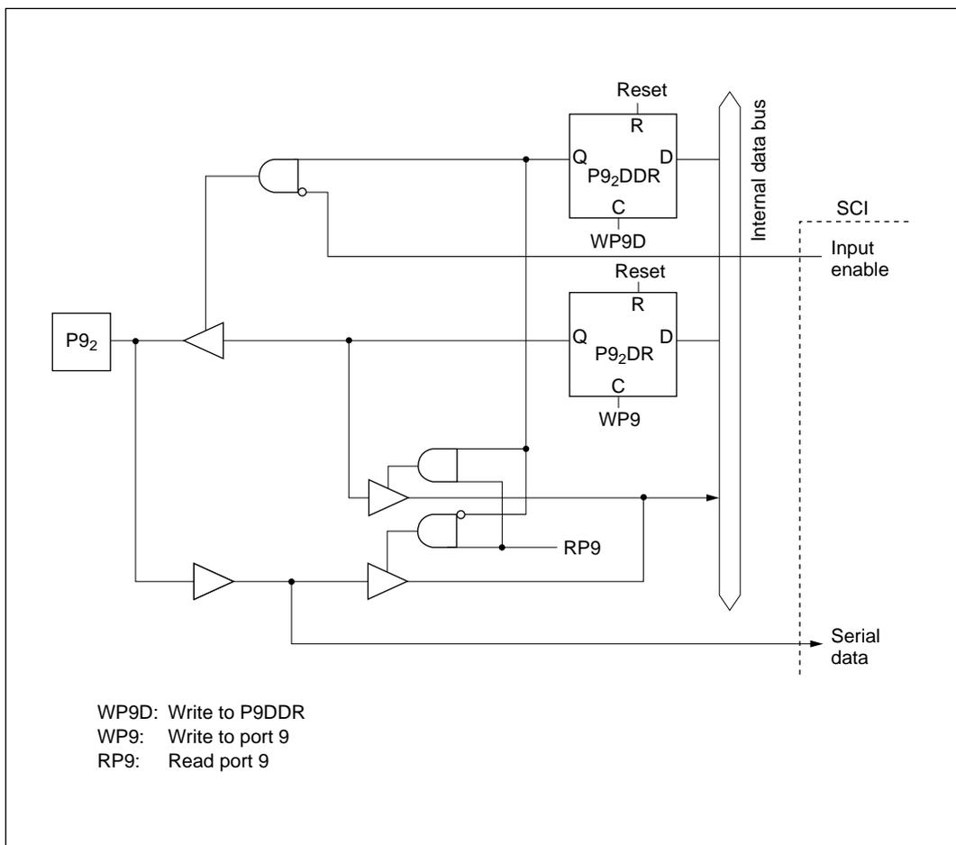
**Figure C-8 (b) Port 9 Block Diagram (Pins P9<sub>2</sub>, P9<sub>3</sub>)**
