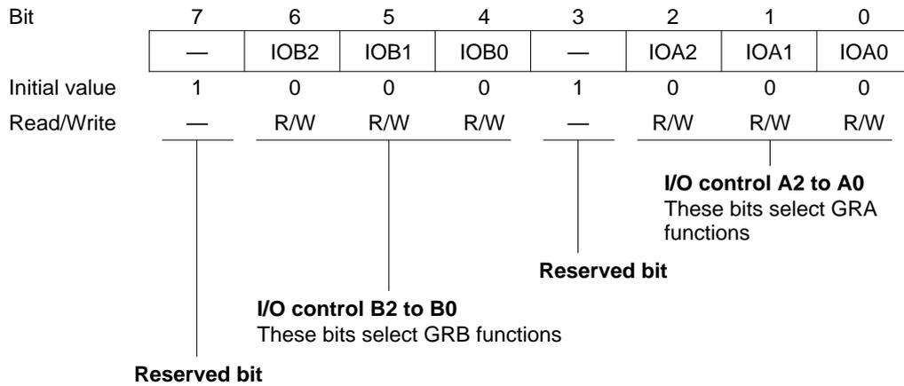
Each TIOR is an 8-bit readable/writable register that selects the output compare or input capture function for GRA and GRB, and specifies the functions of the TIOCA and TIOCB pins. If the output compare function is selected, TIOR also selects the type of output. If input capture is selected, TIOR also selects the edge or edges of the input capture signal.
