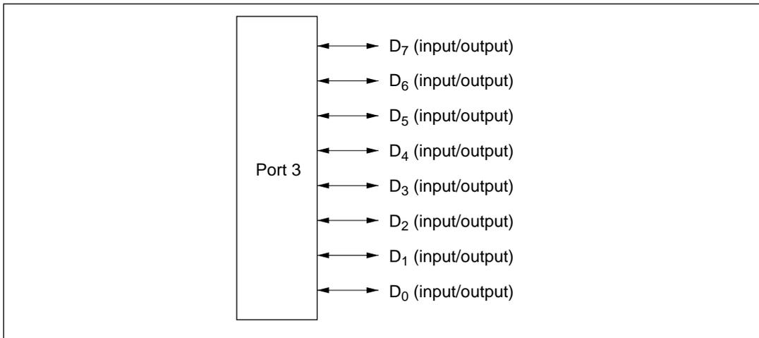
**Figure 7-8 Pin Functions in Mode 1 (Port 3)**
