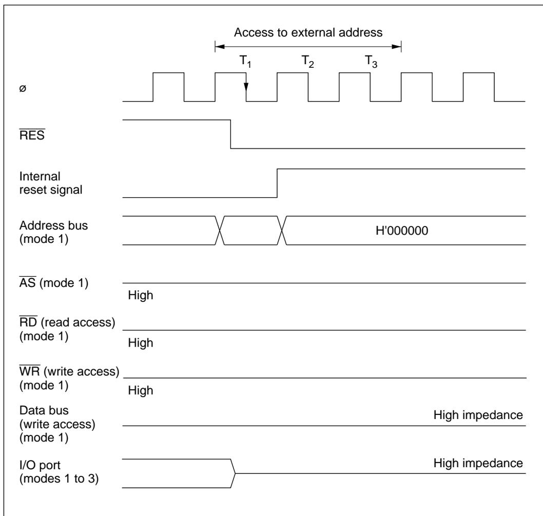
Figure D-1 Reset during Memory Access (Reset during T<sub>1</sub> State)
