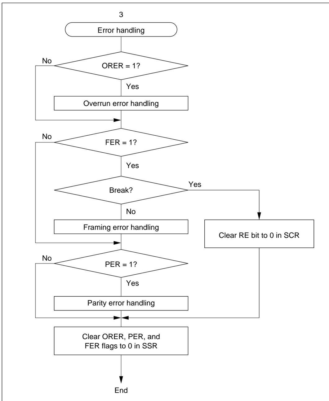
Figure 11-7 Sample Flowchart for Receiving Serial Data (2)
