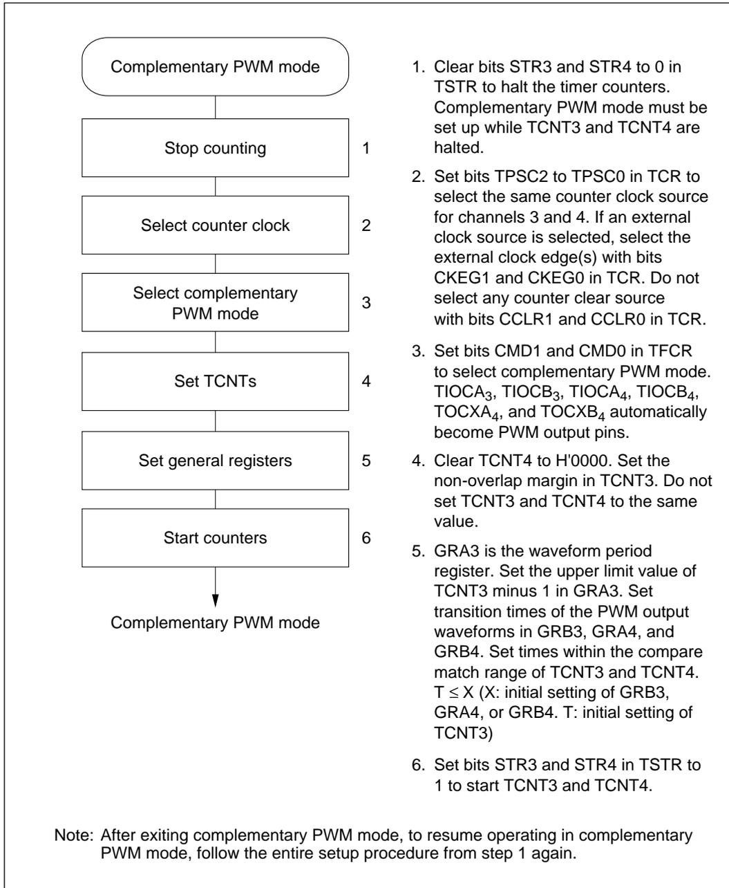
**Figure 8-33 Setup Procedure for Complementary PWM Mode (Example)**
