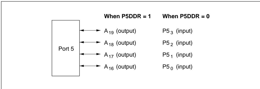
**Figure 7-11 Pin Functions in Mode 1 (Port 5)**
