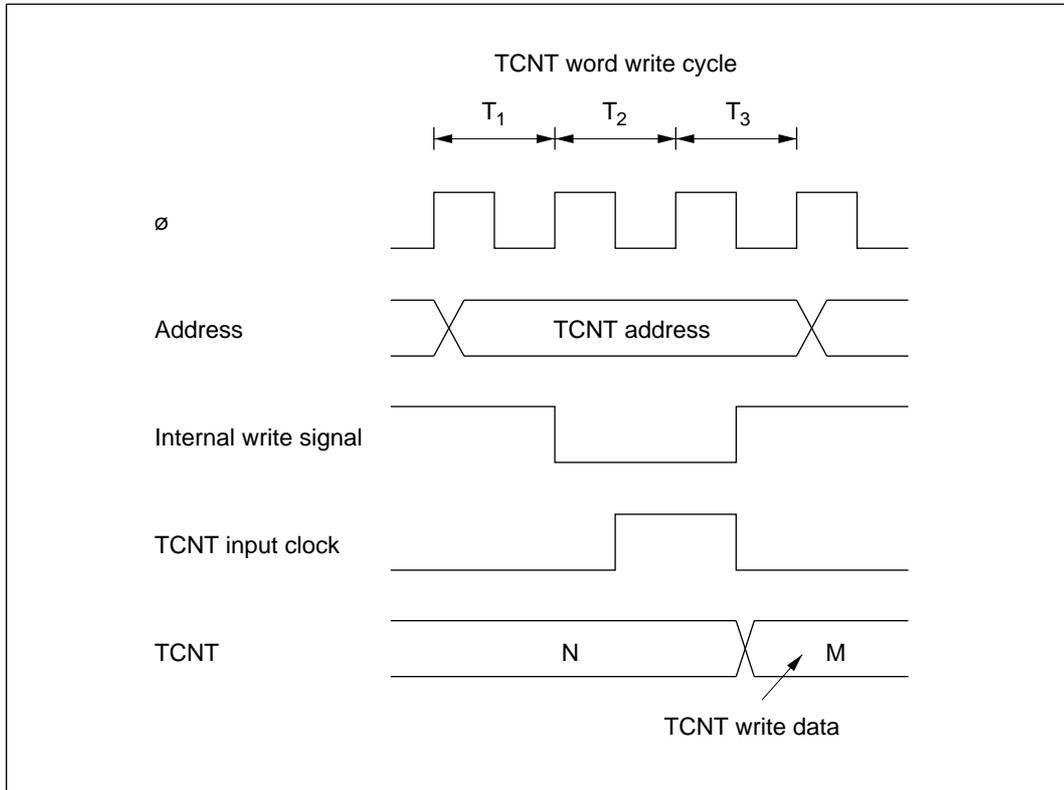
**Figure 8-62 Contention between TCNT Word Write and Increment**
