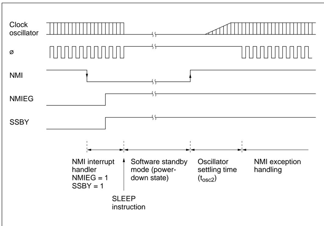
**Figure 16-1 NMI Timing for Software Standby Mode (Example)**
