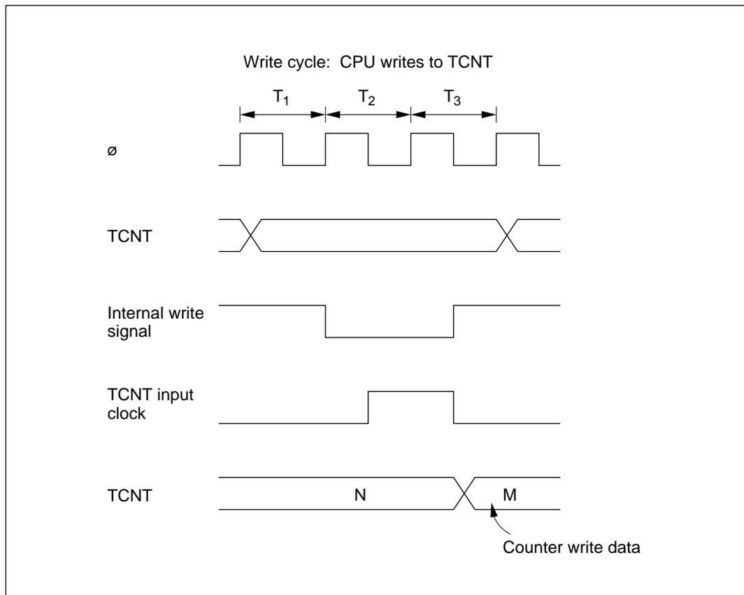
Figure 10-8 Contention between TCNT Write and Increment
