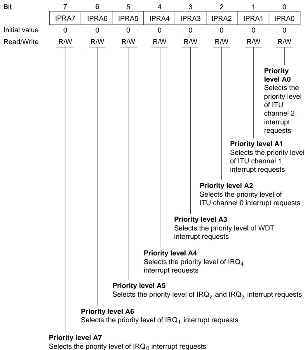
IPRA is initialized to H'00 by a reset and in hardware standby mode.
