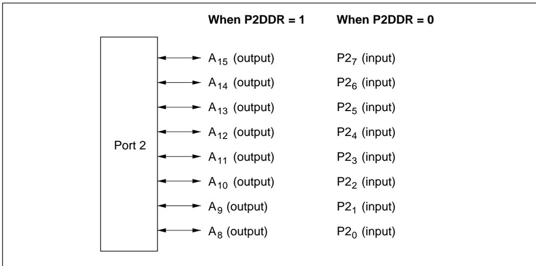
**Figure 7-5 Pin Functions in Mode 1 (Port 2)**
