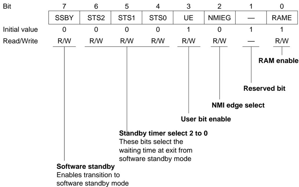
SYSCR is an 8-bit readable/writable register. Bit 7 (SSBY) and bits 6 to 4 (STS2 to STS0) control the power-down state. For information on the other SYSCR bits, see section 3.3, System Control Register.
