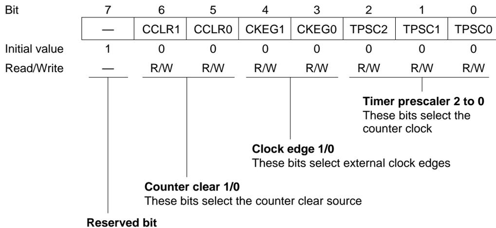
Each TCR is an 8-bit readable/writable register that selects the timer counter clock source, selects the edge or edges of external clock sources, and selects how the counter is cleared.
