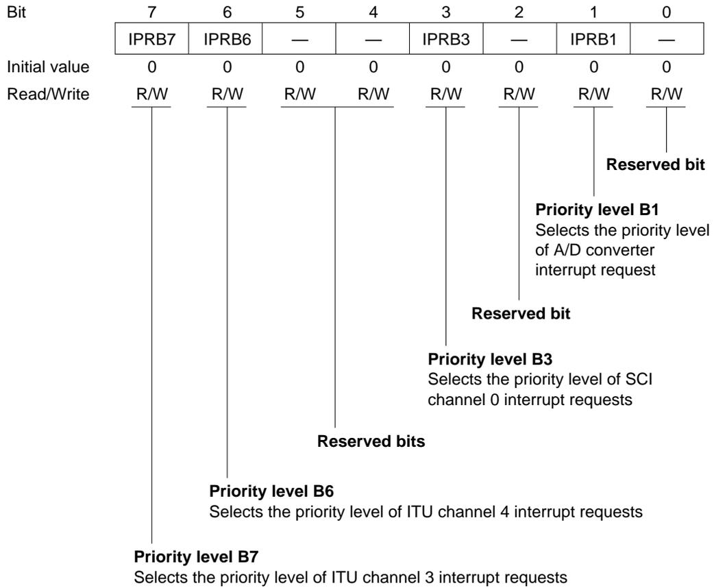
IPRB is initialized to H'00 by a reset and in hardware standby mode.
