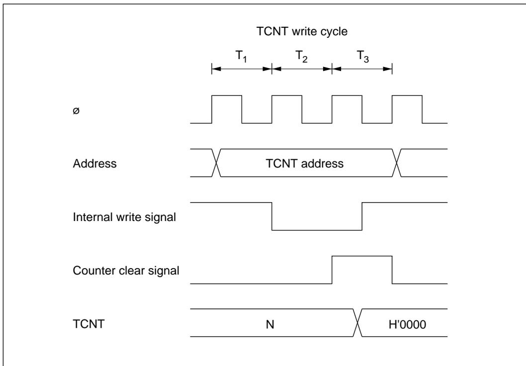
Figure 8-61 Contention between TCNT Write and Clear
