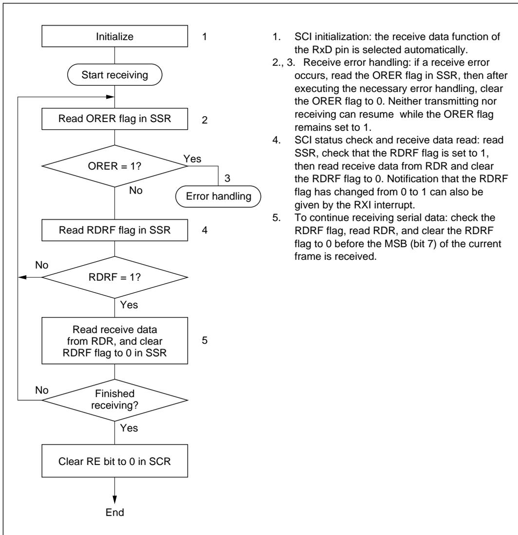
1. SCI initialization: the receive data function of the RxD pin is selected automatically.
