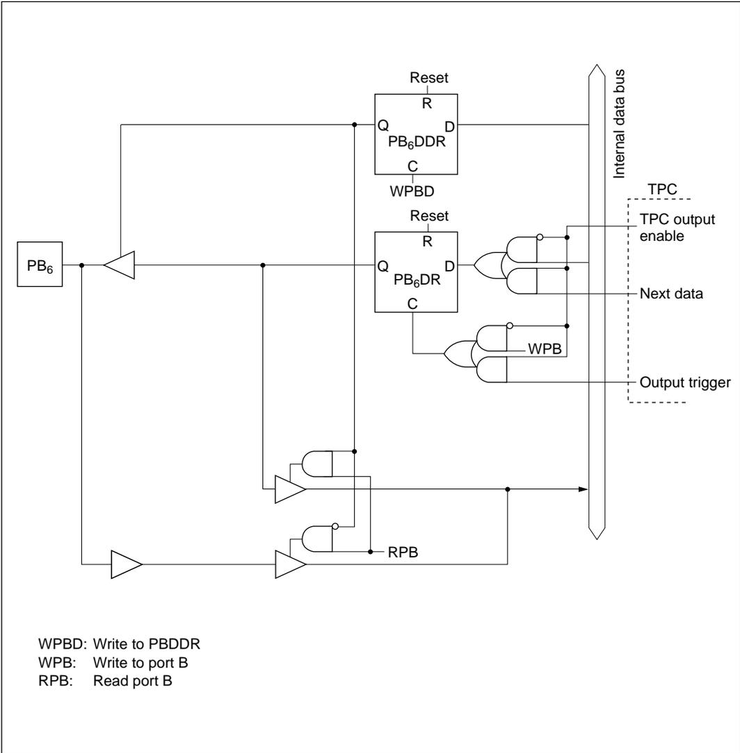
Figure C-10 (c) Port B Block Diagram (Pin PB<sub>6</sub>)
