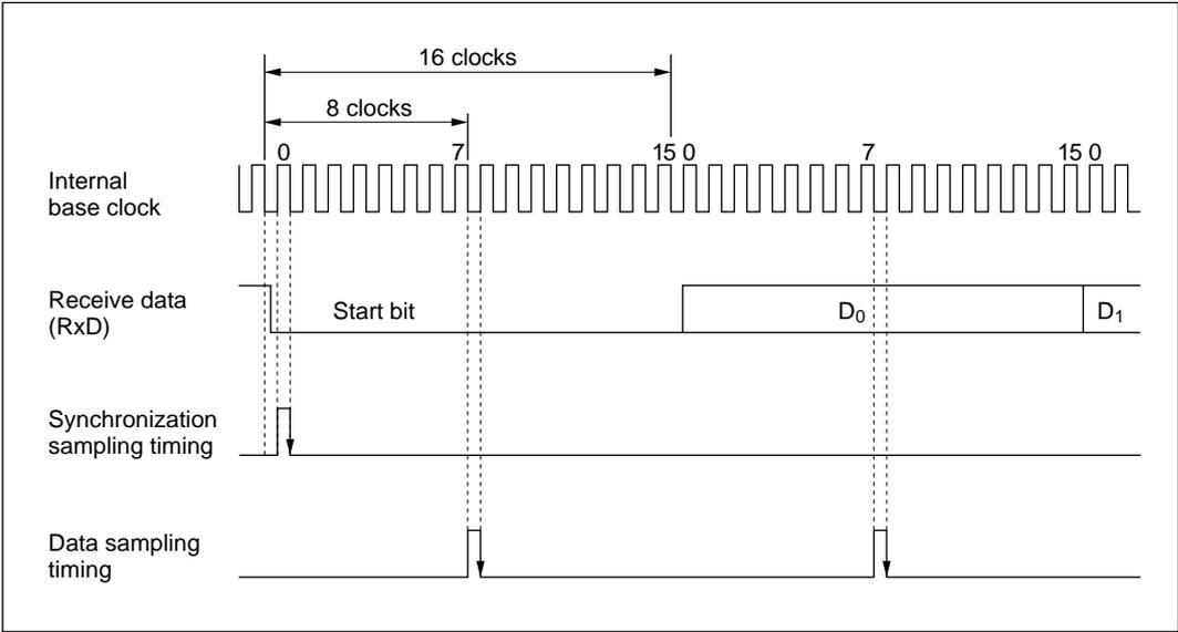
**Figure 11-21 Receive Data Sampling Timing in Asynchronous Mode**
