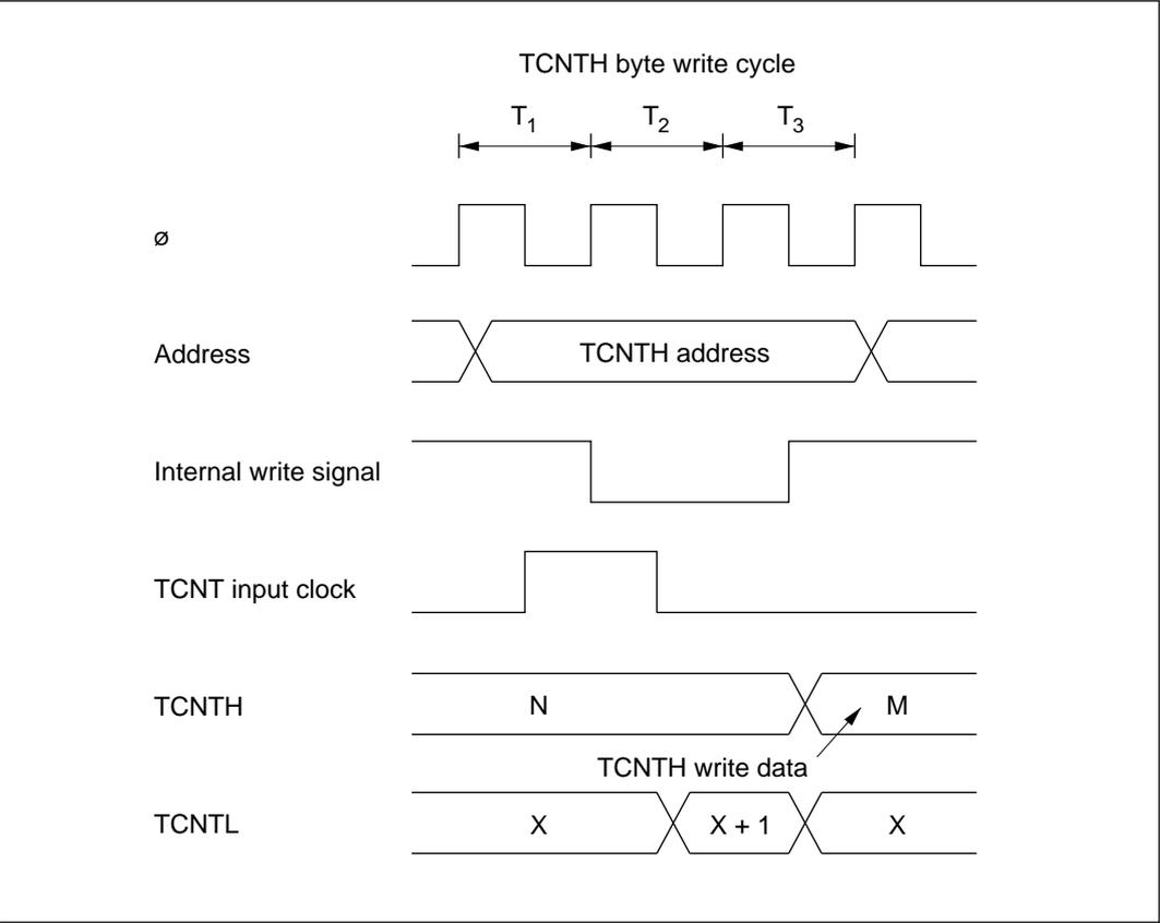
**Figure 8-63 Contention between TCNT Byte Write and Increment**
