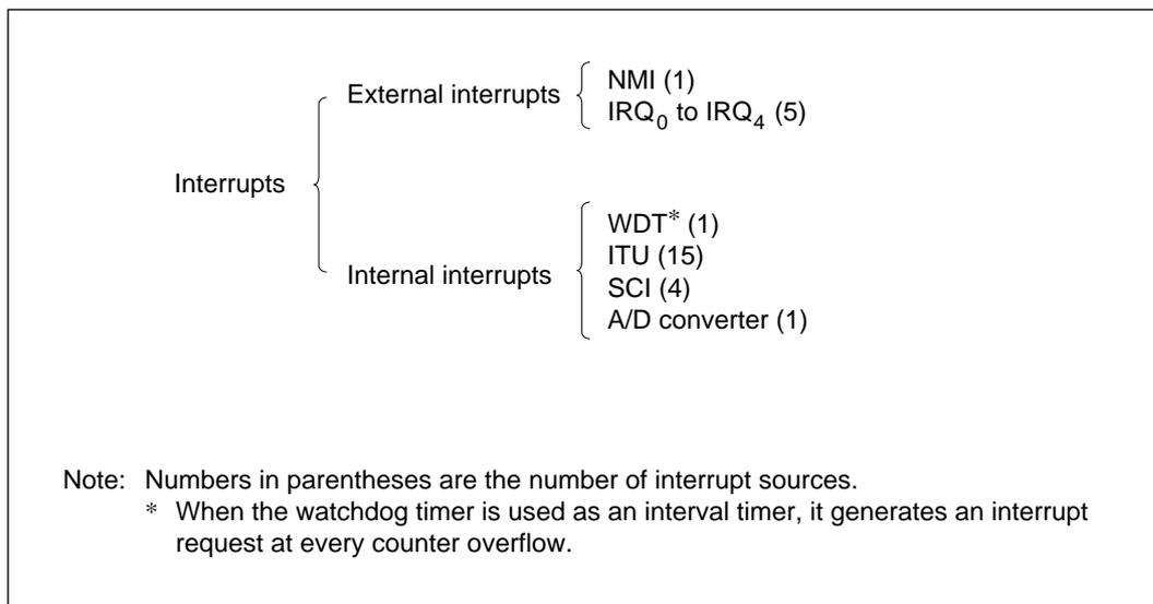
**Figure 4-4 Interrupt Sources and Number of Interrupts**
