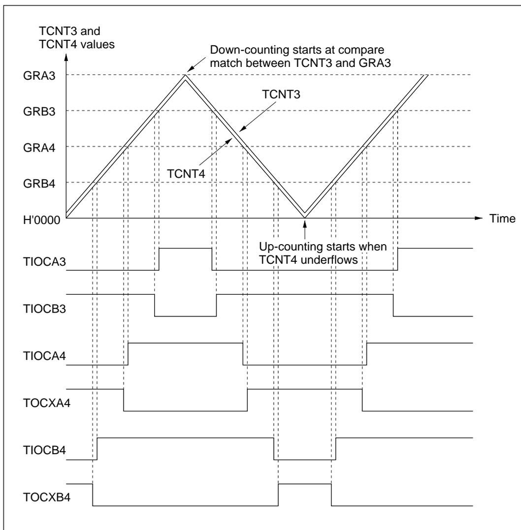
**Figure 8-35 Operation in Complementary PWM Mode (Example 1)**
