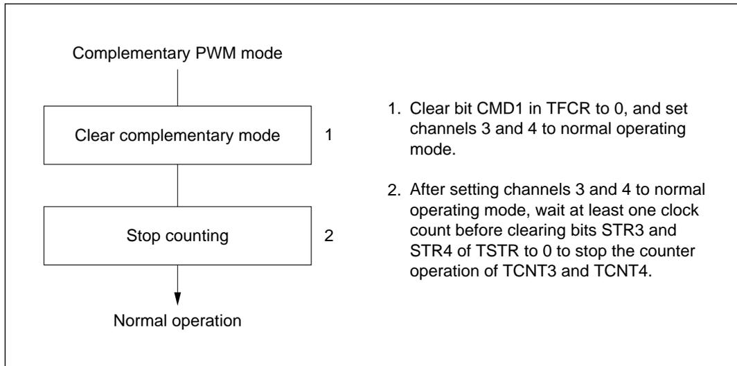
**Figure 8-34 Clearing Procedure for Complementary PWM Mode (Example)**
