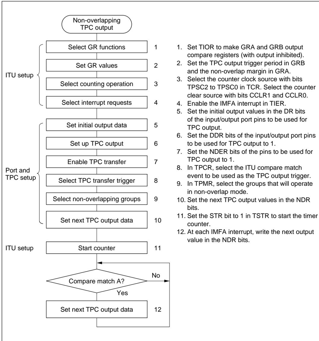
**Figure 9-6 Setup Procedure for Non-Overlapping TPC Output (Example)**
