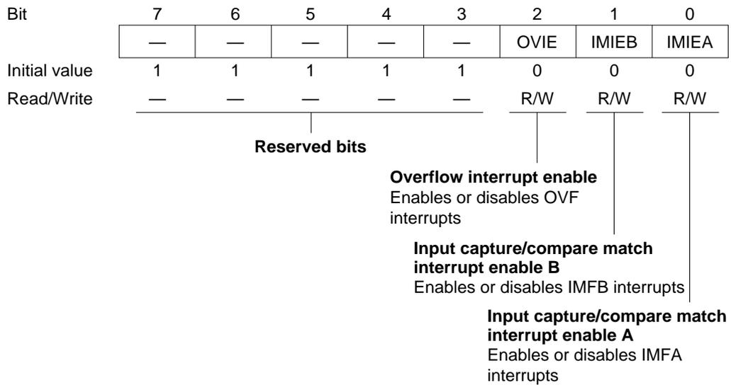
Each TIER is an 8-bit readable/writable register that enables and disables overflow interrupt requests and general register compare match and input capture interrupt requests.
