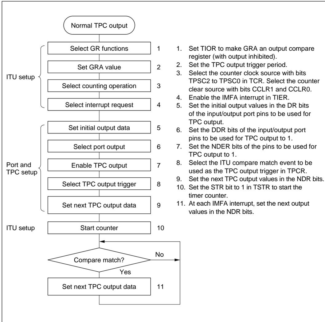
**Figure 9-4 Setup Procedure for Normal TPC Output (Example)**
