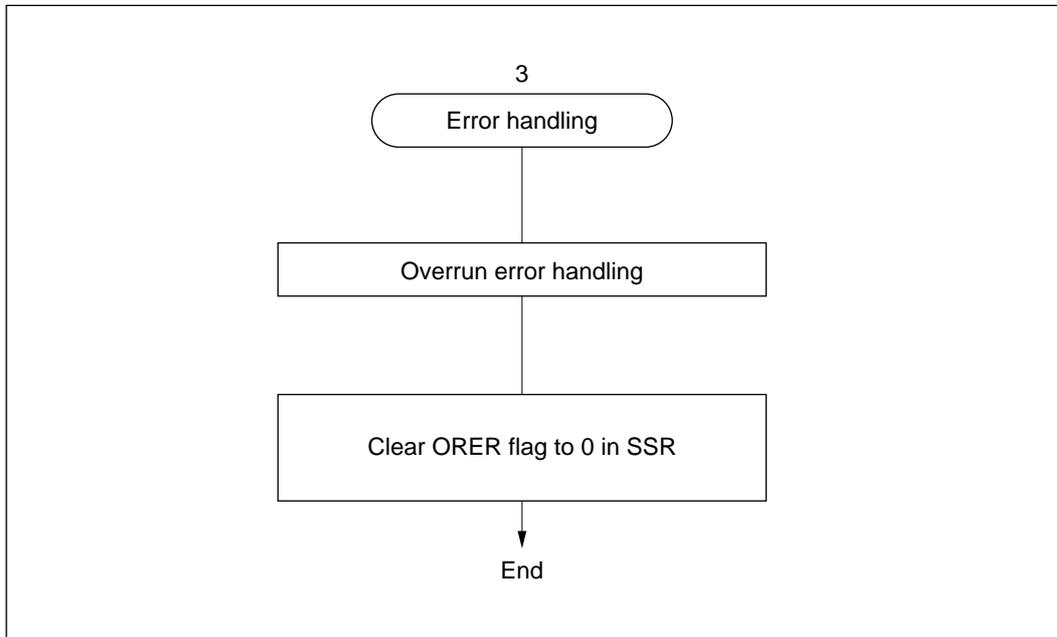
**Figure 11-18 Sample Flowchart for Serial Receiving (2)**
