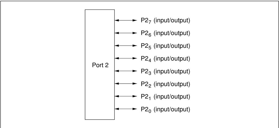
**Figure 9-8 Pin Functions in Modes 6 and 7 (Port 2)**
