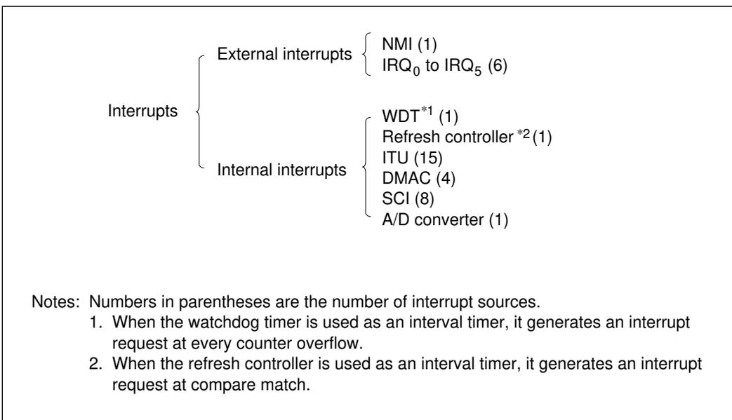
**Figure 4-5 Interrupt Sources and Number of Interrupts**
