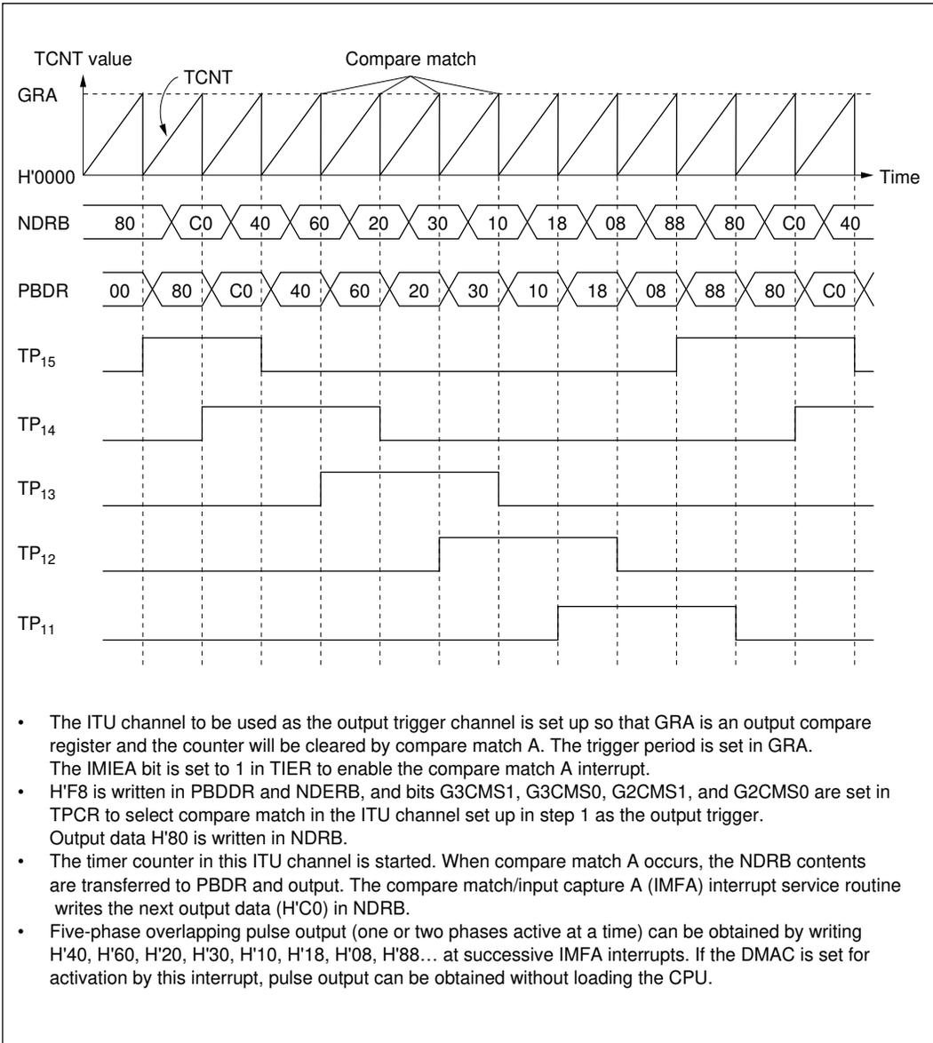
**Figure 11-5 Normal TPC Output Example (Five-Phase Pulse Output)**
