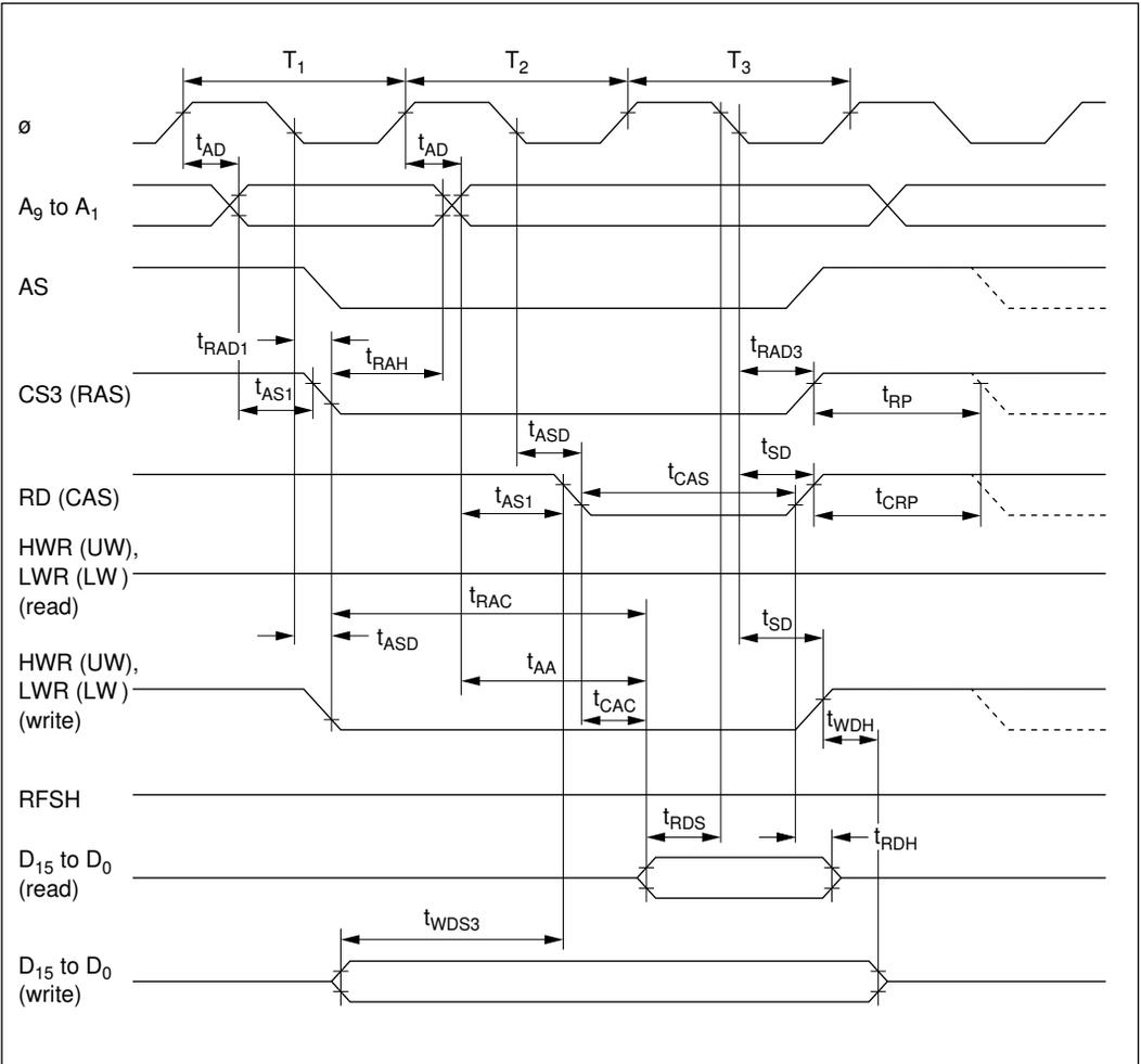
**Figure 20-7 DRAM Bus Timing (Read/Write): Three-State Access**
