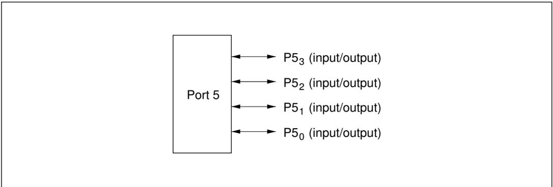
**Figure 9-19 Pin Functions in Modes 6 and 7 (Port 5)**
