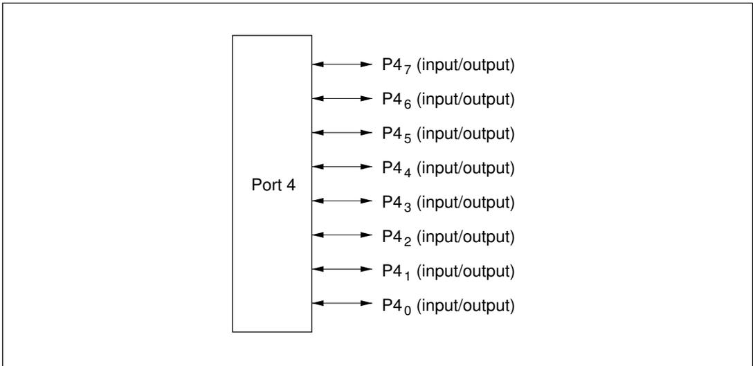
**Figure 9-15 Pin Functions in Modes 6 and 7 (Port 4)**
