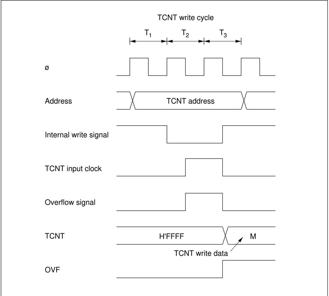
**Figure 10-65 Contention between TCNT Write and Overflow**
