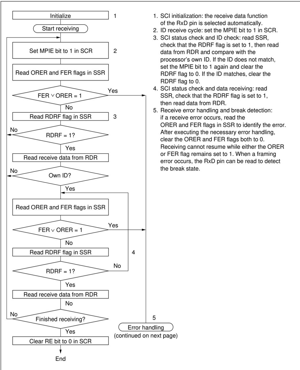
1. SCI initialization: the receive data function of the RxD pin is selected automatically.
