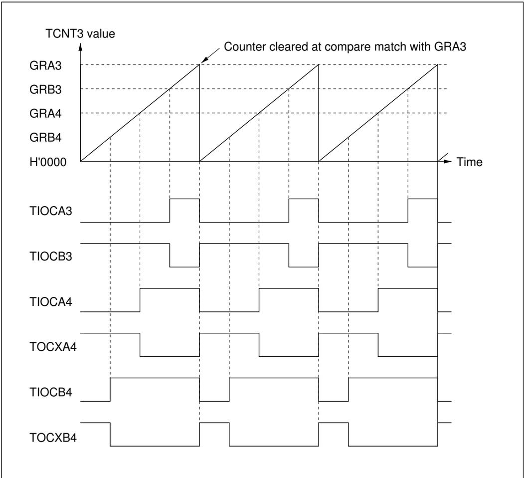
**Figure 10-32 Operation in Reset-Synchronized PWM Mode (Example)**
