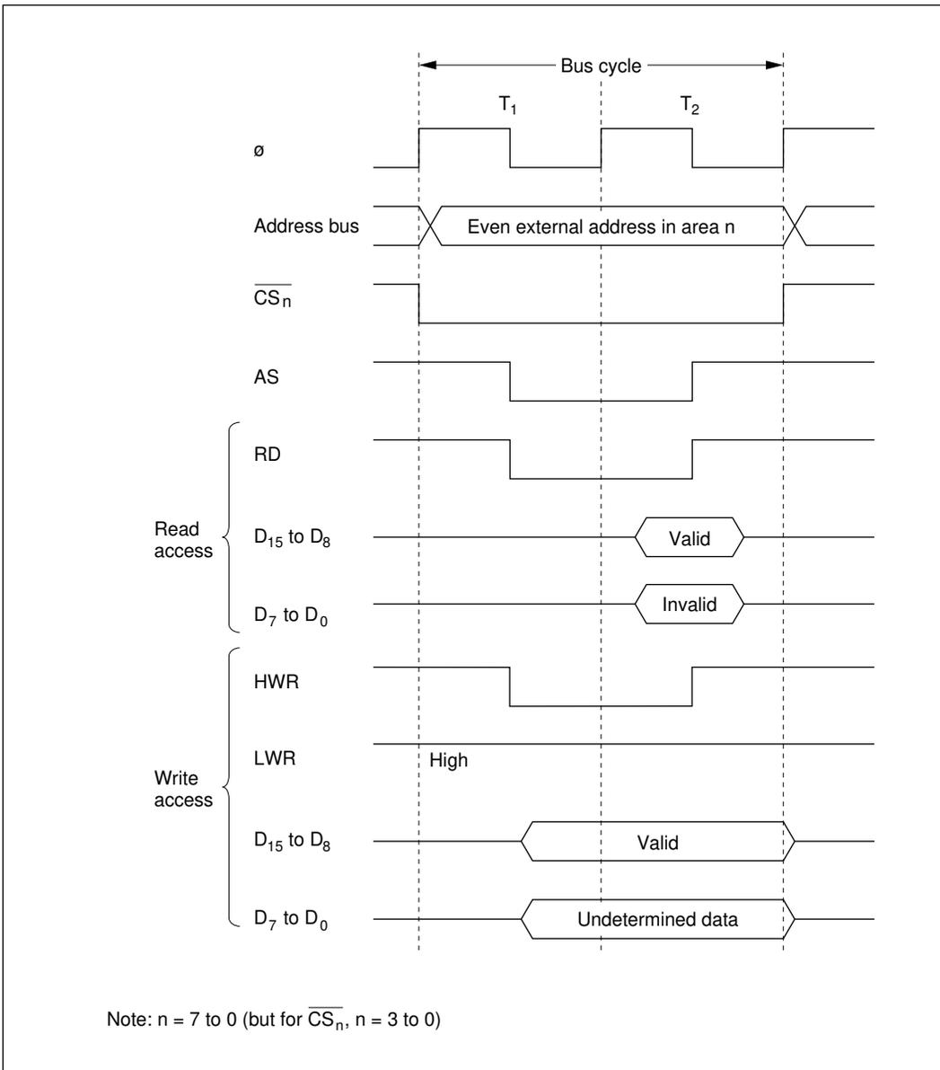
**Figure 6-9 Bus Control Signal Timing for 16-Bit, Two-State-Access Area (1)**
