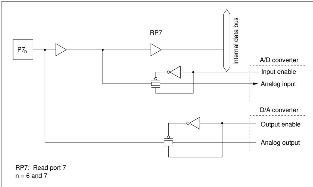
**Figure C-7 (b) Port 7 Block Diagram (Pins P7<sub>6</sub> and P7<sub>7</sub>)**
