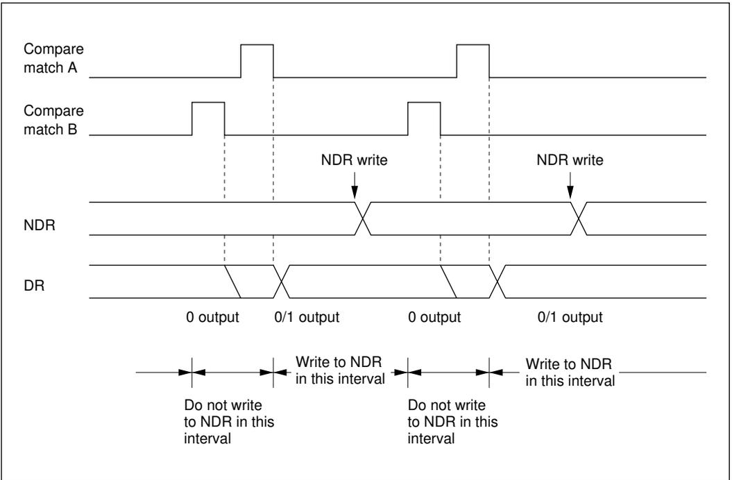
**Figure 11-10 Non-Overlapping Operation and NDR Write Timing**
