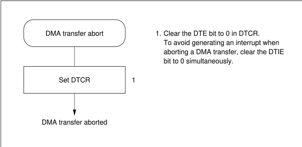
**Figure 8-22 Procedure for Aborting a DMA Transfer**
