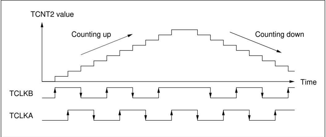
**Figure 10-44 Operation in Phase Counting Mode (Example)**
