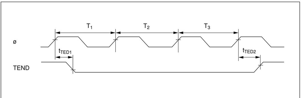
**Figure 20-26 DMAC  $\overline{\text{TEND}}$  Output Timing for 3 State Access**
