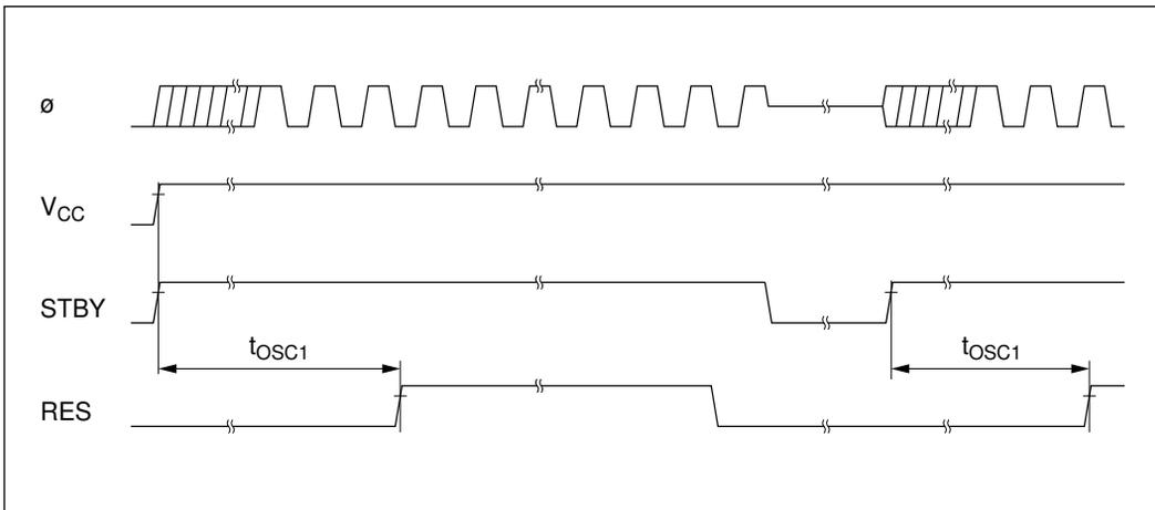
**Figure 20-19 Oscillator Settling Timing**
