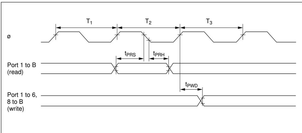
**Figure 20-20 TPC and I/O Port Input/Output Timing**
