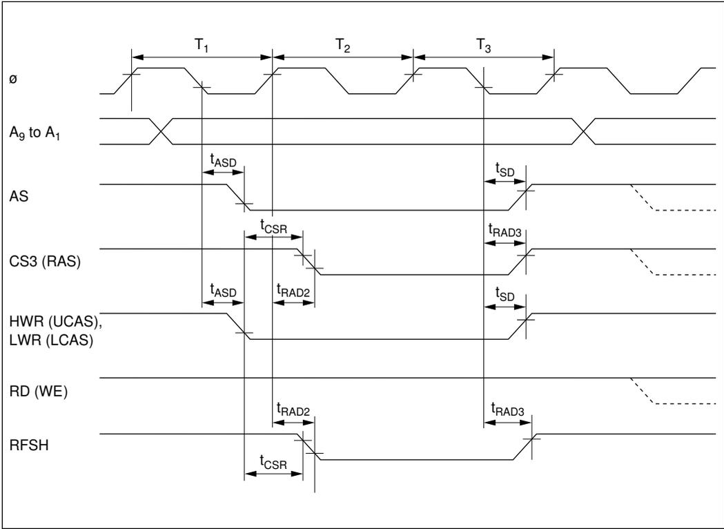
**Figure 20-11 DRAM Bus Timing (Refresh Cycle): Three-State Access**
