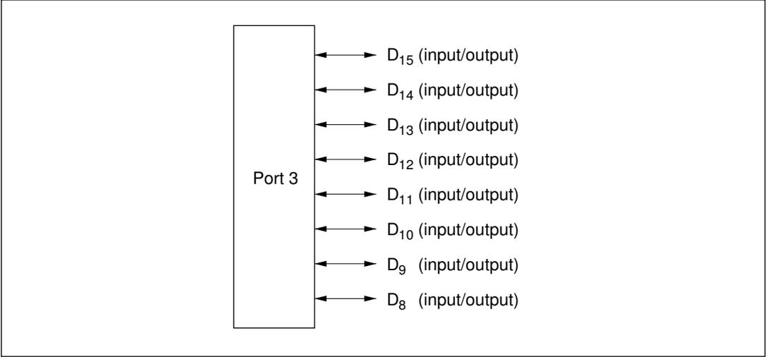
**Figure 9-10 Pin Functions in Modes 1 to 5 (Port 3)**
