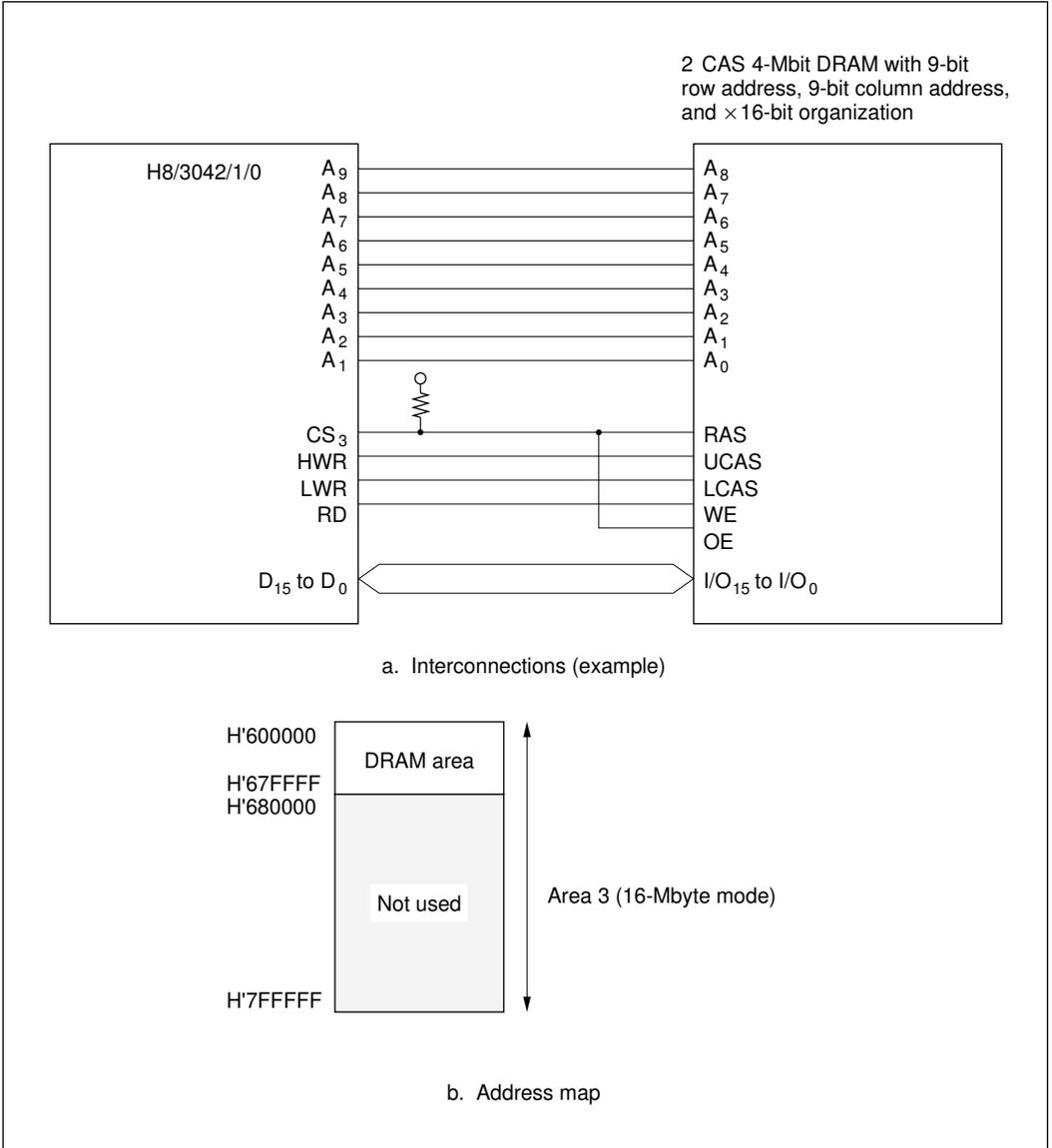
**Figure 7-11 Interconnections and Address Map for  $\overline{2}\text{CAS}$  4-Mbit DRAM (Example)**
