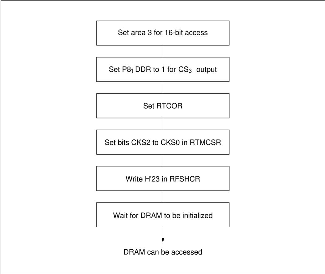
**Figure 7-10 Setup Procedure for  $2\overline{WE}$  4-Mbit DRAM with 10-Bit Row Address and 8-Bit Column Address (16-Mbyte Mode)**
