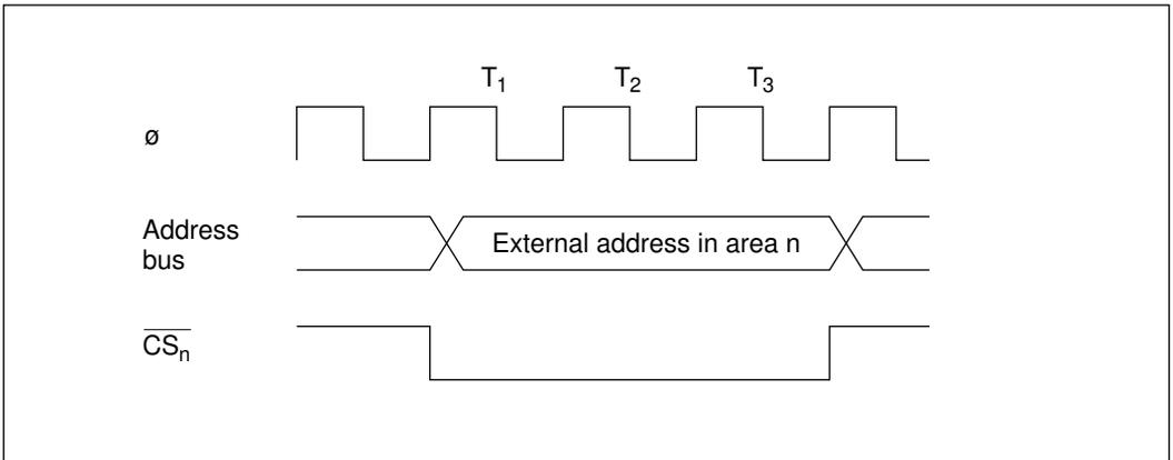
**Figure 6-3  $\overline{CS}_n$  Output Timing ( $n = 0$  to 3)**
