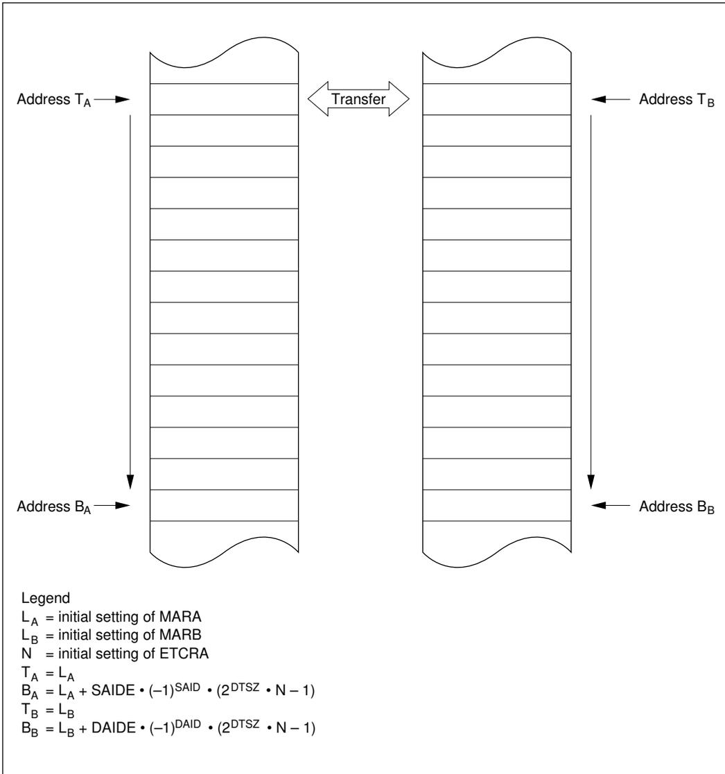
**Figure 8-8 Operation in Normal Mode**
