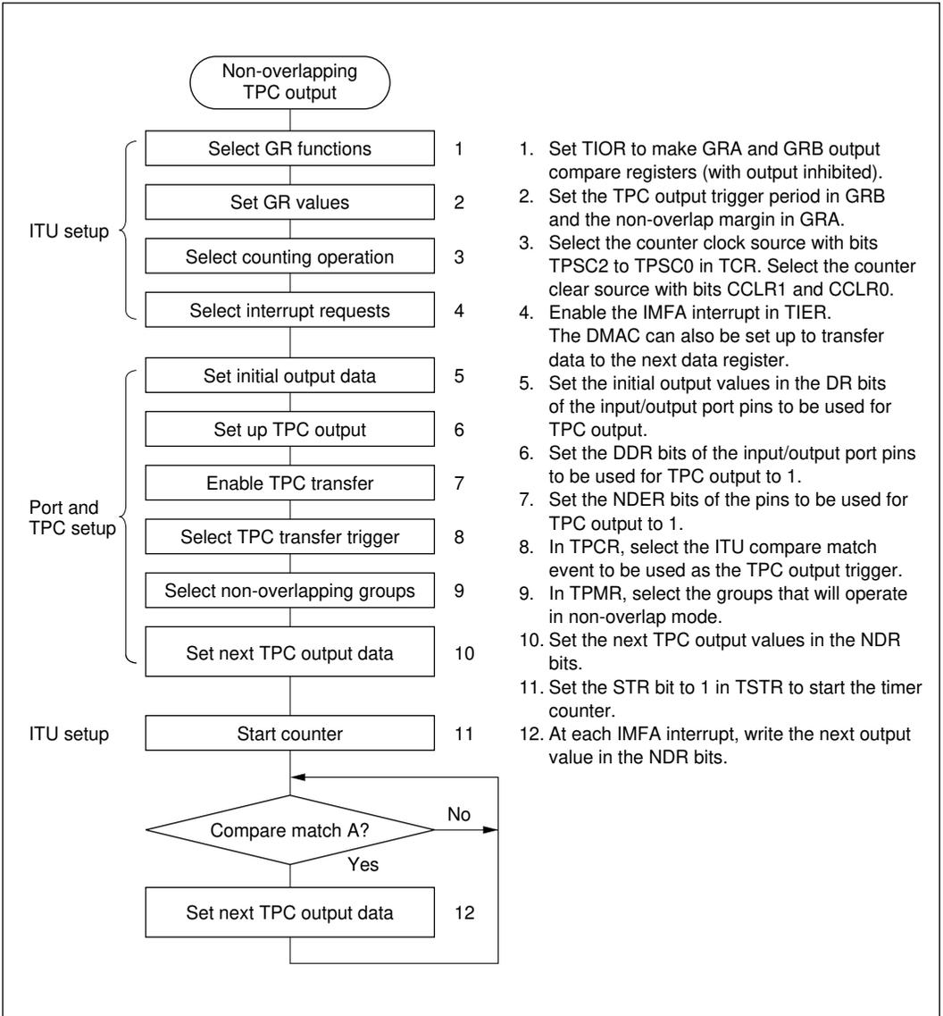
**Figure 11-6 Setup Procedure for Non-Overlapping TPC Output (Example)**
