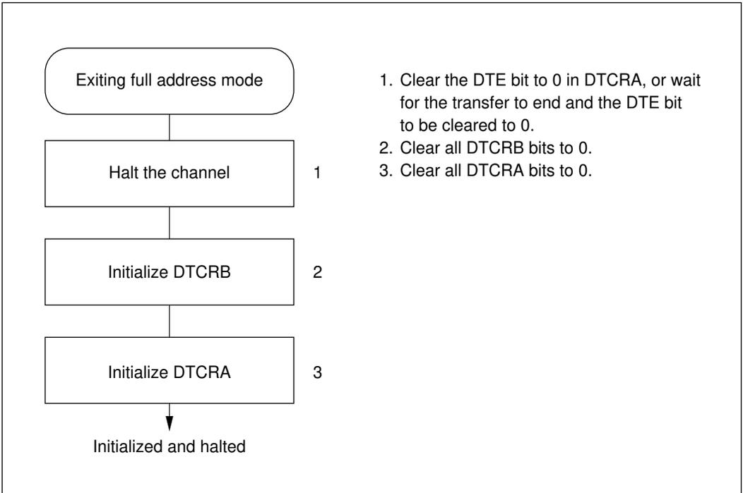
**Figure 8-23 Procedure for Exiting Full Address Mode (Example)**
