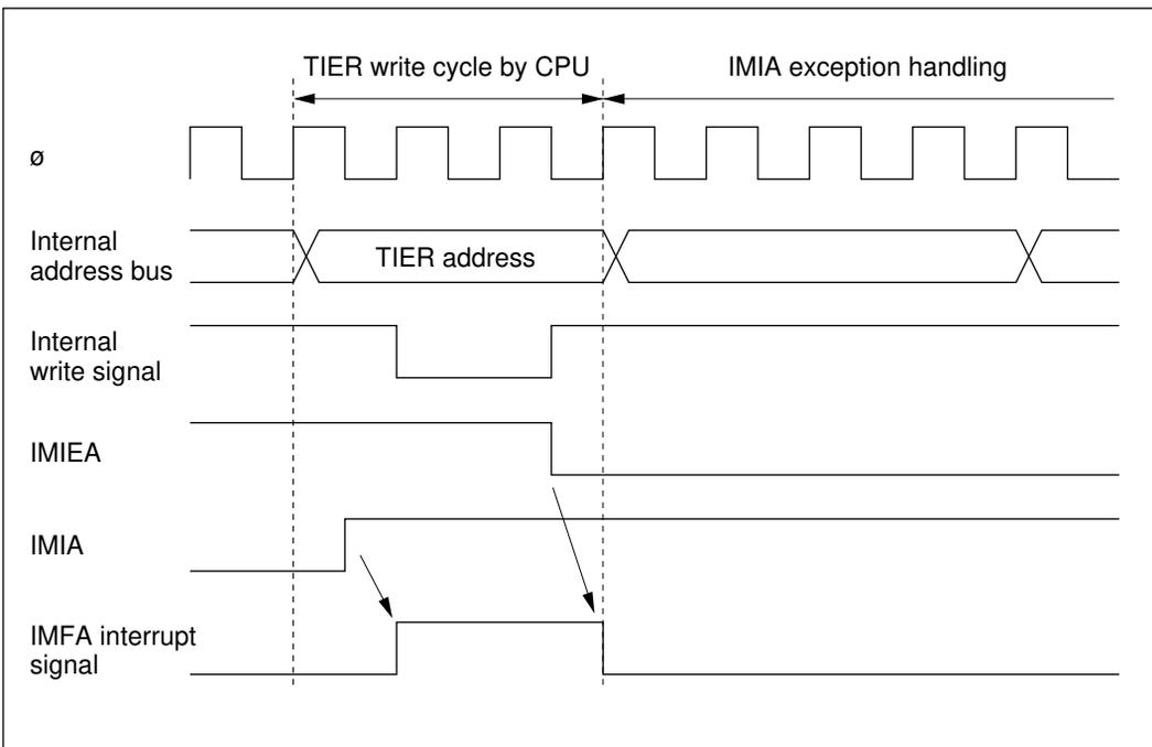
**Figure 5-8 Contention between Interrupt and Interrupt-Disabling Instruction**
