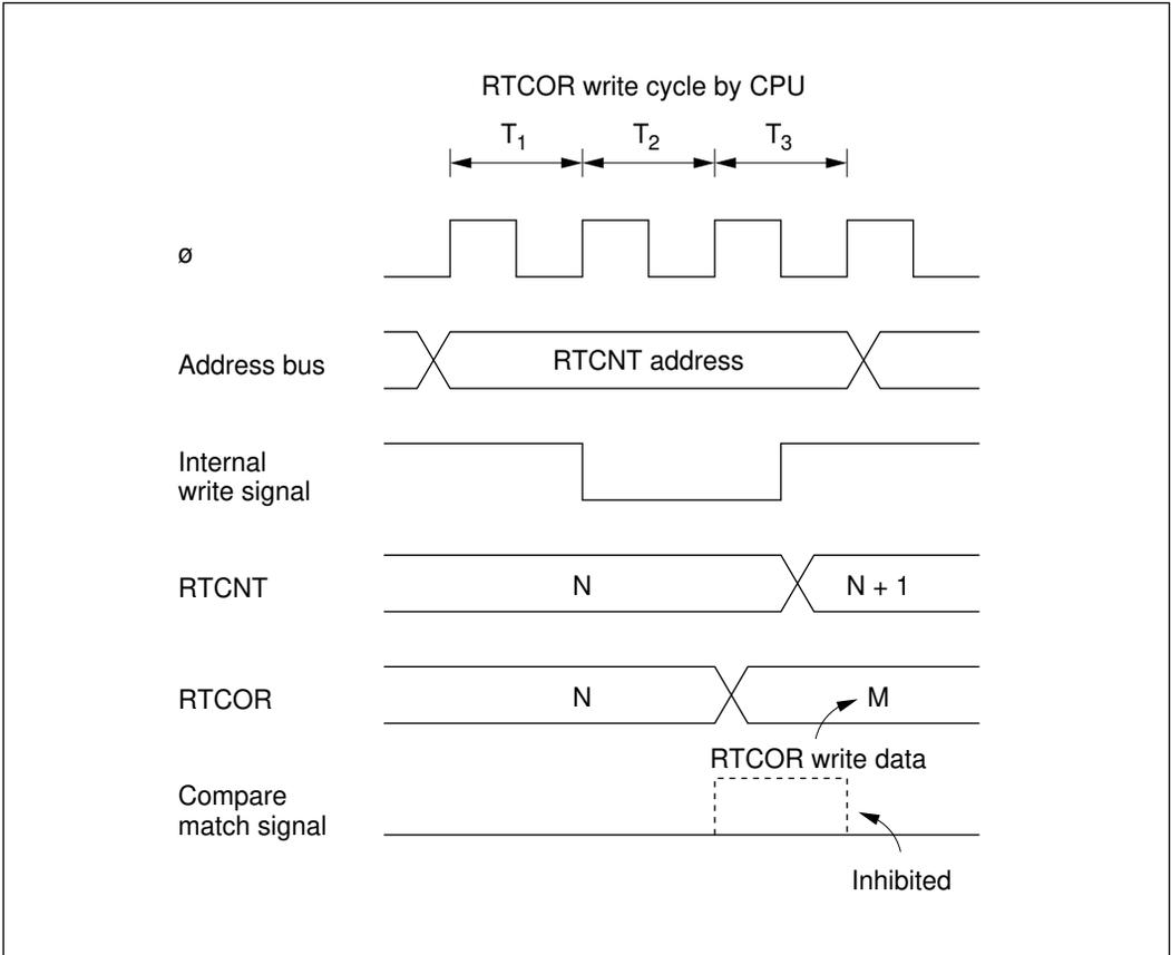
**Figure 7-22 Contention between RTCOR Write and Compare Match**
