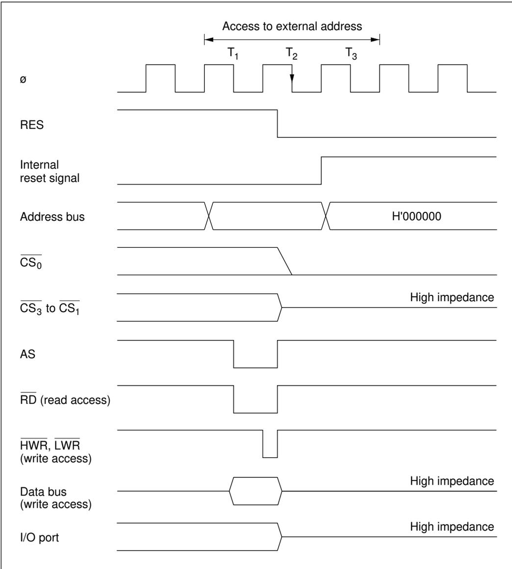
**Figure D-2 Reset during Memory Access (Reset during T<sub>2</sub> State)**
