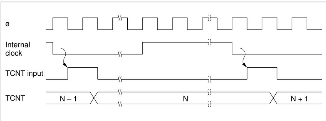
**Figure 10-17 Count Timing for Internal Clock Sources**
