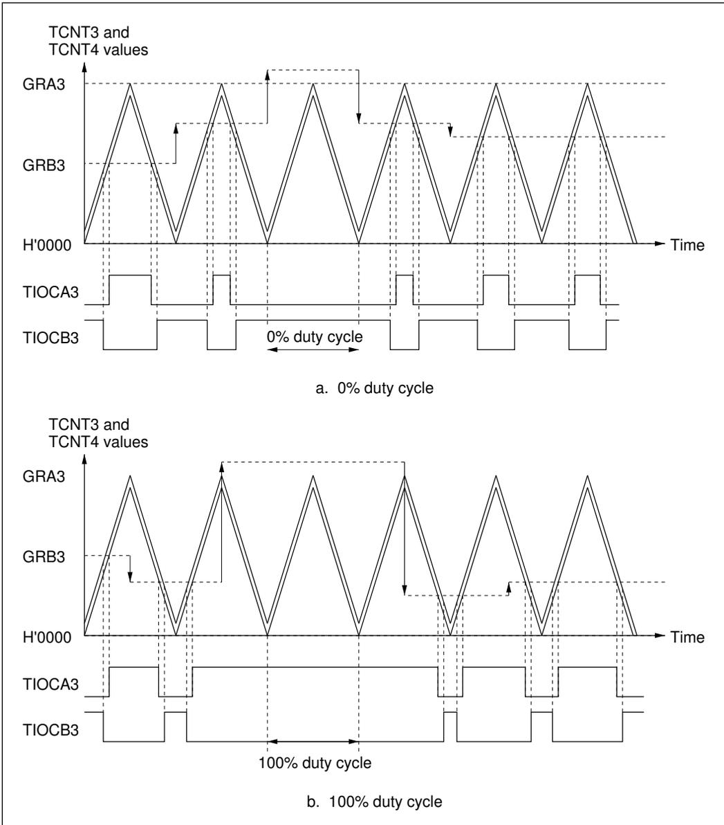
**Figure 10-36 Operation in Complementary PWM Mode (Example 2, OLS3 = OLS4 = 1)**
