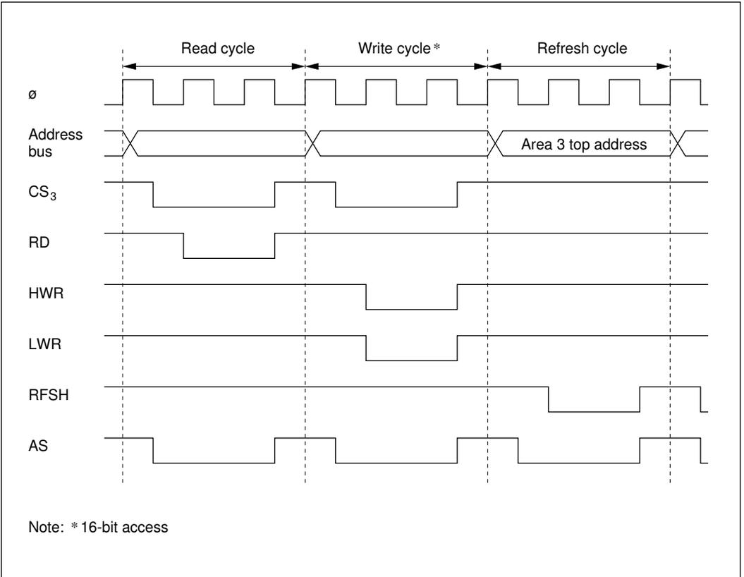
**Figure 7-15 Pseudo-Static RAM Control Signal Output Timing**
