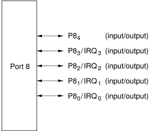
**Figure 9-26 Pin Functions in Modes 6 and 7 (Port 8)**
