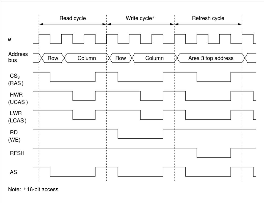
**Figure 7-5 DRAM Control Signal Output Timing (2) (2CAS Mode)**
