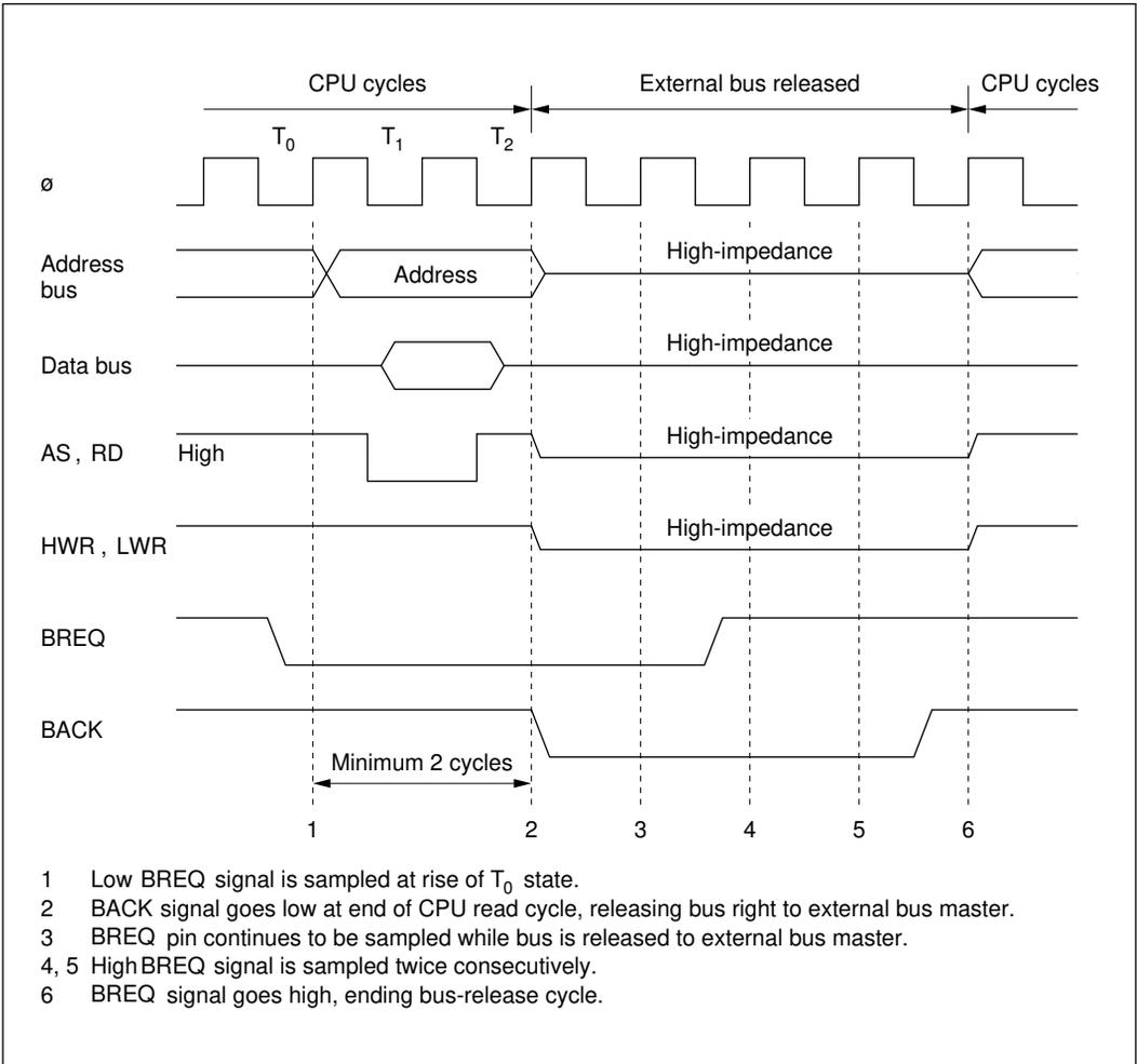
**Figure 6-19 External-Bus-Released State (Two-State-Access Area, During Read Cycle)**
