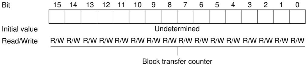
**IOAR0B—I/O Address Register 0B**
