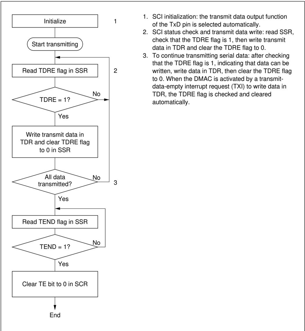
1. SCI initialization: the transmit data output function of the TxD pin is selected automatically.
