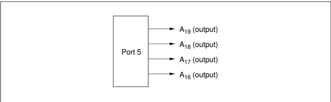
**Figure 9-17 Pin Functions in Modes 1 to 4 (Port 5)**
