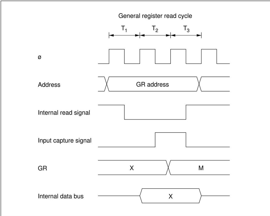
**Figure 10-66 Contention between General Register Read and Input Capture**
