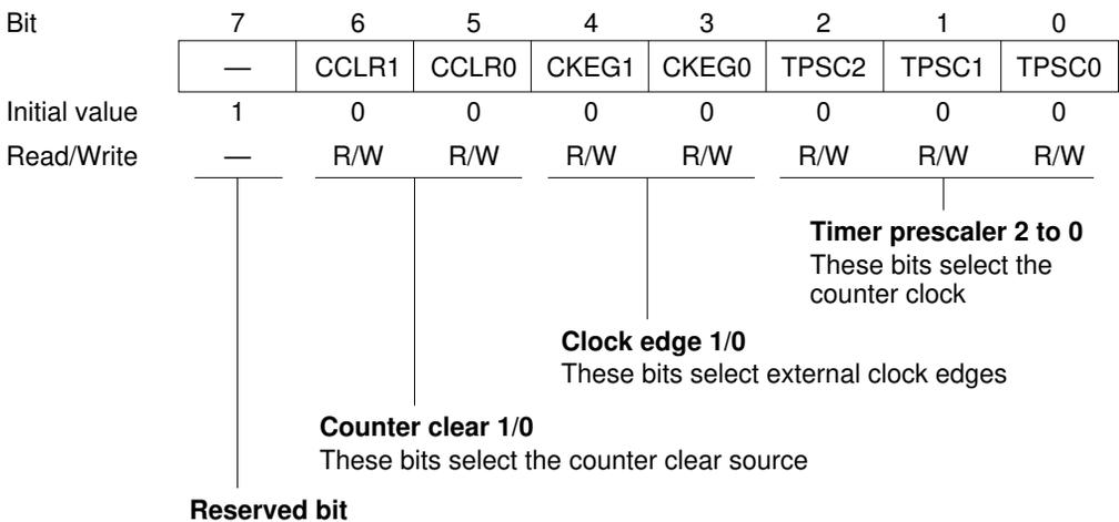
Each TCR is an 8-bit readable/writable register that selects the timer counter clock source, selects the edge or edges of external clock sources, and selects how the counter is cleared.
