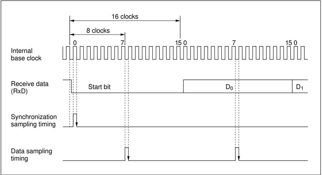
**Figure 13-21 Receive Data Sampling Timing in Asynchronous Mode**
