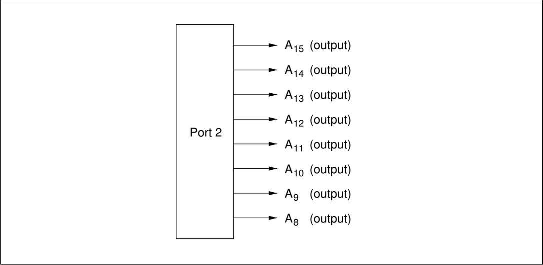
**Figure 9-6 Pin Functions in Modes 1 to 4 (Port 2)**
