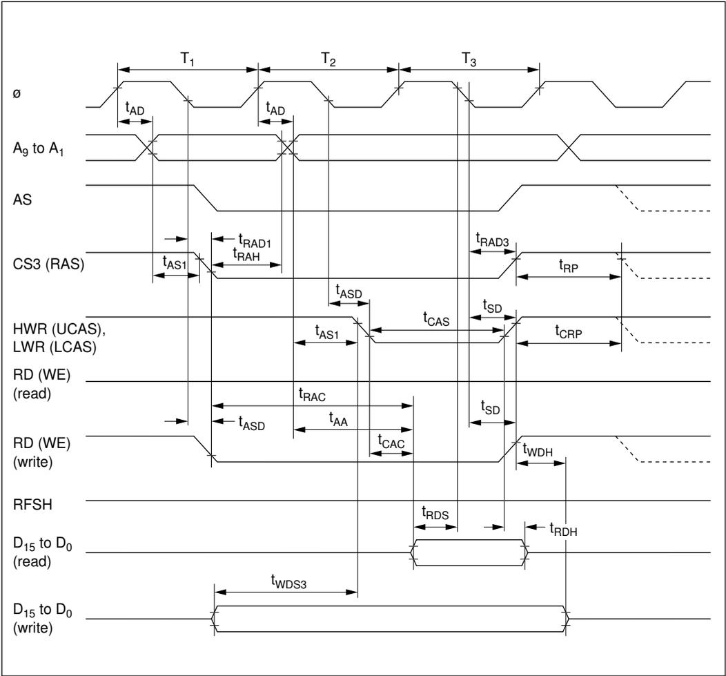
**Figure 20-10 DRAM Bus Timing (Read/Write): Three-State Access**
