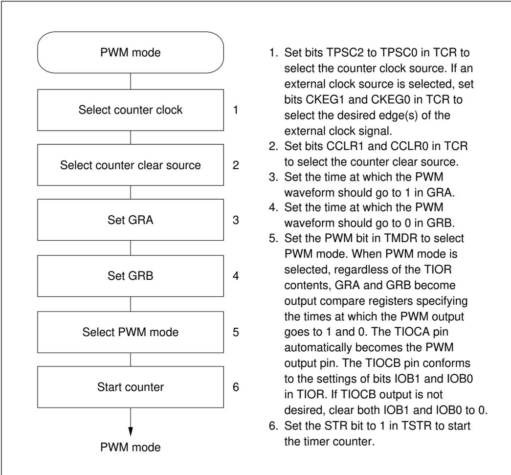
**Figure 10-28 Setup Procedure for PWM Mode (Example)**
