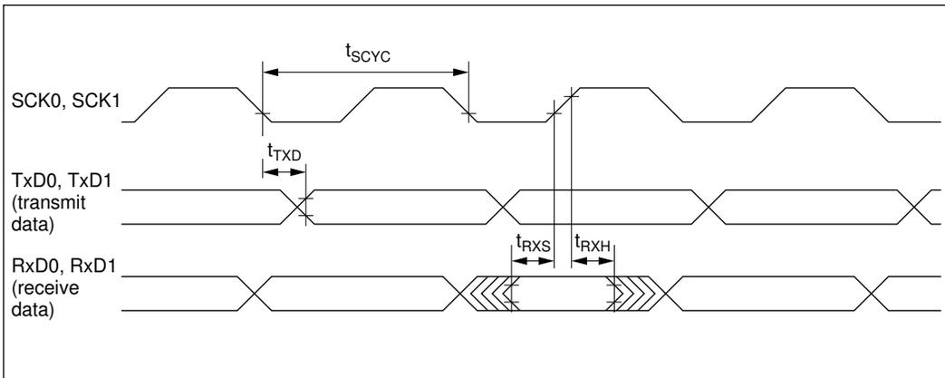
**Figure 20-24 SCI Input/Output Timing in Synchronous Mode**
