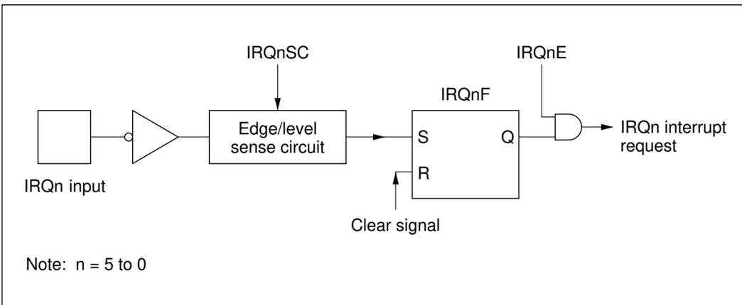
Figure 5-2 Block Diagram of Interrupts IRQ<sub>0</sub> to IRQ<sub>5</sub>
