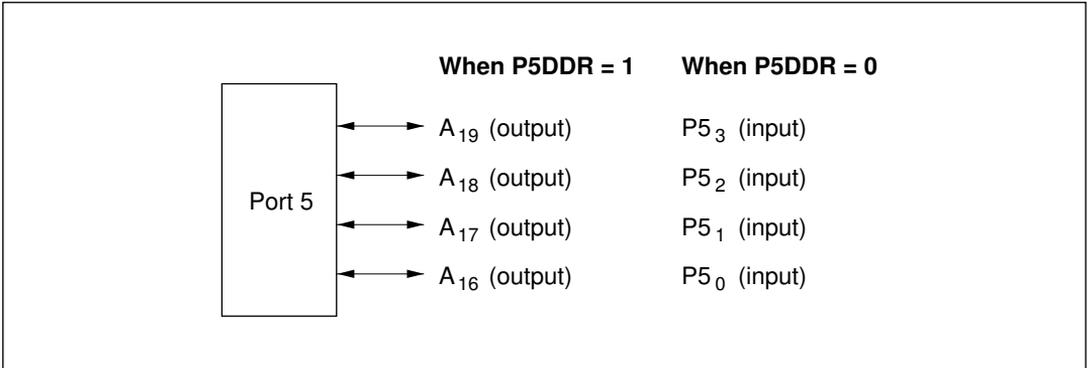
**Figure 9-18 Pin Functions in Mode 5 (Port 5)**
