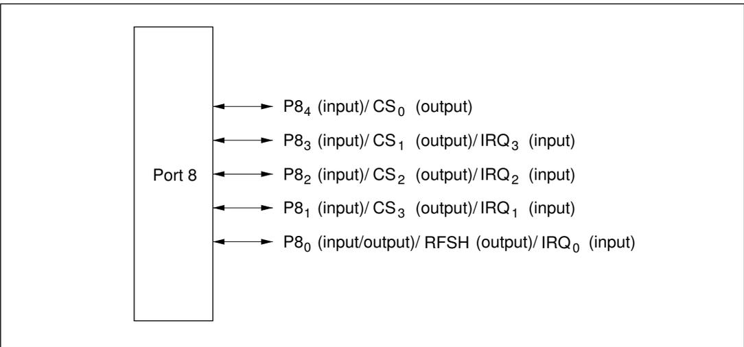
**Figure 9-25 Pin Functions in Modes 1 to 5 (Port 8)**
