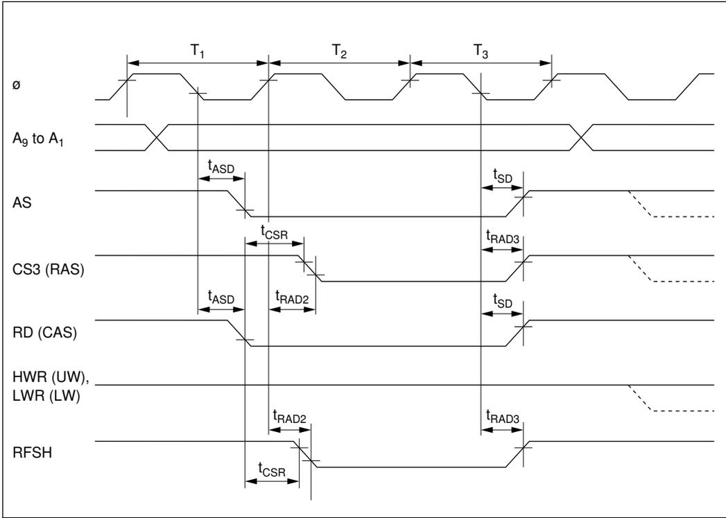
**Figure 20-8 DRAM Bus Timing (Refresh Cycle): Three-State Access**
