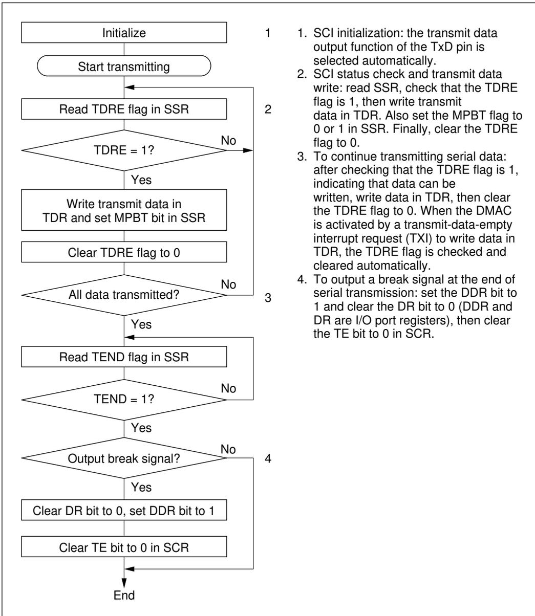
**Figure 13-10 Sample Flowchart for Transmitting Multiprocessor Serial Data**
