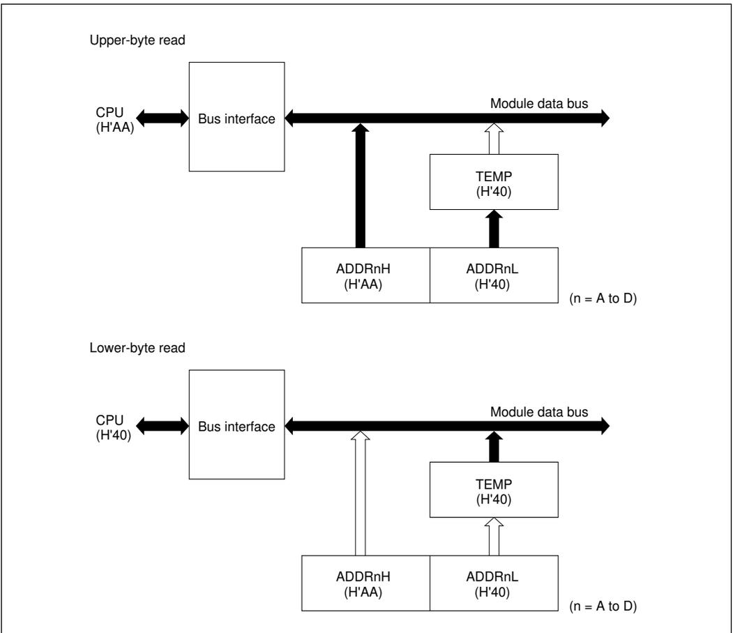
Figure 14-2 A/D Data Register Access Operation (Reading H'AA40)
