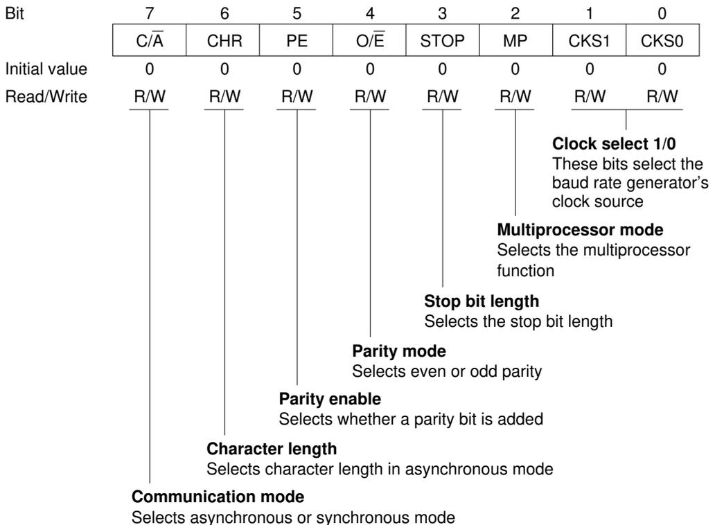
The CPU can always read and write SMR. SMR is initialized to H'00 by a reset and in standby mode.
