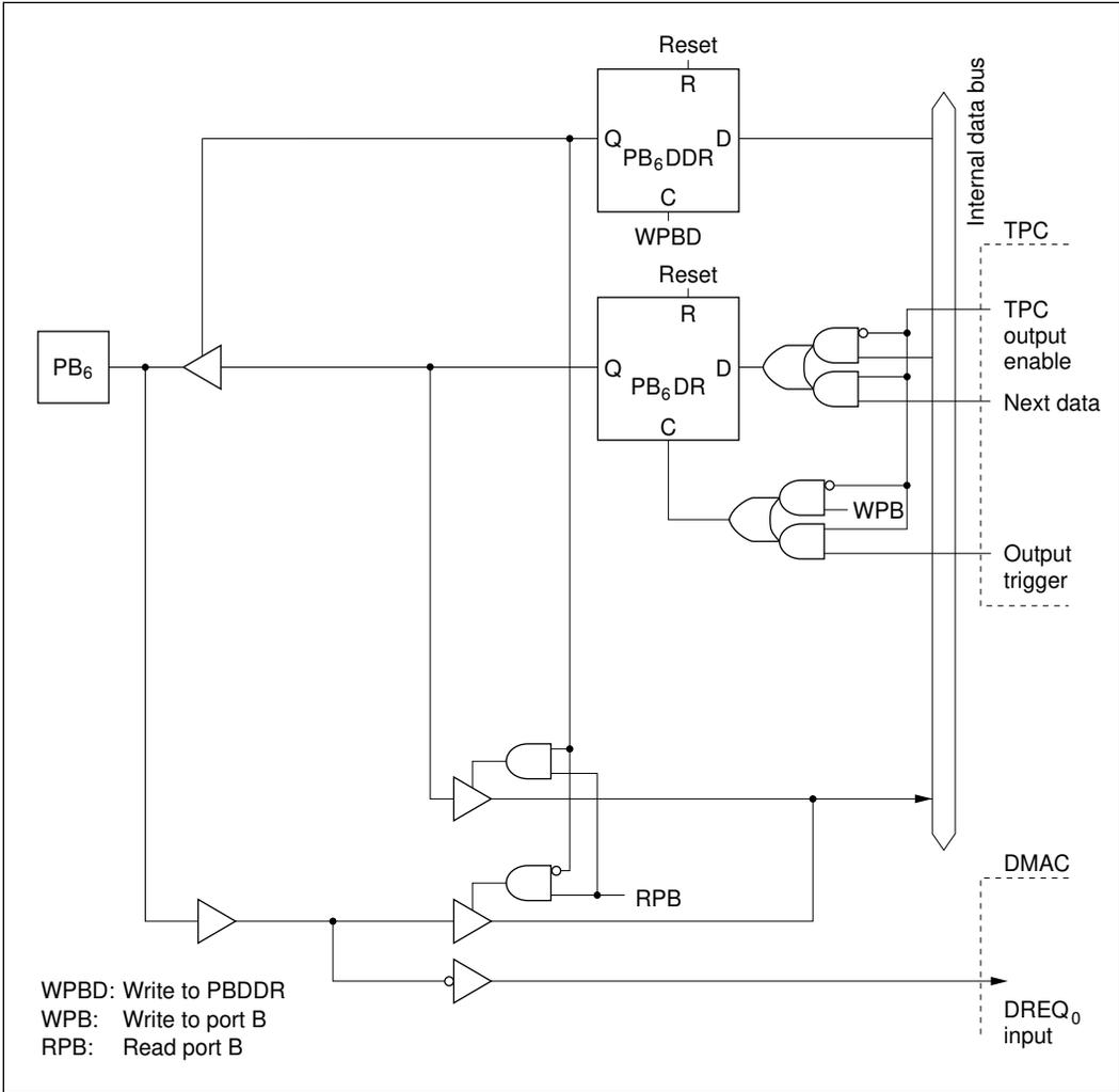
**Figure C-11 (c) Port B Block Diagram (Pin PB<sub>6</sub>)**
