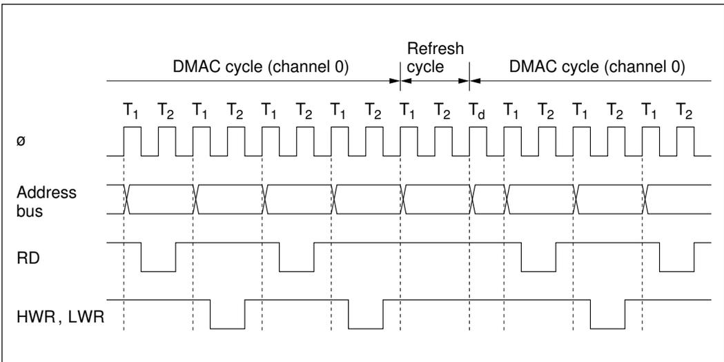
**Figure 8-20 Bus Timing of Refresh Controller and DMAC**
