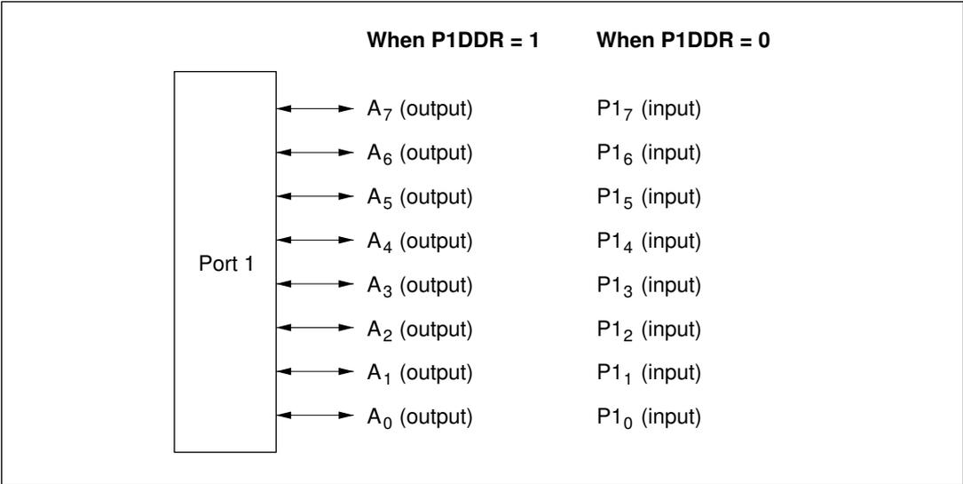
**Figure 9-3 Pin Functions in Mode 5 (Port 1)**
