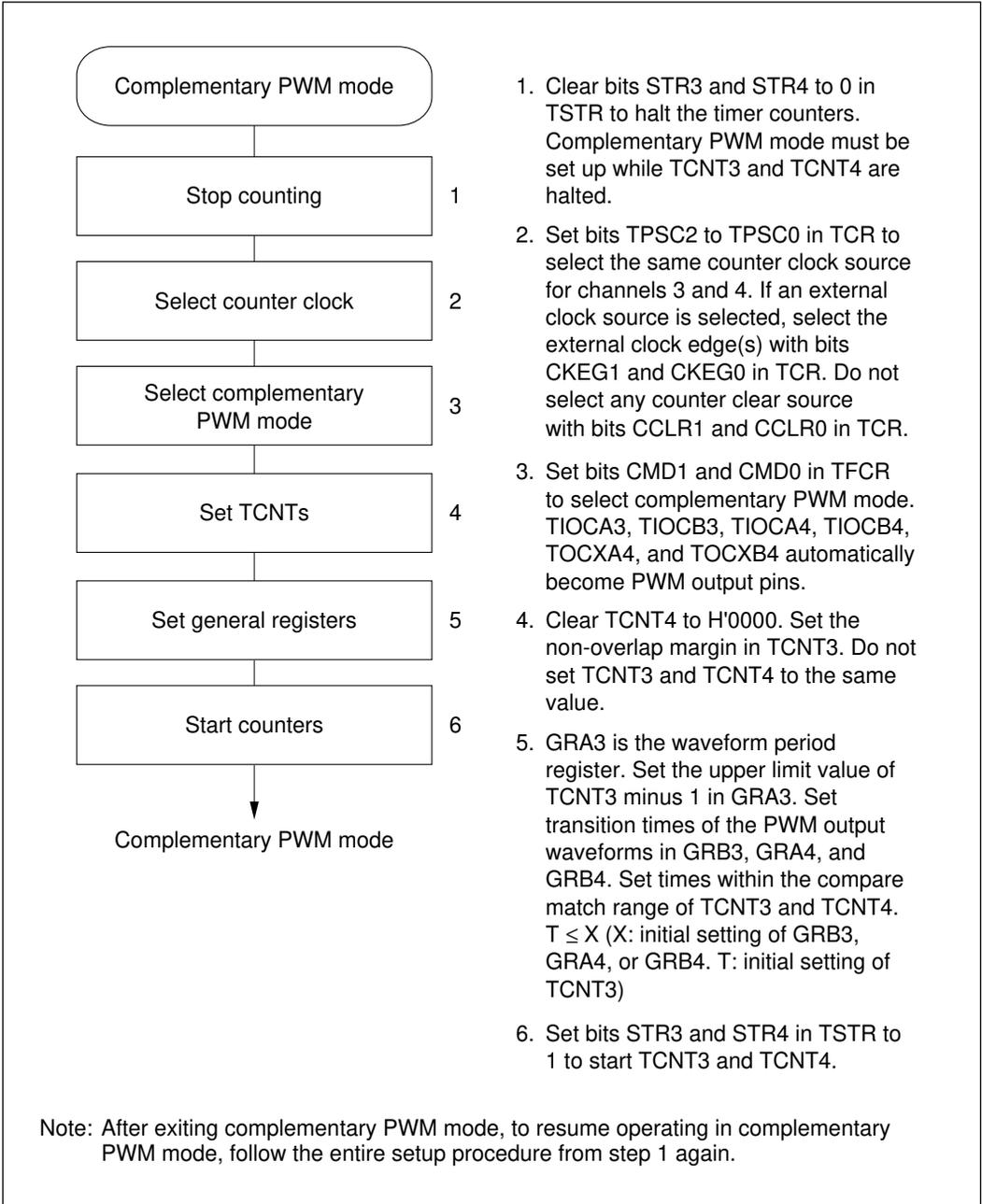
1. Clear bits STR3 and STR4 to 0 in TSTR to halt the timer counters. Complementary PWM mode must be set up while TCNT3 and TCNT4 are halted.
