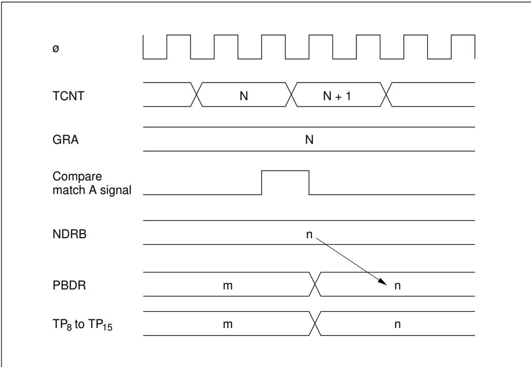
**Figure 11-3 Timing of Transfer of Next Data Register Contents and Output (Example)**
