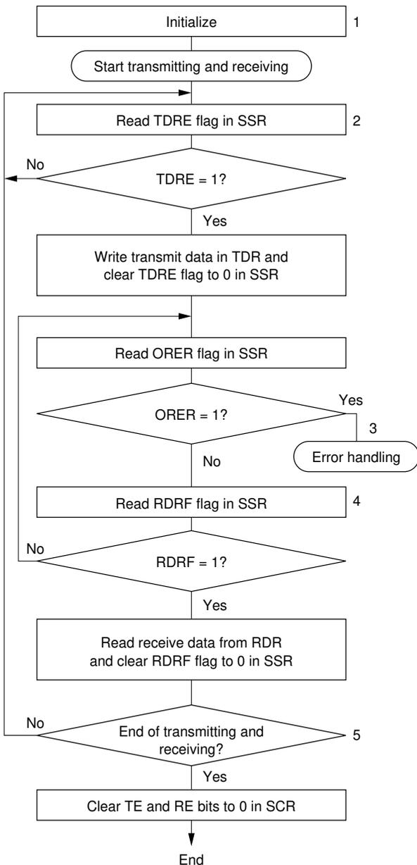
1. SCI initialization: the transmit data output function of the TxD pin and receive data input function of the RxD pin are selected, enabling simultaneous transmitting and receiving.
