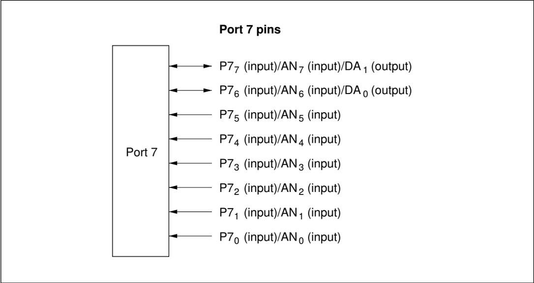
**Figure 9-23 Port 7 Pin Configuration**
