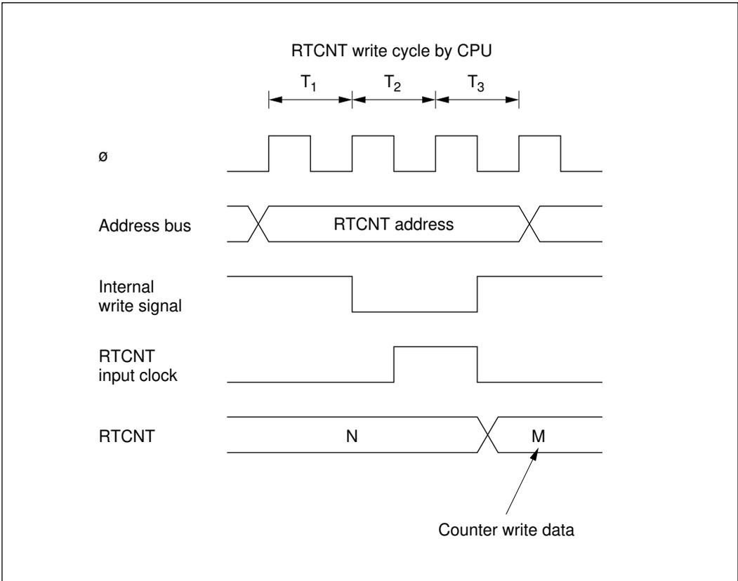
**Figure 7-21 Contention between RTCNT Write and Increment**
