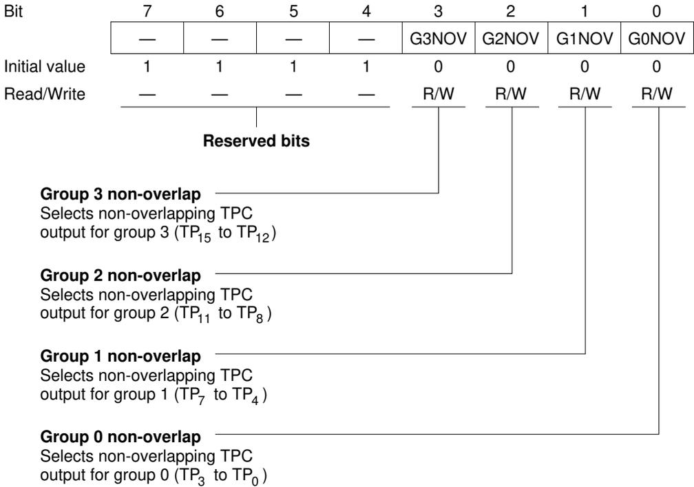
The output trigger period of a non-overlapping TPC output waveform is set in general register B (GRB) in the ITU channel selected for output triggering. The non-overlap margin is set in general register A (GRA). The output values change at compare match A and B. For details see section 11.3.4, Non-Overlapping TPC Output.
