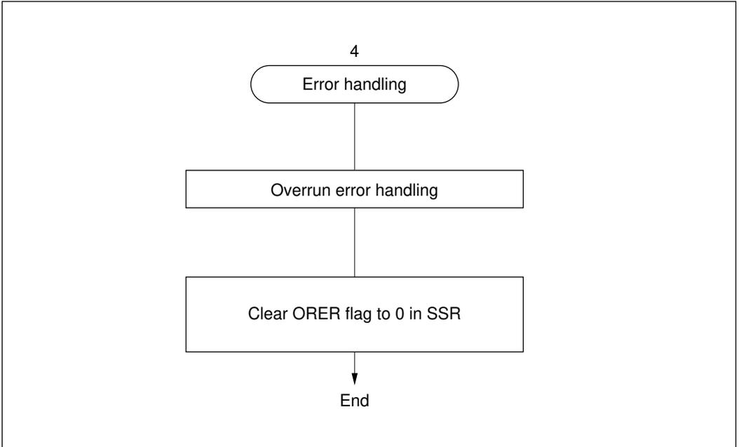
**Figure 13-18 Sample Flowchart for Serial Receiving (2)**
