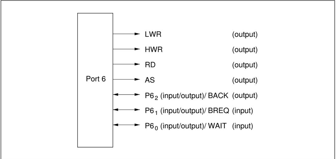
**Figure 9-21 Pin Functions in Modes 1 to 5 (Port 6)**
