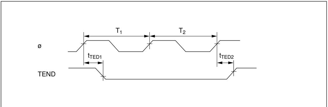
**Figure 20-25 DMAC  $\overline{\text{TEND}}$  Output Timing for 2 State Access**
