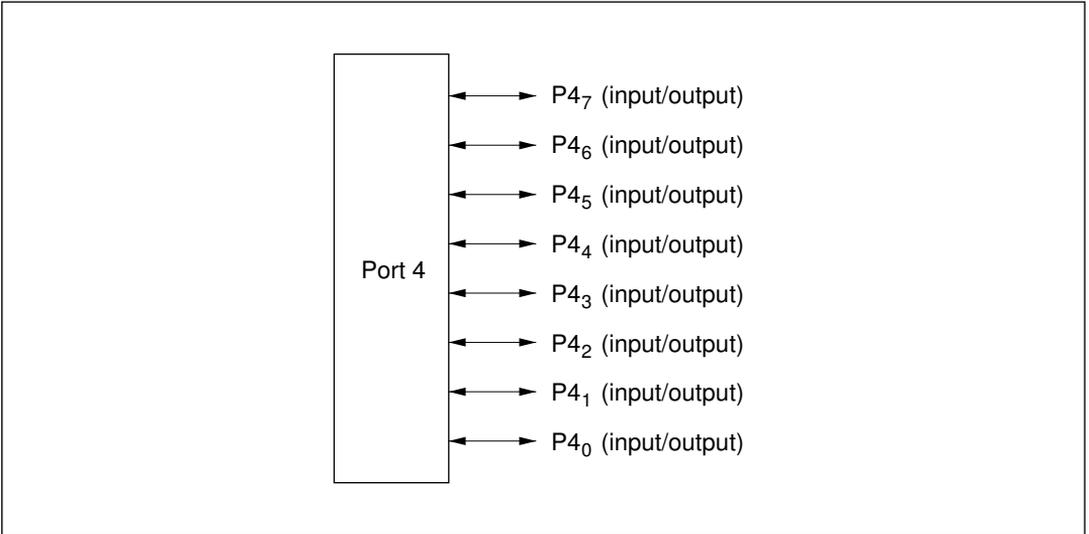
**Figure 9-13 Pin Functions in 8-Bit Bus Mode (Port 4)**
