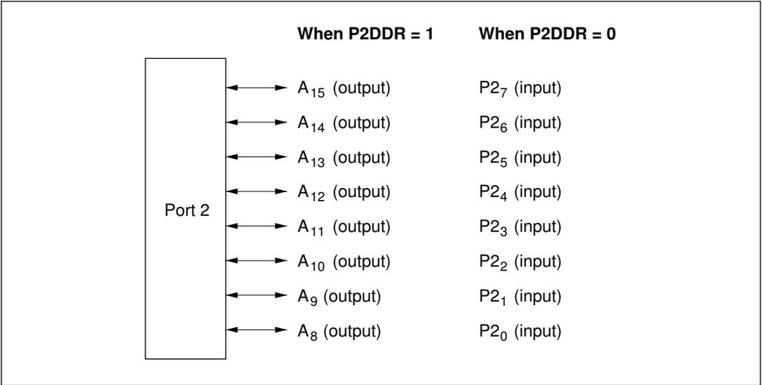
**Figure 9-7 Pin Functions in Mode 5 (Port 2)**
