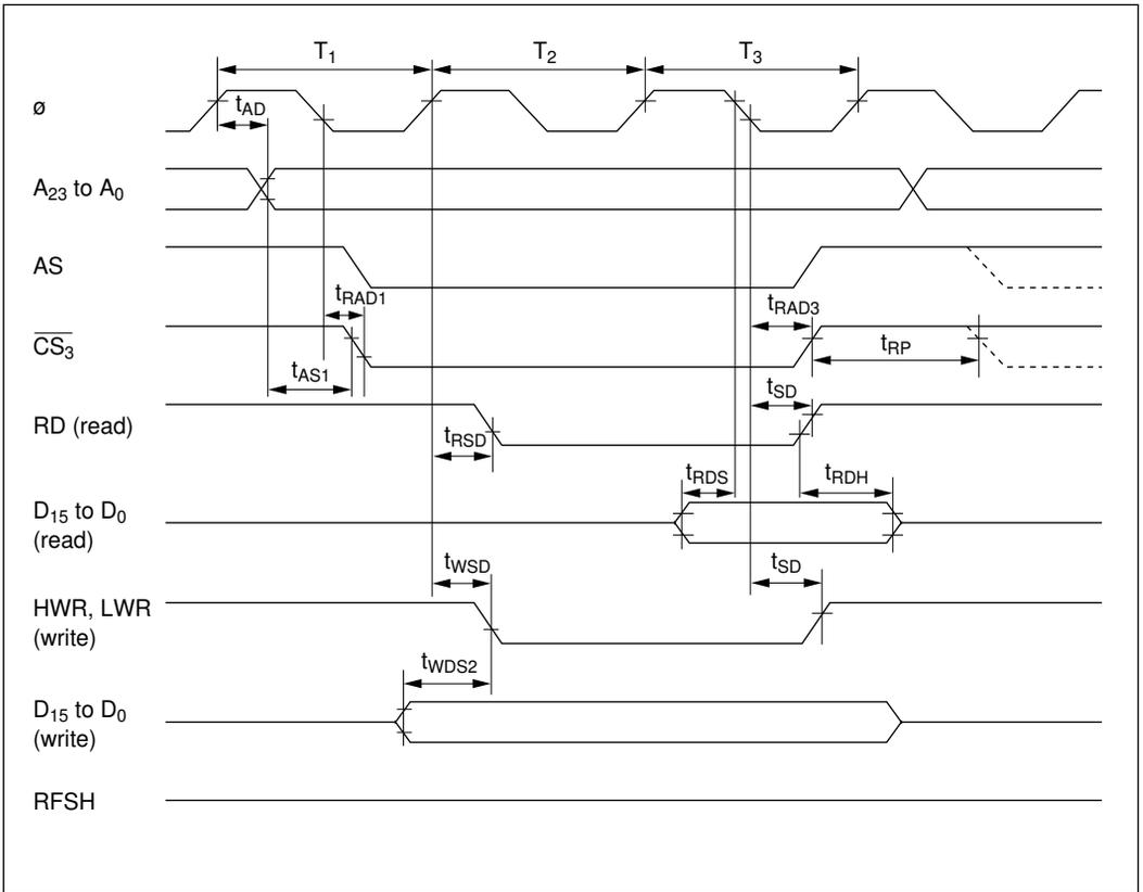
**Figure 20-13 PSRAM Bus Timing (Read/Write): Three-State Access**
