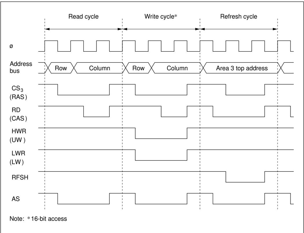
**Figure 7-5 DRAM Control Signal Output Timing (1) ( $\overline{2WE}$  Mode)**
