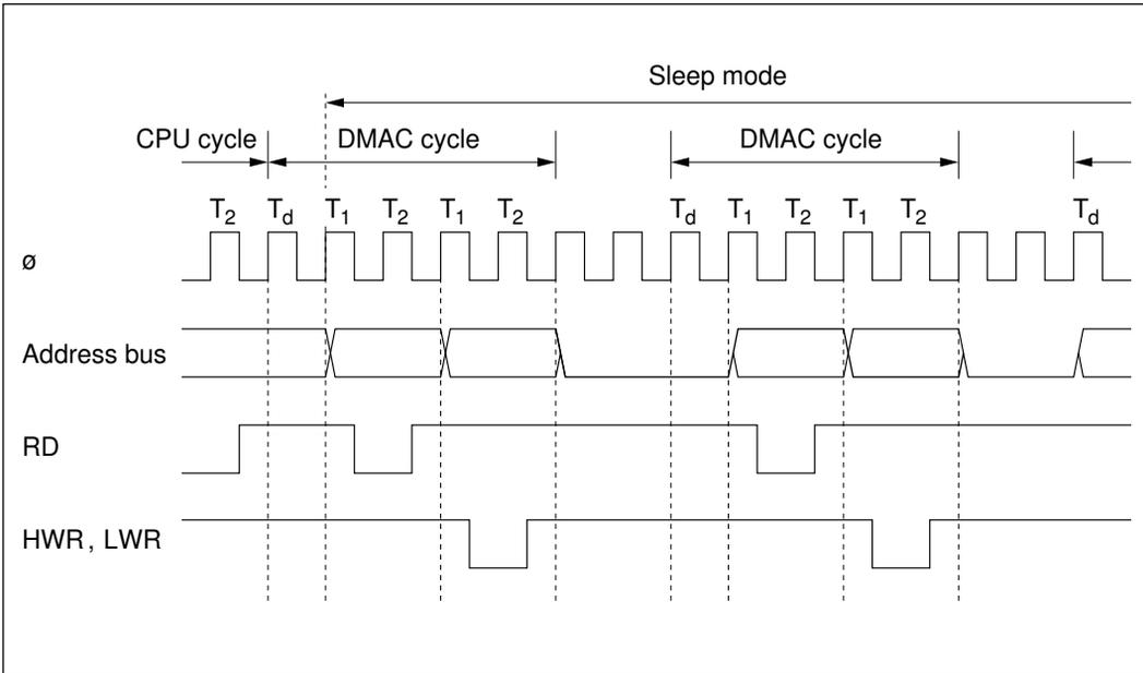
**Figure 8-24 Timing of Cycle-Steal Transfer in Sleep Mode**
