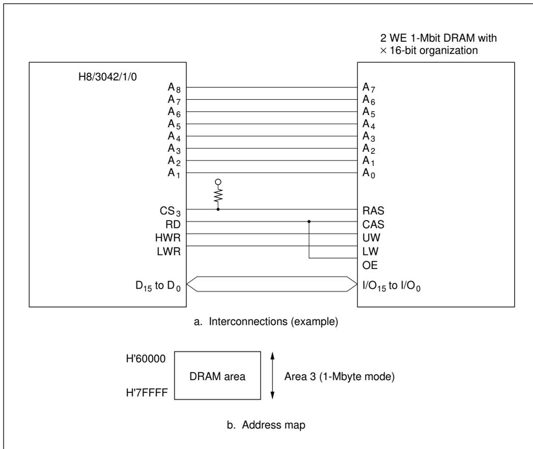
**Figure 7-7 Interconnections and Address Map for  $2\overline{\text{WE}}$  1-Mbit DRAM (Example)**
