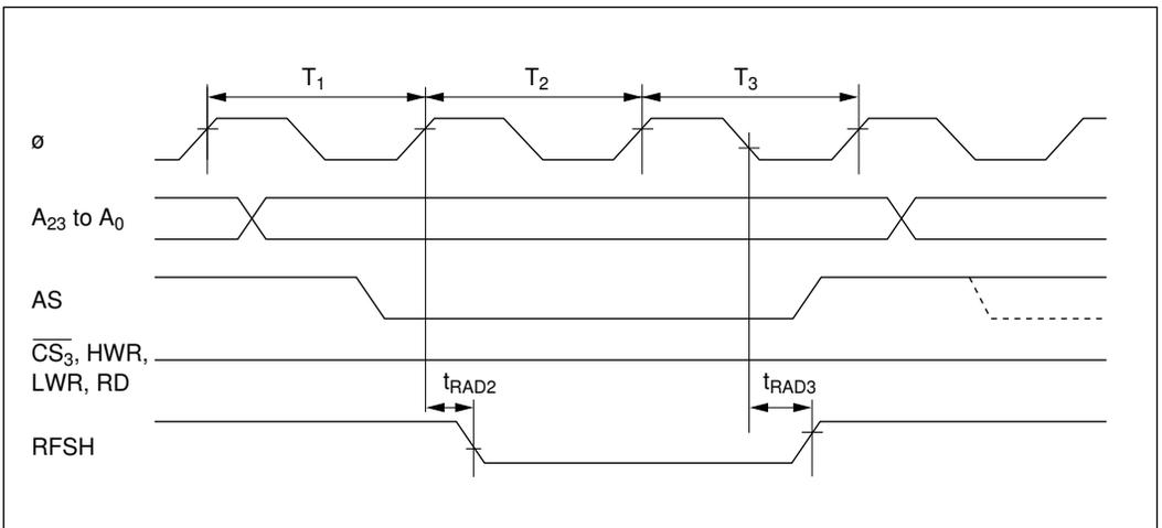
**Figure 20-14 PSRAM Bus Timing (Refresh Cycle): Three-State Access**
