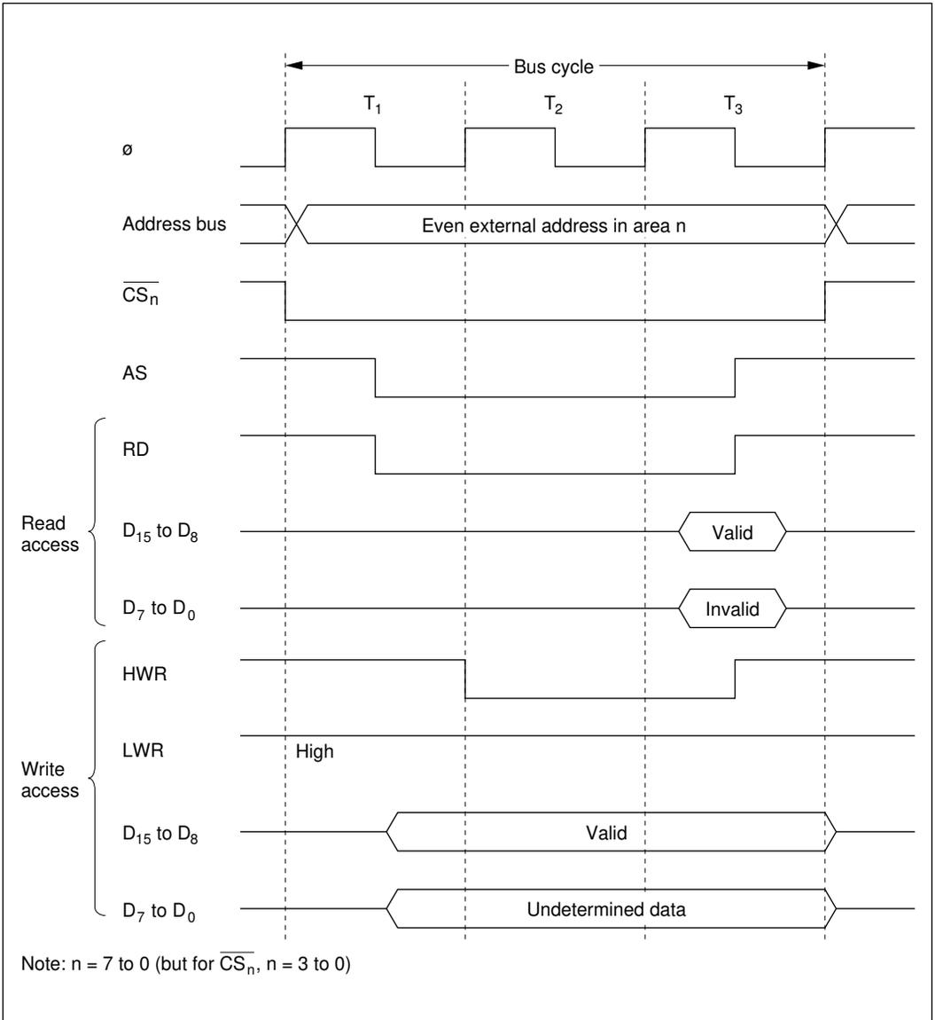
**Figure 6-6 Bus Control Signal Timing for 16-Bit, Three-State-Access Area (1)
