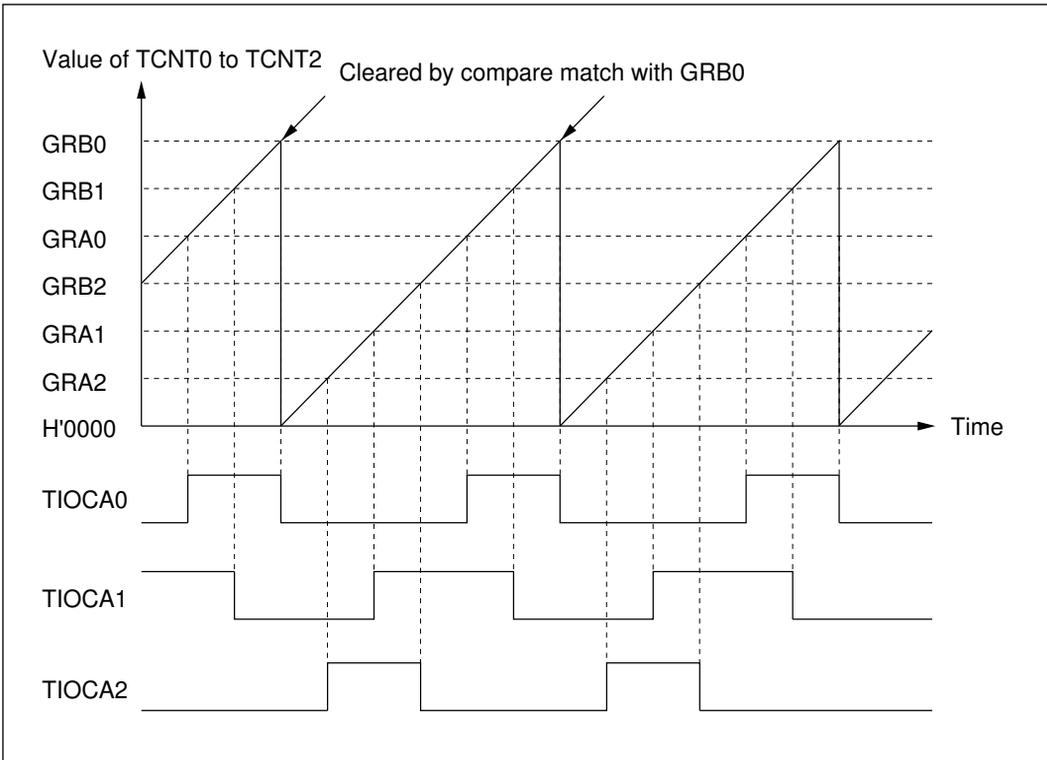
**Figure 10-27 Synchronization (Example)**
