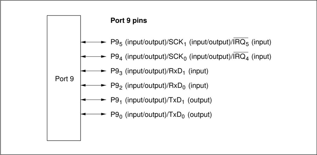
Figure 9-27 Port 9 Pin Configuration
