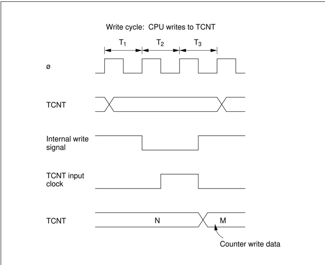
**Figure 12-8 Contention between TCNT Write and Increment**
