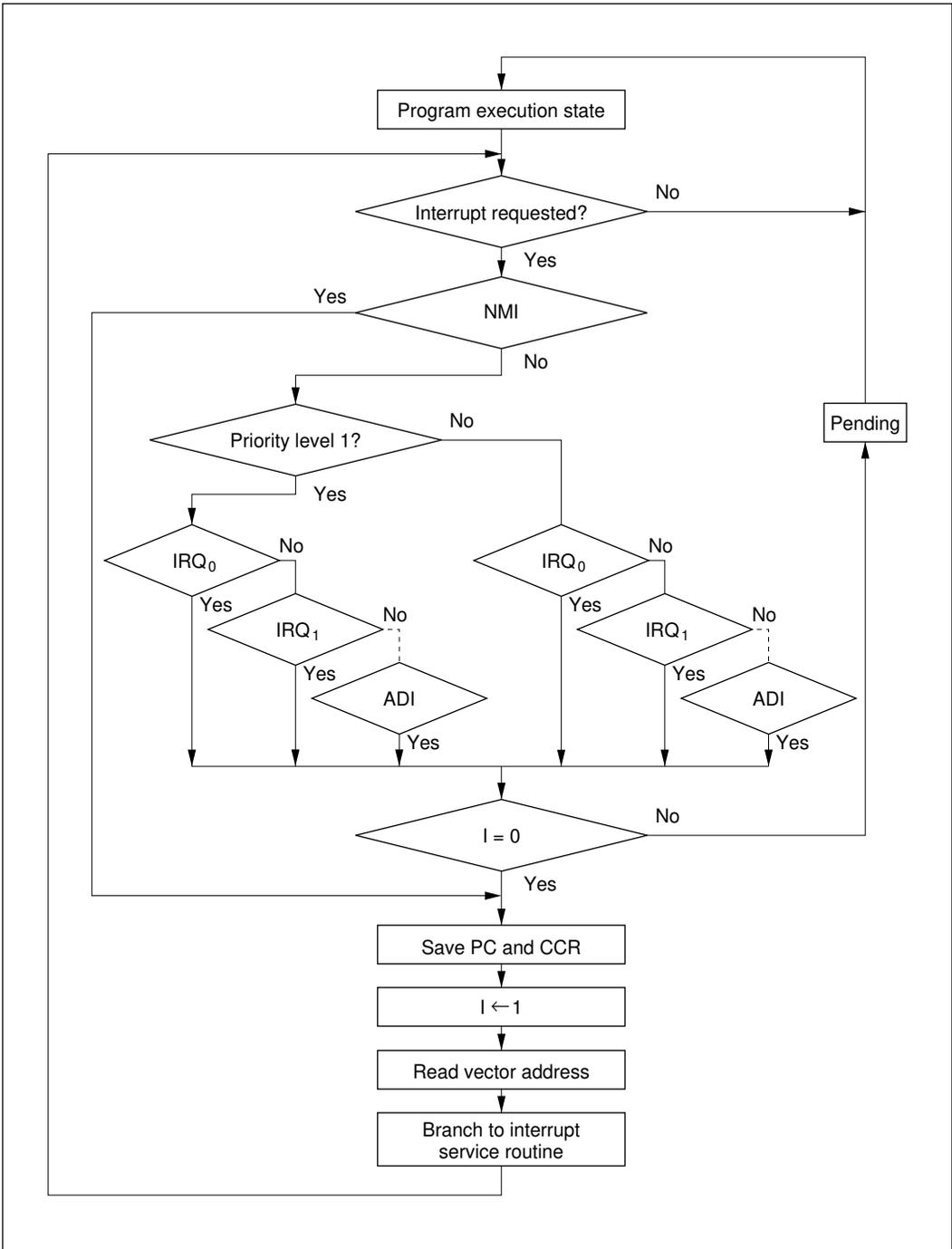
**Figure 5-4 Process Up to Interrupt Acceptance when UE = 1**
