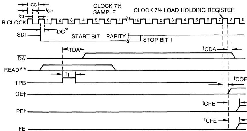
\* IF A START BIT OCCURS AT A TIME LESS THAN  $t_{DC}$  BEFORE A HIGH-TO-LOW TRANSITION OF THE CLOCK, THE START BIT MAY NOT BE RECOGNIZED UNTIL THE NEXT HIGH-TO-LOW TRANSITION OF THE CLOCK. THE START BIT MAY BE COMPLETELY ASYNCHRONOUS WITH THE CLOCK.
