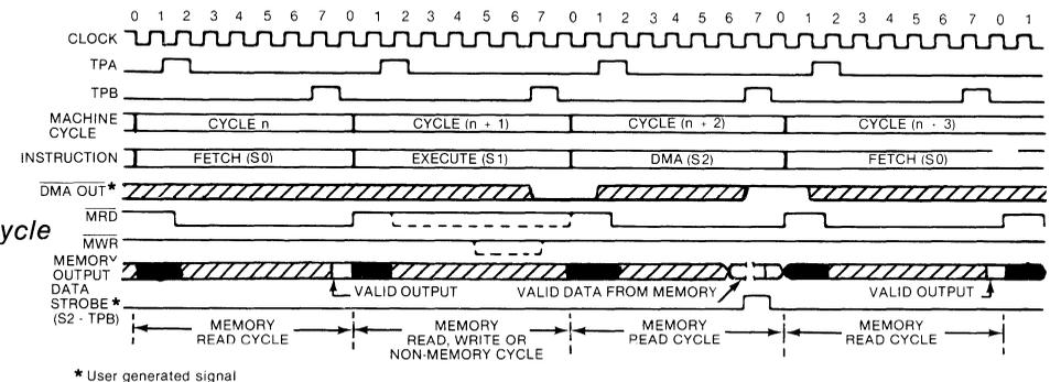
FIG. 10 DMA — Out cycle
