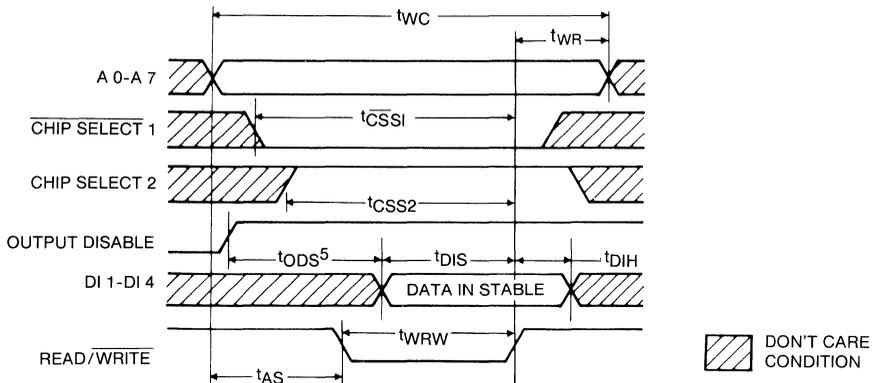
NOTE 5:  $t_{ODS}$  is required for common I/O operation only; for separate I/O operations, Output Disable is Don't Care.
