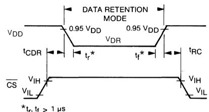
Low V<sub>DD</sub> data retention waveforms and timing diagram.
