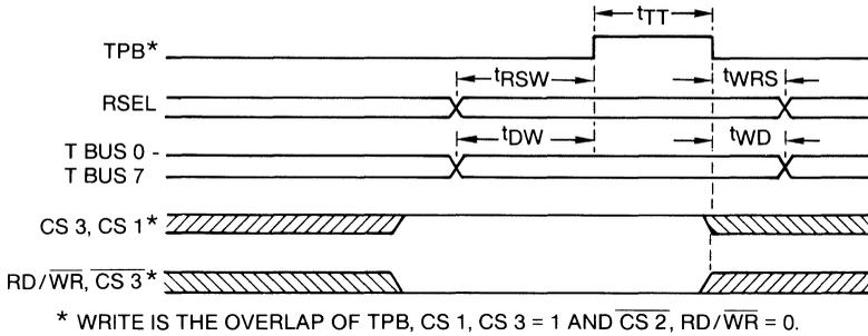
FIGURE 6. MODE 1 CPU INTERFACE (WRITE) TIMING DIAGRAM
