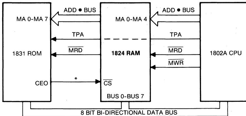
\*Chip select may be derived through (1) address decode, (2) CEO signal from ROM, or (3) always enabled (GND) per system requirements.
