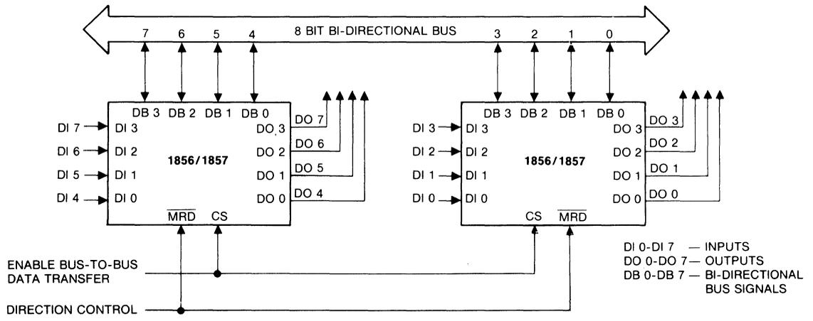
The Figure shows how two 1856 or two 1857 can be used as bus buffers or separators between an 8 Bit Bi-directional Data bus and memories or between an 8 Bit Bi-directional Data bus and I/O devices. The chip select input signal enables the bus separator three-state output drivers. The direction of data flow, when enabled, is controlled by the state of the MRD input signal.
