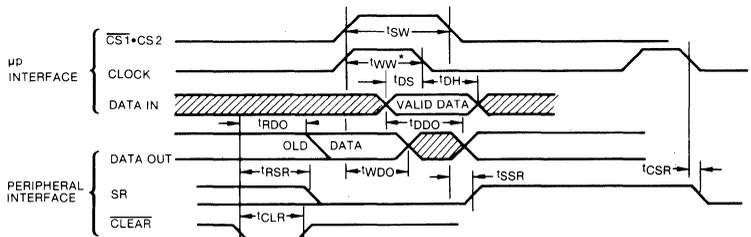
\*Write is the overlap of  $\overline{\text{CS1}} \cdot \text{CS2}$  and Clock
