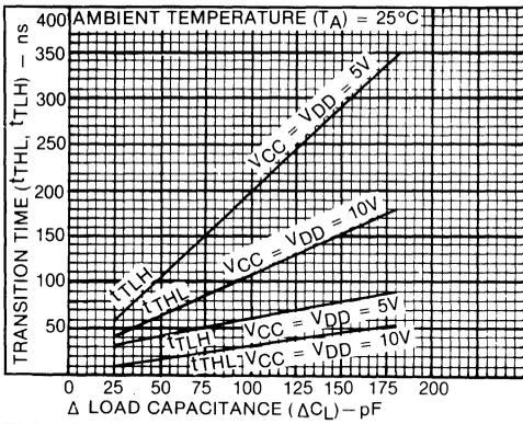
FIG. 2 Typical transition time vs. load capacitance.
