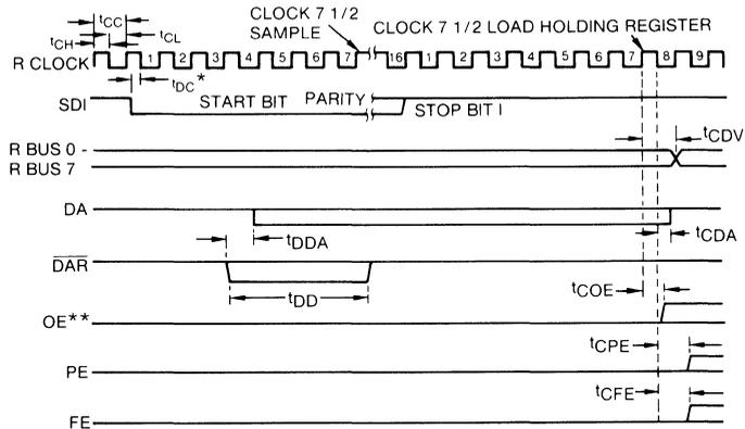
\* IF A START BIT OCCURS AT A TIME LESS THAN  $t_{DC}$  BEFORE A HIGH-TO-LOW TRANSITION OF THE CLOCK, THE START BIT MAY NOT BE RECOGNIZED UNTIL THE NEXT HIGH-TO-LOW TRANSITION OF THE CLOCK. THE START BIT MAY BE COMPLETELY ASYNCHRONOUS WITH THE CLOCK.
