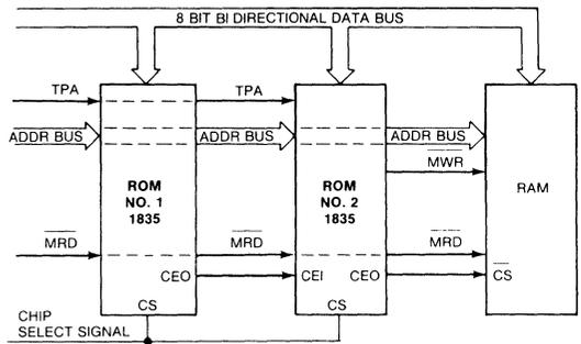
“Daisy Chaining” with CEI inputs and CEO outputs is used to avoid memory conflicts between ROM and RAM in a user system. In the above configuration, if ROM #1 was masked-programmed for memory locations 0000-3FF<sub>16</sub> and ROM #2 masked-programmed for memory locations 0400-07FF<sub>16</sub> for addresses from 0000-07FF<sub>16</sub> the RAM would be disabled and the ROM enabled. For locations above 07FF<sub>16</sub> the ROM’s would be disabled and RAM enabled.
