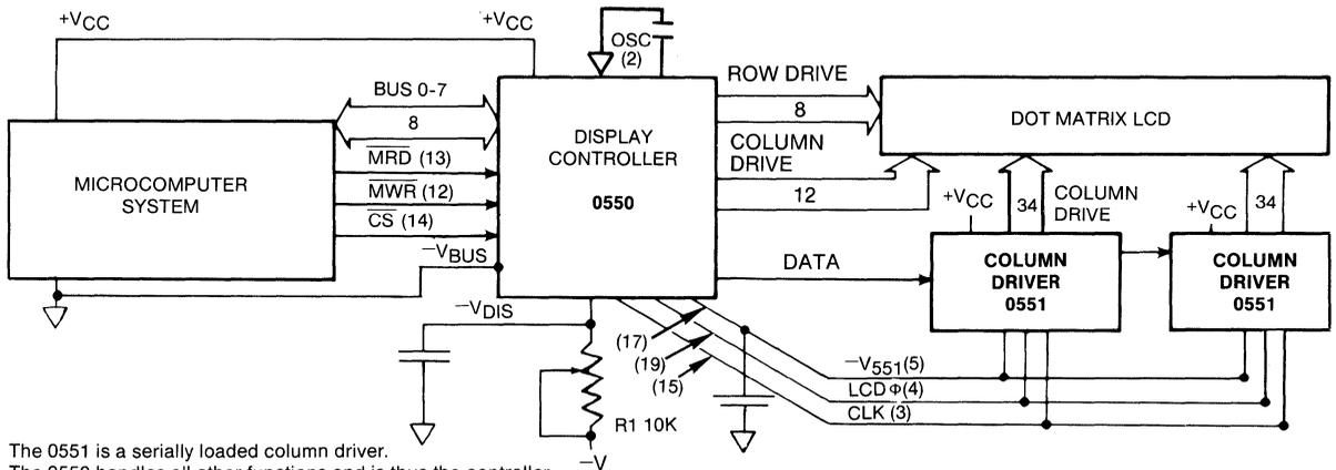
The 0551 is a serially loaded column driver.
