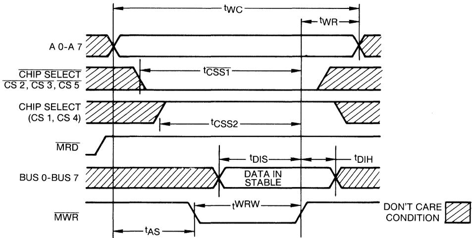
Figure 2 — Write cycle waveforms and timing diagram.
