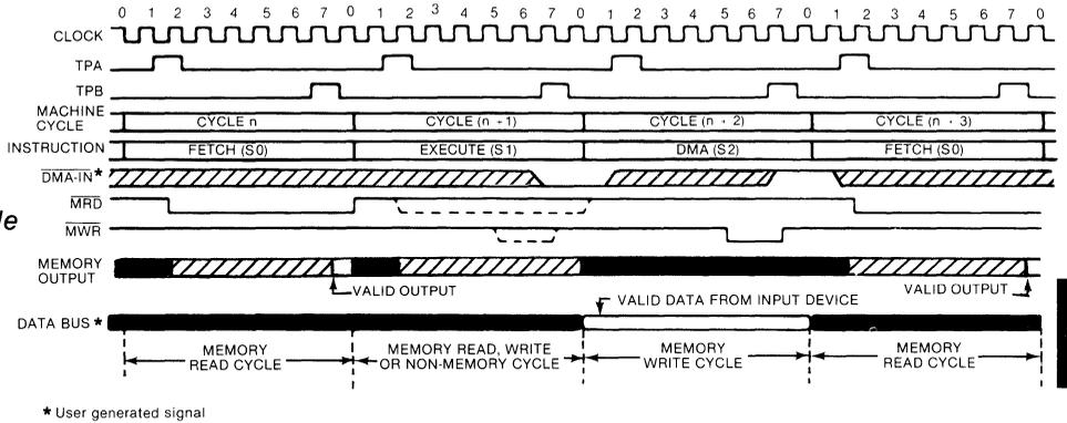
FIG. 9 DMA — In cycle
