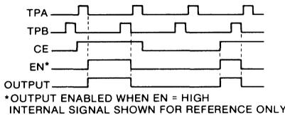
**PROPAGATION DELAY TIMING:**
