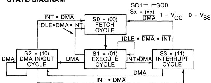
The 1802A state transitions when in the run mode are shown to the left. Each machine cycle requires 8 clock pulses except the initialization cycle, after reset, which requires nine clock pulses.
