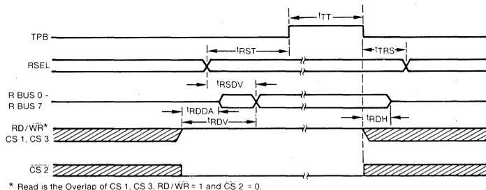
**FIGURE 8. MODE 1 CPU INTERFACE (READ) TIMING DIAGRAM**
