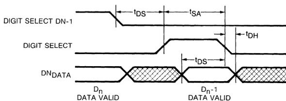
**(b) Microprocessor Interface Input Timing**
