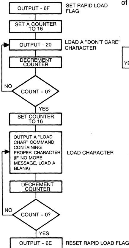
**Character Load Display** - Suppose the display shows the message SUM = 354.2 (left justified) and it is desired that this be changed to SUM = 357.8. Assume the initialization of the example.
