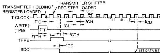
\* The Holding Register is Loaded On the Trailing Edge of TPS.
