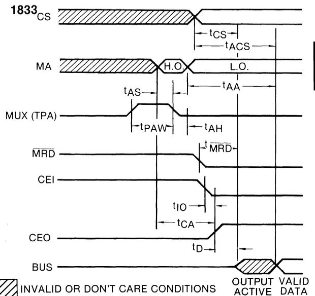
The dynamic characteristic table and the above timing diagrams represent maximum performance capability of the 1831/1833. When used in direct system interface with the 1802A microprocessor, the timing relation will be determined by the clock frequency and timing signal generation of the microprocessor. In the latter case the following general timing conditions hold: t<sub>AH</sub> = 0.5 t<sub>C</sub>
