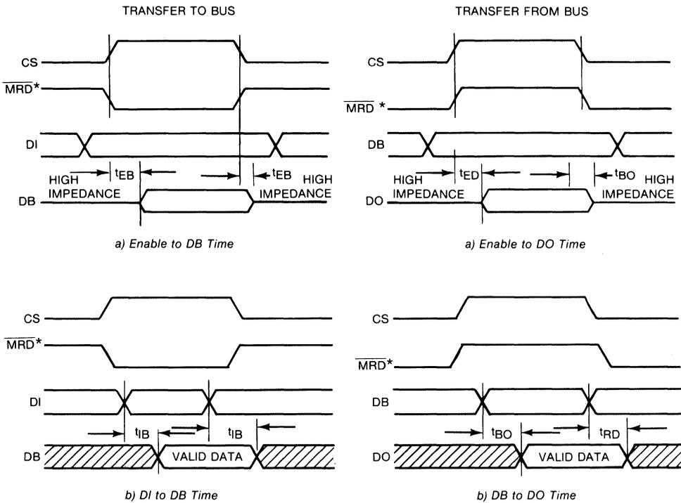
NOTE: ALL TIMES MEASURED FROM 50% POINT TO 50% POINT OF SIGNAL
