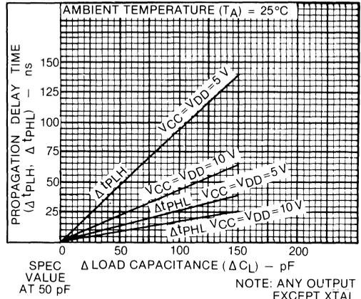
FIG. 3 Typical change in propagation delay as a function of a change in load capacitance.
