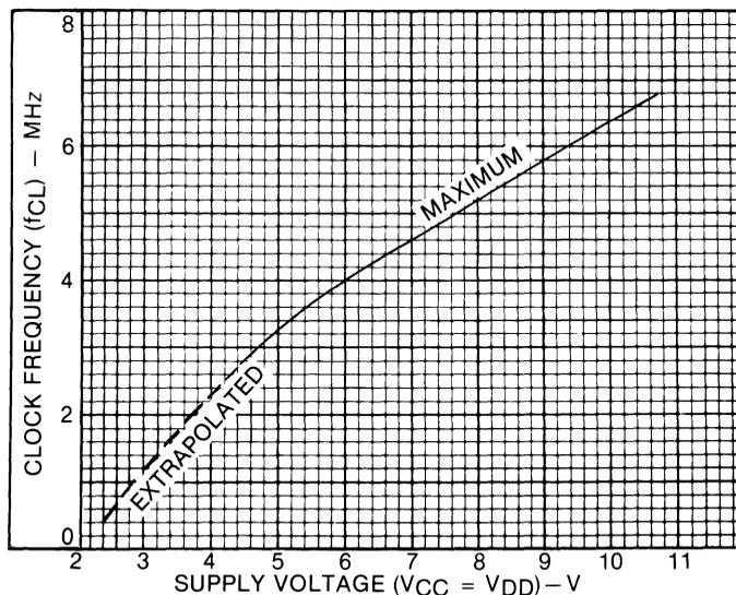
FIG. 6 Clock frequency is a function of supply voltage.
