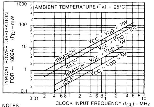
FIG. 5 Typical power dissipation as a function of clock frequency for Branch instruction and Idle instruction for 1802A.
