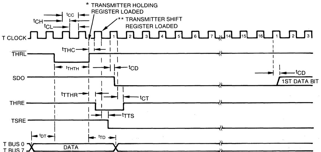
\* THE HOLDING REGISTER IS LOADED ON THE TRAILING EDGE OF THRL
