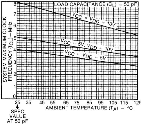
FIG. 4 Typical maximum clock frequency as a function of temperature.
