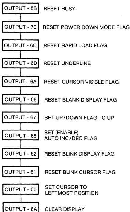
**Rapid Load Display** - This sequence will display a 16 character message using the rapid load feature. Assume initialization was done as in example.
