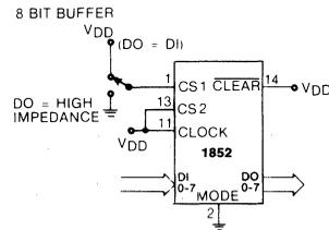
This figure shows 1852 connected as a non-inverting, three state, 8 bit buffer, with  $MODE = 0$ ,  $CLOCK = 1$  and  $CS2 = 1$ .  $CS1$  can be used as a tri-state control. When  $CS1 = 0$ , the output is a high impedance, but when  $CS1 = 1$  data output equals data input. If a high impedance state is not required, the  $CS1$  input can be tied high ( $CS1 = 1$ ).
