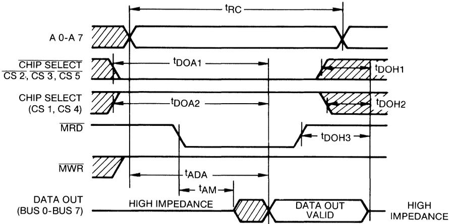
Figure 1 — Read cycle waveforms and timing diagram.
