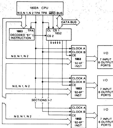
In the 1802A microprocessor systems, when more than 7 input or 7 output ports are required, a two level I/O system can be designed as shown in the figure.
