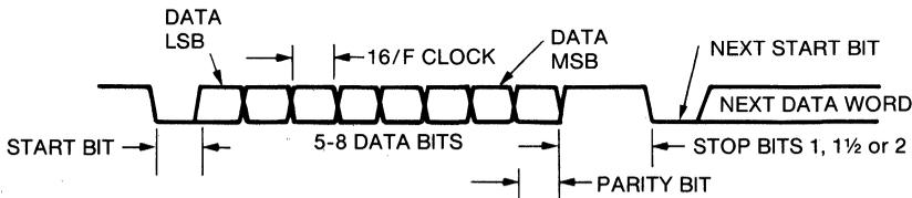
FIGURE 2. SERIAL DATA WORD FORMAT
