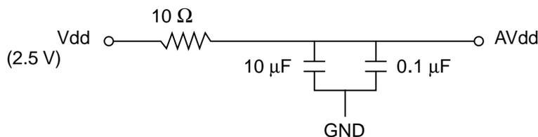
Figure 16. PLL Power Supply Filter Circuit
