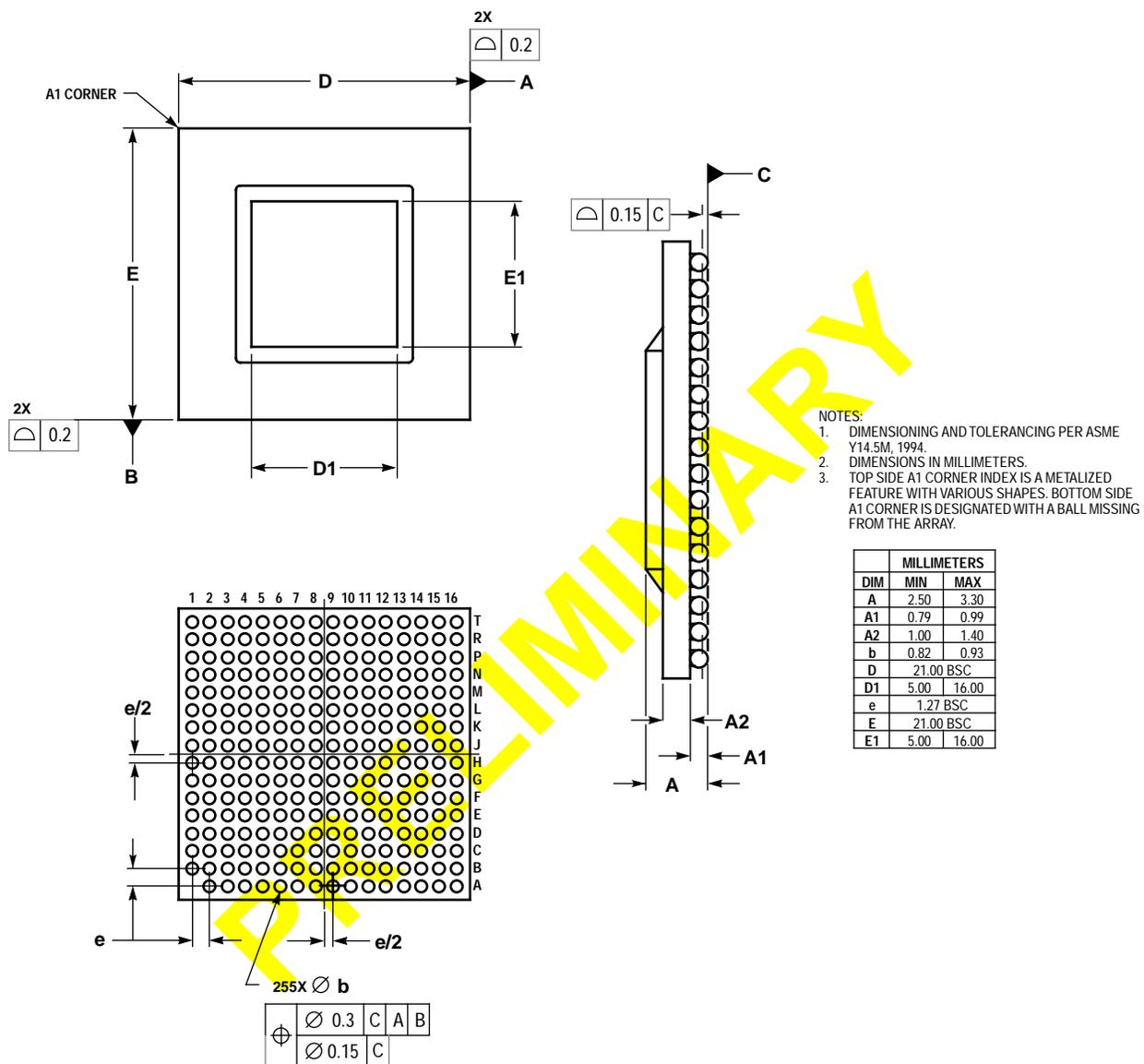
Figure 15. Mechanical Dimensions and Bottom Surface Nomenclature of the BGA Package
