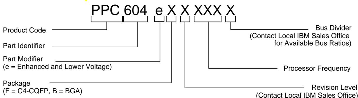
Figure 21. IBM Part Number Key
