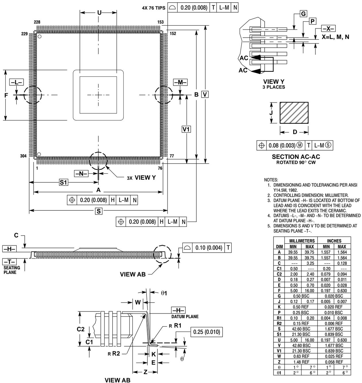
Figure 11. Mechanical Dimensions of the Motorola C4-CQFP Package
