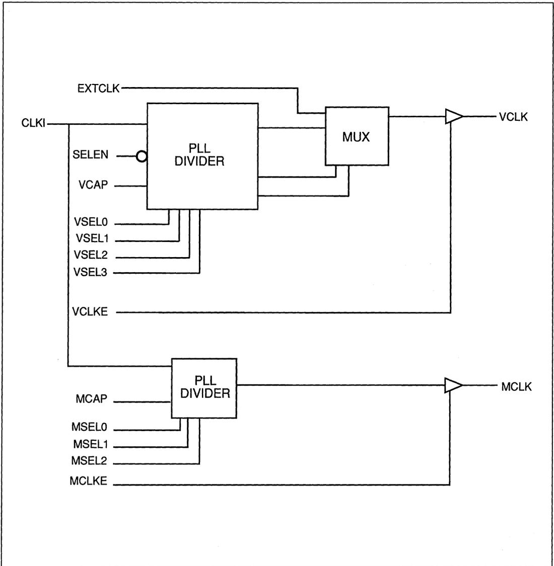
FIGURE 2-2. ICS90C63 FUNCTIONAL BLOCK DIAGRAM
