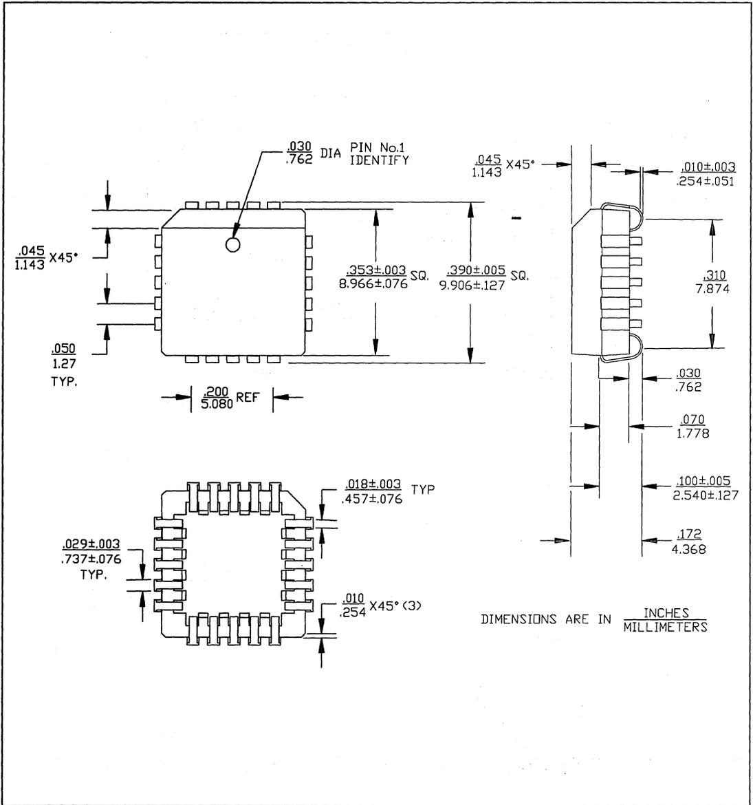
FIGURE 6-1. ICS90C63V 20-PIN PLCC PACKAGE DIMENSIONS
