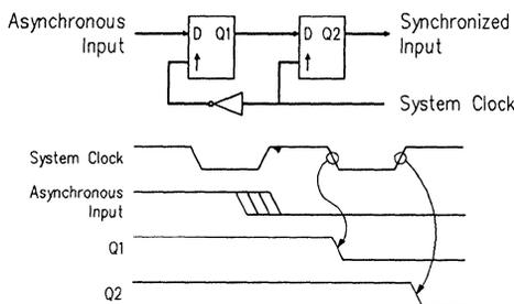
Figure 6. Input synchronization using standard logic
