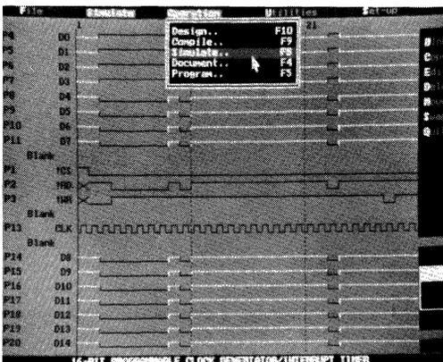
The PACE logic simulator lets external and internal signals be fully simulated, analyzed and edited via a special waveform display. Simulation errors can be marked on the display for quick analysis.
