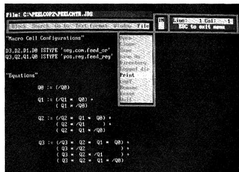
The file editor with pop-down command windows allows for convenient and interactive design entry of APEEL design files.
