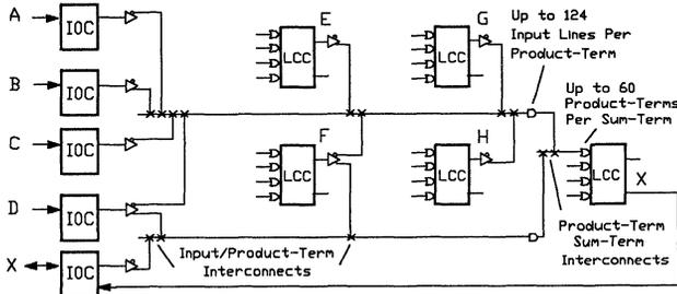
$$X = (\bar{A} * \bar{B} * \bar{C} * \bar{D} * E * \bar{F} * G * H) + (X * D * F)$$
