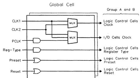
Figure 6. Global Cell for the PA7024 and PA7040
