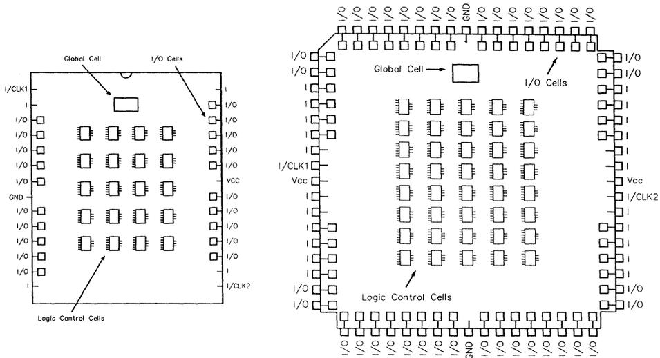
Figure 7. Pin/Block Diagrams for the PA7028 and PA7068
