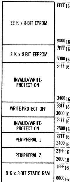
Fig. 4. A block diagram (a) and memory map (b) show the PEEL18CV8 as a Wait-state generator, Address decoder, and Write protector.
