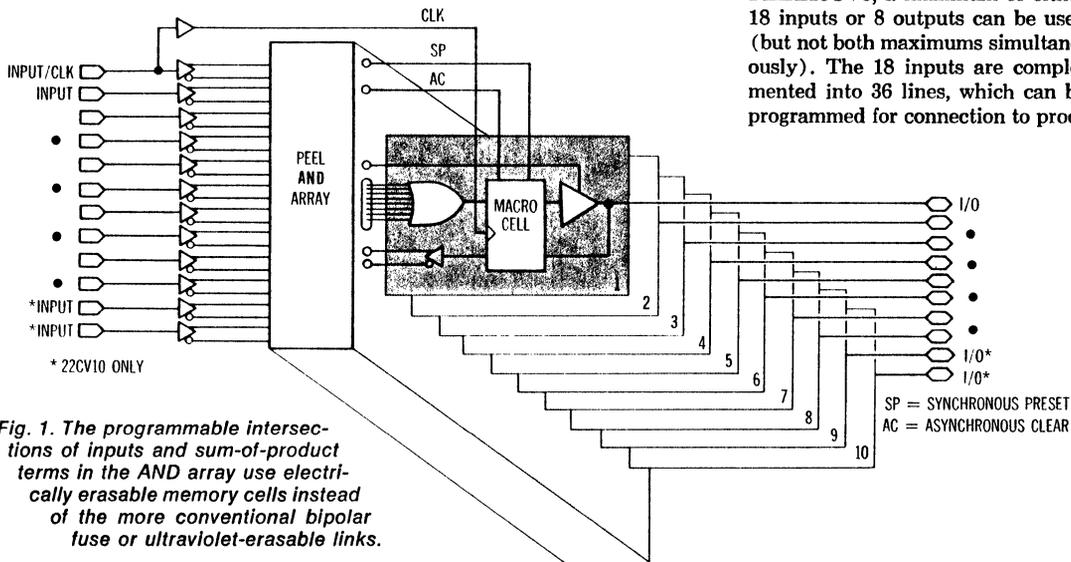
**Fig. 1.** The programmable intersections of inputs and sum-of-product terms in the AND array use electrically erasable memory cells instead of the more conventional bipolar fuse or ultraviolet-erasable links.
