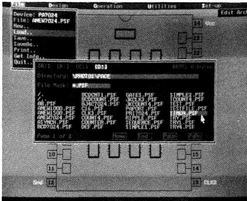
The PACE software functions in a mouse driven windows environment allowing easy access and control of all operations. Shown here is the file selection window.
