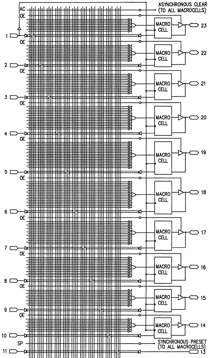
Figure 3. PEEL22CV10 Logic Array Diagram
