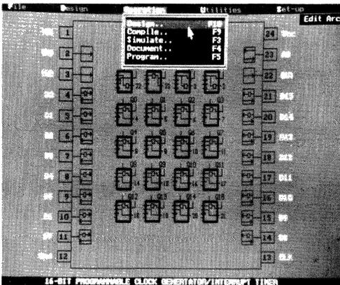
The PACE architectural editors "chip display" provides a global view of design allowing quick access to I/Os, registers, cells and equations.
