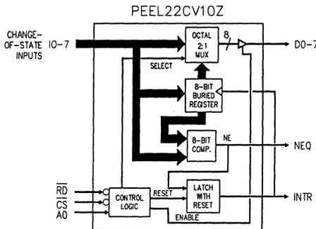
Figure 10. PEEL22CV10Z Change-of-State Detector functional block diagram
