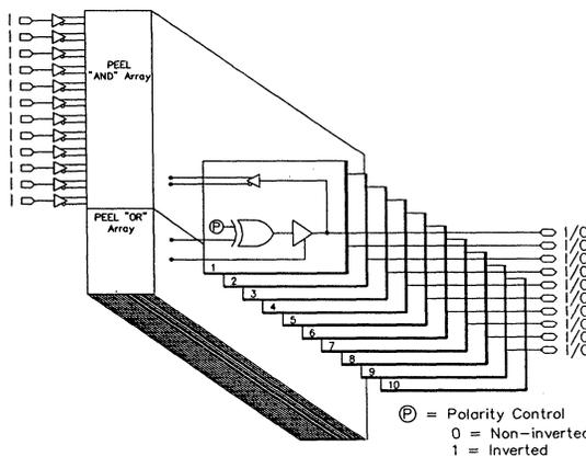
Figure 3. PEEL253 and PEEL273 Block Diagram
