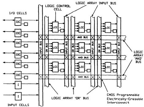
Figure 3. Distributed logic array matrix
