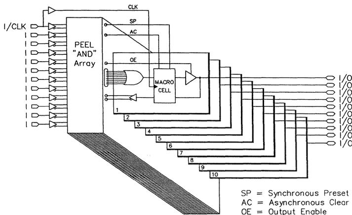
Figure 2. PEEL18CV8, 20CG10 and 22CV10Z Block Diagram
