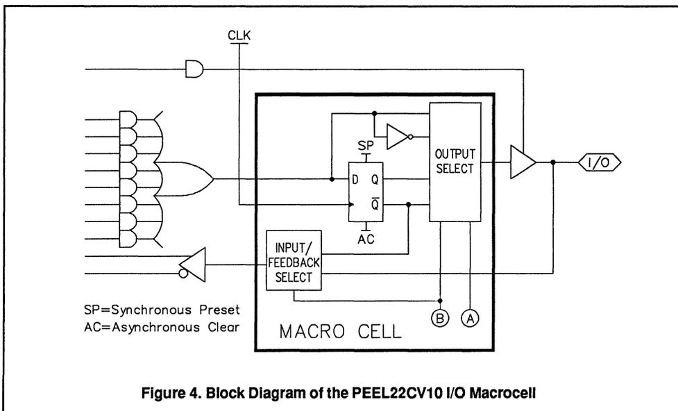
Figure 4. Block Diagram of the PEEL22CV10 I/O Macrocell
