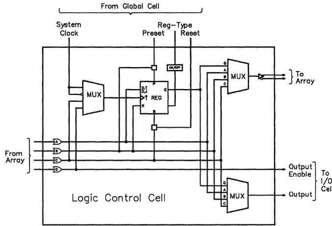
Figure 4. PA7024 Logic Control Cell (LCC)
