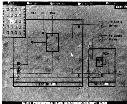
The PACE architectural editor graphically expands individual cells for detailed viewing and control of architecture and equations.
