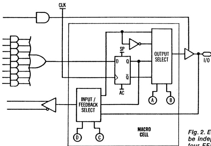
**Fig. 2.** Each I/O pin of a PEEL macrocell can be independently programmed by means of four EEPROM bits to assume one of twelve different I/O configurations.
