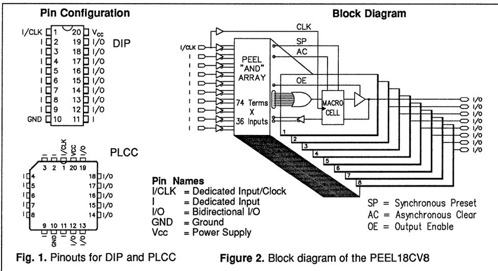
Fig. 1. Pinouts for DIP and PLCC
