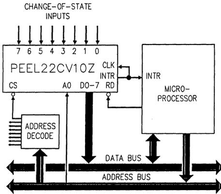
Figure 9. PEEL22CV10Z Change-of-State
