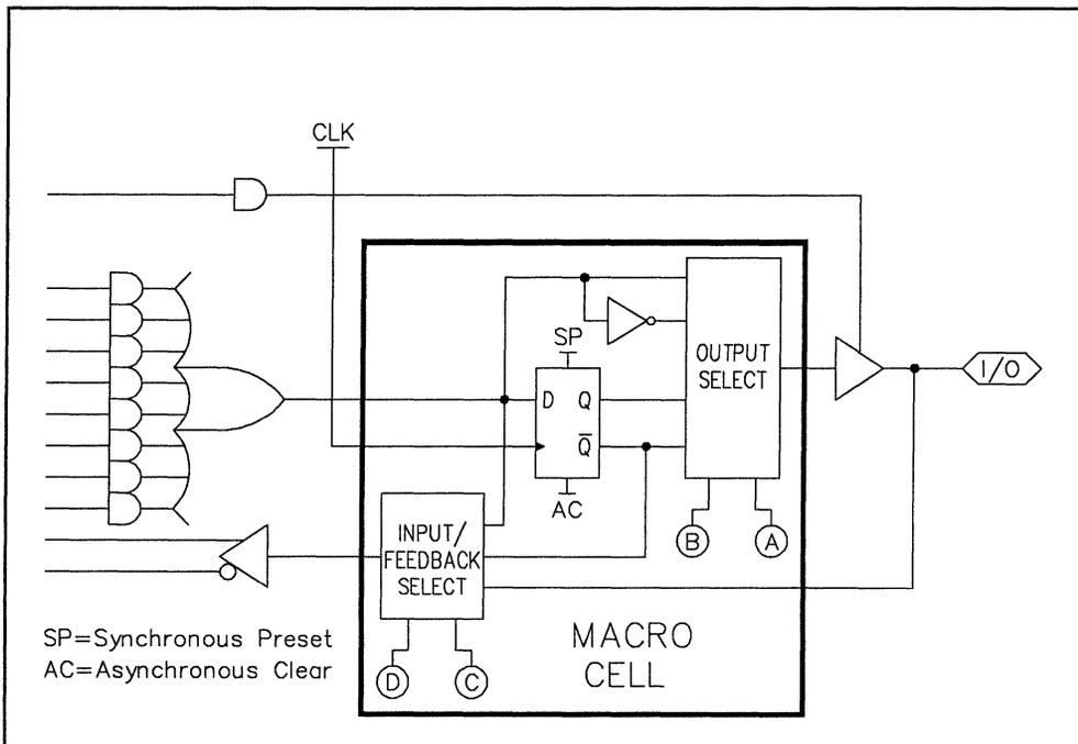
Figure 4. Block Diagram of the PEEL18CV8 I/O Macrocell
