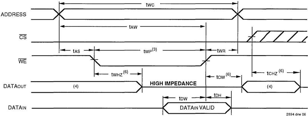
**TIMING WAVEFORM OF WRITE CYCLE NO.2 ( $\overline{CS}$  CONTROLLED TIMING)<sup>(1,2,5)</sup>**
