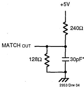
**Figure 1. AC Test Load for MATCH**
