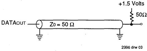
Figure 1. AC Test Load
