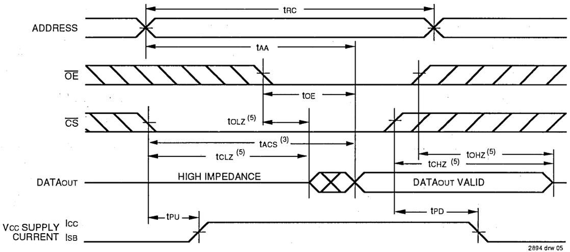
**TIMING WAVEFORM OF READ CYCLE NO. 2<sup>(1,2,4)</sup>**
