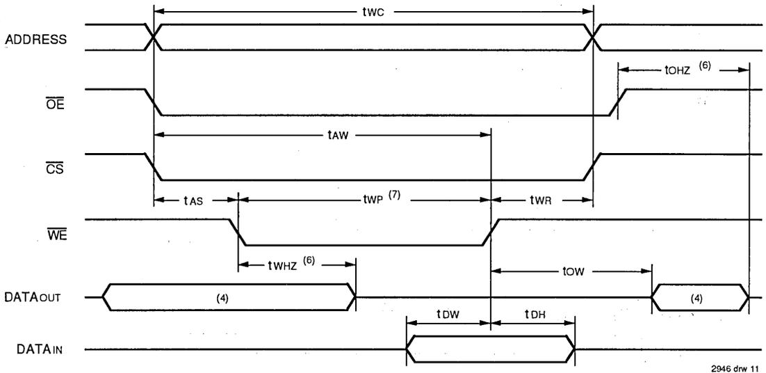
TIMING WAVEFORM OF WRITE CYCLE NO. 2 ( $\overline{CS}$  CONTROLLED TIMING)(1, 2, 3, 5)
