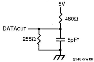
Figure 2. AC Test Load
