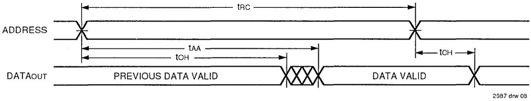
**TIMING WAVEFORM OF READ CYCLE NO. 3<sup>(1, 3, 4)</sup>**
