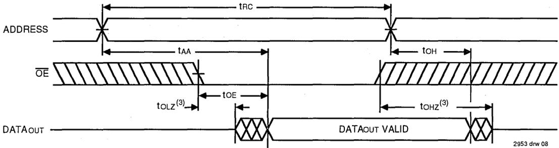
**TIMING WAVEFORM OF READ CYCLE NO. 2<sup>(1,2)</sup>**
