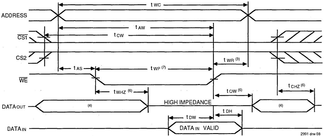
**TIMING WAVEFORM OF WRITE CYCLE NO. 2 ( $\overline{CS1}$  AND  $\overline{CS2}$  CONTROLLED TIMING)<sup>(1, 2, 5)</sup>**
