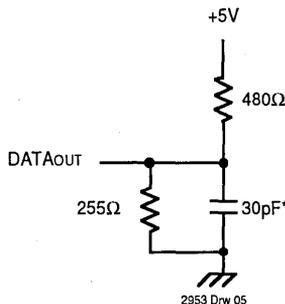
**Figure 2. AC Test Load**
