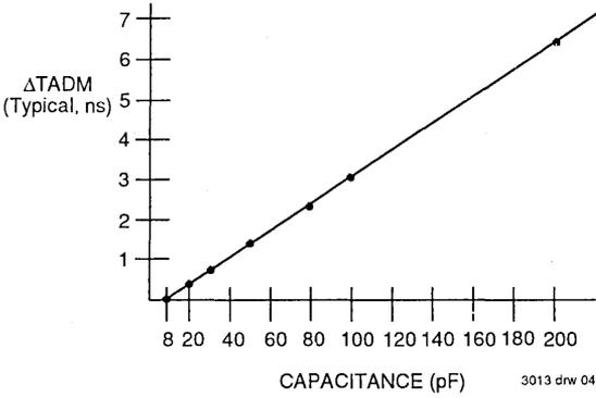
Figure 1A. Lumped Capacitive Load Typical Derating Curve
