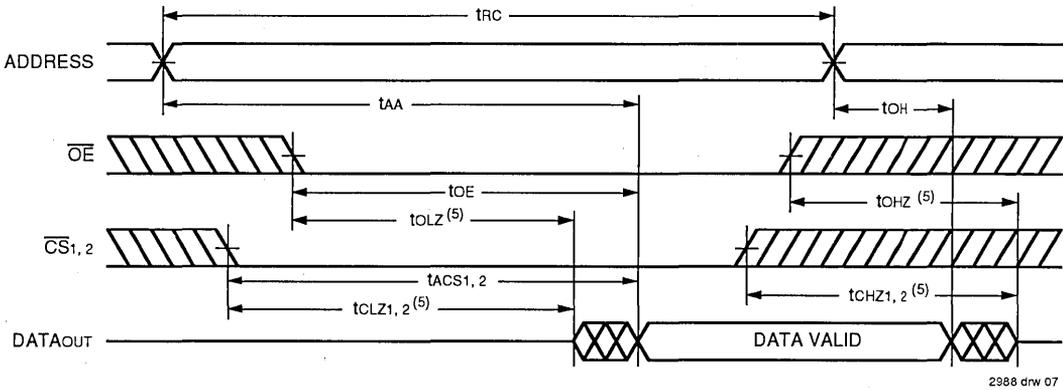
**TIMING WAVEFORM OF READ CYCLE NO. 2<sup>(1, 2, 4)</sup>**
