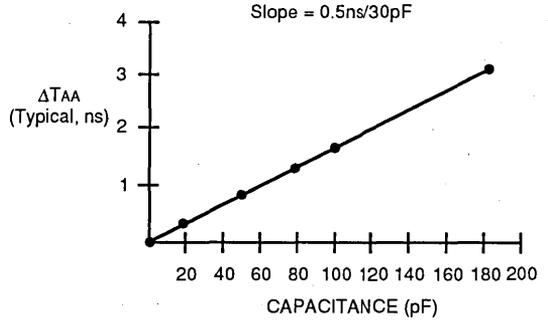
Figure 3. Lumped Capacitive Load, Typical Derating Curve
