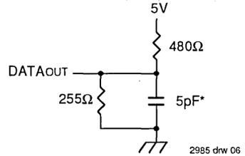
Figure 2. AC Test Load
