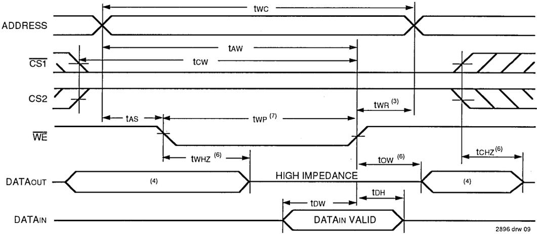
**TIMING WAVEFORM OF WRITE CYCLE NO. 2 ( $\overline{CS1}$  AND CS2 CONTROLLED TIMING)<sup>(1, 2, 5)</sup>**
