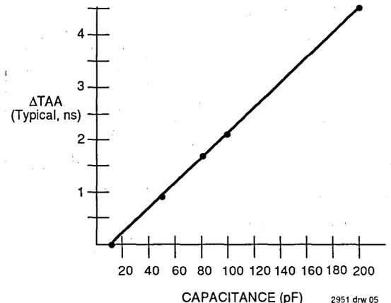
Figure 3. Lumped Capacitive Load, Typical Derating
