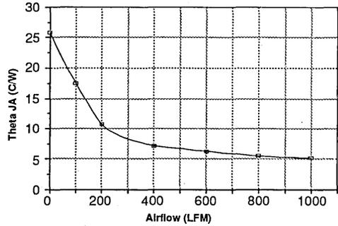
Measurements done with Delco Temp09 Thermal Die (.250"sq.)
