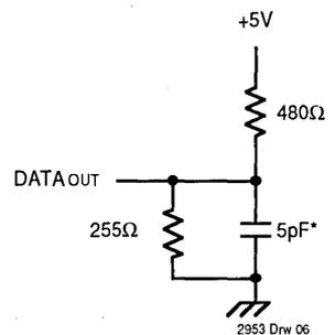
**Figure 3. AC Test Load (for tOLZ, tOHZ, tWHZ, tOW)**
