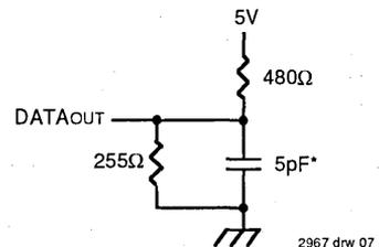
Figure 2. AC Test Load
