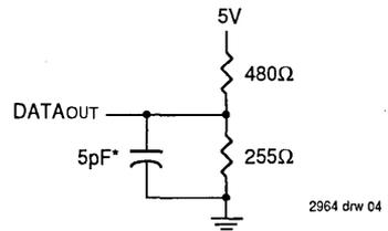
\*Including jig and scope capacitance.
