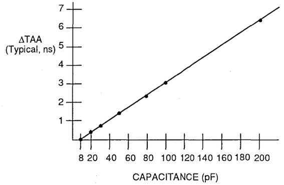
Figure 3A. Lumped Capacitive Load Typical Derating Curve
