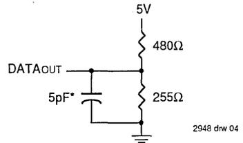
\*Including jig and scope capacitance.
