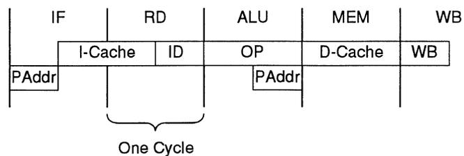
Figure 2.5. 5-Stage Pipeline
