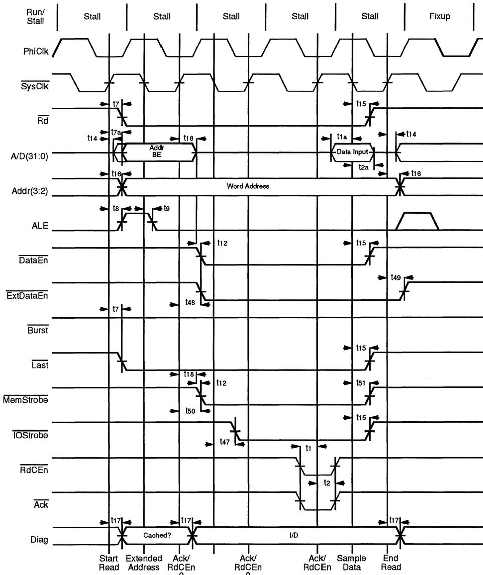
Figure 8.10. Single Word Read With Bus Wait Cycles
