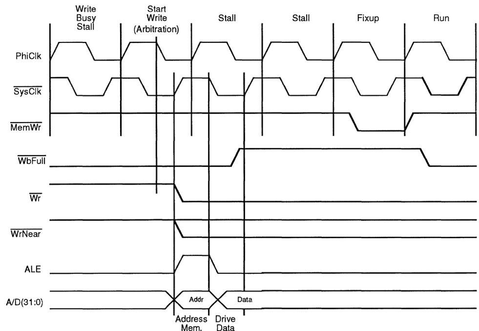
**Figure 9.5. Write Buffer Full Operation**
