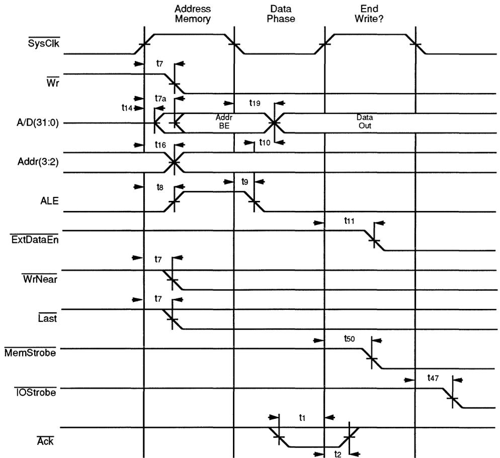
**Figure 9.2. Memory Addressing and Start of Write for non ExtAddrHold Mode**
