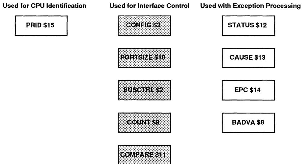
Figure 5.1. R3041 Bus Interface Control Registers
