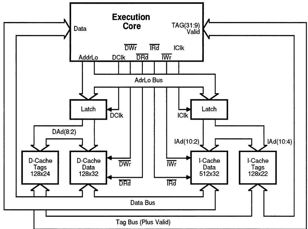
Figure 3.2. R3041 Execution Core and Cache Interface
