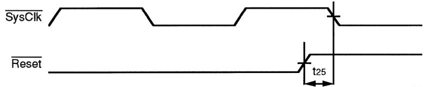
Figure 11.6. Reset Timing
