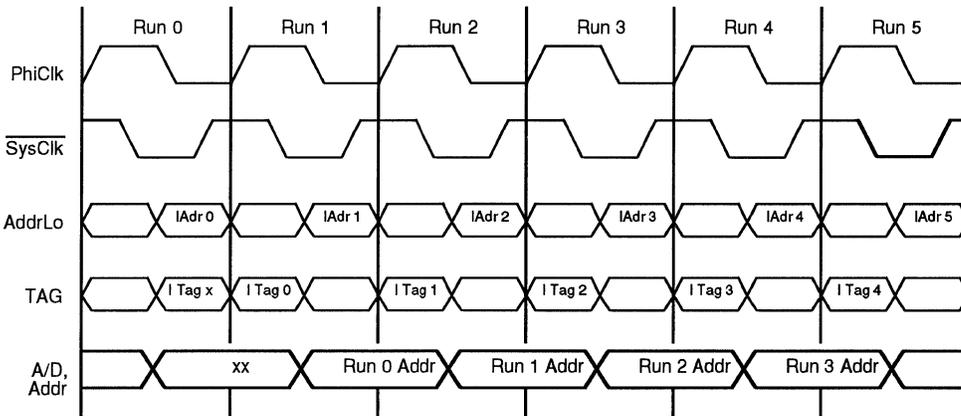
Figure 12.1. R3041 Debug Mode Instruction Address Display
