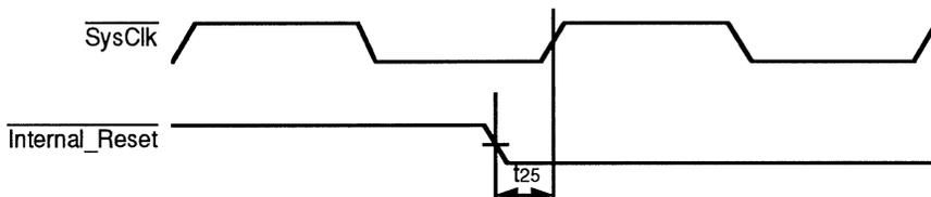
Figure 12.3. R3041 SysClk Phase Initialization Case B
