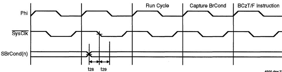
Figure 6.8. Synchronized BrCond Inputs
