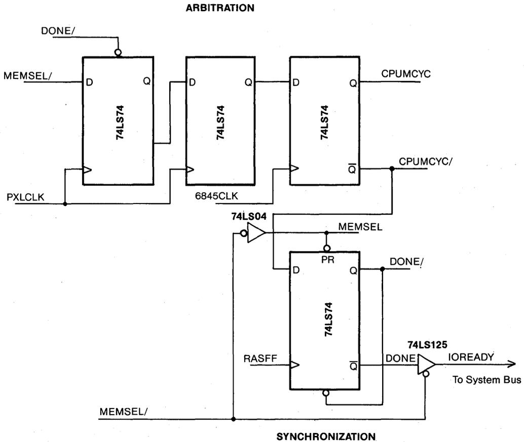
**Figure 6. Arbitration and Synchronization**
