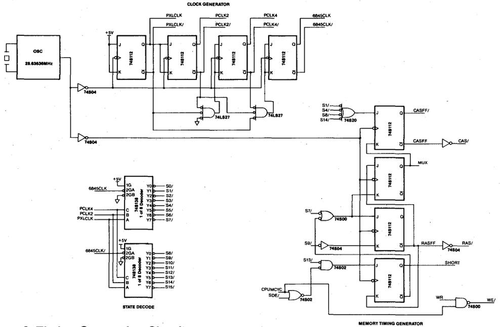
Figure 3. Timing Generation Circuits
