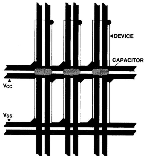
**$V_{CC}$ ,  $V_{SS}$  GRID SHOWING
