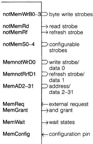
The memory interface uses a 32-bit wide address/data bus and its controller may be configured, on reset, to suit a wide variety of different memory systems. One of 13 preset configurations may be selected or the configuration may be supplied externally.
