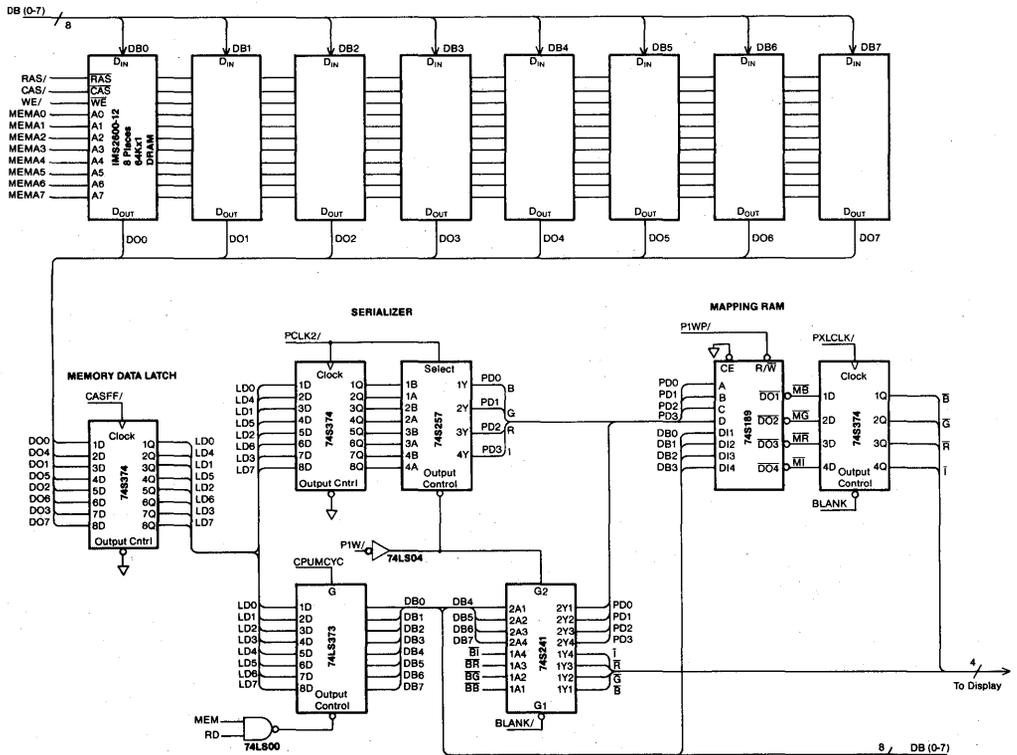
Figure 4. Data Flow Circuits
