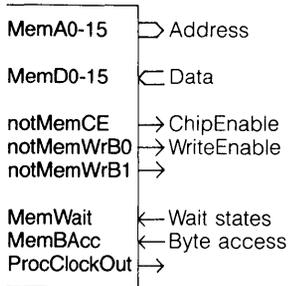
The memory interface consists of a 16 bit address bus and a 16 bit data bus. It performs word reads and word writes in 2 processor cycles. A processor cycle is identified by **ProcClockOut**.
