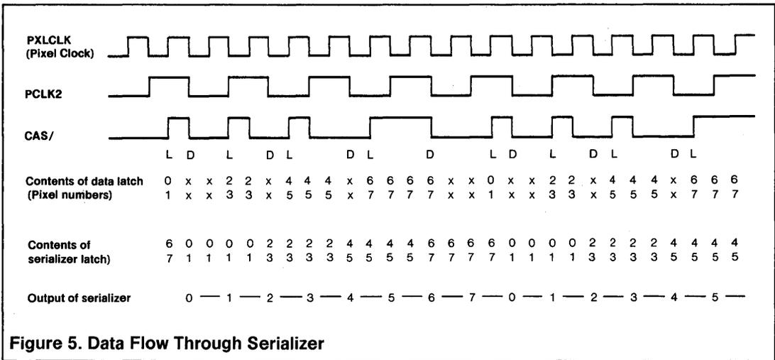
**Figure 5. Data Flow Through Serializer**
