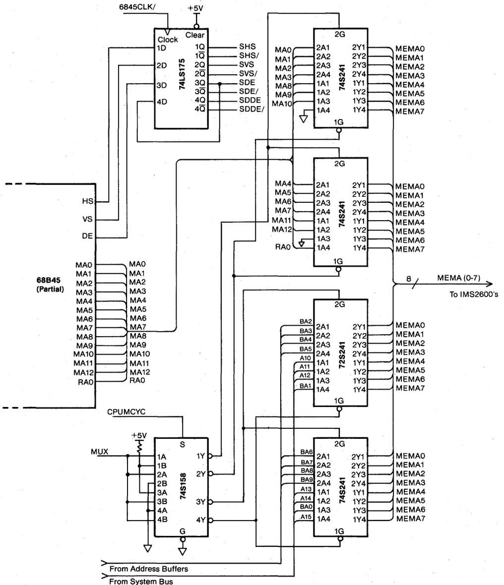
Figure 7. Address Multiplexing Circuits
