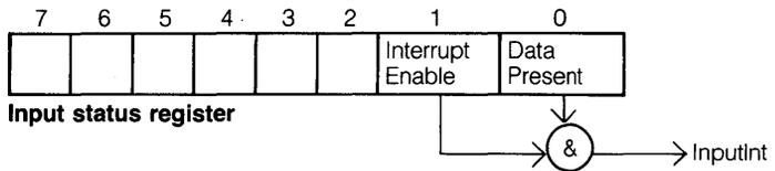
The **data present** status bit indicates that the serial link has received a byte of data. It is reset when the data byte is read from the input data register on the parallel interface, this causes an acknowledgement to be transmitted on the serial link. **InputInt** is set if both **data present** and **interrupt enable** are set.
