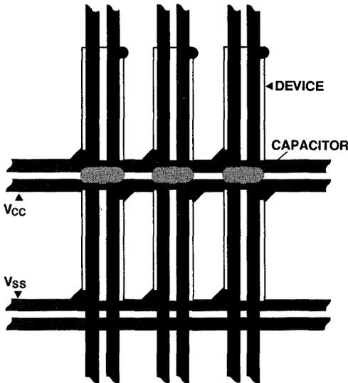
$V_{CC}$ ,  $V_{SS}$  GRID SHOWING
