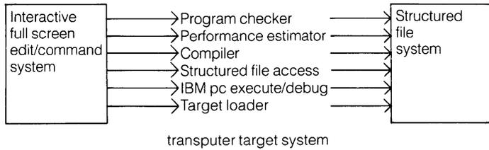
The transputer development system runs on an IBM Personal Computer with 640K bytes of RAM and hard disk under DOS. It provides all the facilities of the occam programming system, and is entered by a simple DOS command. Within the system the user edits, compiles and debugs occam programs, exploiting the full screen text editing facilities and using function keys to access the capabilities of the toolset provided by the system.
