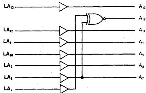
Figure 2: IMS1400 Address Encoder Circuit
