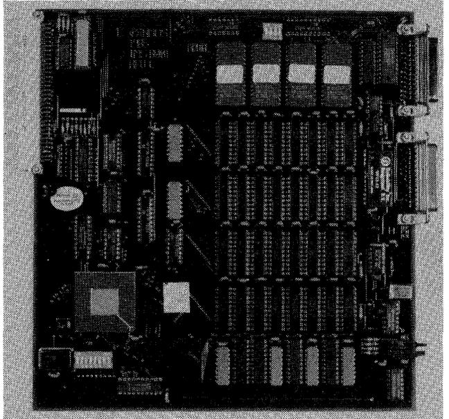
The IMS B001 evaluation board enables users to evaluate and demonstrate the use of transputers. The board is the first of a family of compatible evaluation boards. It provides standard buffered INMOS link connections and external control of the transputer's Reset and Analyse functions. This allows it to control a subsystem consisting of other compatible boards, or to be a component of such a subsystem.
