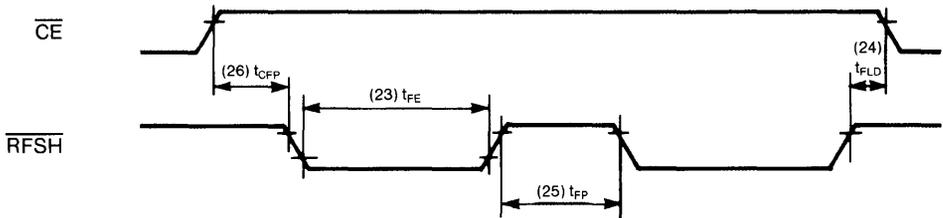
**$\overline{CE}$  REFRESH CYCLE  $CS \leq V_{IL}, \overline{RFSH} \geq V_{IH}, \overline{OE}, \overline{W} = \text{DON'T CARE}$**
