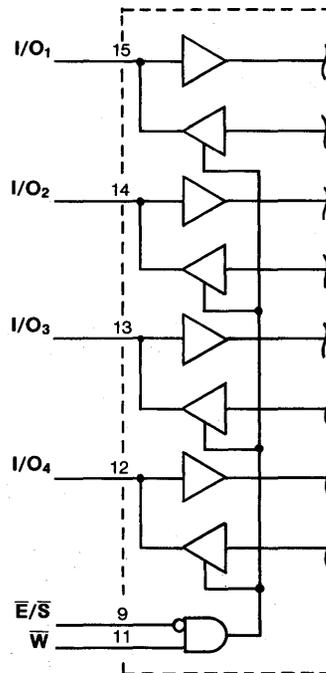
Figure 2: IMS1420/1421 I/O Buffer Enable Conditions
