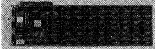
The IMS B004 IBM PC add-in board enables users to evaluate and demonstrate the use of transputers. Containing a 32 bit transputer, the board provides a powerful upgrade to the IBM PC. The board is one of a family of compatible evaluation boards. It provides standard buffered INMOS link connections and external control of the transputer's Reset and Analyse functions. This allows it to control a subsystem consisting of other compatible boards, or to be a component of such a subsystem.
