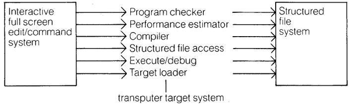
The transputer development station provides all the facilities of the occam programming system on a self contained workstation. Within the system the user edits, compiles and debugs occam programs, exploiting the full screen text editing facilities and using function keys to access the capabilities of the toolset provided by the system.
