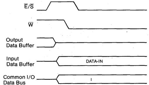
Figure 4:  $\bar{E}/\bar{S}$  Used to Control Output Buffer (No Contention)
