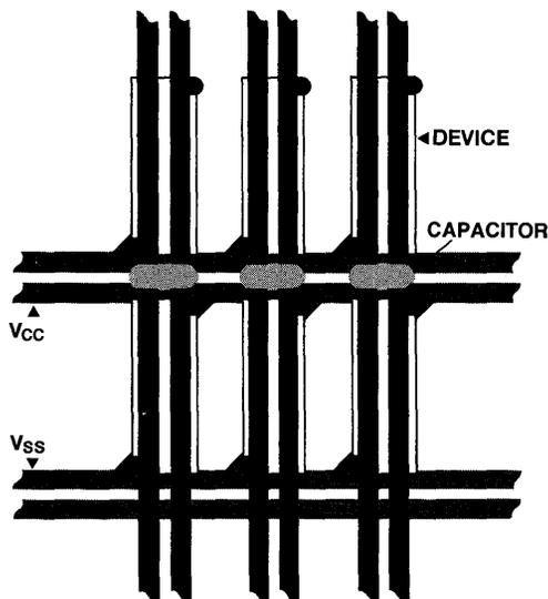
**$V_{CC}$ ,  $V_{SS}$  GRID SHOWING
