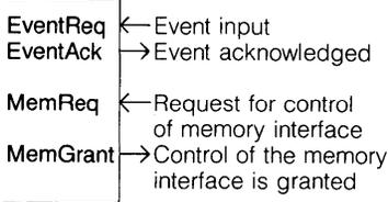
An interrupt request from a peripheral may be signalled via the **EventReq** pin, which is handshaken using **EventAck**. This will normally be used to trigger a high priority process. The request appears to the process as an input on a hardware channel.
