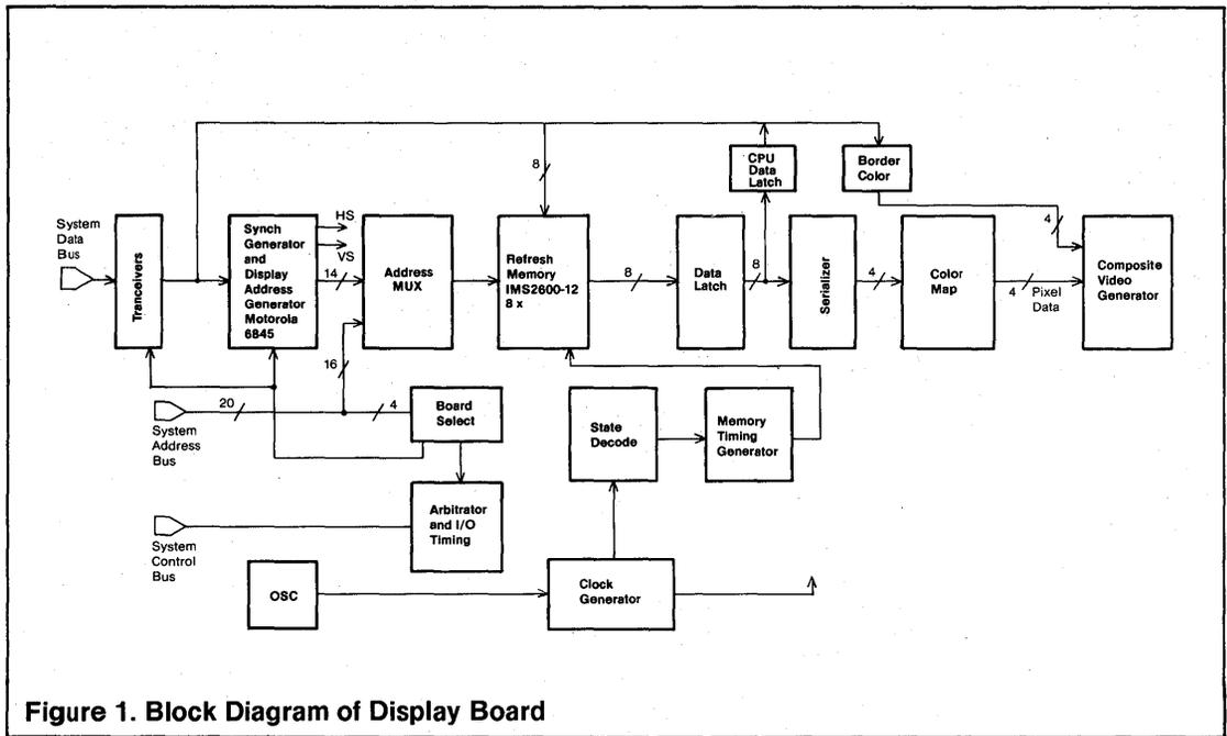
**Figure 1. Block Diagram of Display Board**
