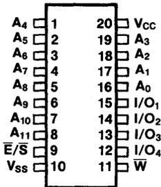
Figure 1: IMS1420/1421 Pin Configuration
