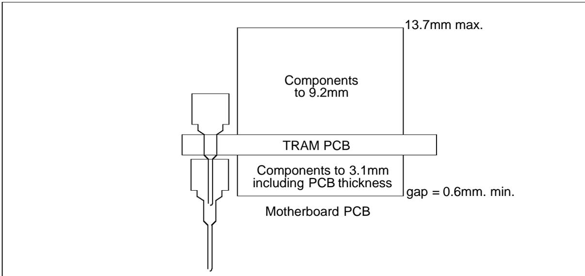
Figure 1.2 IMS B452 height specification
