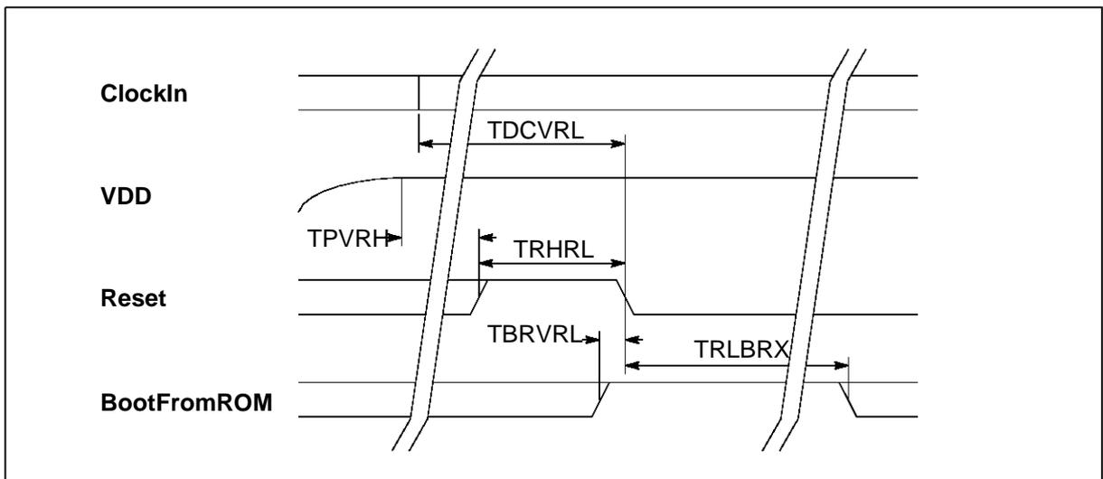
Figure 4.4 Transputer **Reset** timing with **Analyse** low
