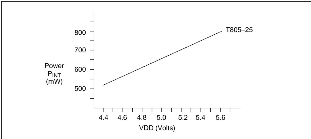
Figure 9.6 IMS T805 internal power dissipation vs VDD
