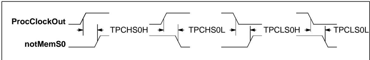
Figure 6.7 IMS T805 skew of **notMemS0** to **ProcClockOut**
