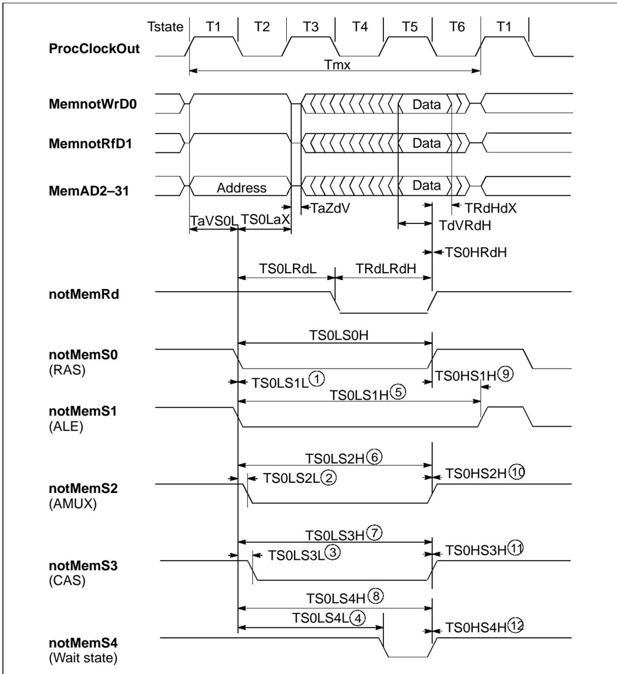
Figure 6.5 IMS T805 external read cycle: dynamic memory
