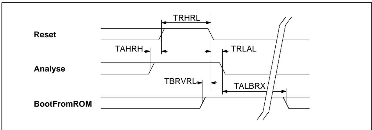
Figure 4.5 Transputer **Reset**, **Analyse** and **BootFromROM** timing
