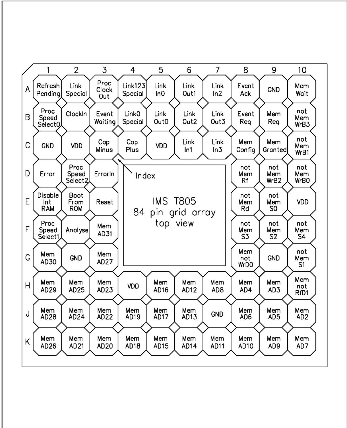
Figure 10.1 IMS T805 84-pin grid array package pinout
