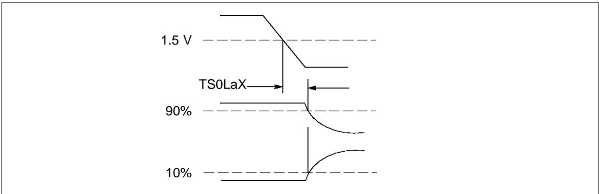
Figure 9.4 IMS T805 tristate timing relative to **notMemS0**
