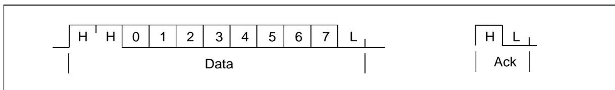
Figure 8.1 IMS T805 link data and acknowledge packets
