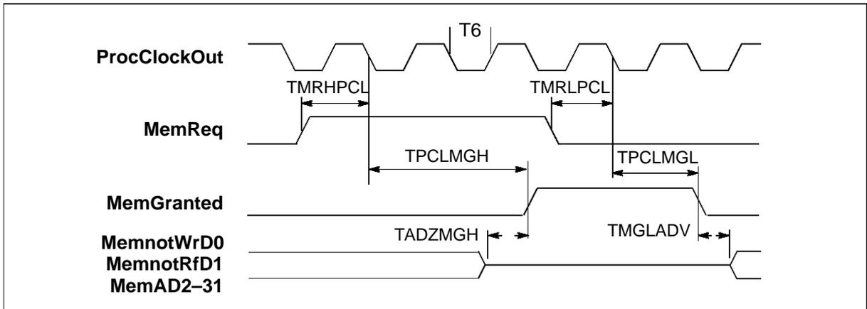
Figure 6.13 IMS T805 memory request timing
