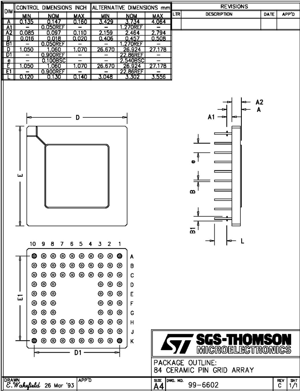
Figure 10.2 IMS T805 84-pin grid array package dimensions
