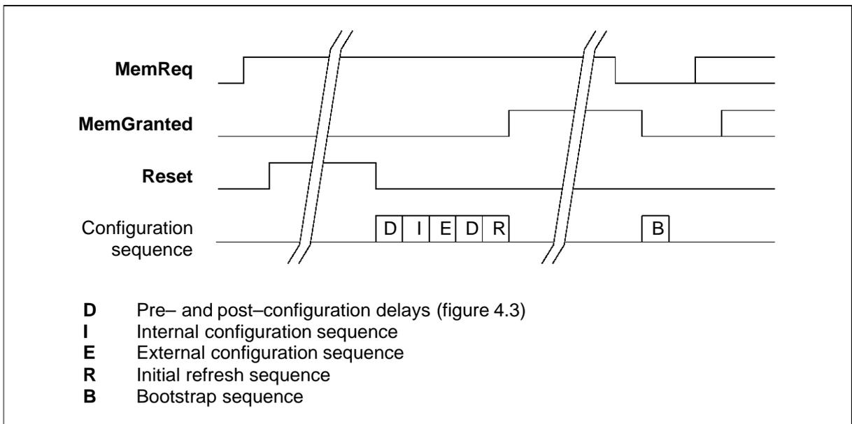
Figure 6.14 IMS T805 DMA sequence at reset
