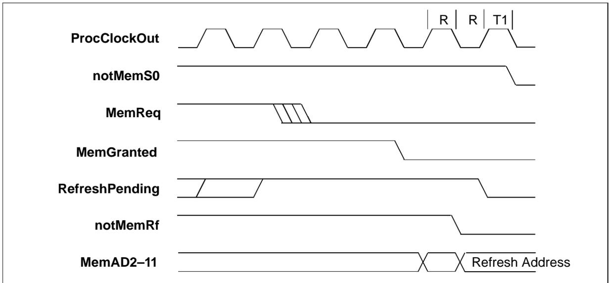
Figure 6.12 IMS T805 refresh pending timing diagram
