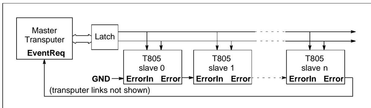
Figure 4.6 Error handling in a multi-transputer system
