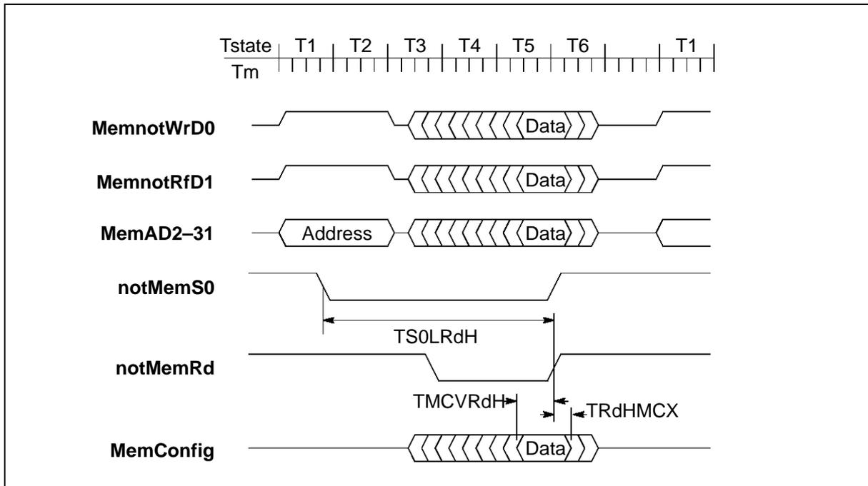
Figure 6.21 IMS T805 external configuration read cycle timing
