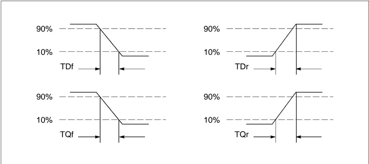
Figure 9.3 IMS T805 input and output edge timing
