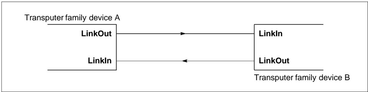
Figure 8.4 Links directly connected
