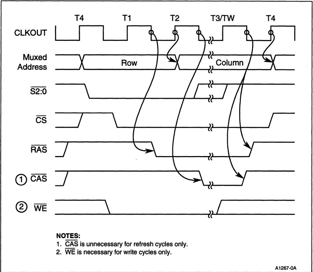
**Figure 7-4. Suggested DRAM Control Signal Timing Relationships**
