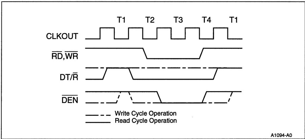
Figure 3-30.  $\overline{DEN}$  and  $DT/\overline{R}$  Timing Relationships
