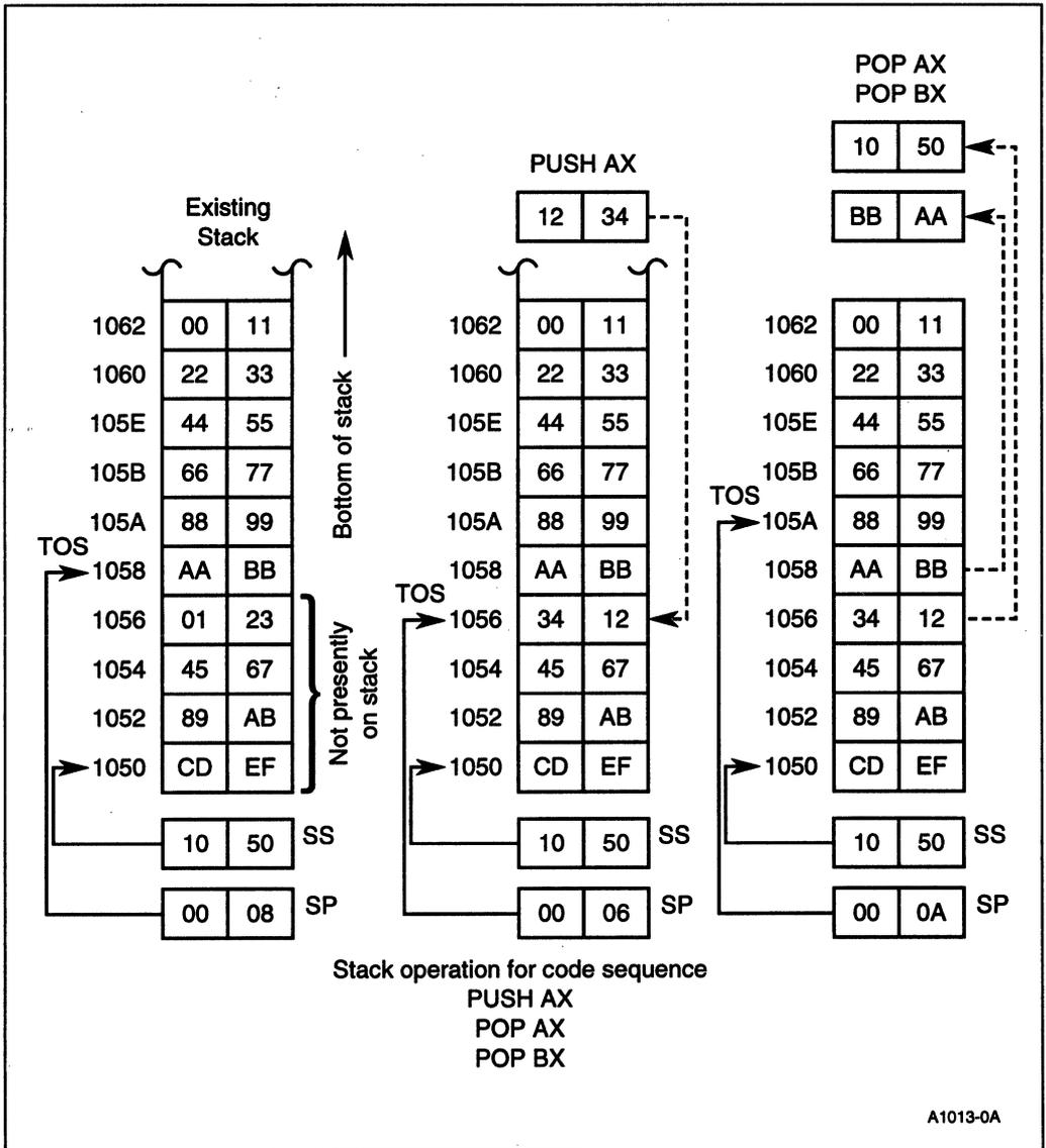
Figure 2-10. Stack Operation
