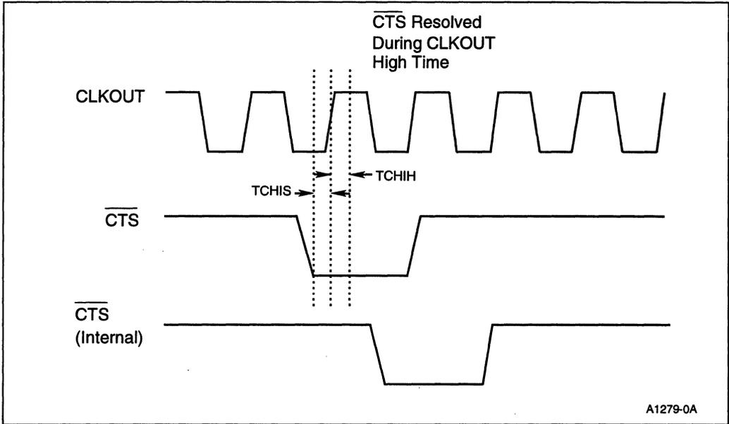
Figure 10-15.  $\overline{\text{CTS}}$  Recognition Sequence
