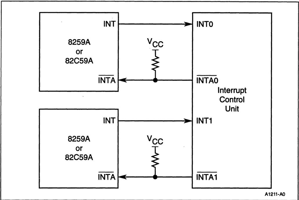
Figure 8-2. Using External 8259A Modules in Cascade Mode
