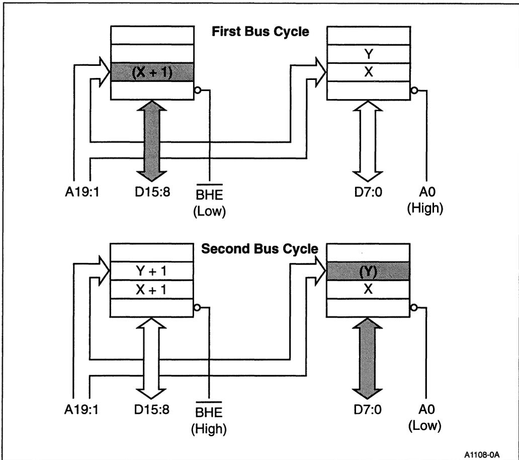
**Figure 3-4. 16-Bit Data Bus Odd Word Transfers**
