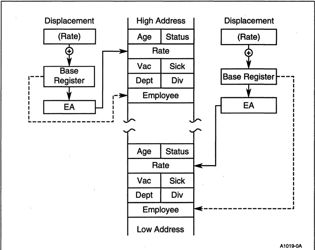
**Figure 2-16. Accessing a Structure with Based Addressing**
