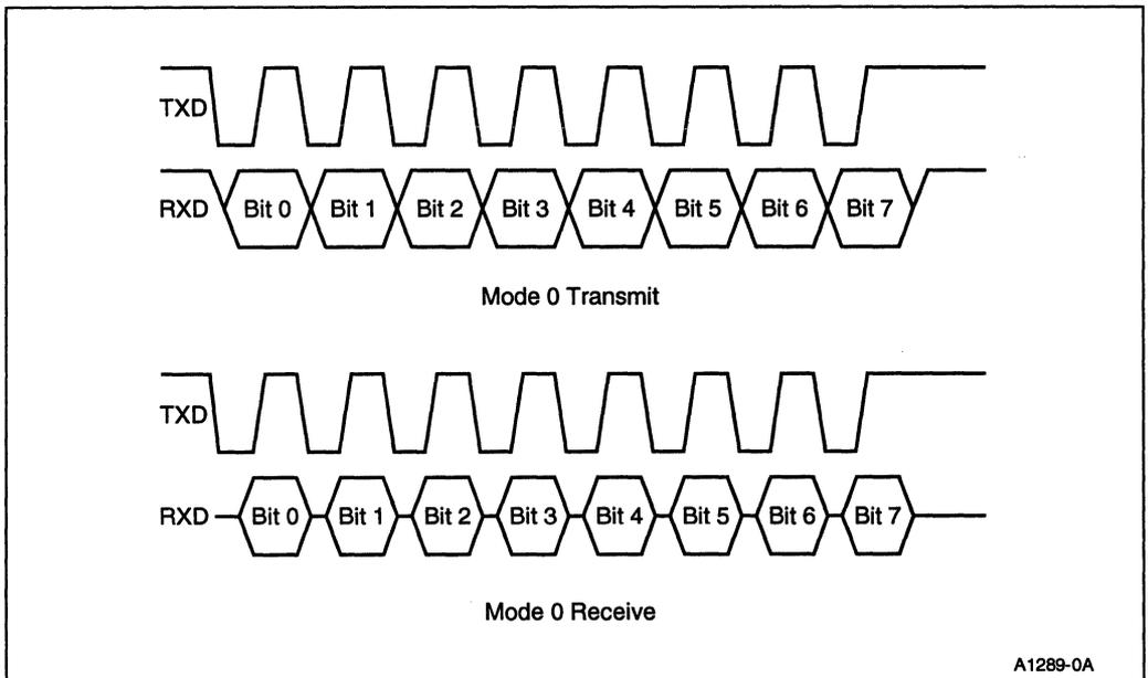
Figure 10-7. Mode 0 Waveforms
