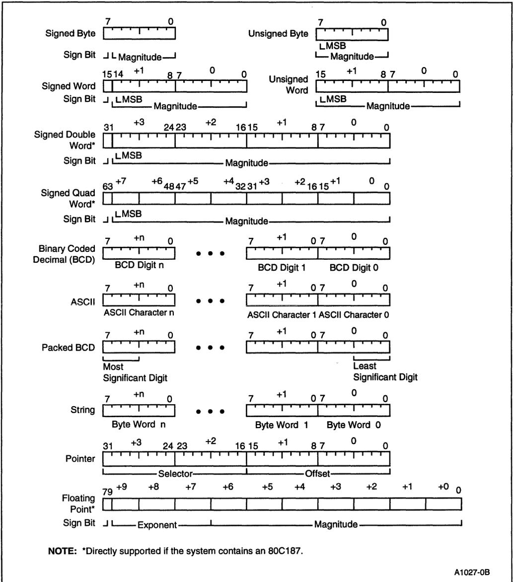
Figure 2-23. 80C186 Modular Core Family Supported Data Types
