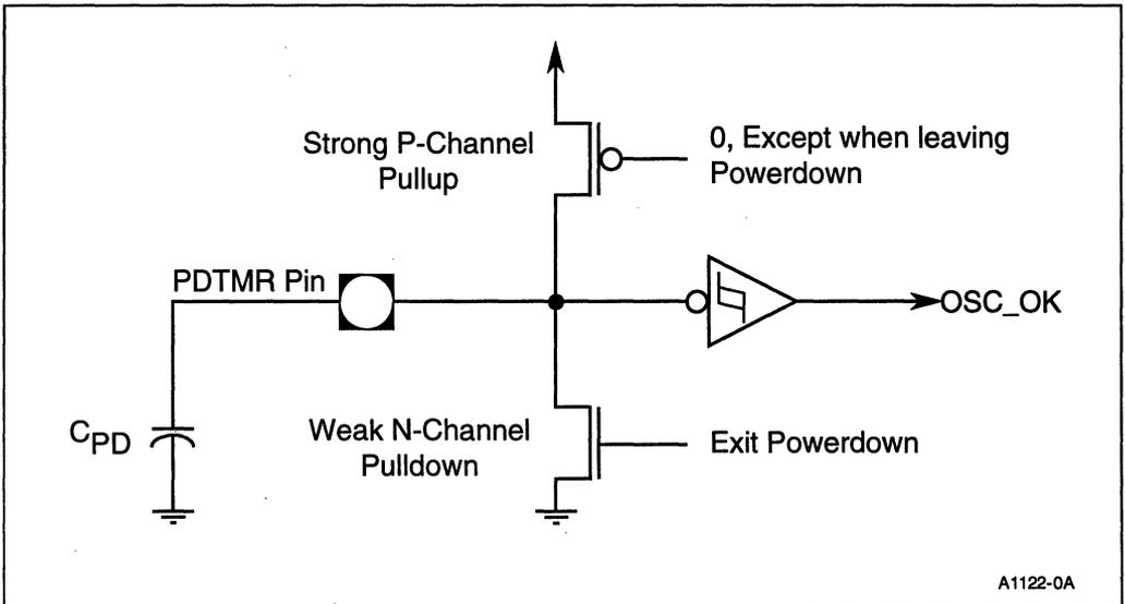
Figure 5-13. Powerdown Timer Circuit
