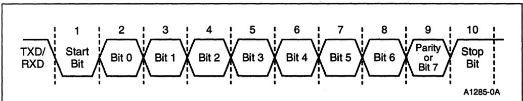
**Figure 10-4. Mode 1 Waveform**
