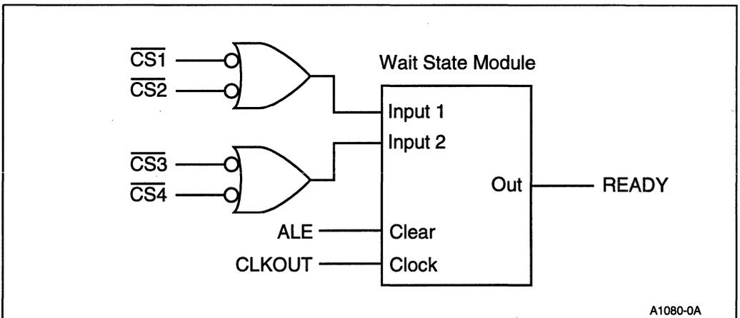
**Figure 3-15. Generating a Normally Not-Ready Bus Signal**
