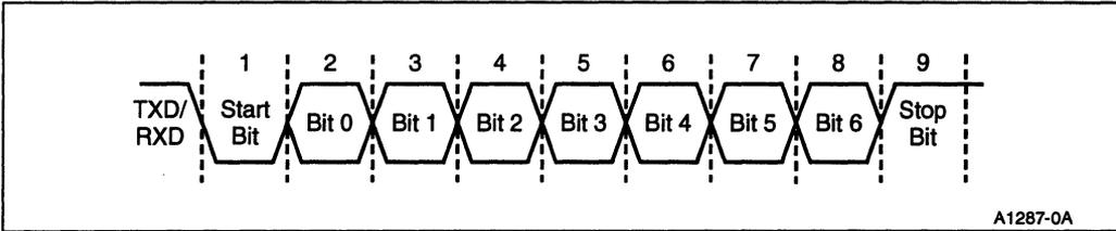
Figure 10-6. Mode 4 Waveform
