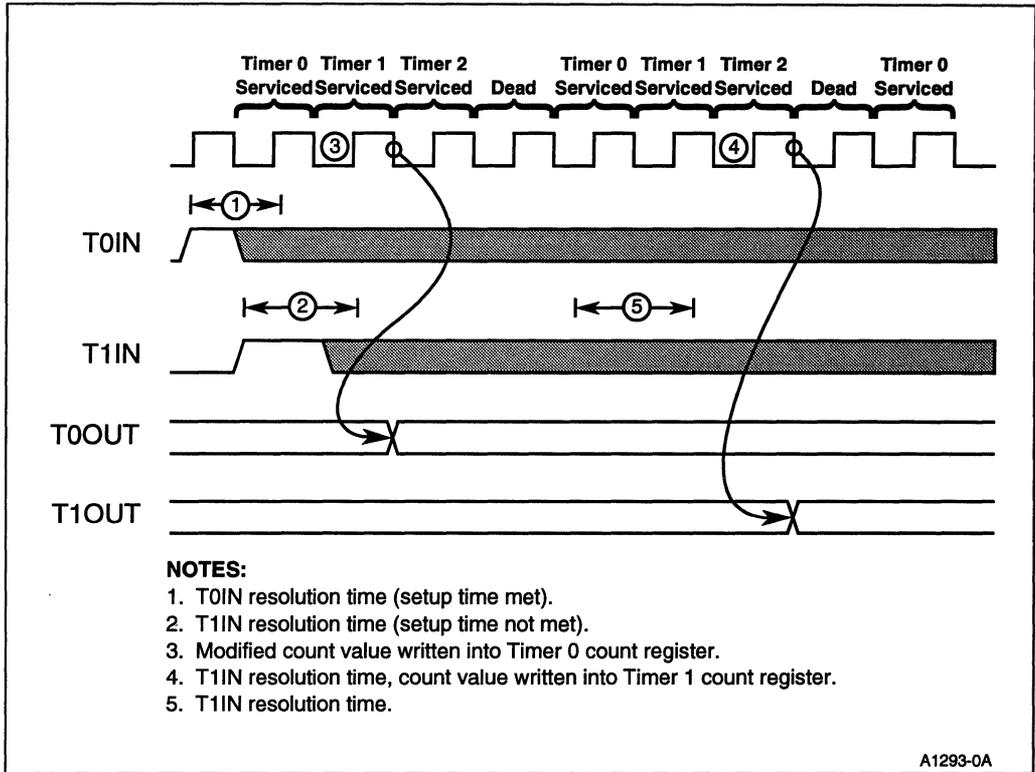
Figure 9-2. Counter Element Multiplexing and Timer Input Synchronization
