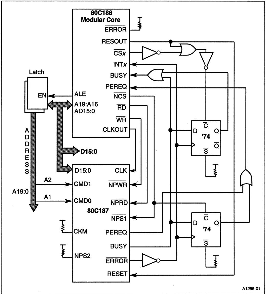
Figure 12-4. 80C187 Exception Trapping via Processor Interrupt Pin
