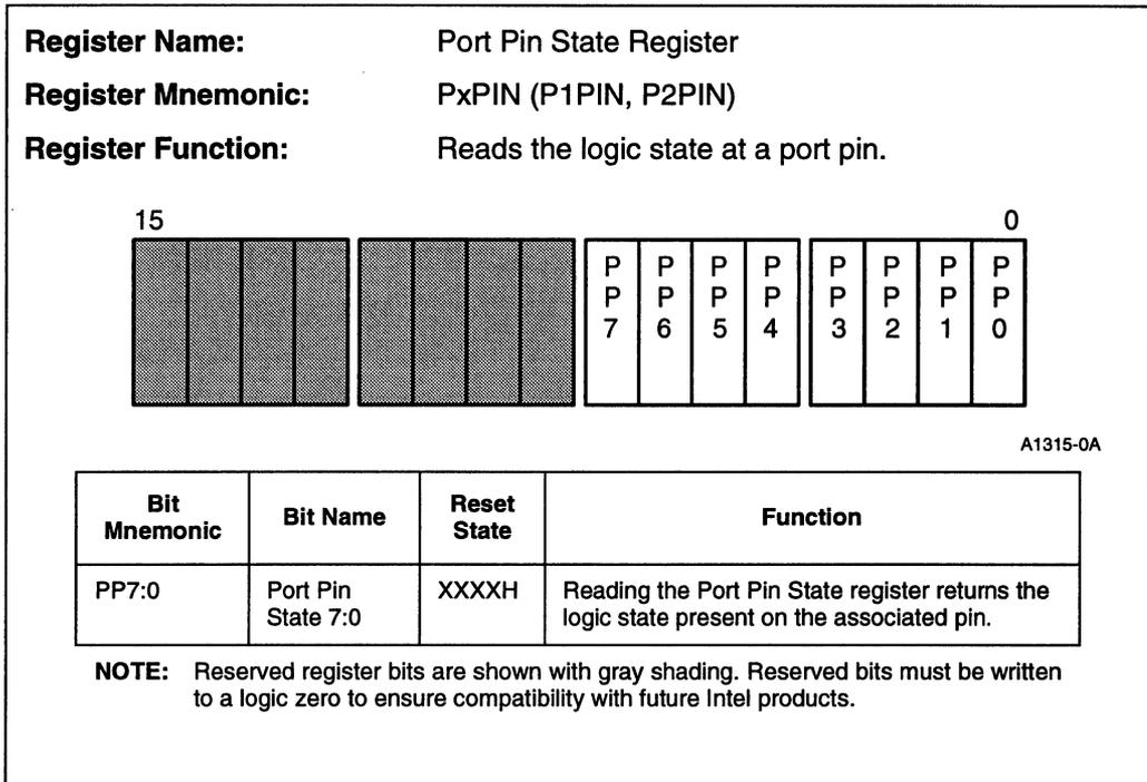
**Figure 11-8. Port Pin State Register (P<sub>x</sub>PIN)**
