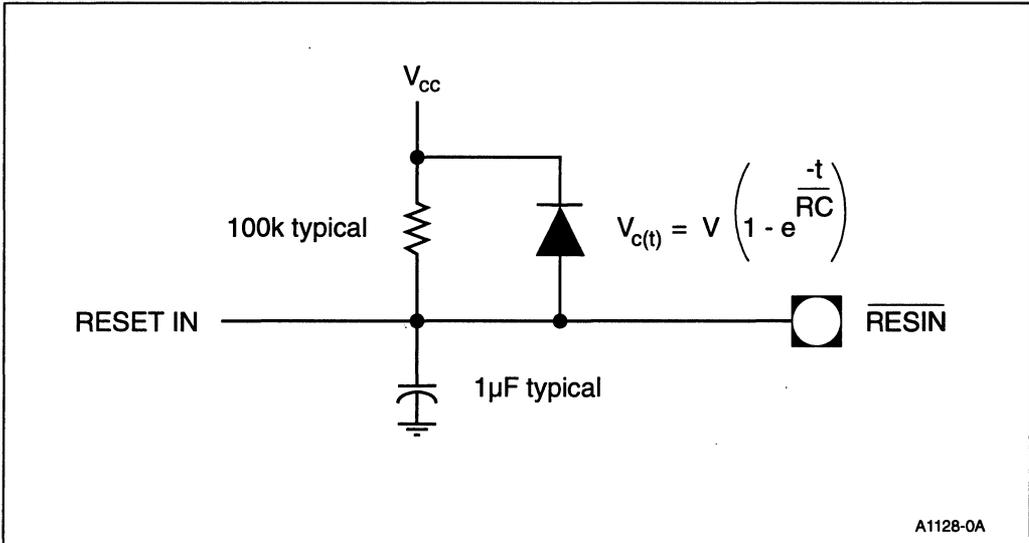
**Figure 5-5. Simple RC Circuit for Powerup Reset**
