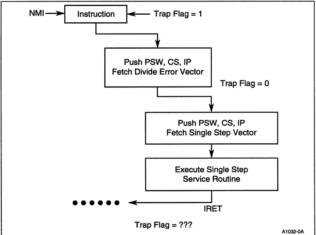
**Figure 2-29. Simultaneous NMI and Single Step Interrupts**
