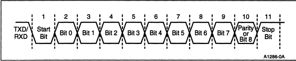
Figure 10-5. Mode 3 Waveform
