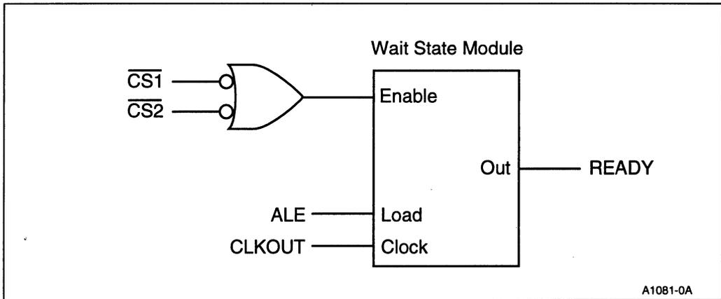
**Figure 3-16. Generating a Normally Ready Bus Signal**
