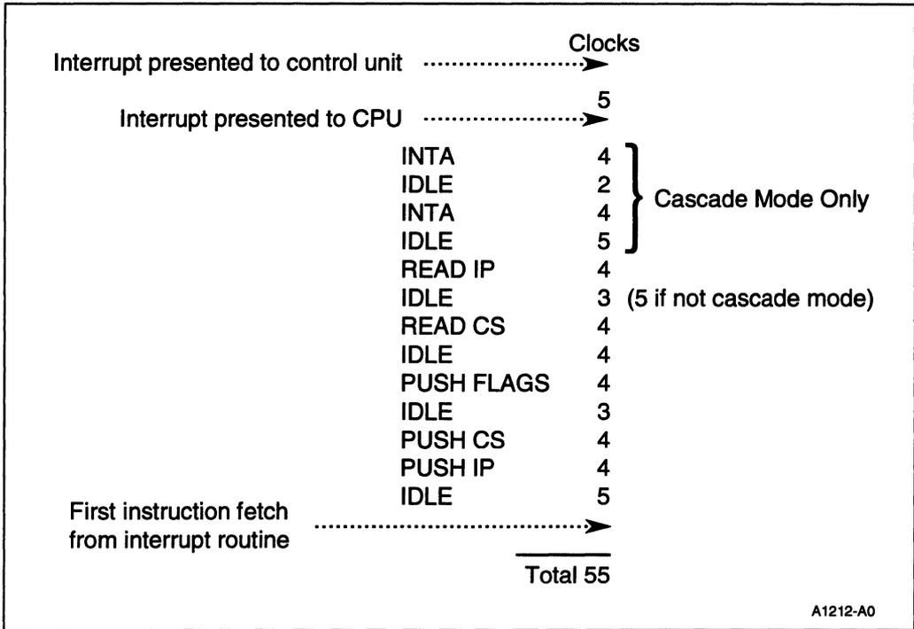
Figure 8-3. Interrupt Control Unit Latency and Response Time
