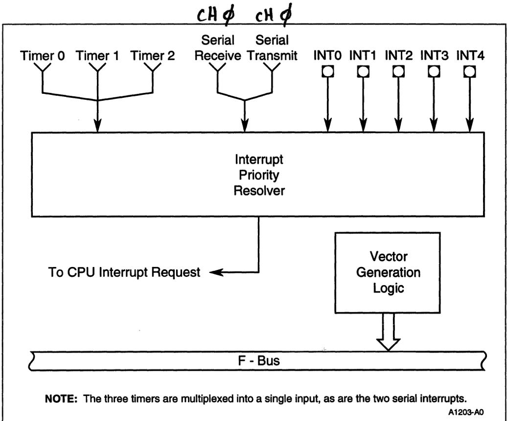
Figure 8-1. Interrupt Control Unit Block Diagram
