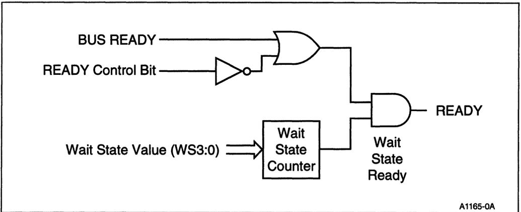
**Figure 6-7. Wait State and Ready Control Functions**
