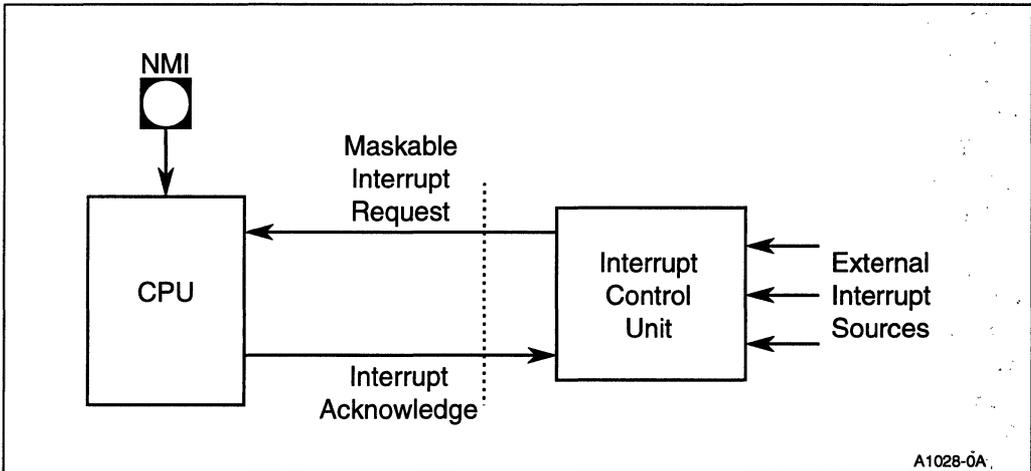
Figure 2-24. Interrupt Control Unit
