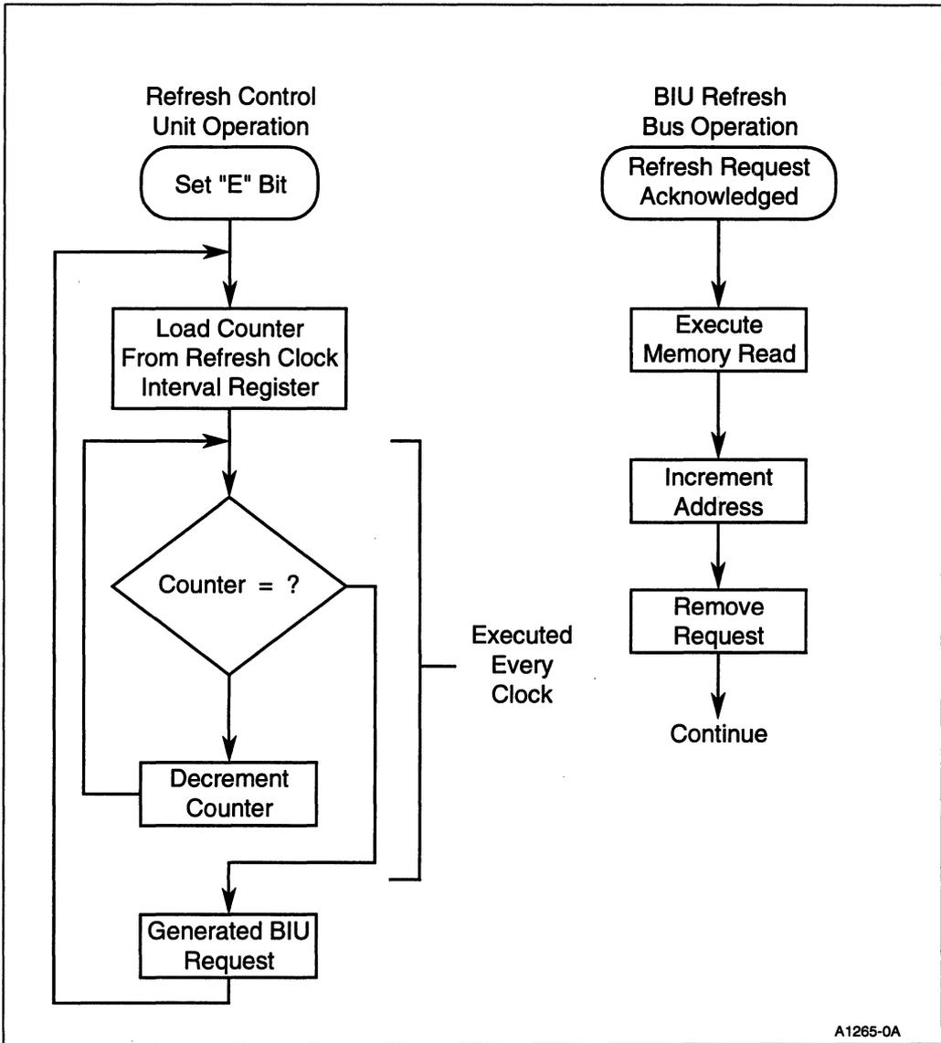
**Figure 7-2. Refresh Control Unit Operation Flow Chart**
