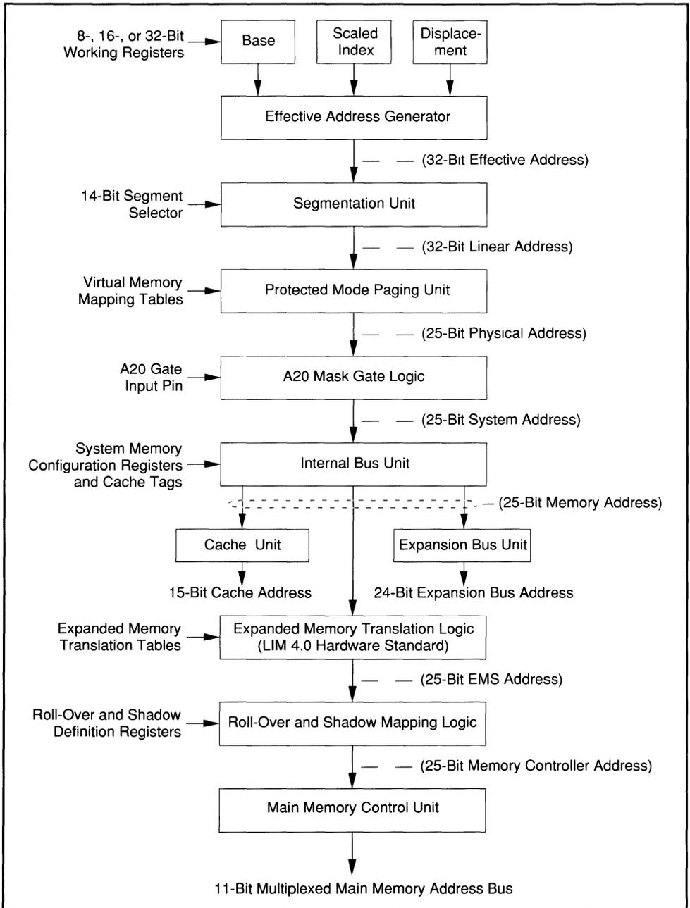
**Figure 3-1. Intel386™ SL Processor Memory Address Translation Logic Eliminates External Propagation Delays**
