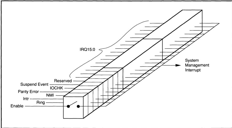
Figure 4-3. System Management Interrupt Requests and Mask Registers
