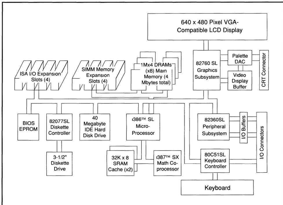
Figure 5-4. Lap-Top PC Block Diagram
