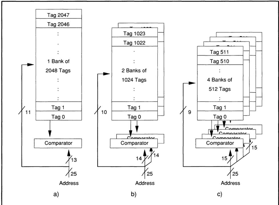
**Figure 2-6. 64K Cache Set-Associativity Options: (a) Direct-Mapped, (b) Two-Way, or (c) Four-Way**
