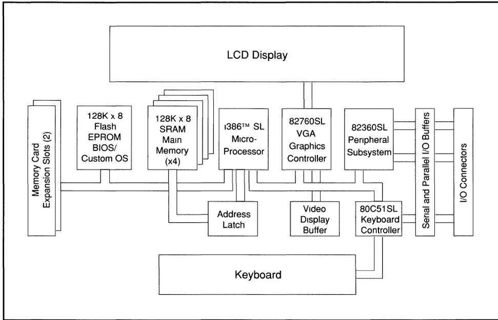
Figure 5-1. Ten-Chip Palm-Top PC Block Diagram
