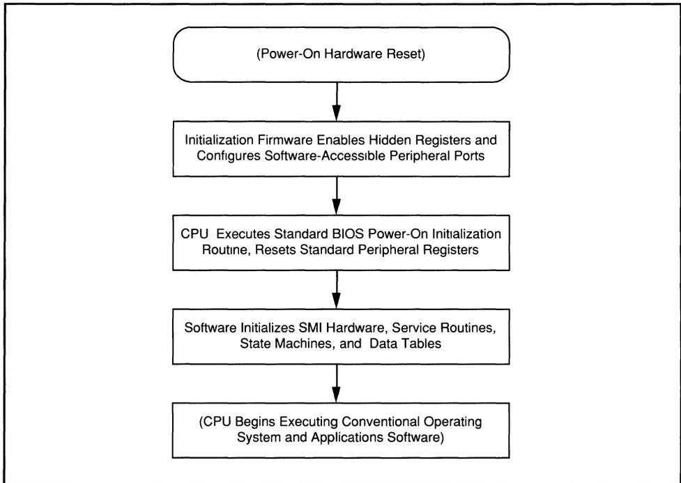
**Figure 4-4. System Management Mode Initialization Sequence**
