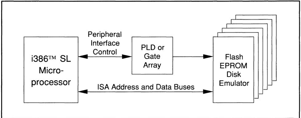
**Figure 2-9. Dedicated Control Signals Simplify Flash EPROM Disk Emulator Systems**
