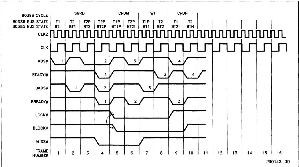
Figure 5-3K. LOCK # /BLOCK # in Non-Cacheable or Miss Cycles—(N = 1)
