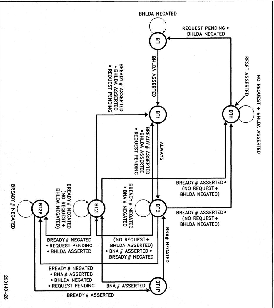
Figure 5-1B. 82385 Local Bus State Machine—Slave Mode
