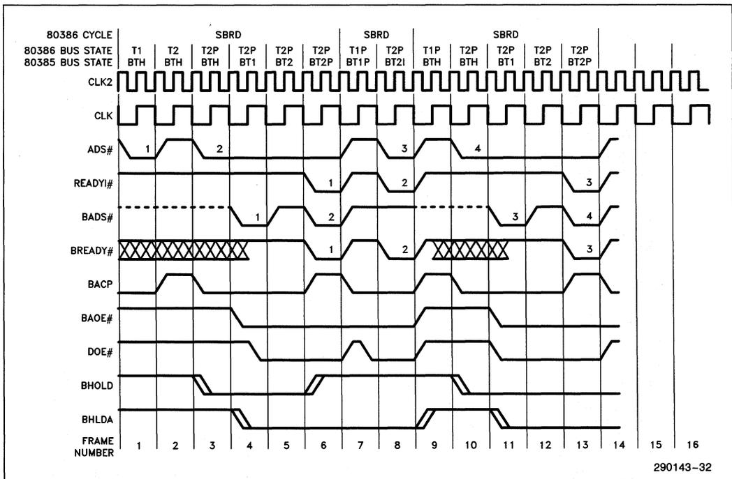
Figure 5-3D. SBRD Cycles Interleaved with BTH States—(N = 1)
