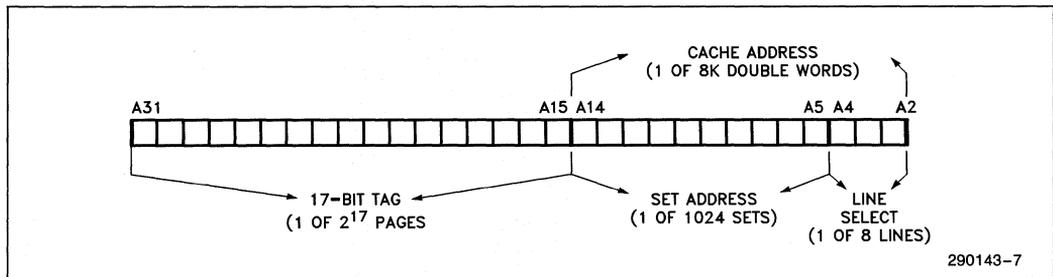
Figure 2-2. 80386 Address Bus Bit Fields—Direct Mapped Organization
