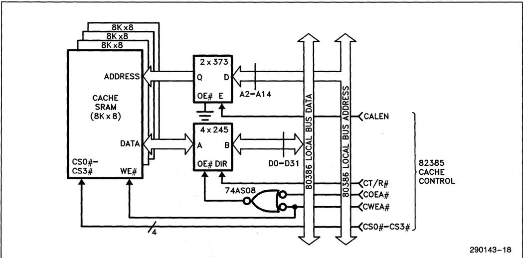
Figure 4-4B. Direct Mapped Cache with Data Buffers
