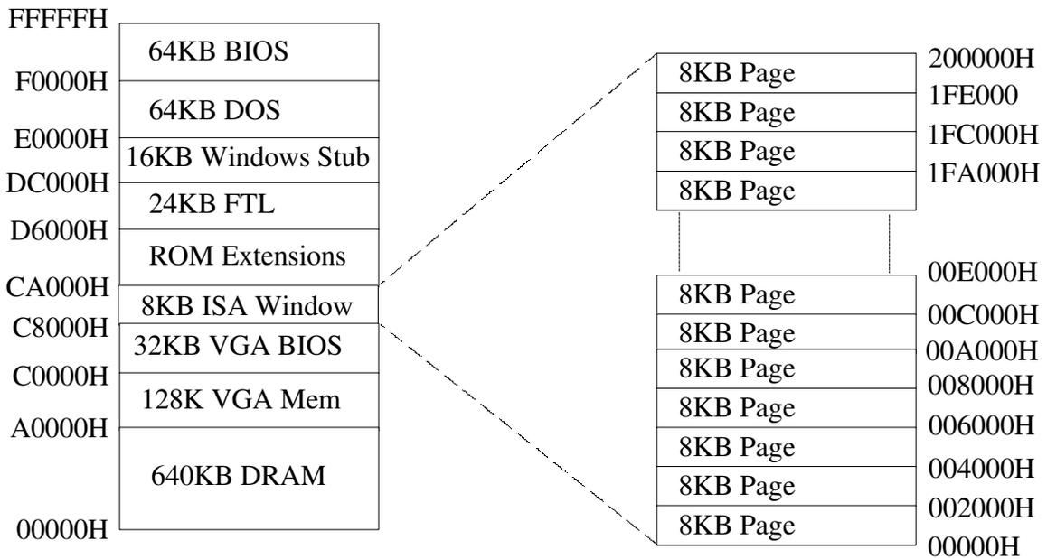
Flash file systems can use a window like this to access a flash array.
