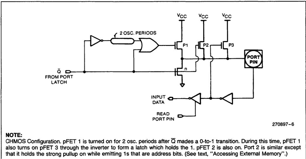
Figure 4. Ports 1, 3, 4, and 5 Internal Pullup Configuration
