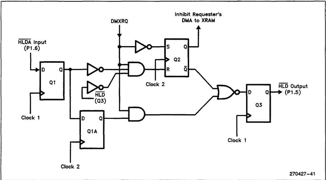
Figure 4.10. Internal Logic of the Requester
