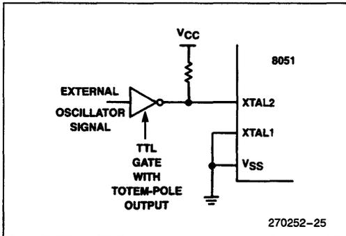
**Figure 32. Driving the HMOS MCS<sup>®</sup>-51 Parts with an External Clock Source**
