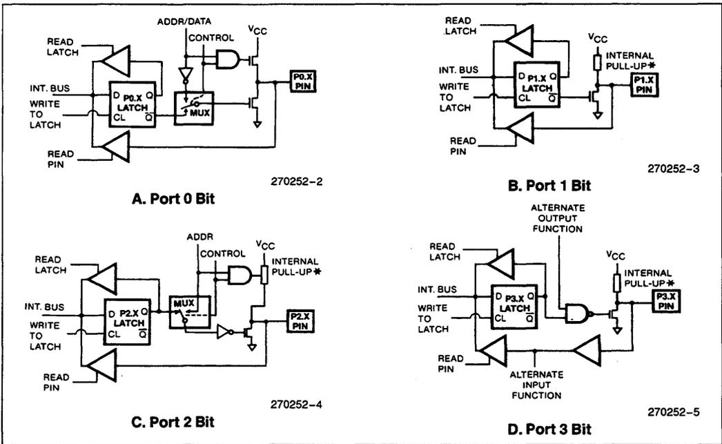
**Figure 4. 8051 Port Bit Latches and I/O Buffers**
