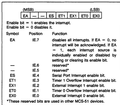
**Figure 17. IE (Interrupt Enable) Register in the 8051**
