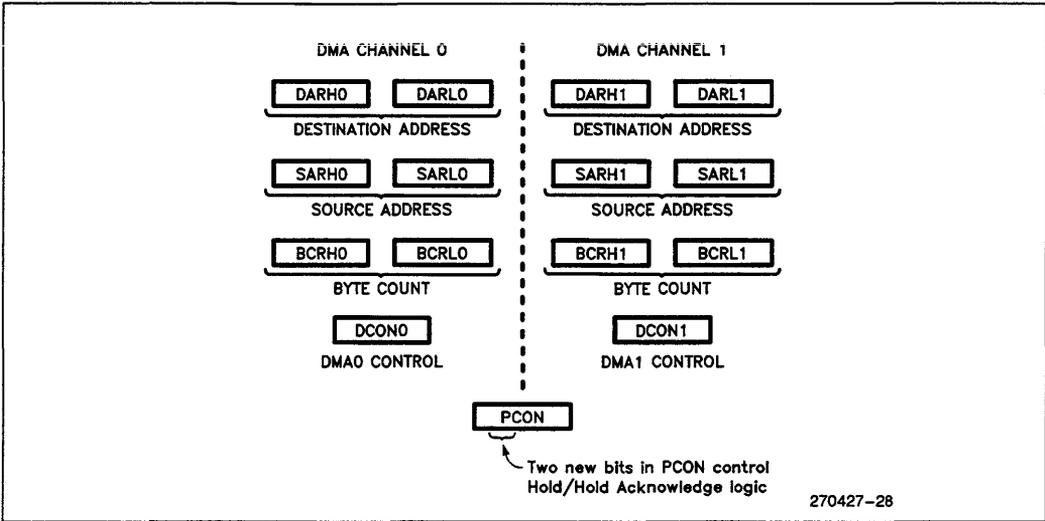
Figure 4.1. DMA Registers
