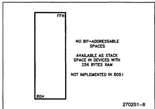
**Figure 8. The Upper 128 Bytes of Internal RAM**
