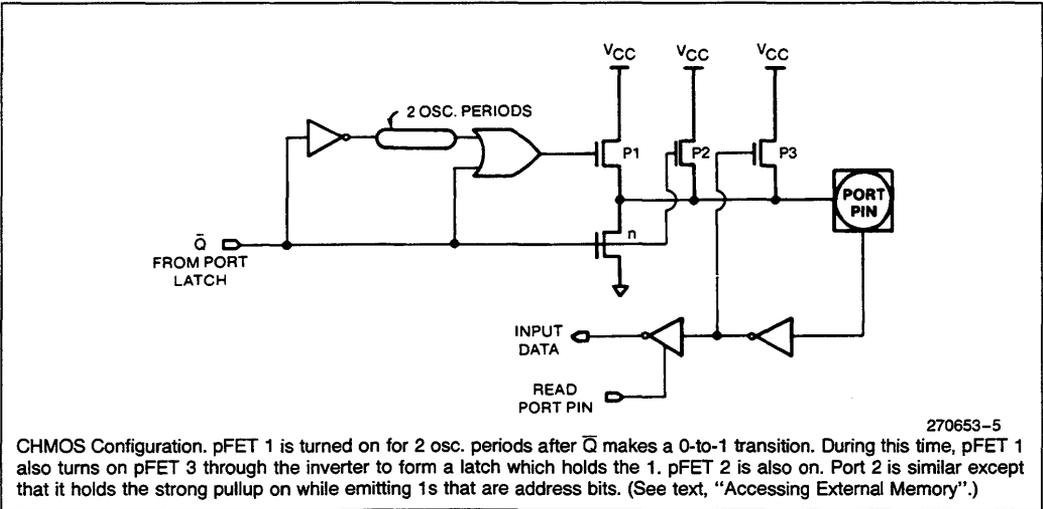
CHMOS Configuration. pFET 1 is turned on for 2 osc. periods after Q-bar makes a 0-to-1 transition. During this time, pFET 1 also turns on pFET 3 through the inverter to form a latch which holds the 1. pFET 2 is also on. Port 2 is similar except that it holds the strong pullup on while emitting 1s that are address bits. (See text, "Accessing External Memory".)
