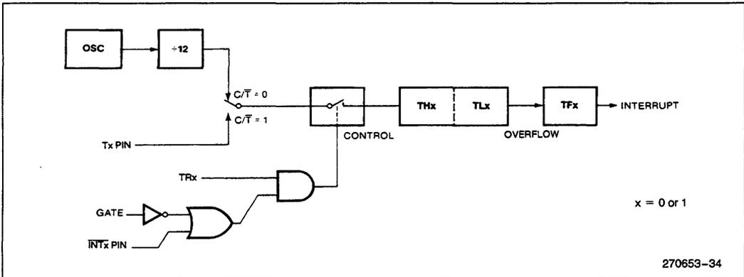
Figure 9. Timer/Counter 0 or 1 in Mode 1: 16-Bit Counter
