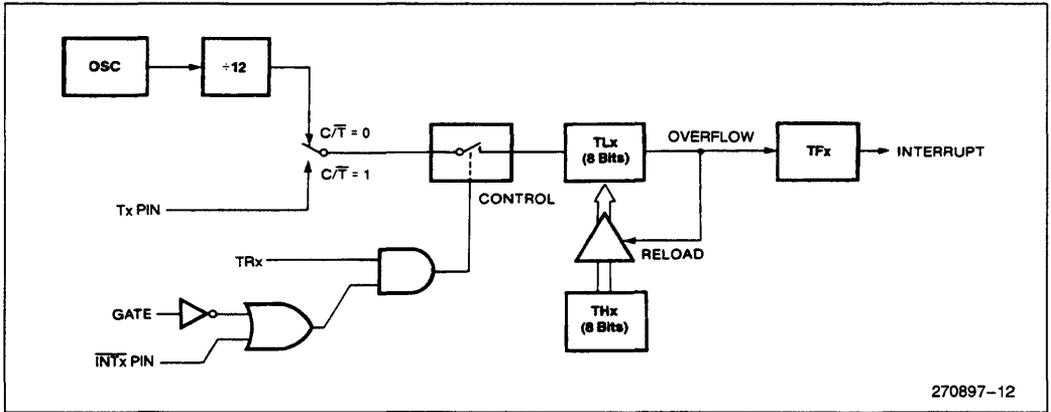
Figure 10. Timer/Counter 1 Mode 2: 8-Bit Auto-Reload
