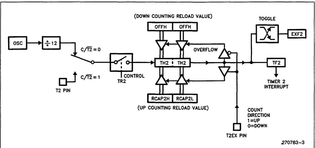
Figure 3. Timer 2 Auto Reload Mode (DCEN = 1)
