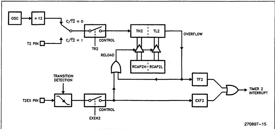
Figure 13. Timer 2 Auto Reload Mode (DCEN = 0)
