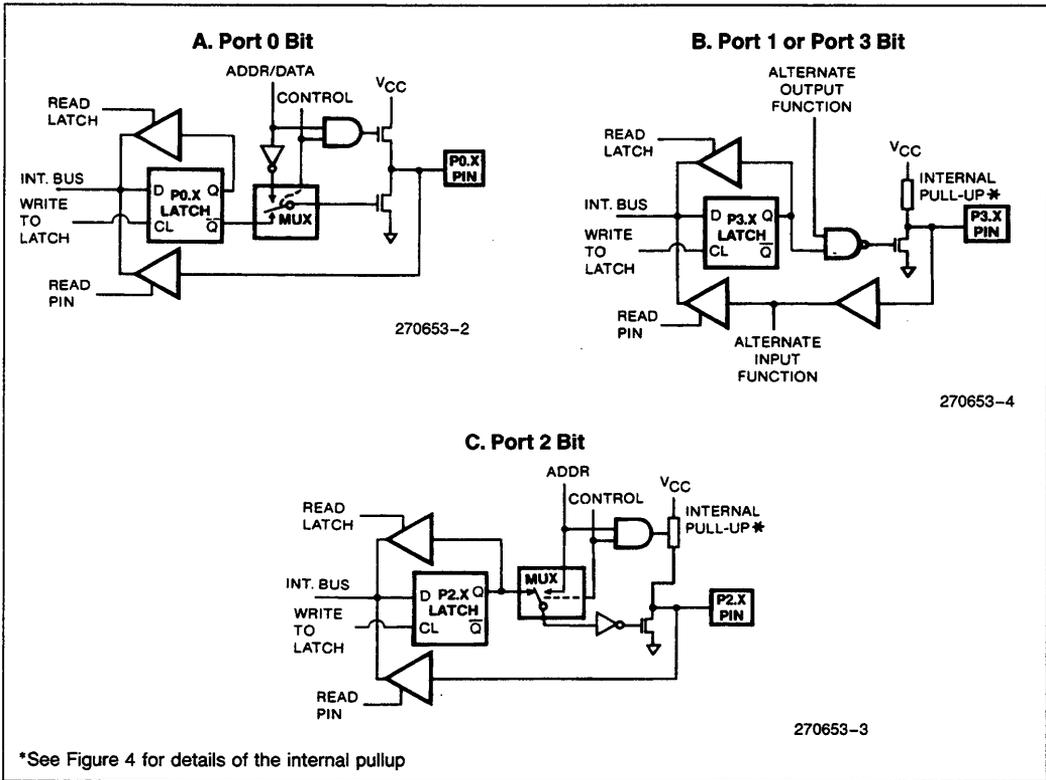
Figure 2. C51FX Port Bit Latches and I/O Buffers
