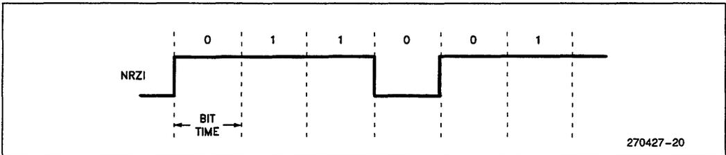
Figure 3.9. NRZI Encoding
