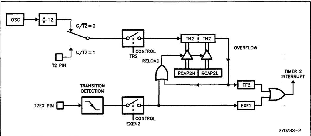
Figure 2. Timer 2 Auto Reload Mode (DCEN = 0)
