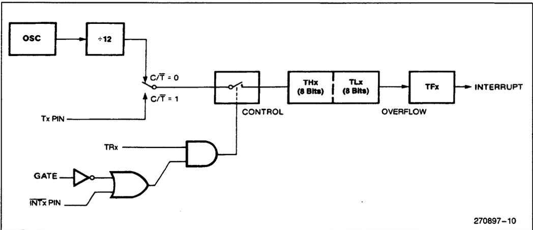
Figure 8. Timer/Counter 0 or 1 in Mode 0: 13-Bit Counter
