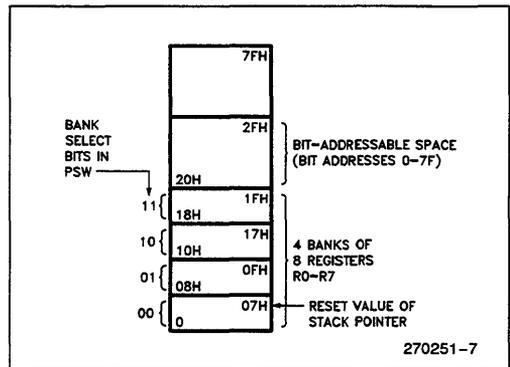
**Figure 7. The Lower 128 Bytes of Internal RAM**
