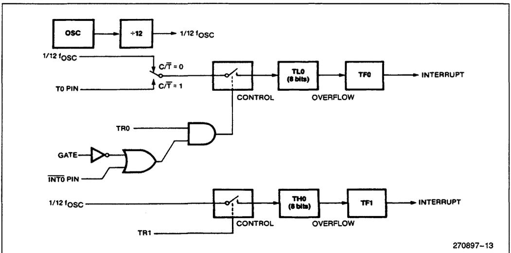
Figure 11. Timer/Counter 0 Mode 3: Two 8-Bit Counters
