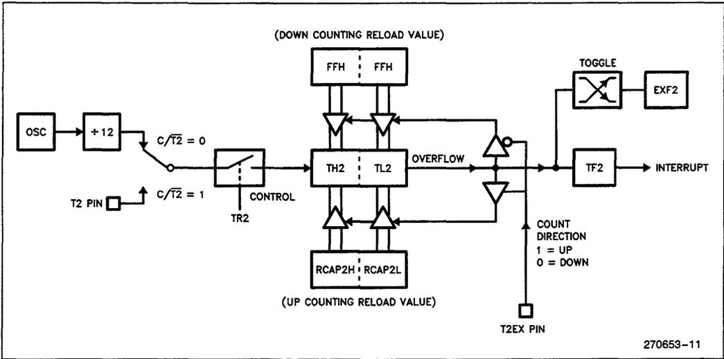
Figure 14. Timer 2 Auto Reload Mode (DCEN = 1)
