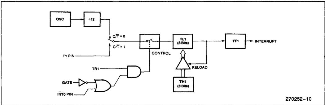
Figure 9. Timer/Counter 1 Mode 2: 8-Bit Auto-Reload
