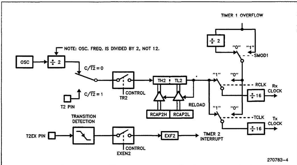
Figure 5. Timer 2 in Baud Rate Generator Mode
