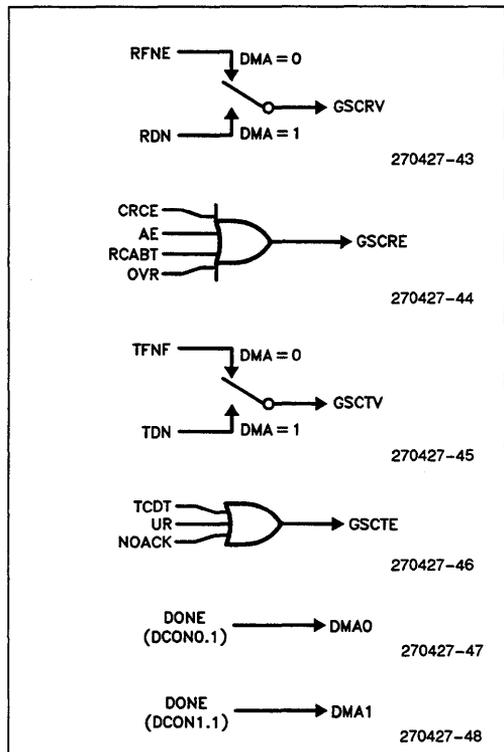
Figure 5.1. Six New Interrupts in the 8XC152
