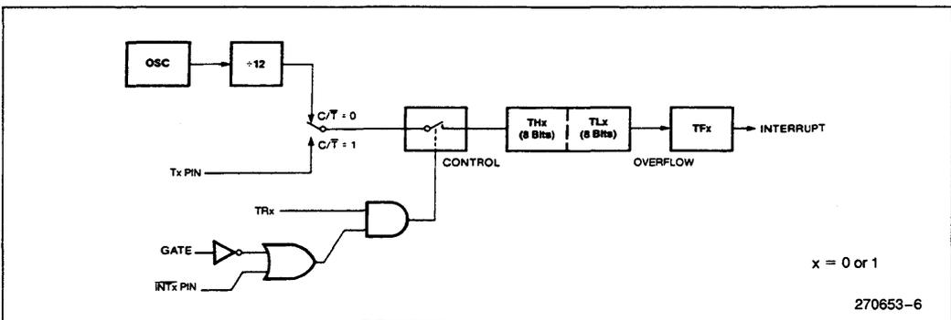
**Figure 8. Timer/Counter 0 or 1 in Mode 0: 13-Bit Counter**
