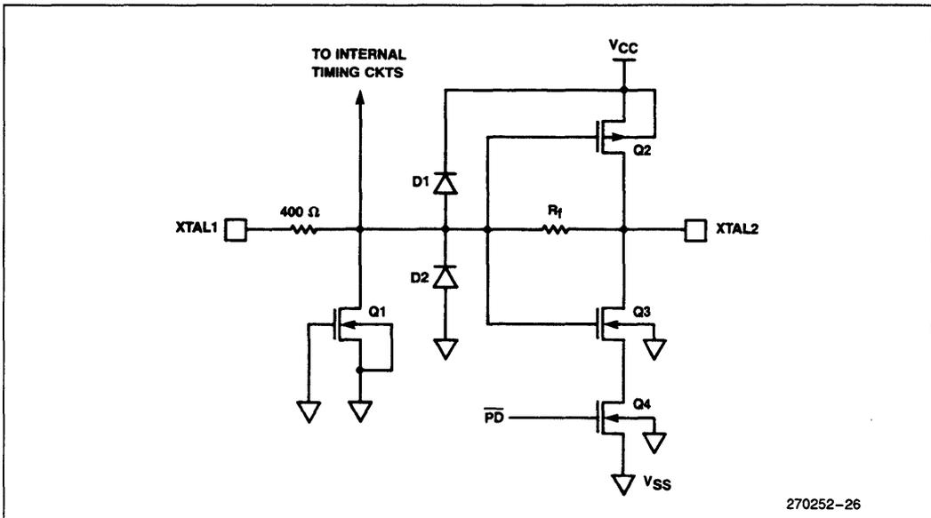
**Figure 33. On-Chip Oscillator Circuitry in the CHMOS Versions of the MCS<sup>®</sup>-51 Family**
