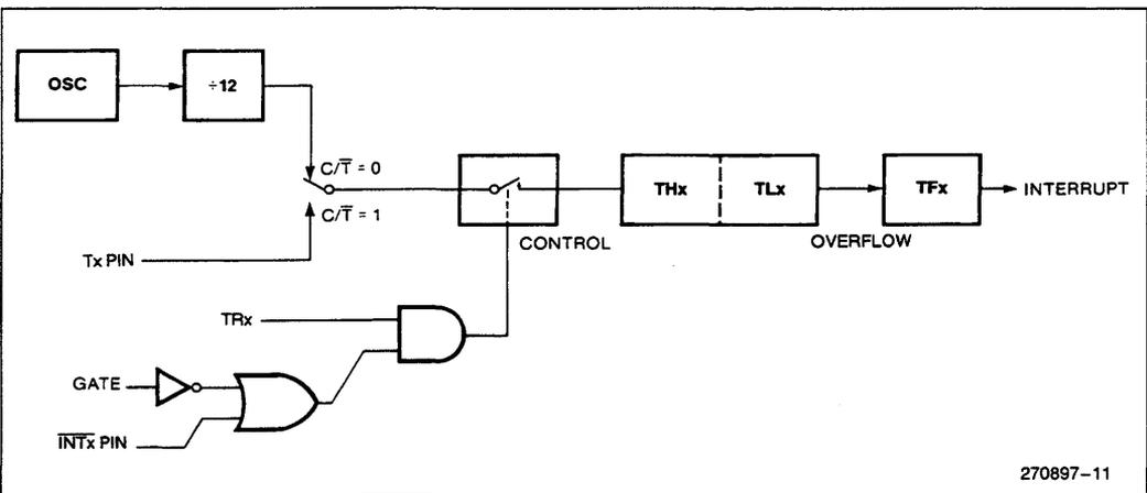
**Figure 9. Timer/Counter 0 or 1 in Mode 1: 16-Bit Counter**
