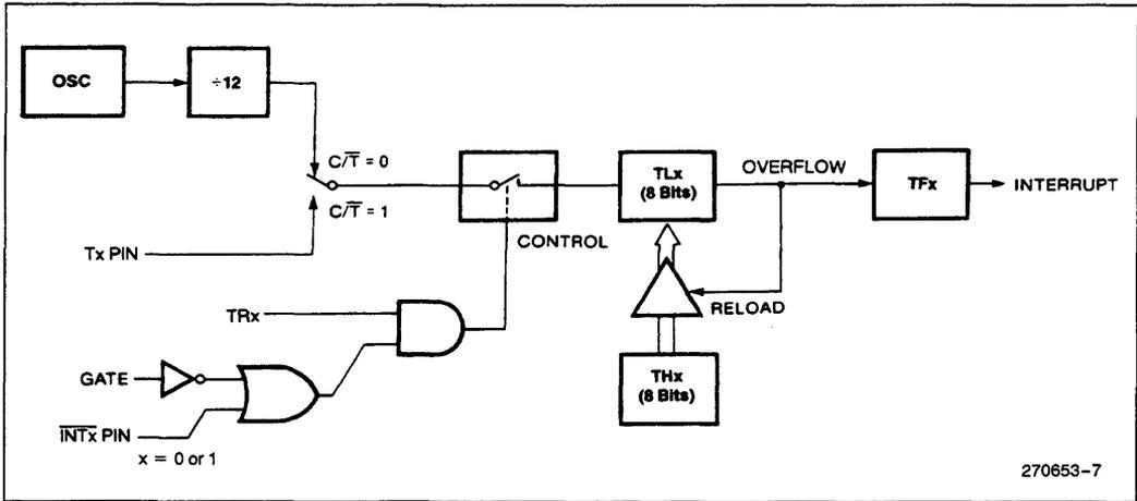
Figure 10. Timer/Counter 1 Mode 2: 8-Bit Auto-Reload
