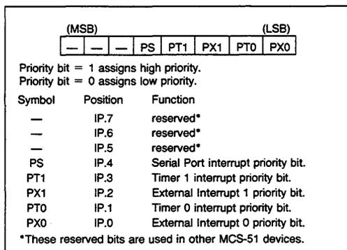
**Figure 18. IP (Interrupt Priority) Register in the 8051**
