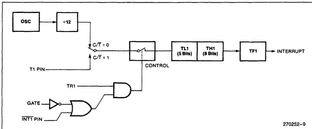
Figure 7. Timer/Counter 1 Mode 0: 13-Bit Counter
