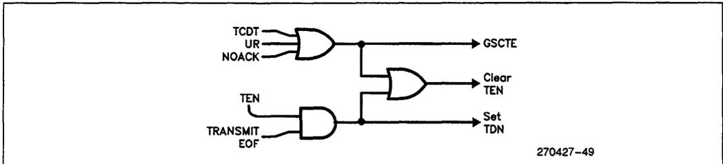
Figure 5.2. Transmit Error Flags (Logic for Clearing TEN, Setting TDN)
