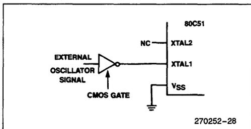
Figure 35. Driving the CHMOS MCS<sup>®</sup>-51 Parts with an External Clock Source
