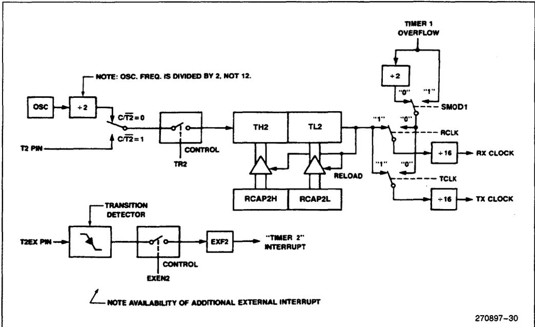
Figure 29. Timer 2 in Baud Rate Generator Mode
