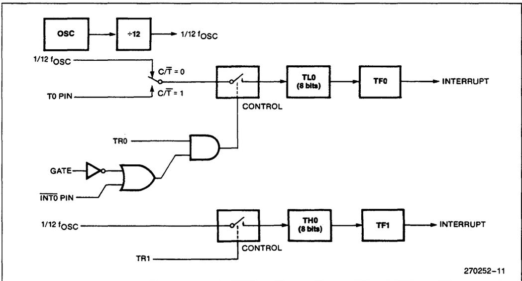
Figure 10. Timer/Counter 0 Mode 3: Two 8-Bit Counters
