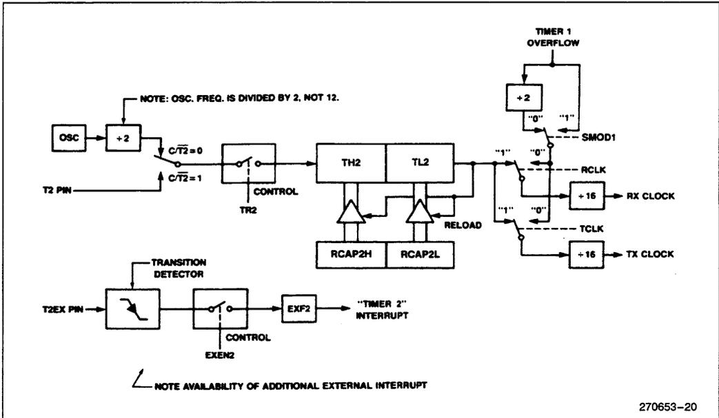
**Figure 23. Timer 2 in Baud Rate Generator Mode**
