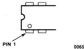
Whether or not pin 1 is marked, it is always in the same position with respect to the notch. Viewed from the top side of the component, with the notched end upward, pin 1 is the highest pin in the row to the left of the notch.
