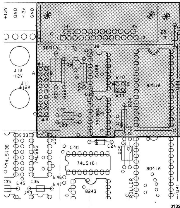
Figure 3-26. Serial I/O Port Area, Detail
