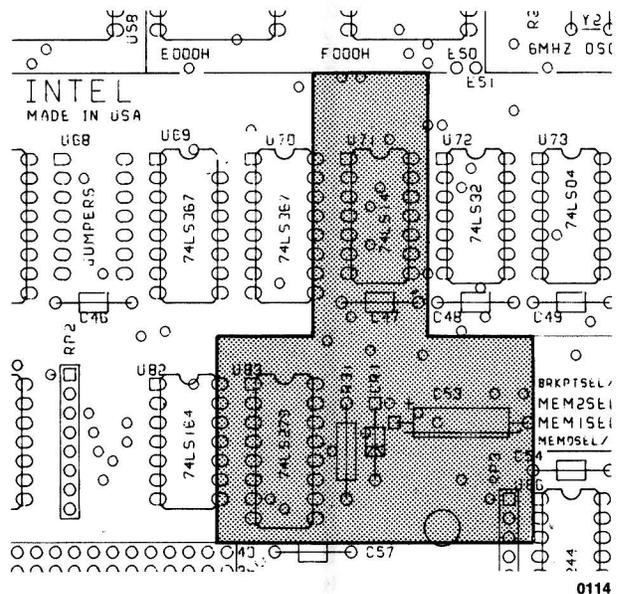
Figure 3-8. Reset Area, Detail
