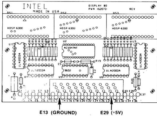
Figure 3-2. Display Board With Check Points
