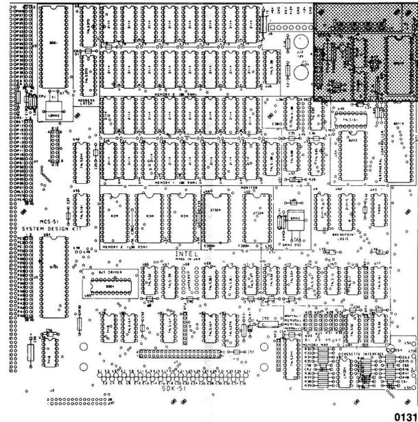
Figure 3-25. Serial I/O Port Area
