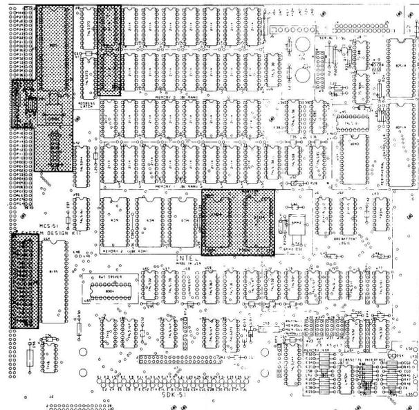
Figure 3-22. Microcontroller, Monitor and RAM Areas
