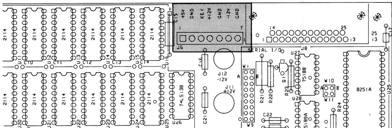
Figure 3-1. Power Connector J6, CPU Board
