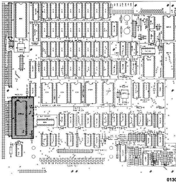
Figure 3-24. Parallel I/O Controller
