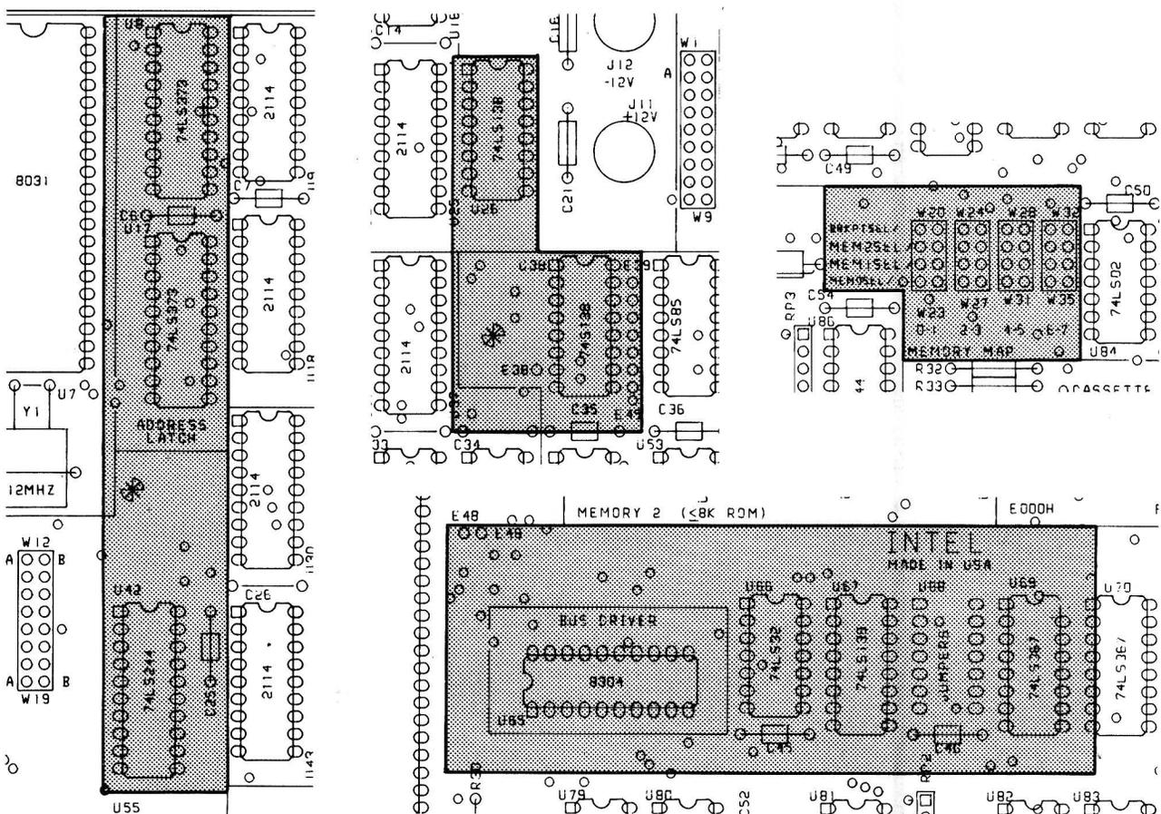
**Figure 3-17. Address Bus and Data Bus Areas, Details**
