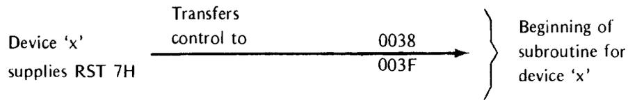
Note that any of these 8-byte subroutines may in turn call longer subroutines to process the interrupt, if necessary.
