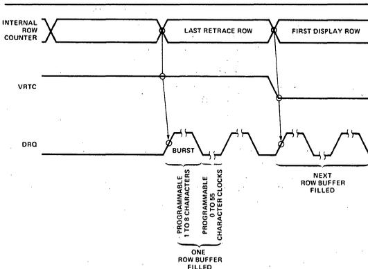
Figure 18. DMA Timing
