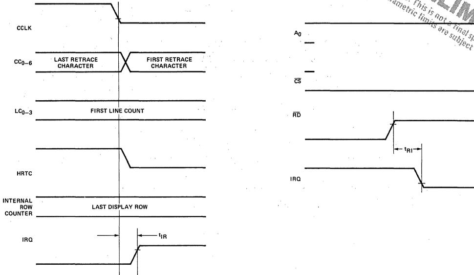
**Figure 29. Interrupt Timing**
