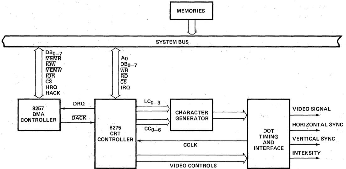
Figure 3. 8275 Systems Block Diagram Showing Systems Operation
