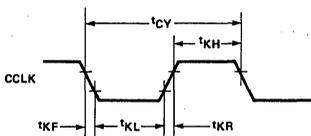
**Input Waveforms (For A.C. Tests)**
