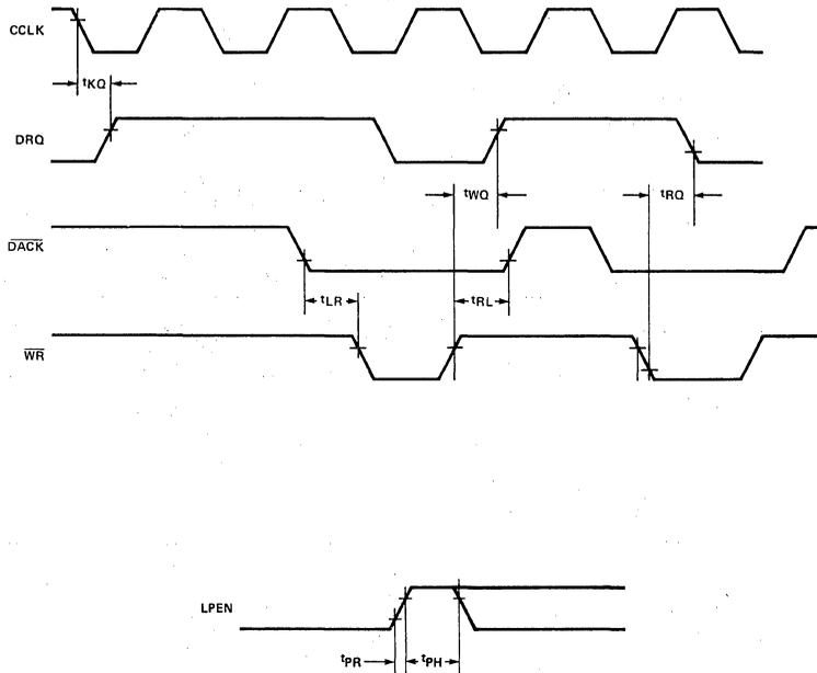
**Figure 30. DMA Timing**
