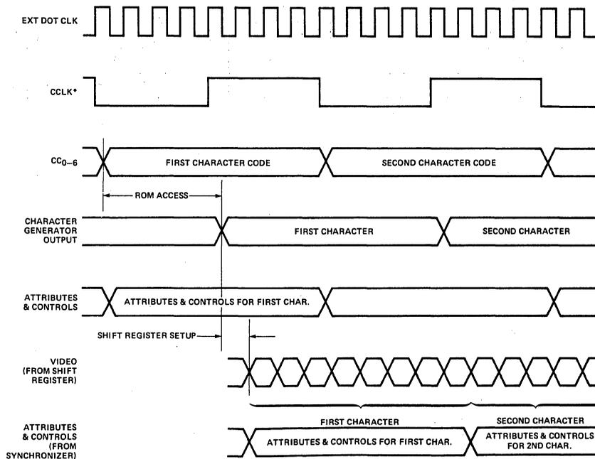
\*CCLK IS A MULTIPLE OF THE DOT CLOCK AND AN INPUT TO THE 8275.
