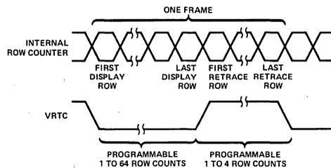
Figure 17. Frame Timing
