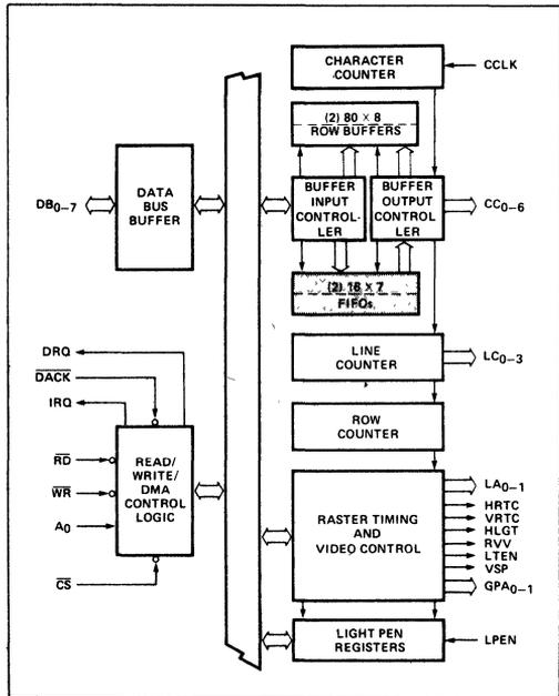
Figure 24. Block Diagram Showing FIFO Activation
