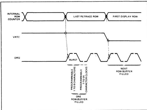
**Figure 19. DMA Timing**
