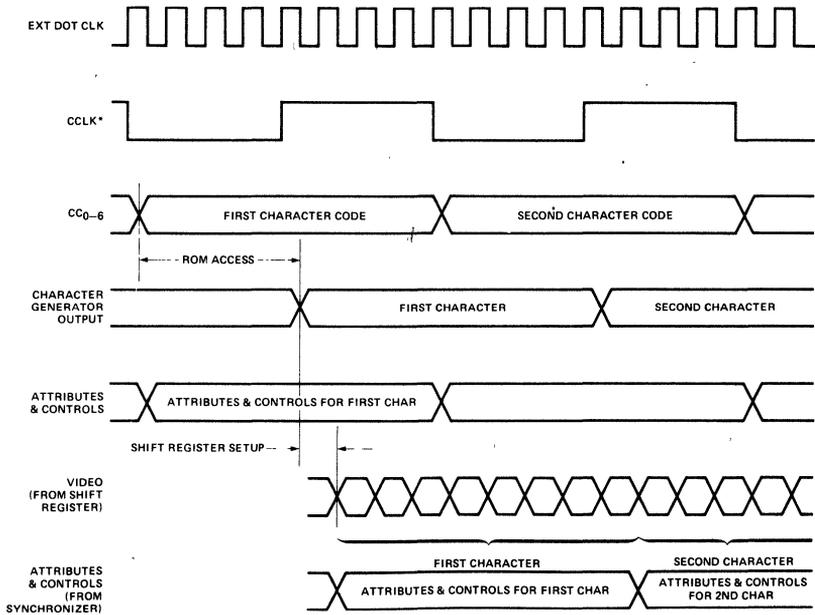
\*CCLK IS A MULTIPLE OF THE DOT CLOCK AND AN INPUT TO THE 8275
