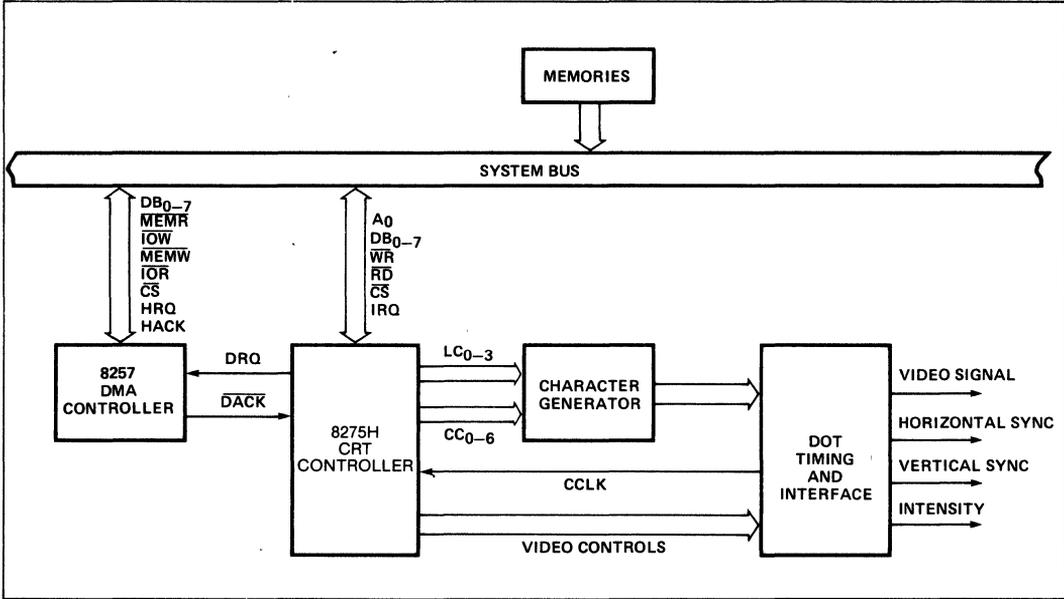
**Figure 4. 8275H Systems Block Diagram Showing Systems Operation**
