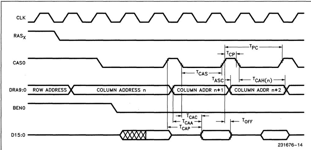
**DRAM SIGNALS—NON INTERLEAVED FAST PAGE MODE WRITE**
