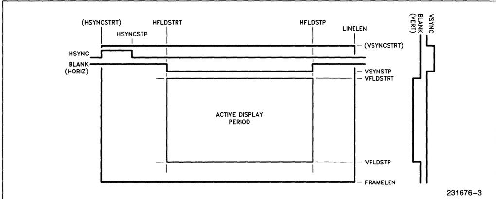
Figure 3. Timing Parameters
