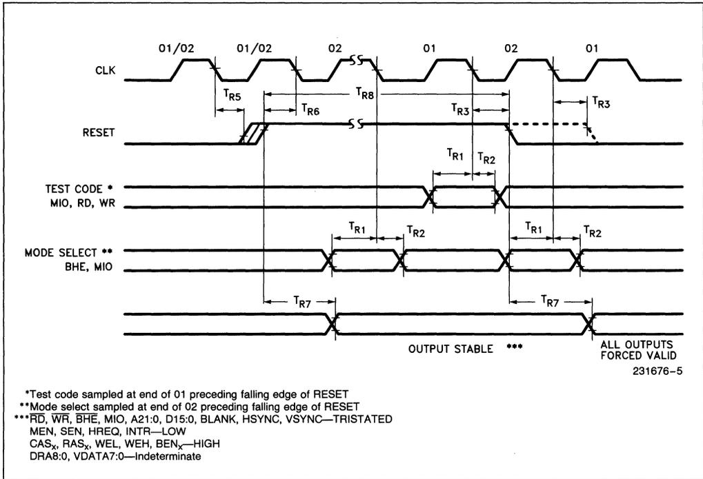
CLOCK AND AC TEST CONDITIONS
