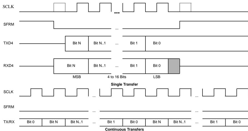
**Note:** The phase and polarity of SCLK can be configured for four different modes. This example shows just one of those modes. See the [Section 11.12.10, "SSP Control Register 1"](#) on page 11-159 for a complete description of each mode.
