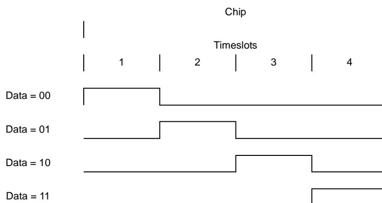
**Figure 11-26. 4PPM Modulation Example**
