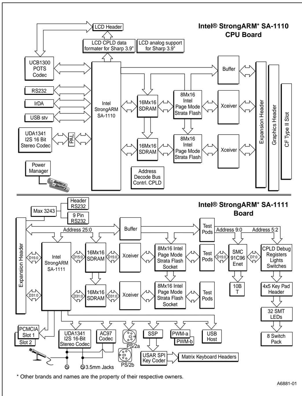
The block diagram shown in Figure 3-1 illustrates the modularity, flexibility and extend ability of the design. The SA-1110 Development Board supports two 140 pin fully buffered daughter board expansion headers. One of these expansion headers is for the SA-1111 Development Module, the other is for a graphics accelerator board.
