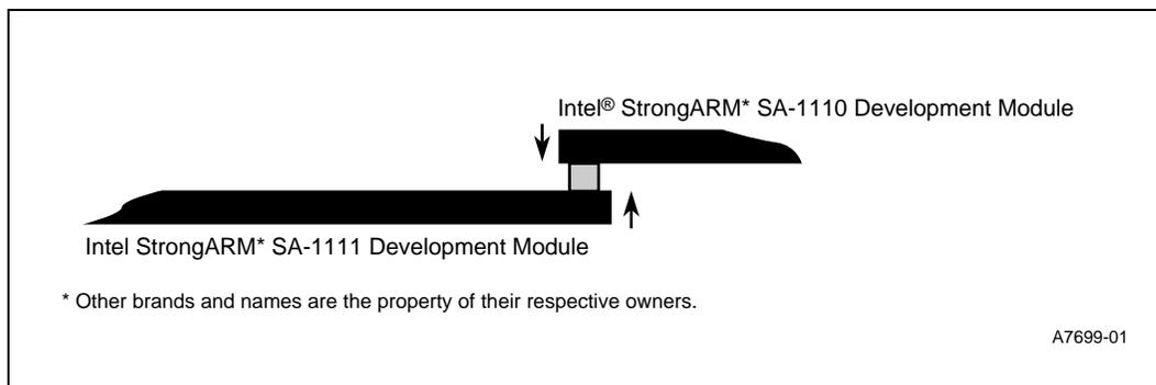
5. To remove the SA-1111 Development Module, evenly pull the modules apart as shown in [Figure 2-7](#).
