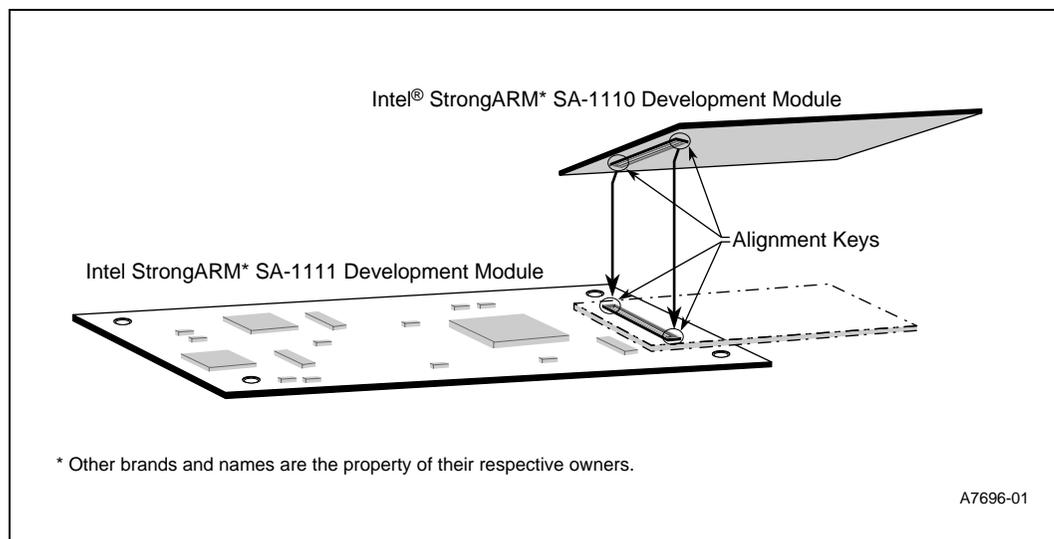
4. Nearest the board edges, gently press together and install the mounting hardware as shown in [Figure 2-5](#) and [Figure 2-6](#). Slide the connector in until it is firmly seated.
