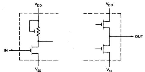
Figure 3-5. Typical MCS-4 Input and Output Circuitry.
