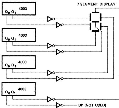
Figure 2-2. Shift Registers Driving Seven Segment LED Displays
