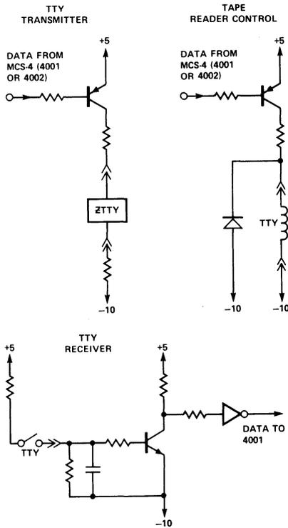
Figure 3-3. MCS-40 and Teletype Interface Circuits.
