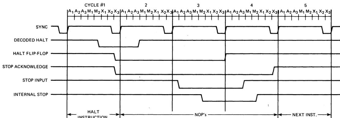
Figure 1-10. Halt Timing (Exit Using Stop Input).
