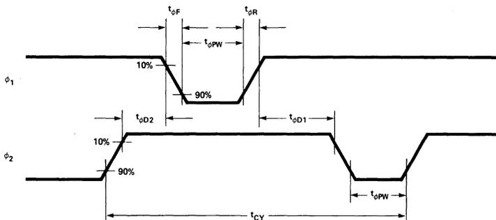
\*  $V_{DD} = V_{SS} - 15\text{V} \pm 5\%$ . For TTL compatability use  $V_{DD} = -10\text{V}$ ,  $V_{SS} = 5\text{V}$ .
