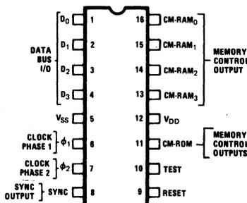
Figure 1-1. 4004 Pin Configuration.
