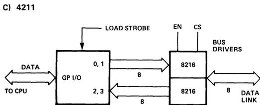
Figure 4-19. Typical GP I/O Applications.
