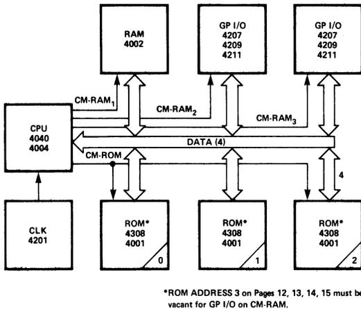
Figure 3-9. System Diagram Illustrating GP I/O on CM-RAM.
