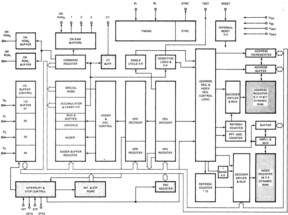
Figure 1-8. Detailed 4040 Block Diagram.
