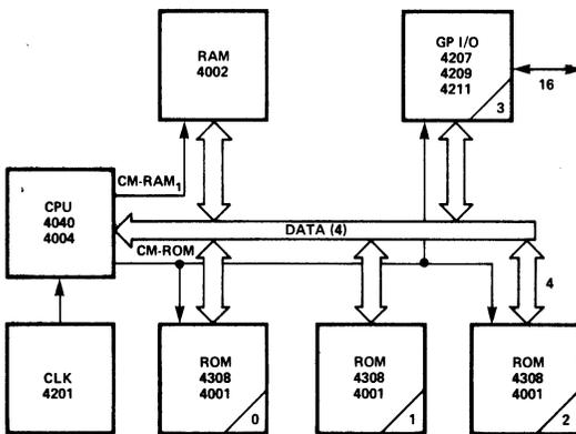
Figure 3-10. Typical System Using GP I/O.
