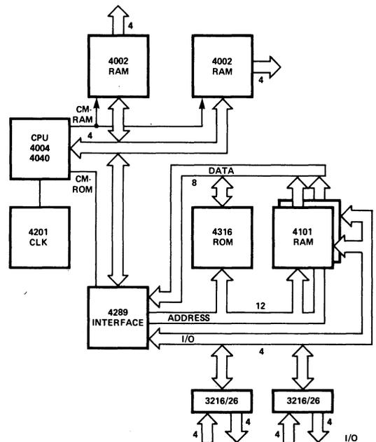
Figure 3-8. System Diagram Using Standard Memory Components.
