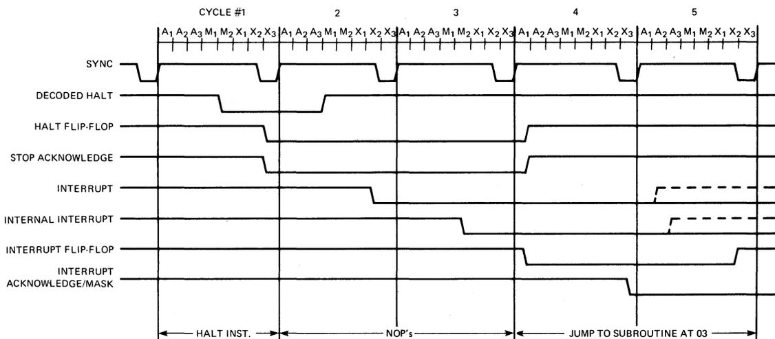
Figure 1-13. Halt Timing (Exit Using Interrupt).
