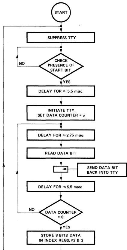
Figure 3-2. Flow Chart for Teletype Interfaces.
