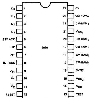
Figure 1-5. 4040 Pin Configuration.
