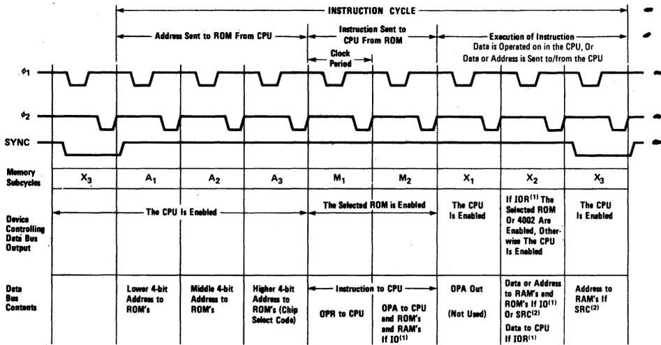
(1) IO instructions control the flow of information between accumulator in CPU, I/O lines in ROM's and RAM's and RAM storage. IOR stands for IO Read. In this case the CPU will receive data from RAM storage locations or I/O input lines.
