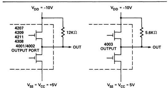
Figure 3-4. MCS-4 Output Configuration for TTL Compatibility.
