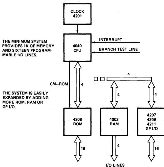
Figure 3-7. The Minimum System Provides 1K of Memory and Sixteen Programmable I/O Lines.
