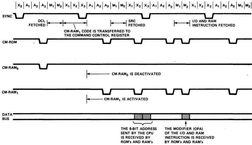
**Figure 1-21. Operation of the Command Control Lines.**
