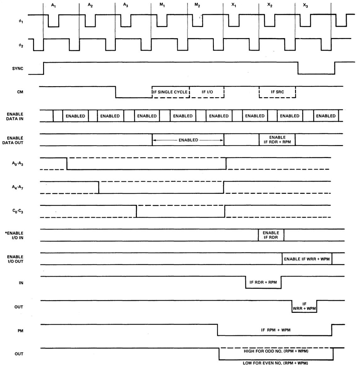
Figure 4-24. 4289 Timing Diagram.
