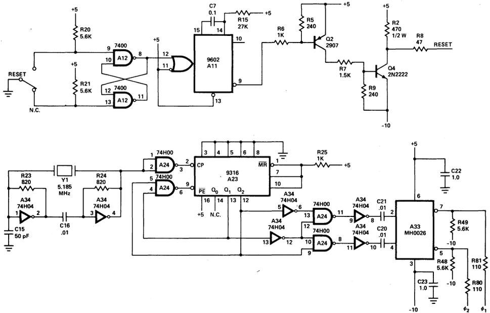
Figure 3-14. Suggested Clock and Reset Circuit.
