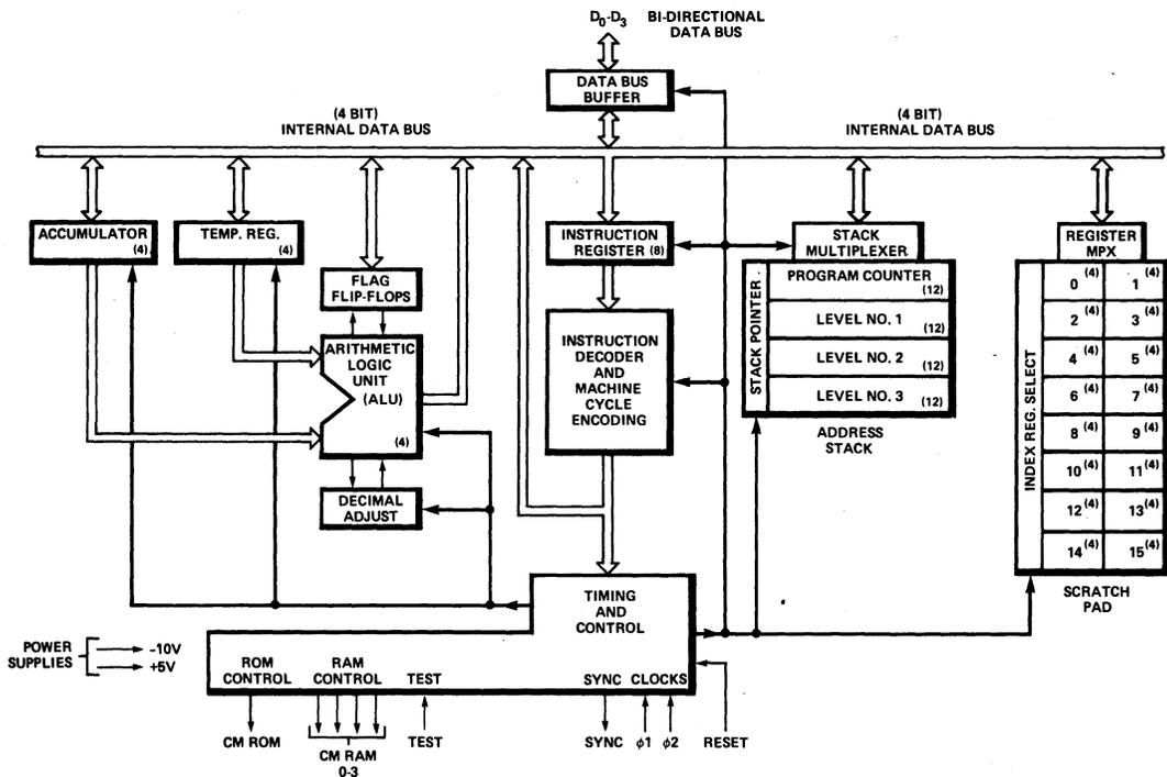
Figure 1-3. 4004 CPU Block Diagram.
