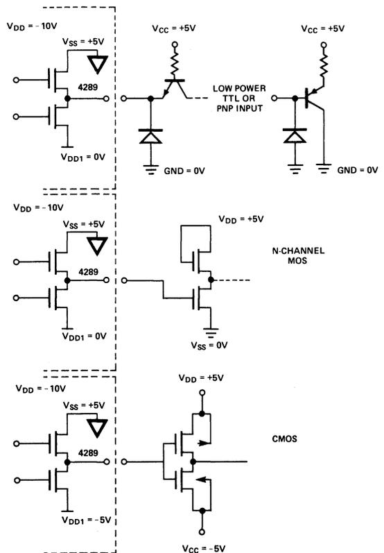
Figure 3-6. 4289 Interface Method by Using  $V_{DD1}$ .
