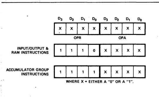
Figure 1-18. I/O and Accumulator Group Instruction Formats.
