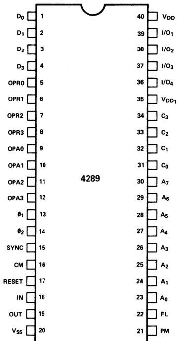
Figure 4-23. 4289 Pin Configuration.
