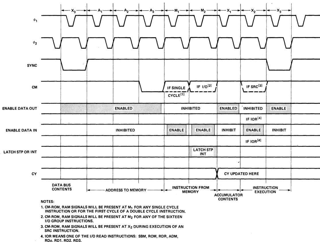
Figure 1-6. 4040 Basic Timing Diagram.
