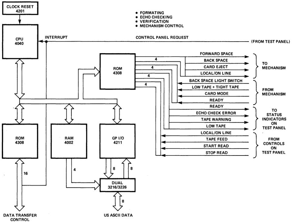
Figure 3-19. Paper Tape Reader and Punch Controller.
