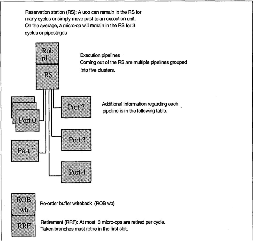
Figure 2-4. Out-Of-Order Core and Retirement Pipeline
