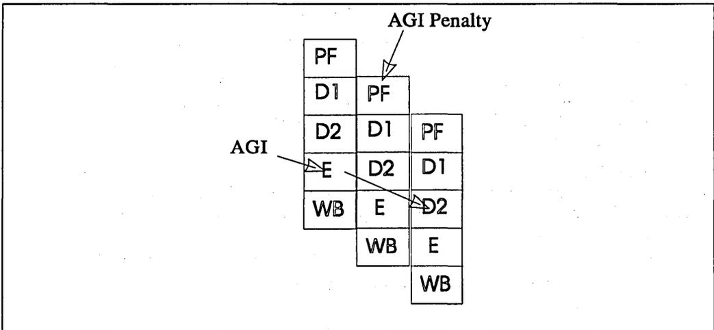
Figure 3-1. Pipeline Example of AGI Stall
