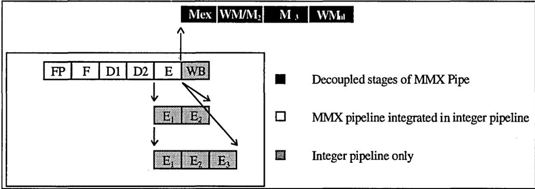
Figure 2-1. MMX™ Pipeline Structure
