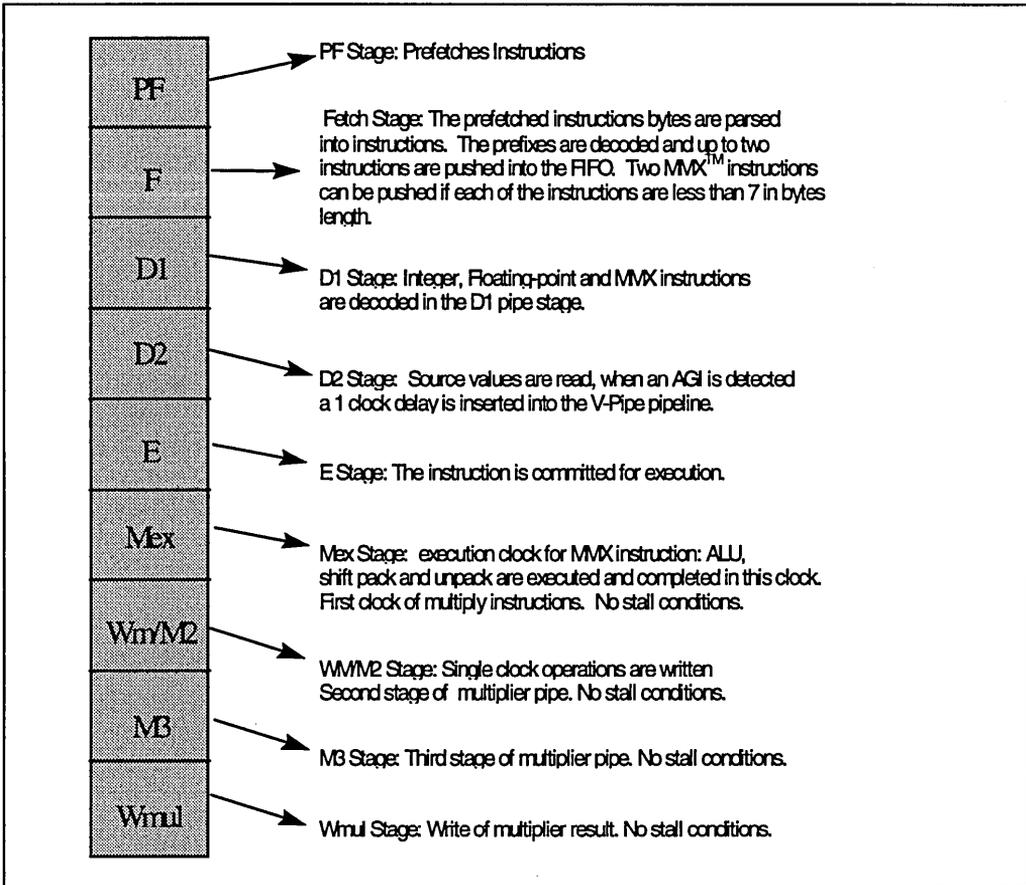
Figure 2-2. MMX™ Instruction Flow in a Pentium® Family Processor with MMX Technology
