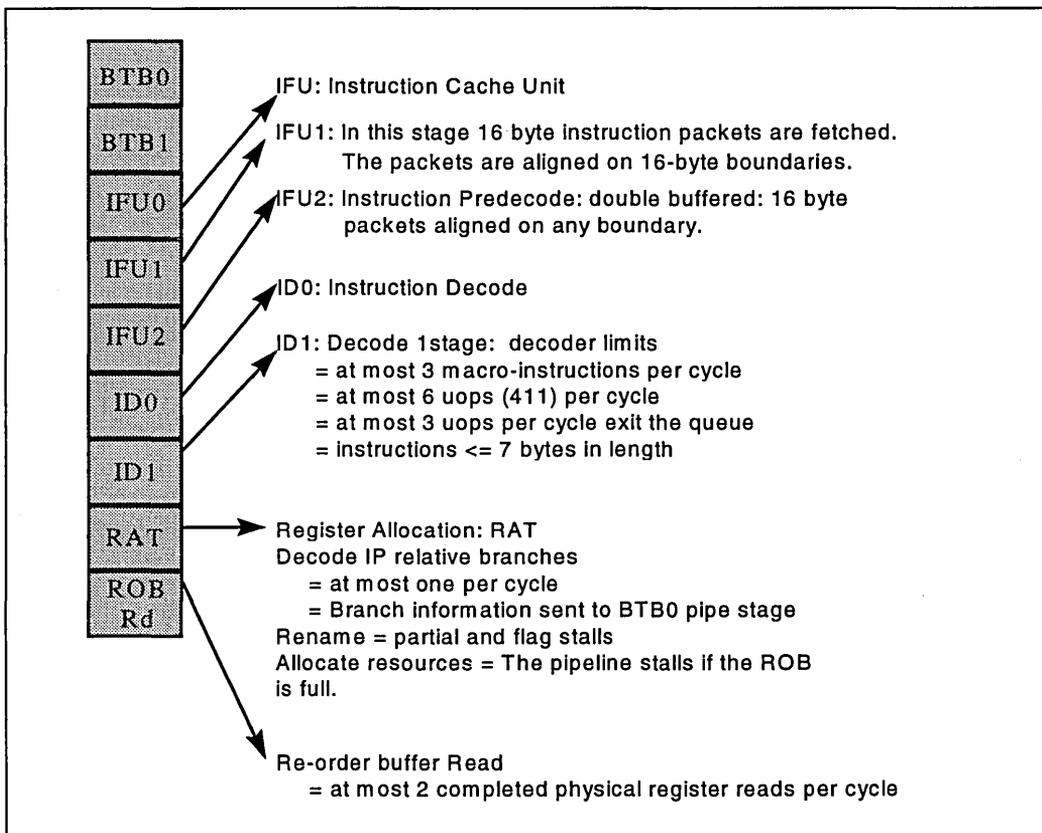
Figure 2-3. Out-Of-Order Core and Retirement Pipeline
