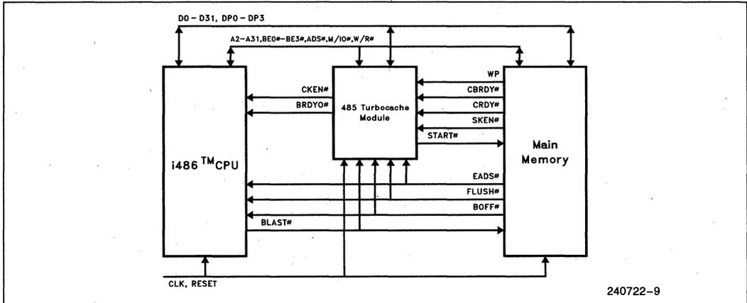
Figure 2.1. 485Turbocache Module Typical Configuration
