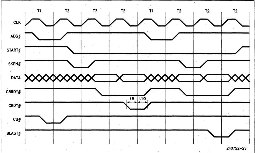
Figure 9.5. Multiple Cycle Line Fill
