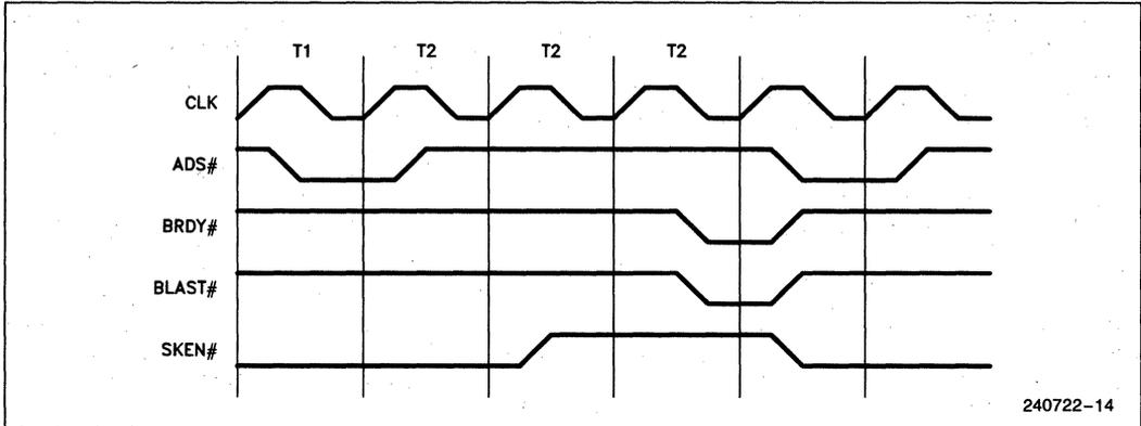
Figure 4.2 Method of SKEN# Generation Not Recommended
