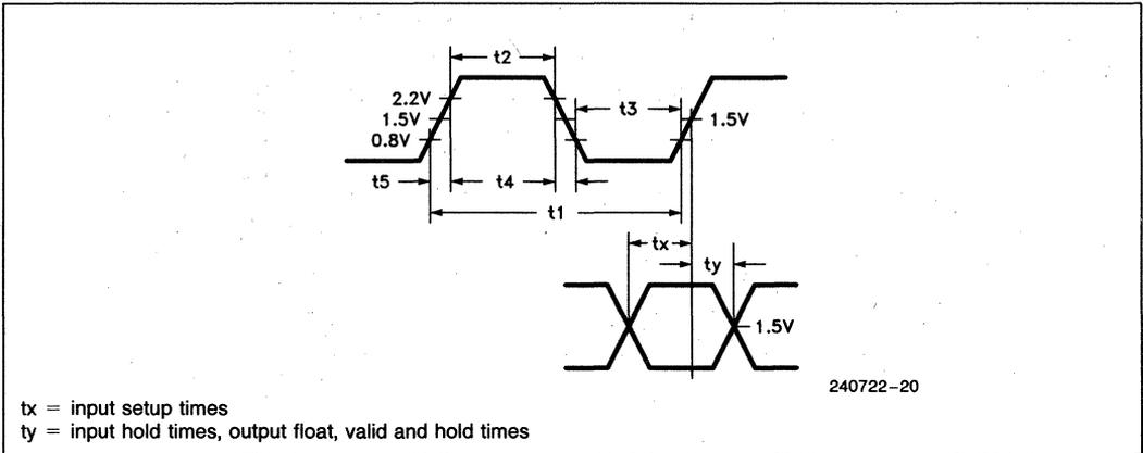
Figure 9.1. CLK Waveforms
