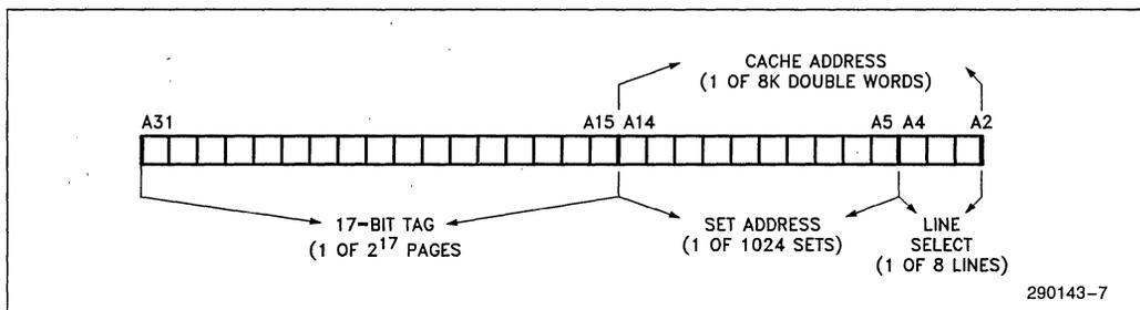
Figure 2-2. 386 DX Address Bus Bit Fields—Direct Mapped Organization
