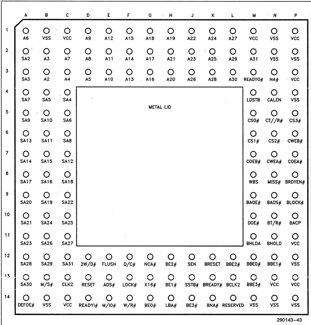
Figure 8-2. 82385 PGA Pinout—View from PIN Side
