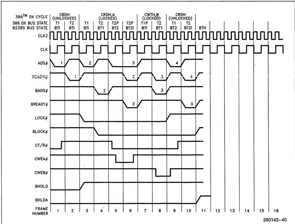
Figure 5-3L. LOCK # /BLOCK # in Cache Read Hit Cycle—(N = 1)
