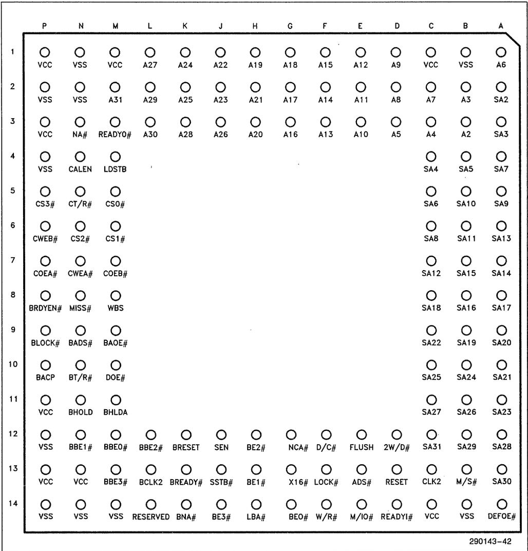
Figure 8-1. 82385 PGA Pinout—View from TOP Side
