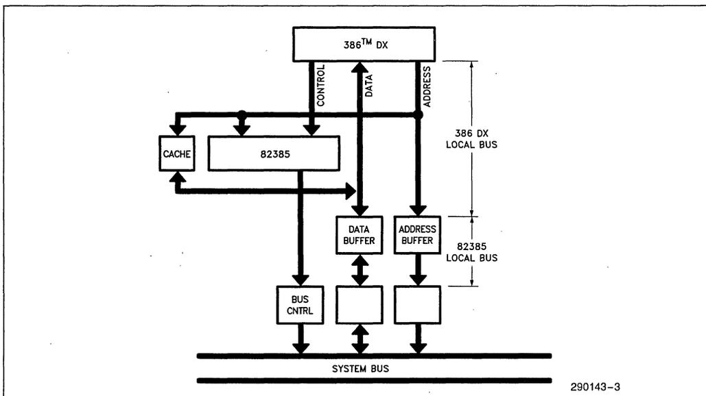
Figure 1-2. 386™ DX CPU/82385 System Bus Structure
