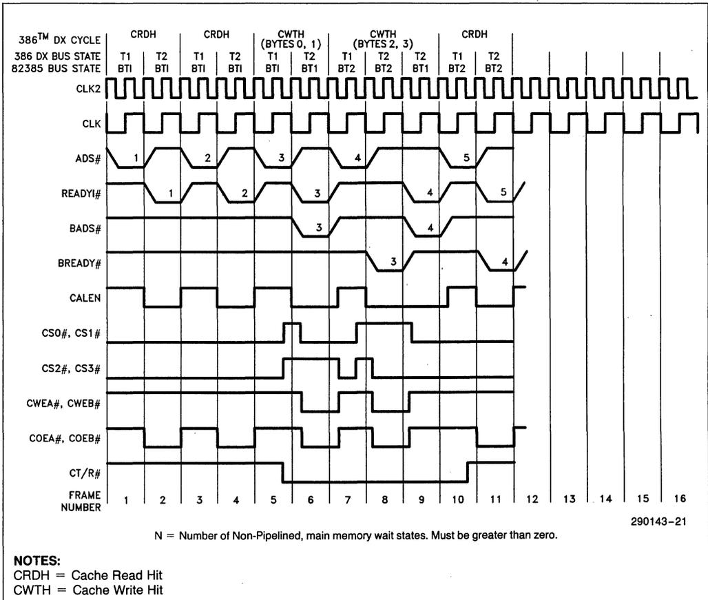
Figure 4-5A. Cache Read and Write Cycles—Direct Mapped (N = 1)
