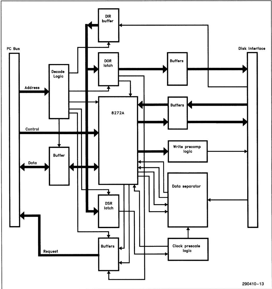
Figure 10-1. Standard IBM PC/AT Floppy Disk Controller
