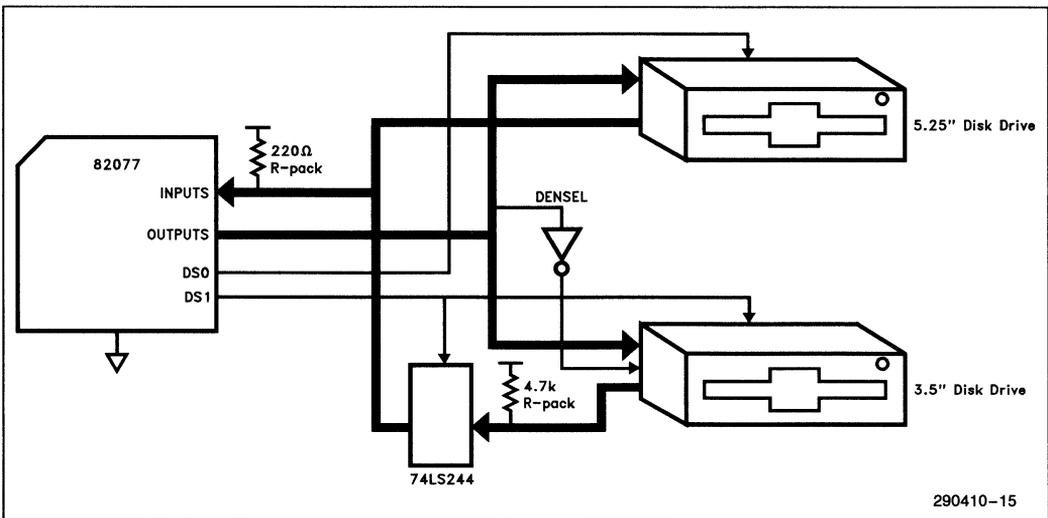
**Figure 10-4. Combined 3.5" and 5.25" Drive Interface**
