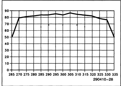
**Figure 13-2. Typical Jitter Tolerance vs Data Rate (Capture Range) (300 Kbps)**
