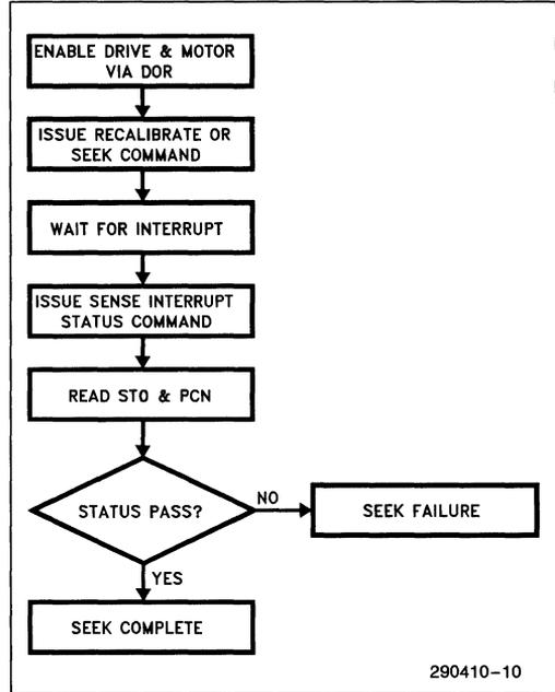
Figure 9-4. Recalibrate and Seek Operations
