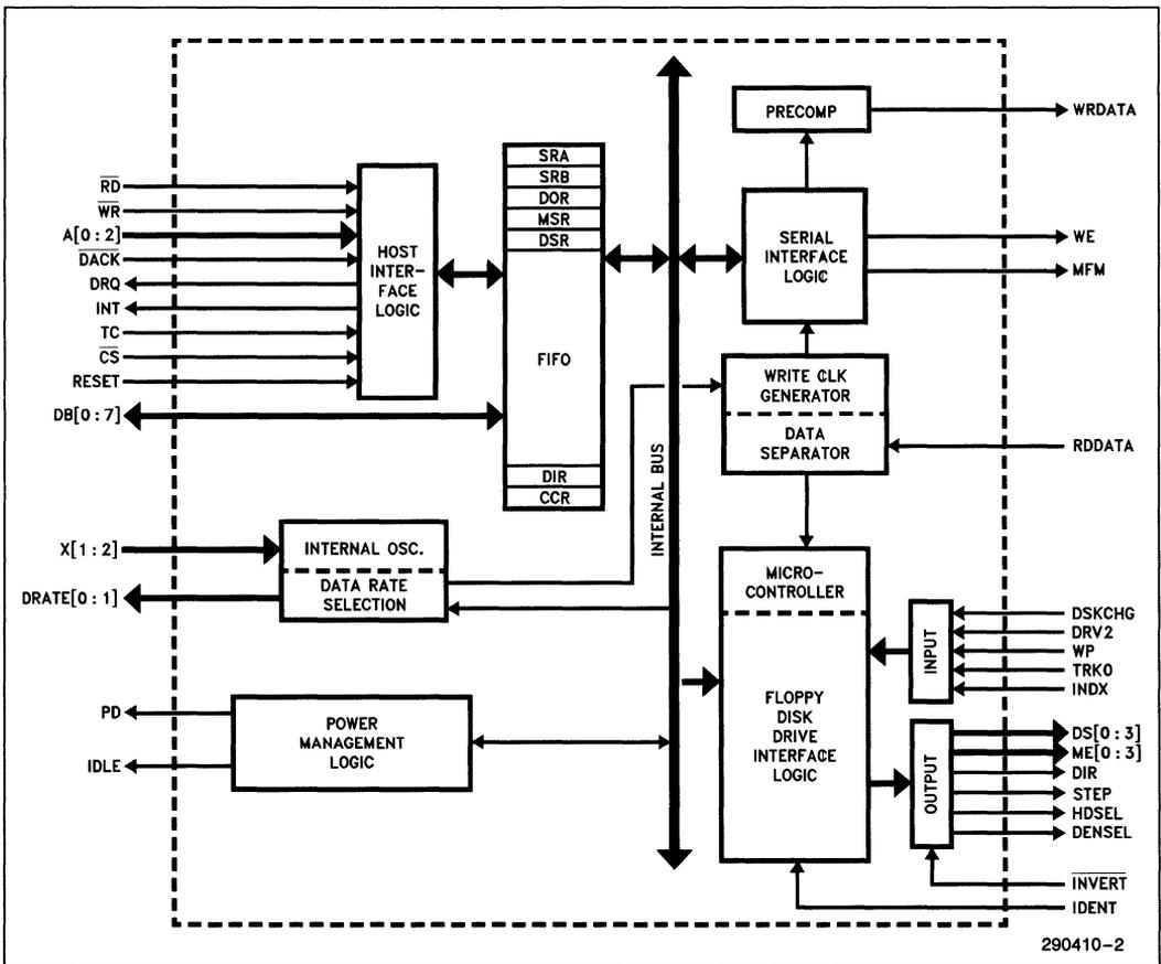
Figure 1-1. 82077SL Block Diagram
