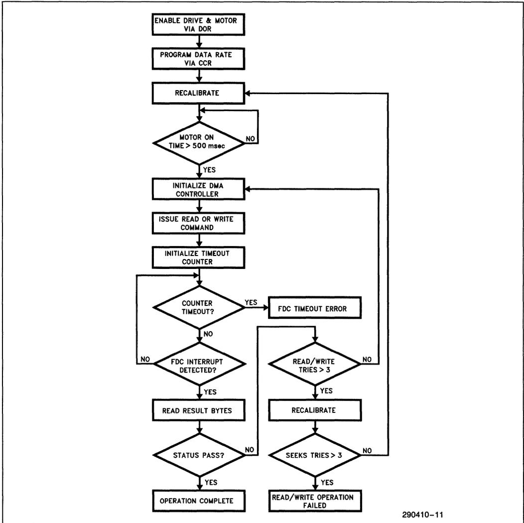
Figure 9-5. Read/Write Operation
