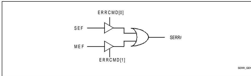
Figure 8. SERR# Generation for Single- or Double-bit Error
