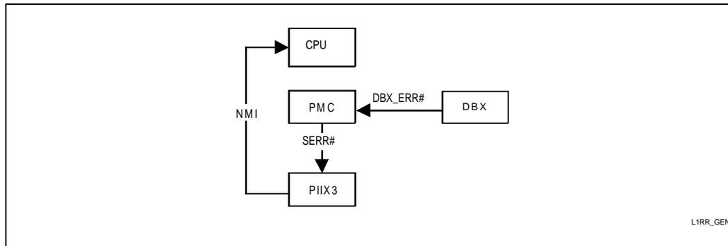
Figure 9. Level 1 SERR# Generation for ECC and Parity
