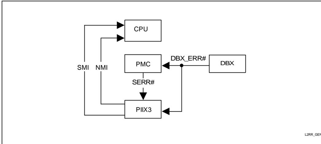
**Figure 10. Level 2 SERR# Generation for ECC and Parity**
