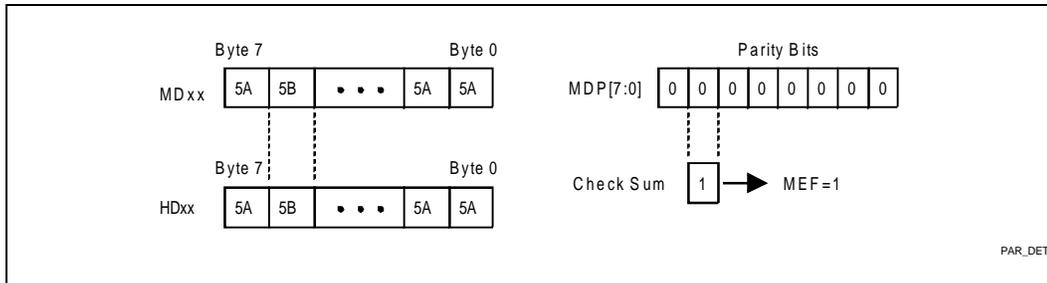
Figure 5. Parity Detection
