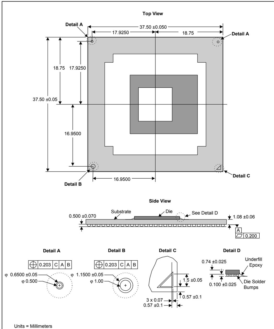
Figure 7-4. Intel® 82845G GMCH Package Dimensions (Bottom View)
