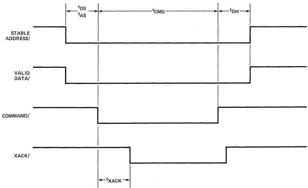
Figure 2. Write Data Transfer
