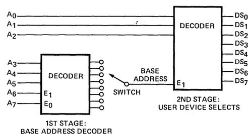
Figure 5. Two Stage Decoding Scheme
