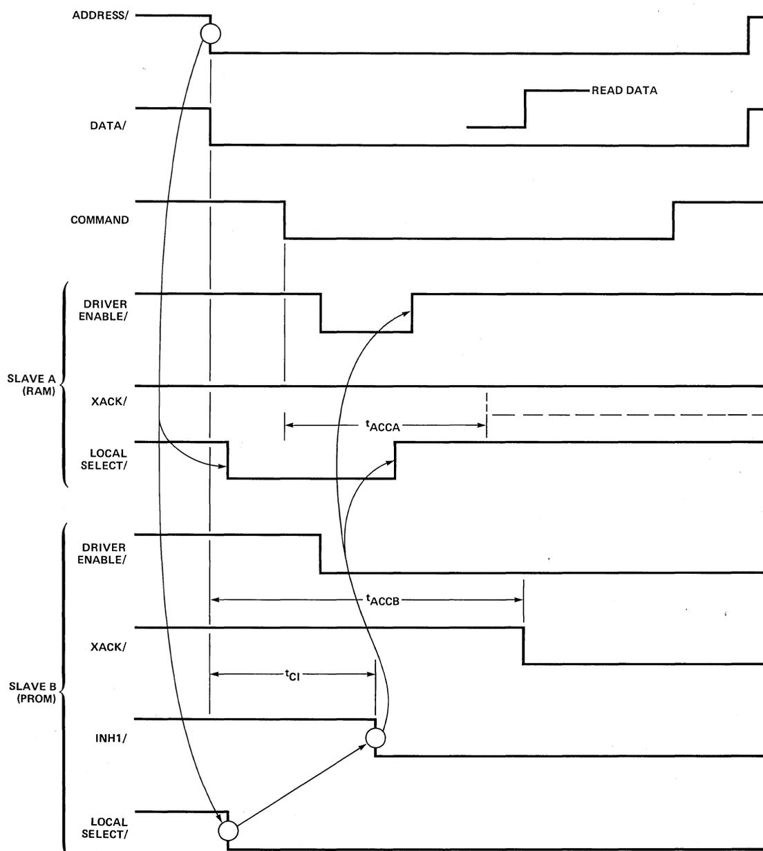
Figure 3. Inhibit Operation
