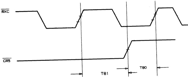
FIGURE 8.15: CRS TIMING RELATIVE TO RxC
