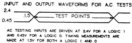
FIGURE 8.10: TTL INPUT/OUTPUT VOLTAGE LEVELS FOR TIMING MEASUREMENTS
