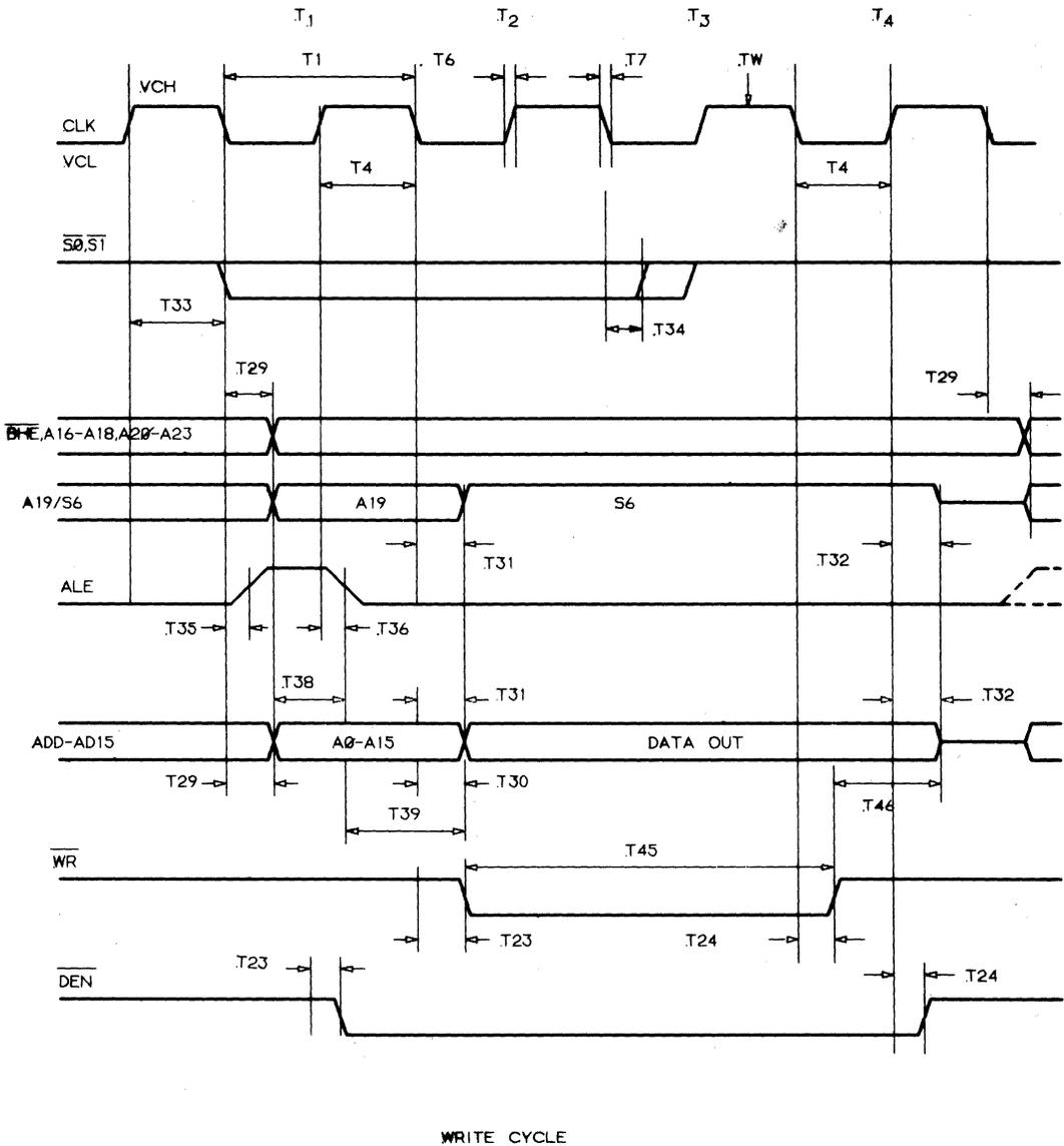
FIGURE 8.9: WRITE CYCLE TIMING
