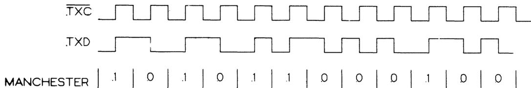
FIGURE 7.4: 82586 MANCHESTER TRANSMITTED DATA RELATIVE TO Tx̄C
