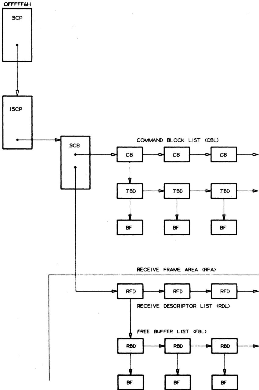
FIGURE 3.1: THE SHARED-82856/CPU MEMORY STRUCTURE
