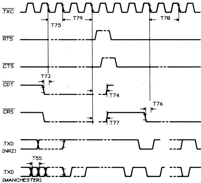
FIGURE 8.13: TRANSMIT CONTROL & DATA TIMING (CONTINUED...)
