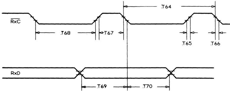
FIGURE 8.14: RxD TIMING RELATIVE TO RxC
