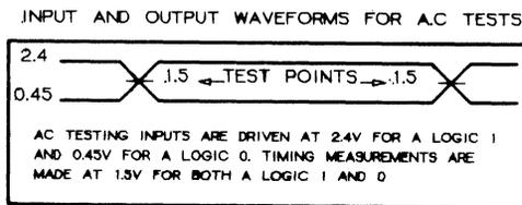
FIGURE 8.1: TTL INPUT/OUTPUT VOLTAGE LEVELS FOR TIMING MEASUREMENTS
