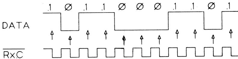
FIGURE 7.2: NRZ RELATIVE TO  $\overline{RxC}$
