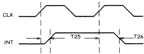
FIGURE 8.3: INT OUTPUT TIMING
