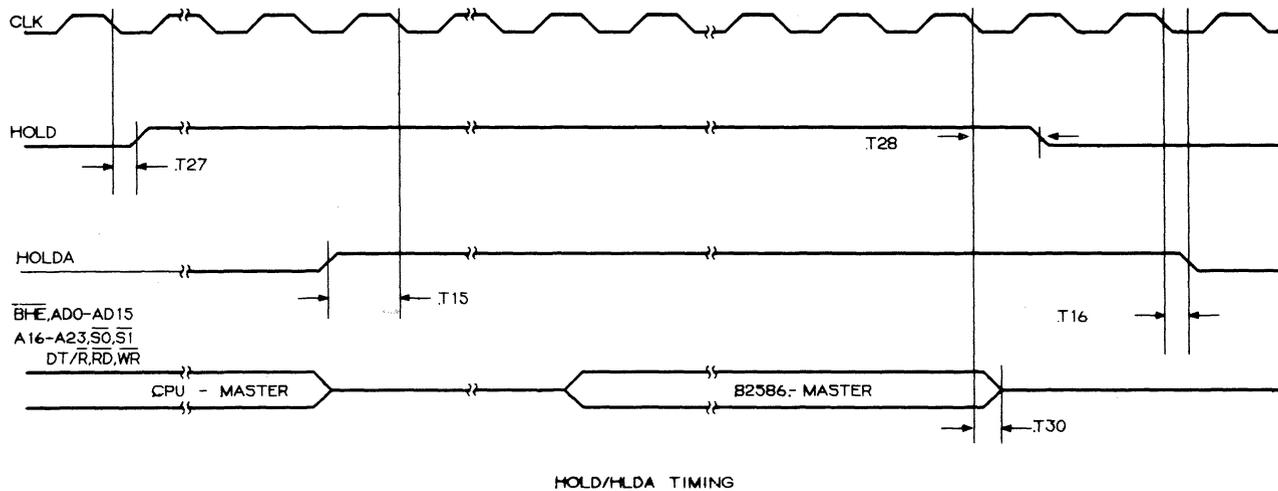
FIGURE 8.7 HOLD/HLDA TIMING RELATIVE TO CLK
