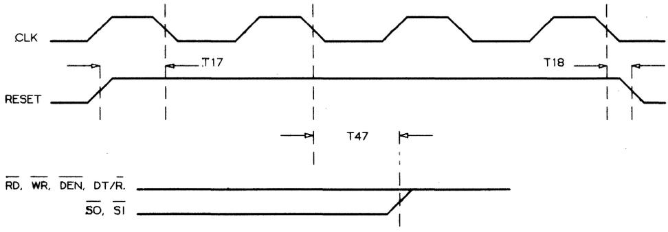
FIGURE 8.5: RESET TIMING
