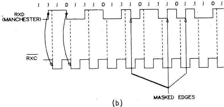
FIGURE 7.5b RECOVERED RxC TIMING RELATIVE TO RxD (b)
