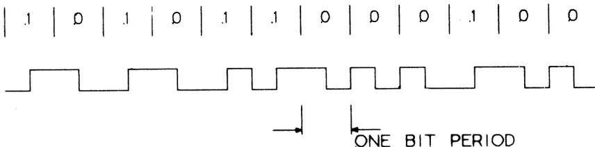
FIGURE 7.3: AN EXAMPLE OF MANCHESTER ENCODED DATA
