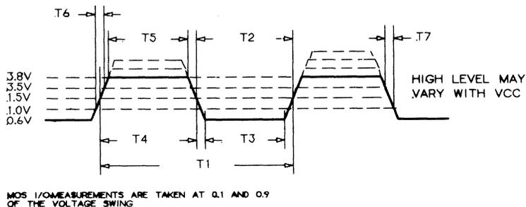
FIGURE 8.2: SYSTEM CLOCK MOS INPUT VOLTAGE LEVELS FOR TIMING MEASUREMENTS
