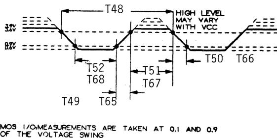
FIGURE 8.11: SERIAL CLOCK INPUT VOLTAGE LEVELS FOR TIMING MEASUREMENTS
