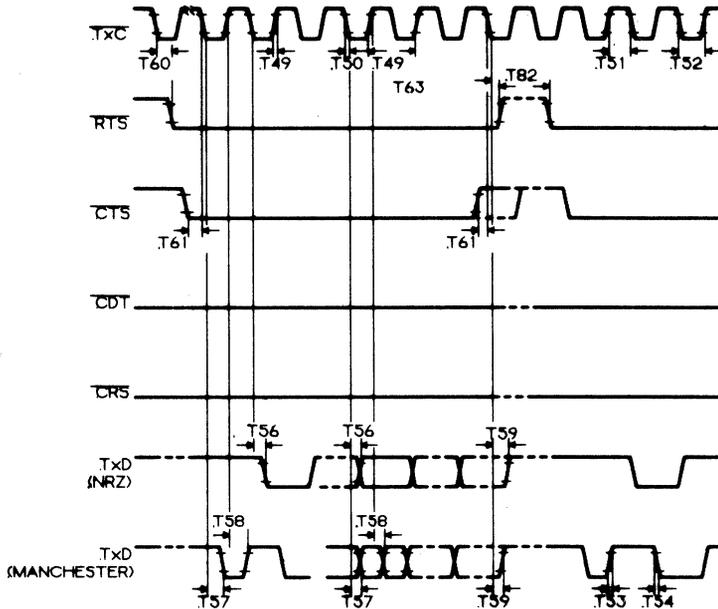
FIGURE 8.12: TRANSMIT AND CONTROL AND DATA TIMING
