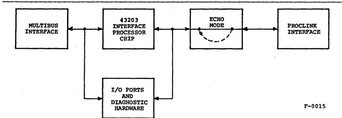
Figure 6-1. Interface Processor Board Functions
