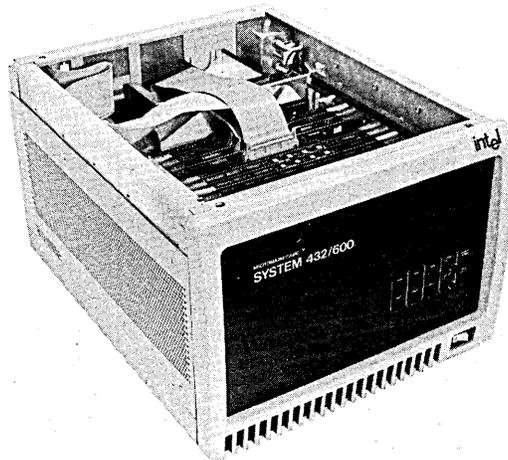
Figure 2-7. iSBC 432/630 Chassis with the System 432/670 Configuration
