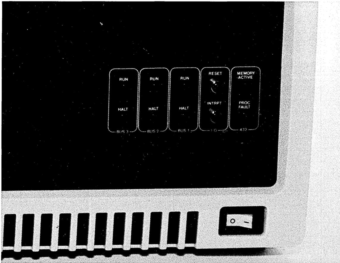
Figure 2-8. Operator's Panel
