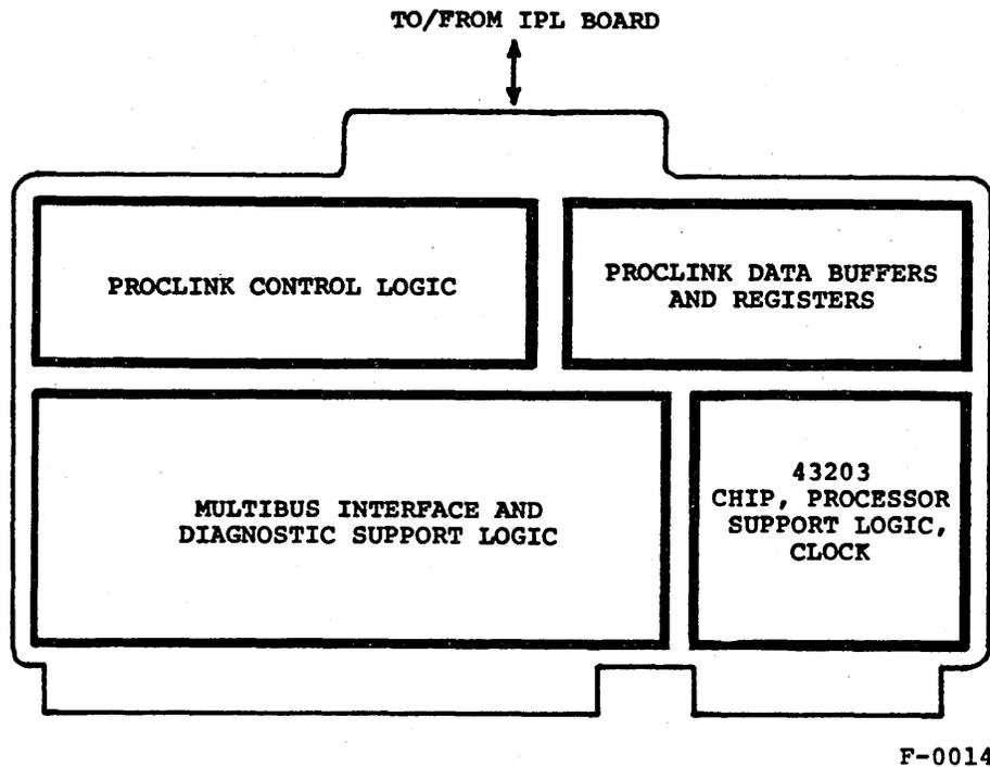
Figure 3-2. Interface Processor Board Block Diagram
