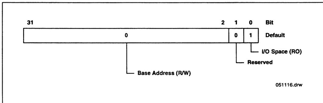
Figure 10. PCI-PCMCIA Bridge Base Address Register
