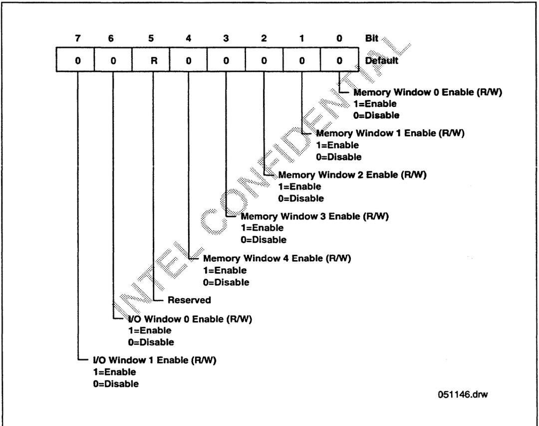
Figure 30. Address Window Enable Register
