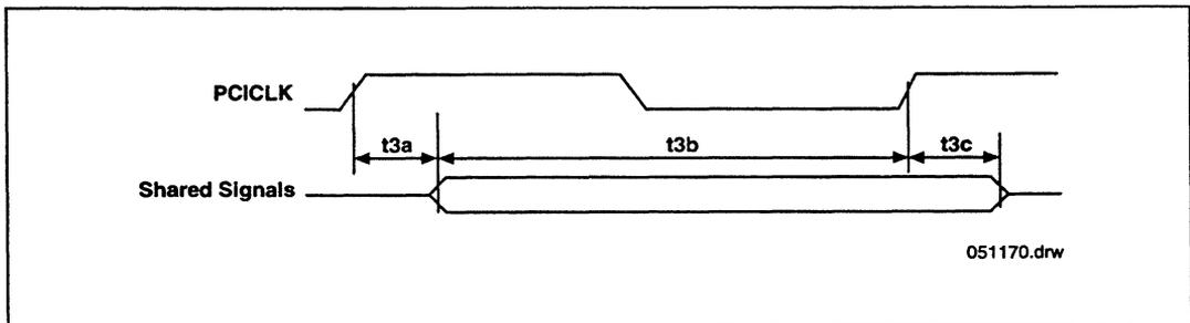
Figure 40. Shared Signal Timing
