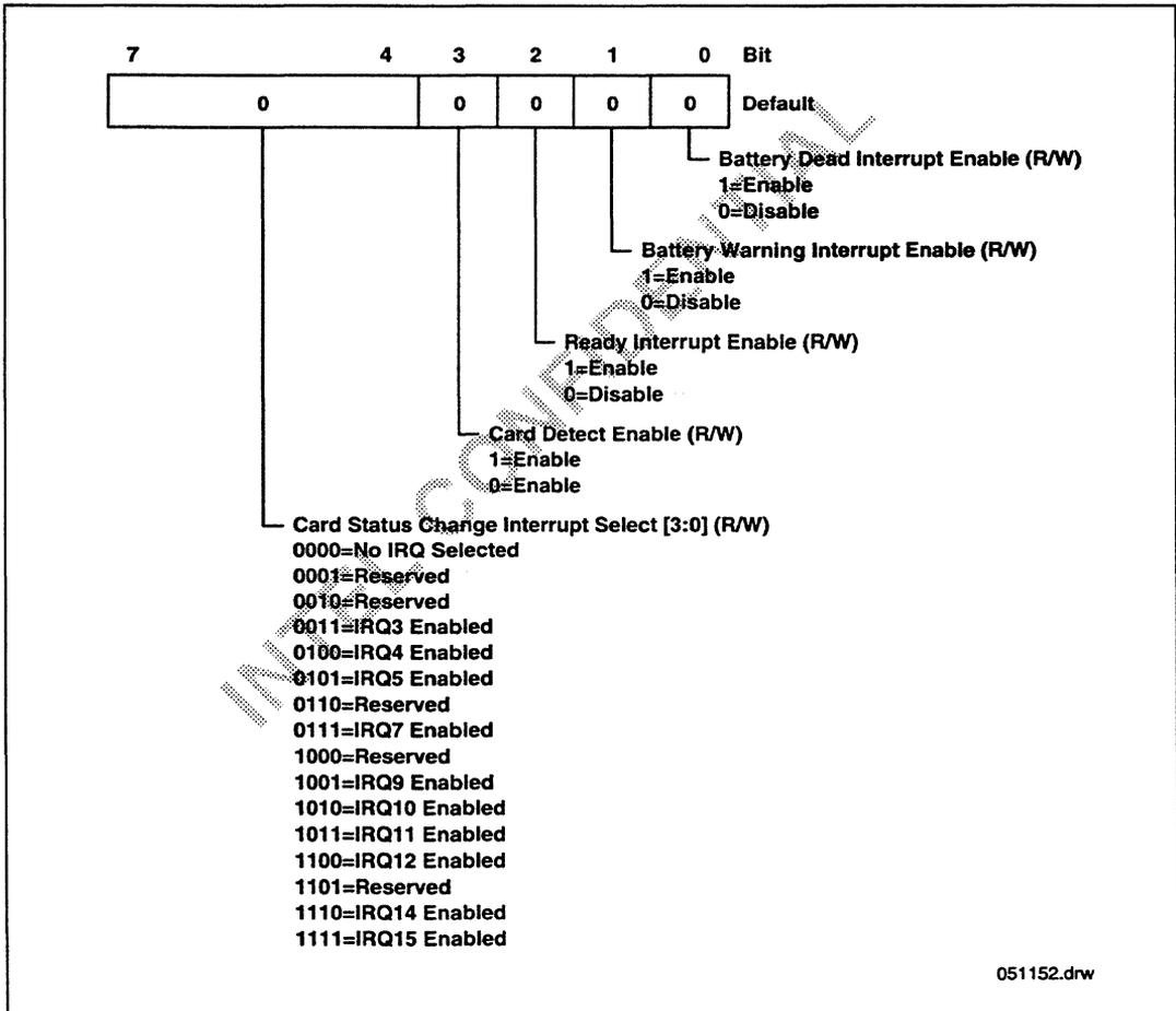
Figure 35. Card Status Change Interrupt Configuration Register
