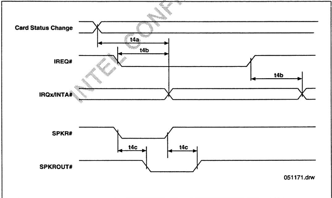
Figure 41. System Signal Timing
