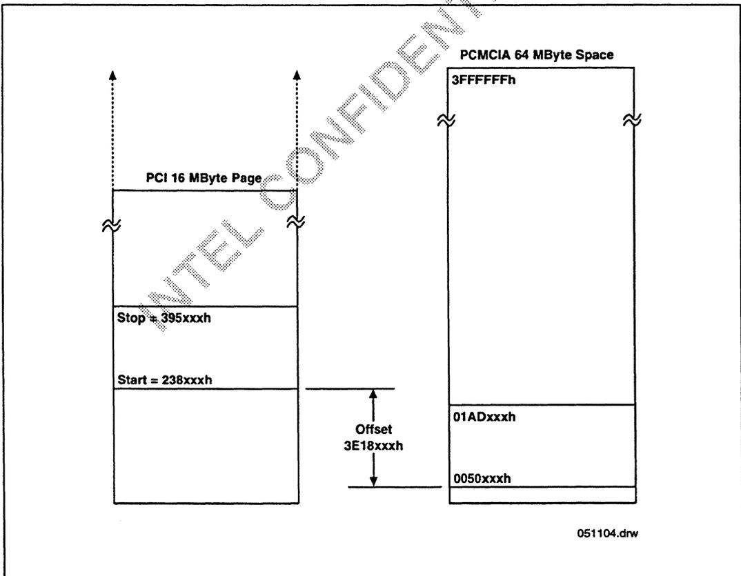
Figure 4. PCMCIA Memory Address Mapping
