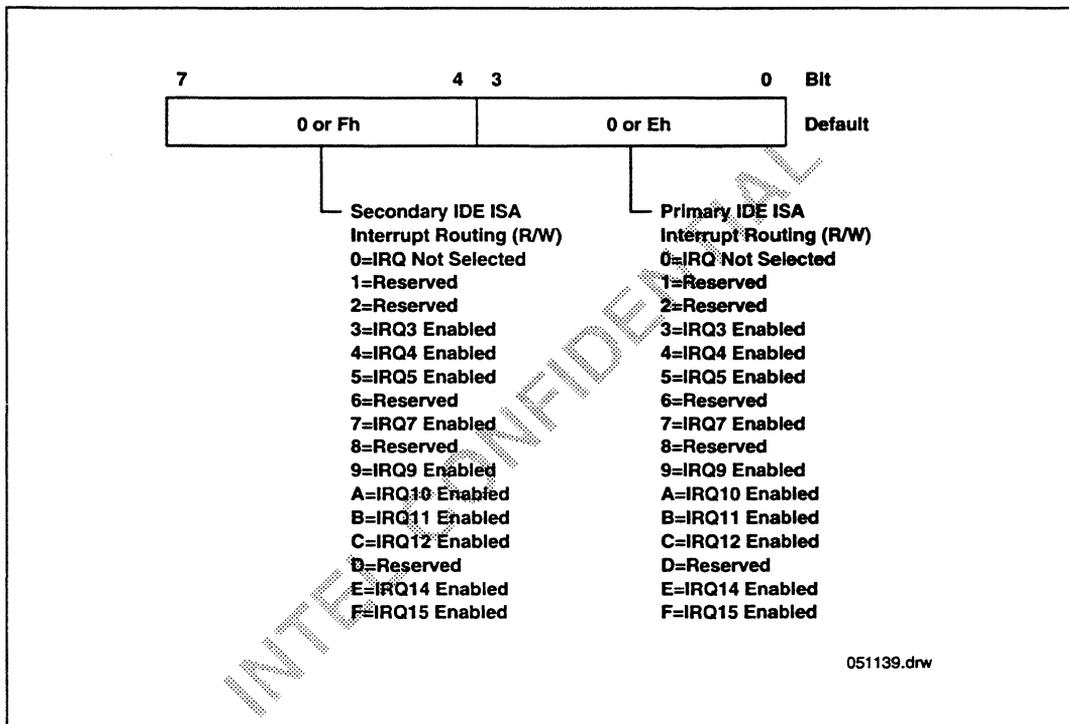
Figure 23. IDE-ISA Interrupt Routing Register
