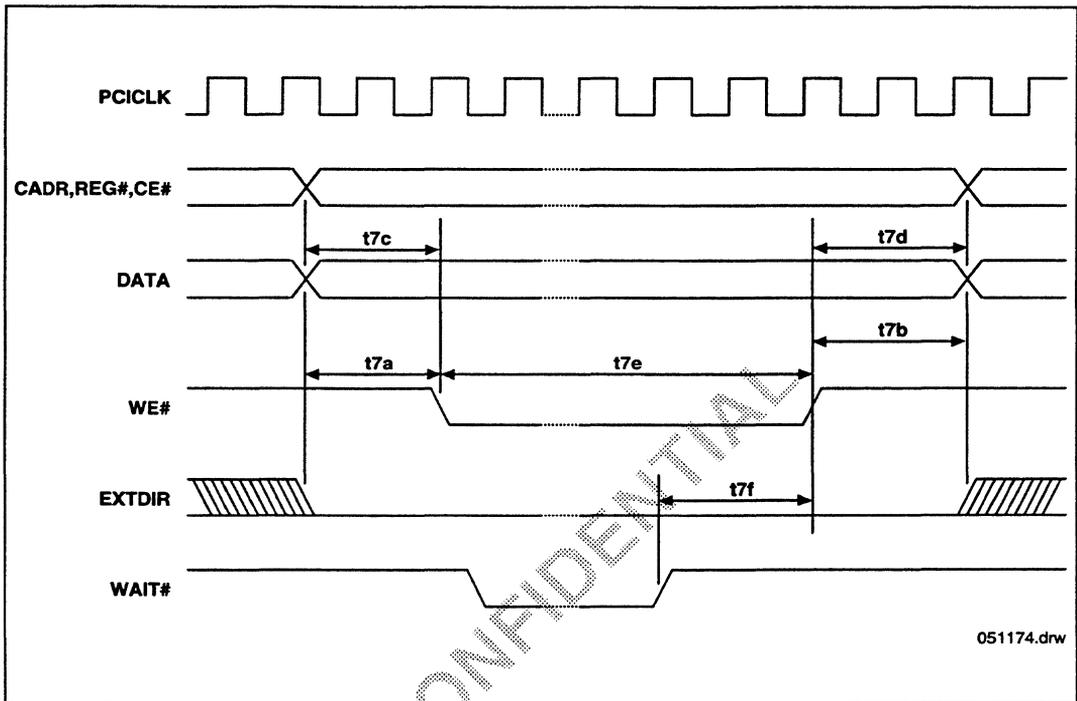
Figure 44. Memory Write Timing
