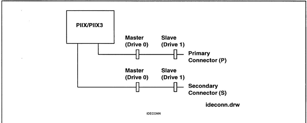
Figure 4. IDE Connector and Drive Nomenclature
