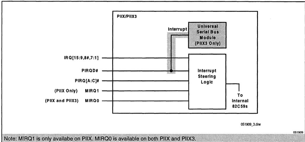
**Figure 8. Interrupt Steering**
