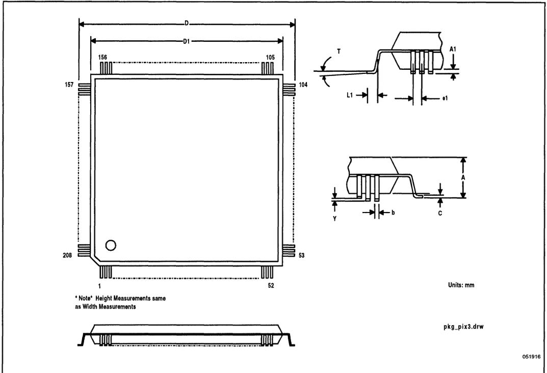
Figure 12. 208 Pin Quad Flat Pack (QFP) Dimensions
