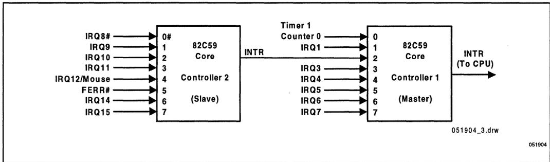
Figure 7. Block Diagram of the Interrupt Controller
