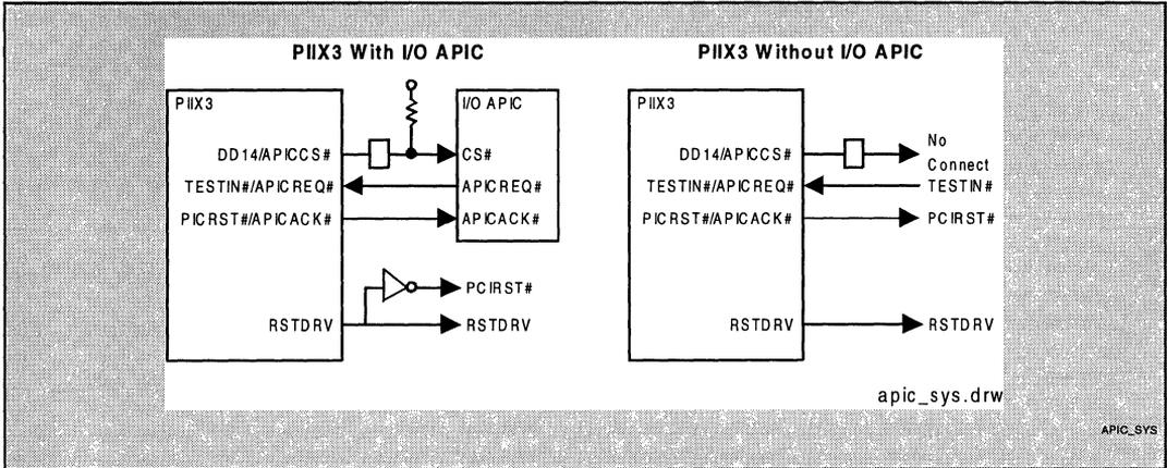
**Figure 9. APIC Signal Connections**
