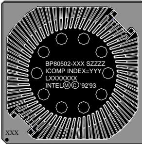
C2, cB1, cC0 and E0-Step Early Boxed Pentium® Processor Fan Heatsink Base Marking:
