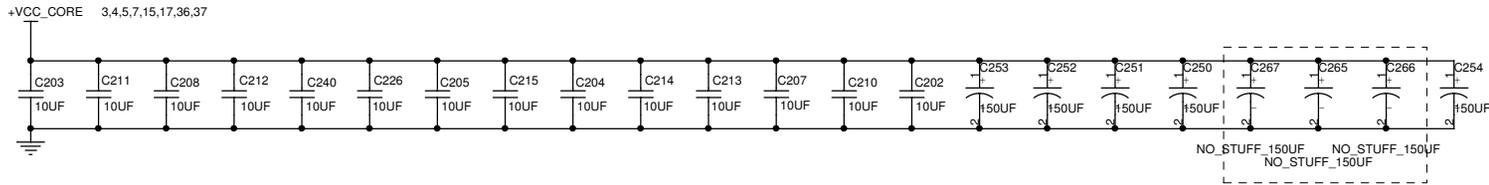
**High Frequency Decoupling (Place underneath Processor)**
