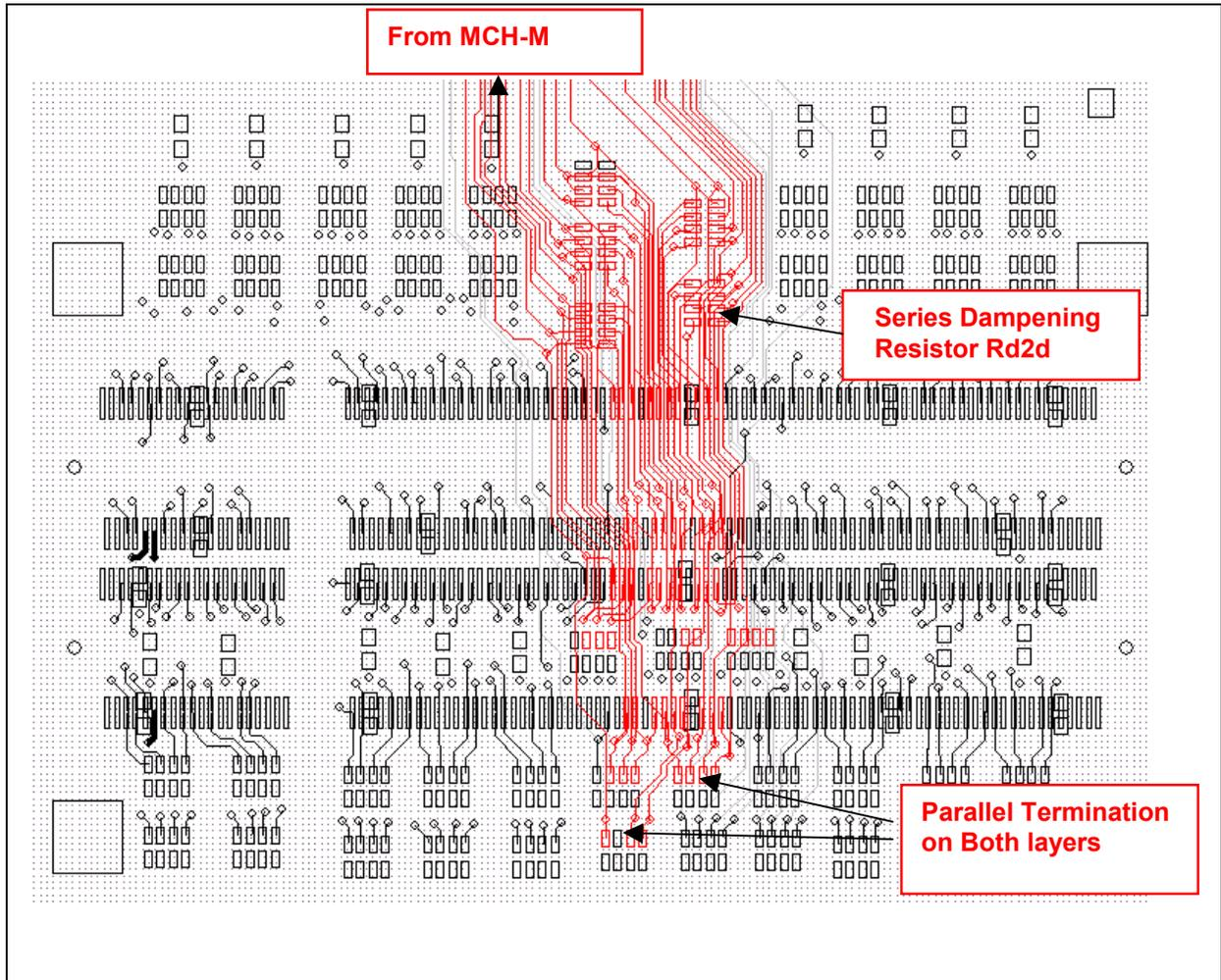
**NOTE:** Red signals are command routing. The majority of the command signal route is on an internal layer; both external layers are used for parallel termination R-pack placement. Note that the series dampening R-packs are rotated to allow for improved power distribution.
