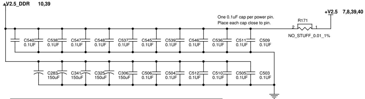
Layout note: Place capacitors between and near DDR connector if possible.
