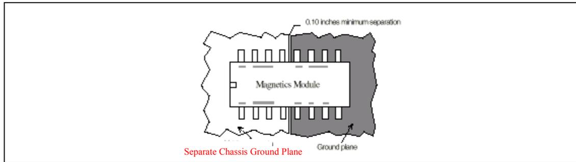
Good grounding requires minimizing inductance levels in the interconnections and keeping ground returns short, signal loop areas small, and power inputs bypassed to signal return, will significantly reduce EMI radiation.
