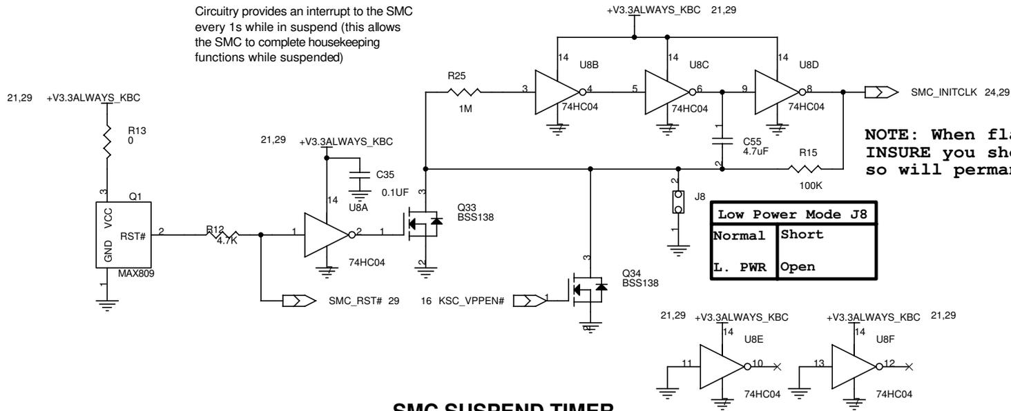
**NOTE: When flashing the KSC INSURE you short J8. Not doing so will permanently damage the KSC.**
