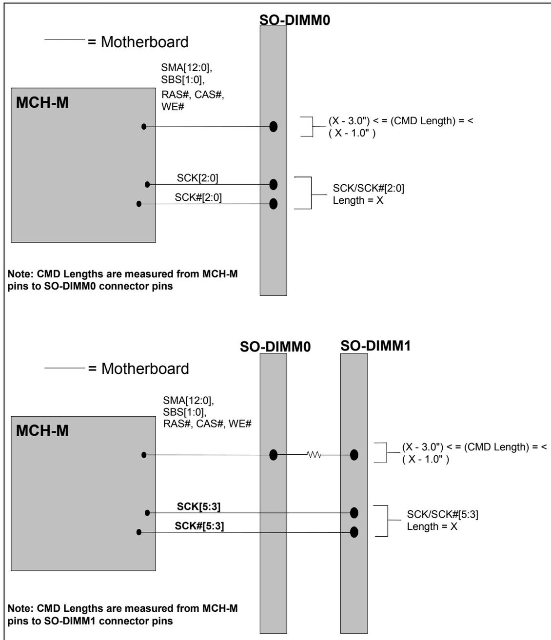
Figure 31. Command Routing Example for Topology 1
