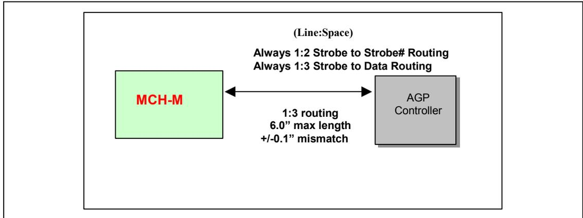
If the AGP interface is less than 6.0 inches, a 1:2 trace spacing is required for 2X/4X lines. These 2X/4X signals must be matched their associated strobe within  $\pm 0.1$  inches. This is for designs that require less than 6 inches between the graphics device and the MCH-M.
