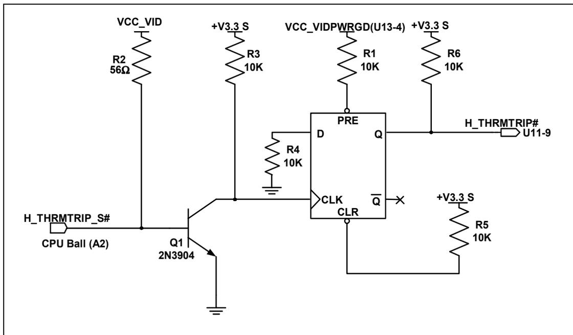
**3.4.4.1.1. Topology #1: Asynchronous AGTL+ Signals Driven by the Processor; FERR#, IERR#, PROCHOT# and THRMTRIP#**
