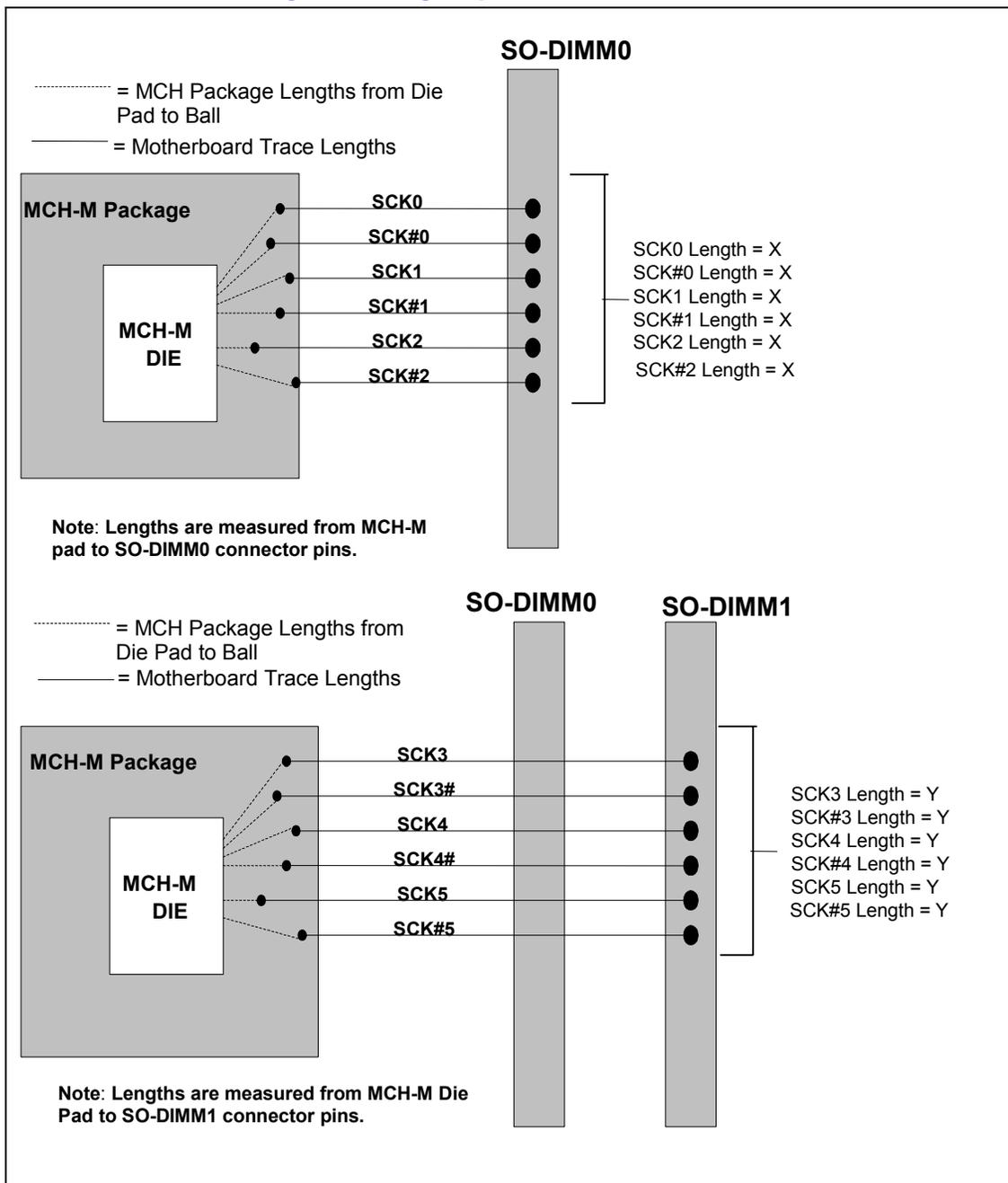
Figure 39. Clock Pair Trace Length Matching Requirements
