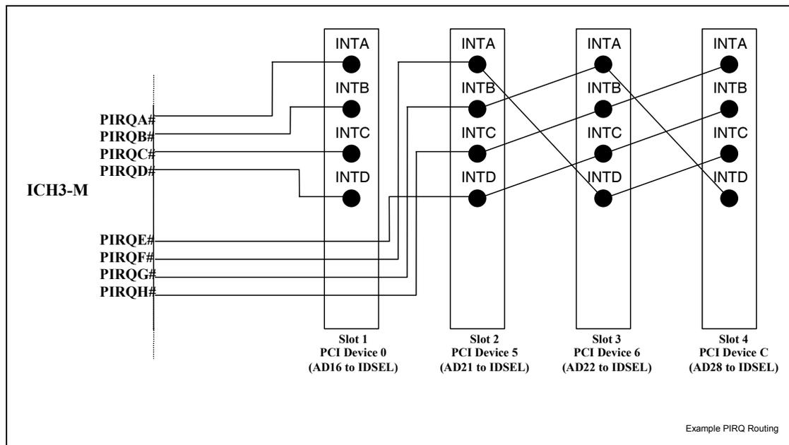
Figure 53 is an example. It is up to the board designer to route these signals in a way that will prove the most efficient for their particular system. A PCI slot can be routed to share interrupts with any of the ICH3-M's internal device/functions (but at a higher latency cost).
