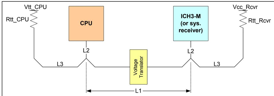
**Note:** If the design is not using the recommended THRMTRIP# latch circuit in Figure 9, THRMTRIP# can be routed through a Voltage Translator to a system logic that can provide the equivalent latching function.
