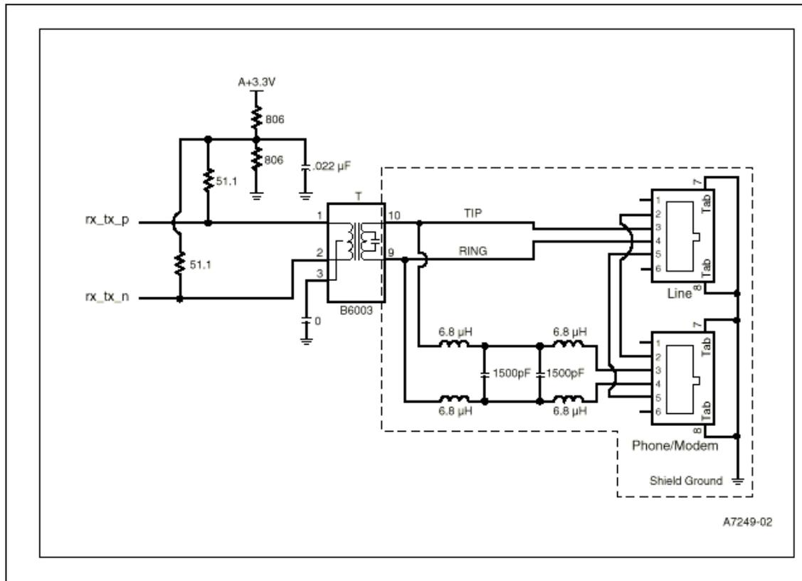
The filter and magnetic component T1, integrates the required filter network, high-voltage impulse protection, and transformer to support the HomePNA\* LAN interface.
