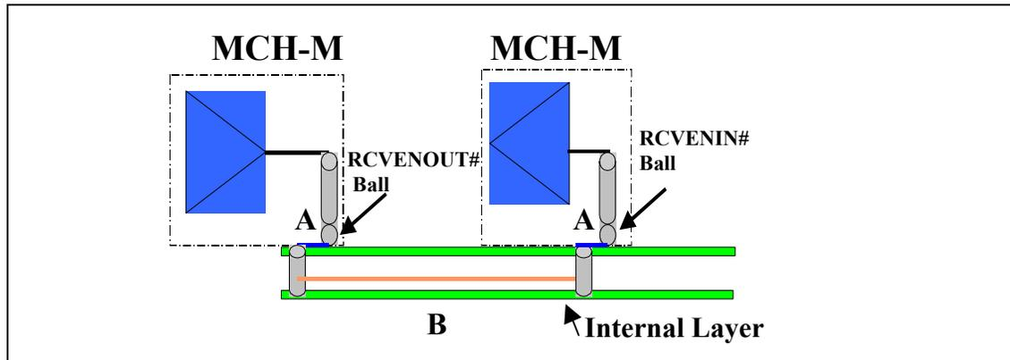
**Table 22. DDR Feedback Signal Routing Guidelines**
