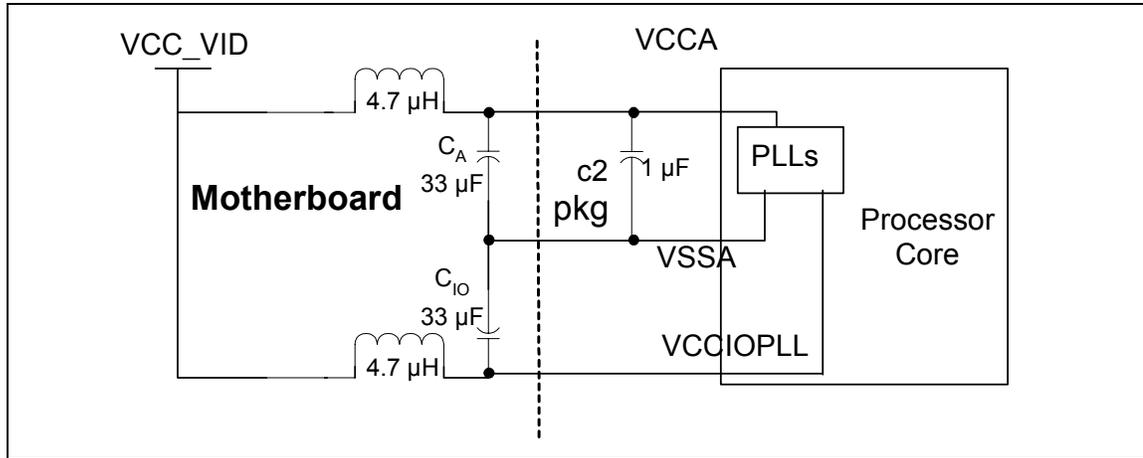
The function of the filter is two-fold. It protects the PLL from external noise through low-pass attenuation. It also protects the PLL from internal noise through high-pass filtering. In general, the low-pass description forms an adequate description for the filter. For simplicity this document will address the recommendation for the  $V_{CCA}$  filter design. The same characteristics and design approach is applicable for the  $V_{CCIOPLL}$  filter design.
