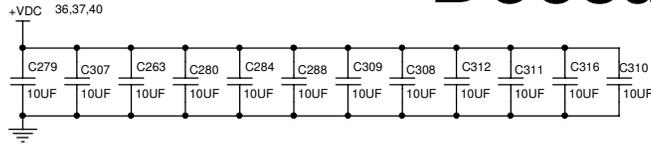
**V CORE Bulk Decoupling**
