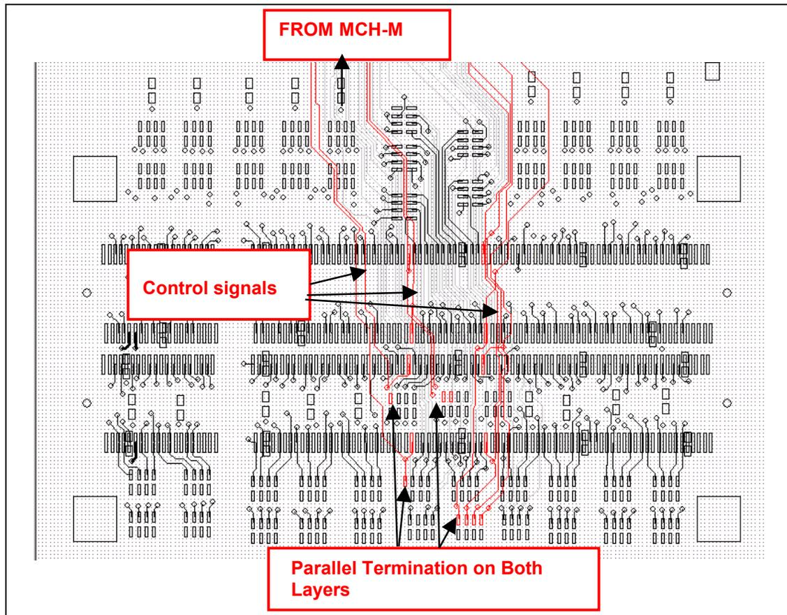
Control routing is shown in red. The majority of the control signal route is on an internal layer, both external layers are used for parallel termination R-pack placement.
