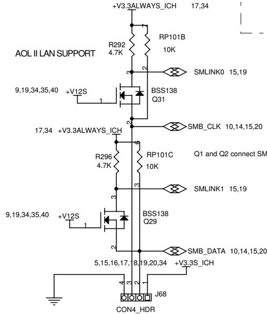
Q1 and Q2 connect SMLINK and SMBUS in S0 for SMBus 2.0 compliance.
