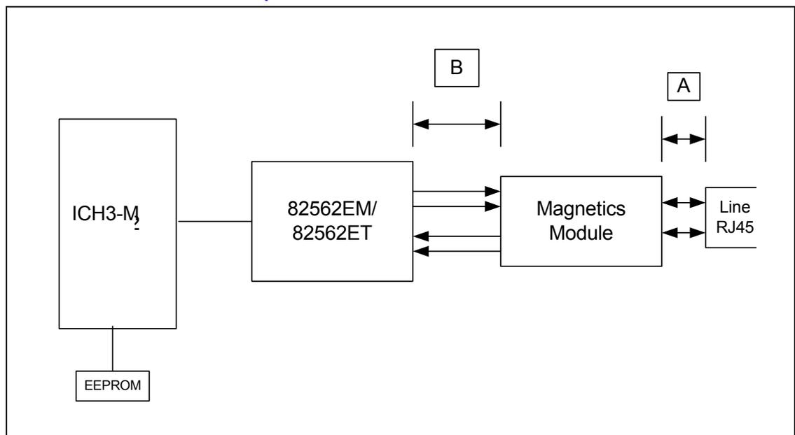
**Table 46. 82562ET / 82562EM Critical Dimensions for Component Placement**
