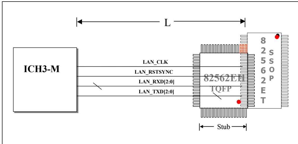
**Figure 74. Dual Footprint Analog Interface**
