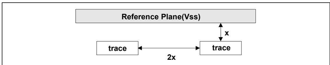
**NOTE:** This is the edge-to-edge trace spacing versus trace to reference plane height.
