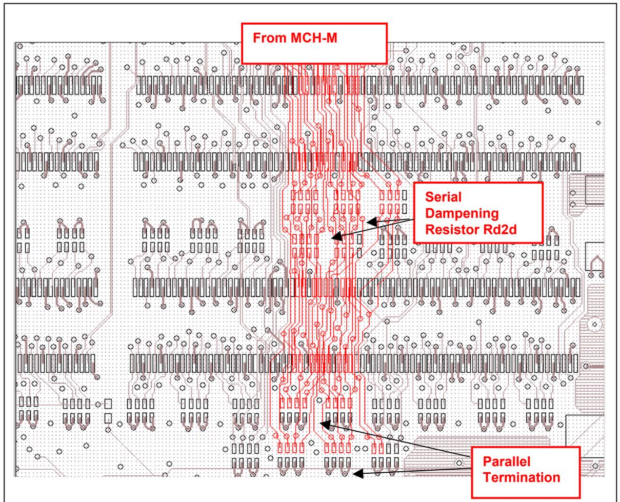
**NOTE:** Red signals are command routing. The majority of the command signal route is on an internal layer.
