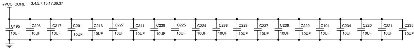
**V CORE Bulk Decoupling (Optional)**
