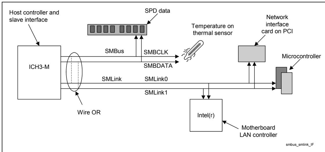
**NOTE:** Intel does not support external access of the ICH3-M's Integrated LAN Controller via the SMLink interface. Also, Intel does not support access of the ICH3-M's SMBus Slave Interface by the ICH3-M's SMBus Host Controller.
