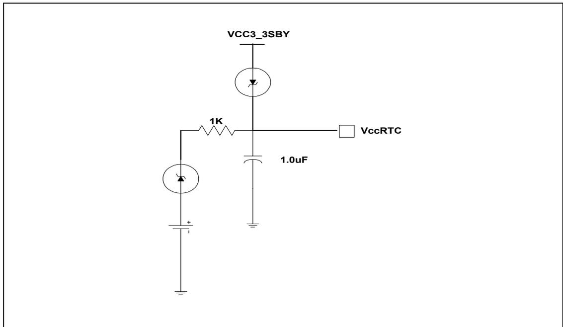
A standby power supply should be used in a mobile system to provide continuous power to the RTC when available, which will significantly increase the RTC battery life and thereby the RTC accuracy.
