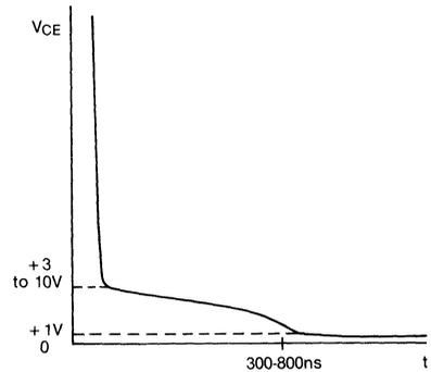
Figure 11. Bipolar Turn-on Plateau
