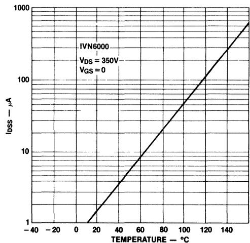
Figure 35. Drain-Source Leakage Current versus Temperature
