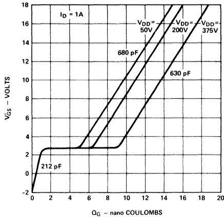
**Figure 3.** Gate Drive Dynamic Characteristics
