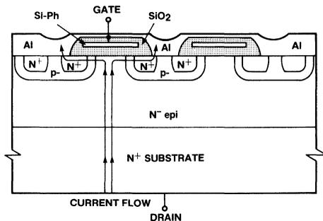
Figure 1. Vertical DMOS Structure
