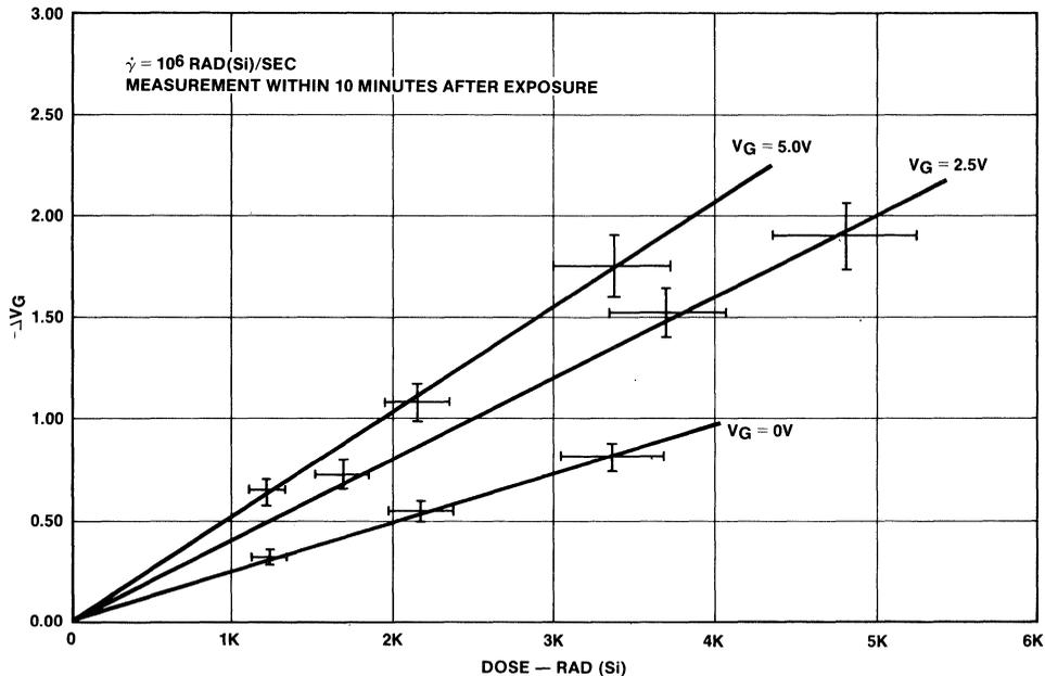
Figure 33. VMOS LINAC Test Results
