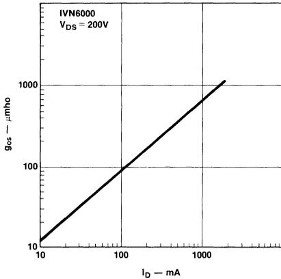
Figure 8. Output Conductance vs. Drain Current
