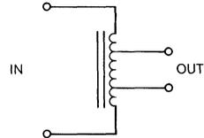
Figure 23. Transmission Line Transformers
