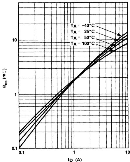
Figure 10. IVN5200  $g_{OS}$  vs.  $I_D$
