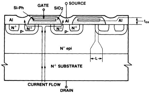
Figure 2. Vertical DMOS Structure
