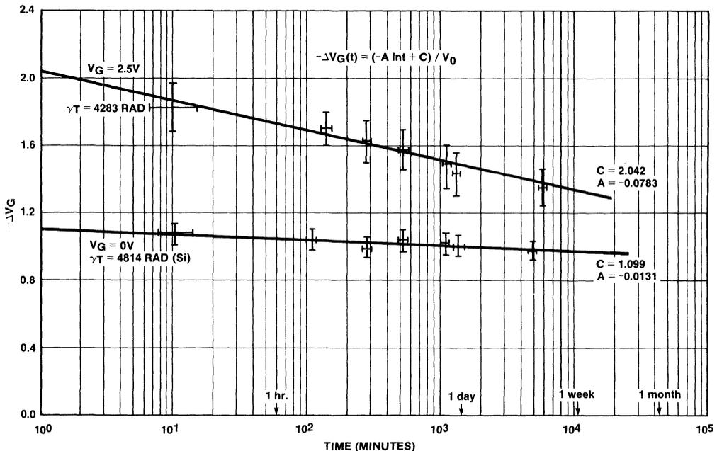
Figure 32. VMOS LINAC Annealing Curves
