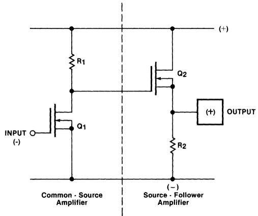
Figure 22. Linear Amplification
