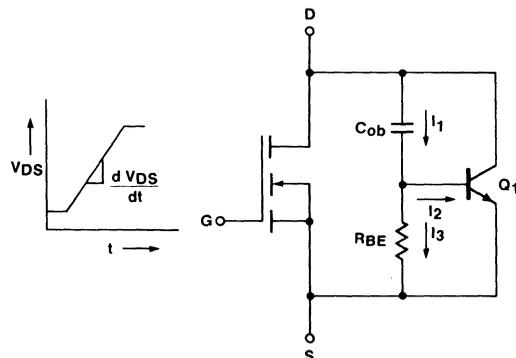
Figure 28. Parasitic Bipolar Switchback Equivalent Circuit
