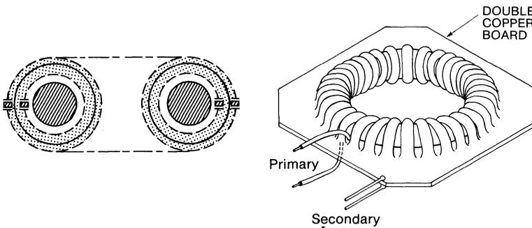
Figure 25. Coaxial Wound Toroid
