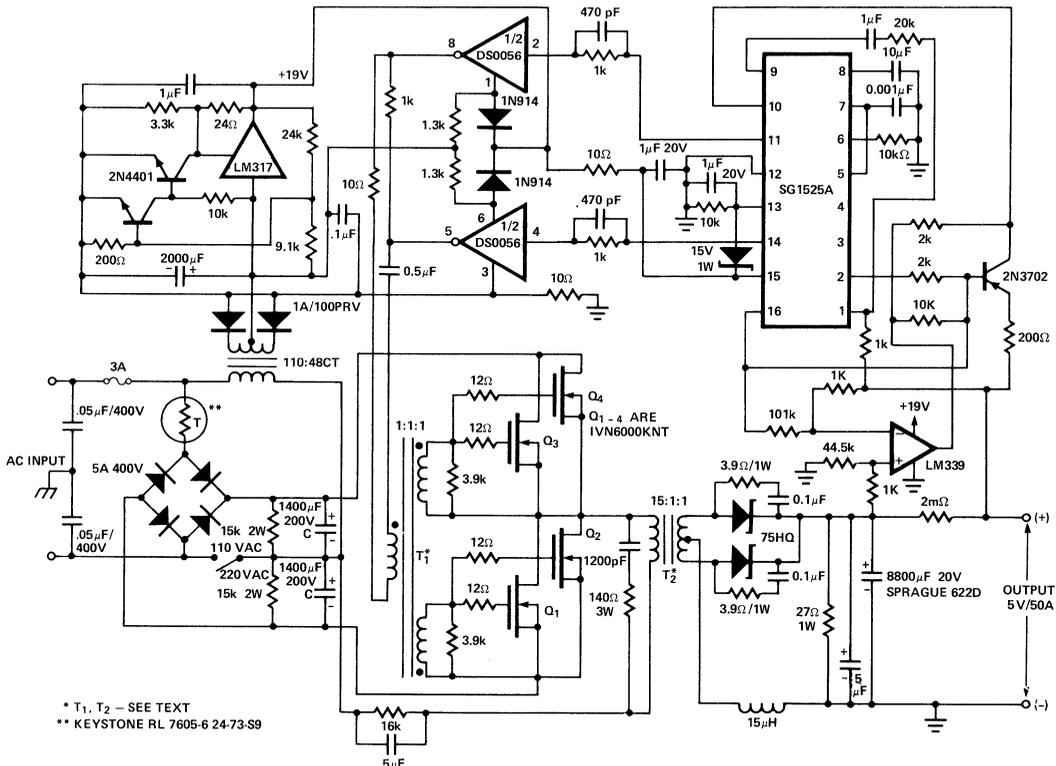
Figure 6. Power MOSFET SMPS
