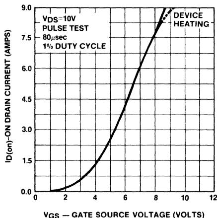
Figure 11. Transfer Characteristic
