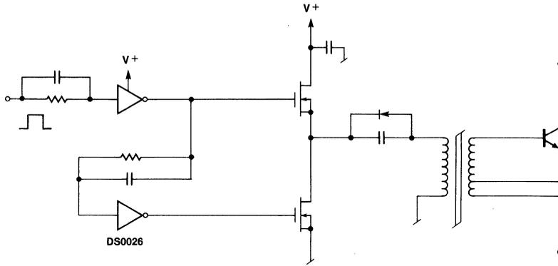
Figure 57. Proportional Base Drive Circuit
