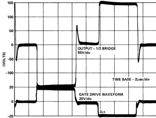
Figure 8. Half Bridge Waveforms (5V/25A Load)
