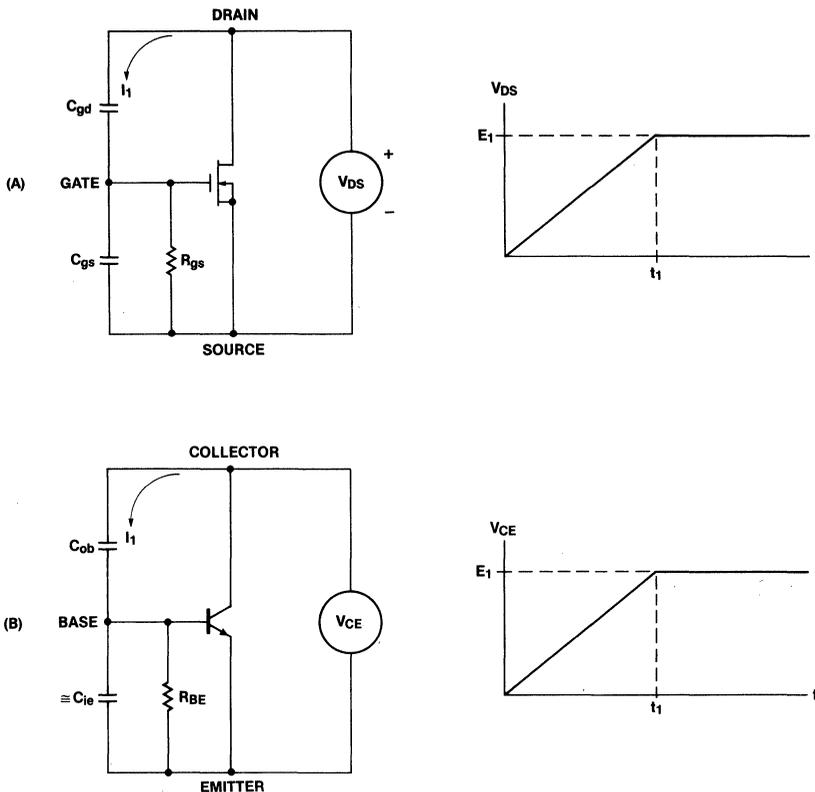
Figure 46. MOSFET and BJT Equivalent Circuits
