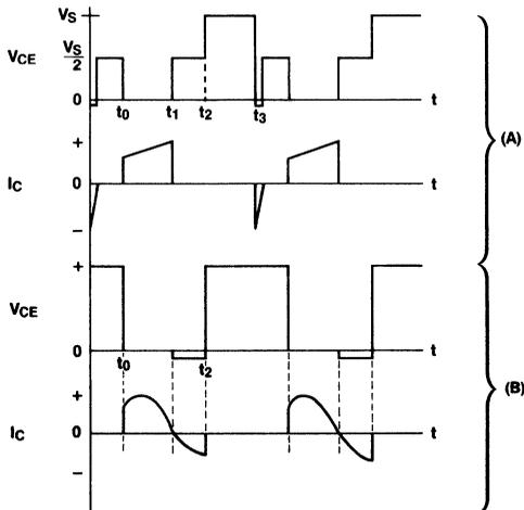
Figure 45. Q<sub>1</sub> Voltage and Current Waveforms
