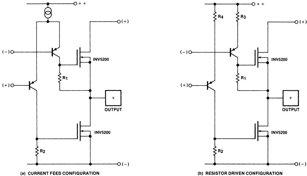
Figures 26a and b. Differential-Complementary Output Configurations
