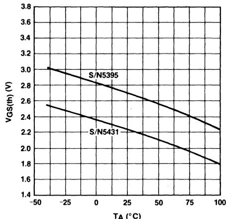
Figure 12. IVN5200  $V_{GS(th)}$  vs.  $T_A$
