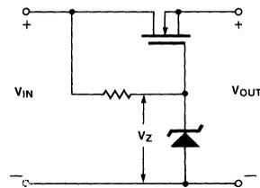
Figure 19. Basic Voltage Regulator
