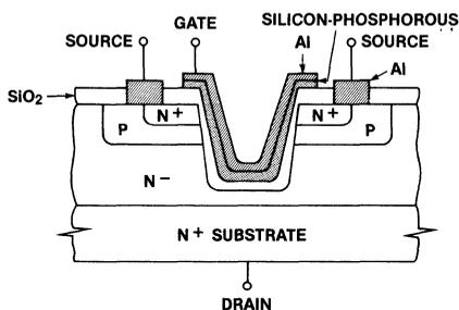
Figure 1. V-Groove MOSFET
