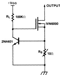
Figure 16. Current Regulator with Loop Gain
