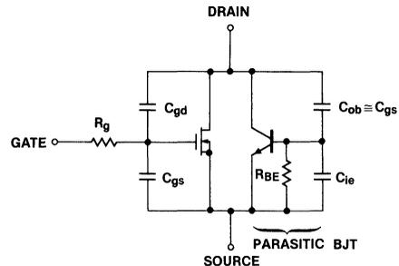
Figure 49. MOSFET Model Including Parasitic BJT
