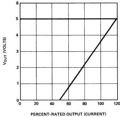
Figure 10. Current Fold-Back Characteristics
