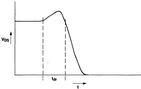
Figure 14. Turn-On Overshoot Due to  $C_{gd}$  and  $t_{dr}$
