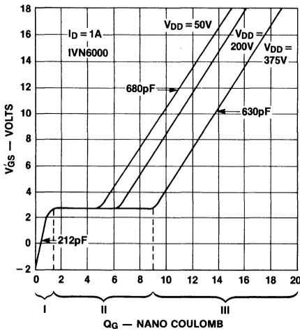
**Figure 6.** Gate Dynamic Characteristics
