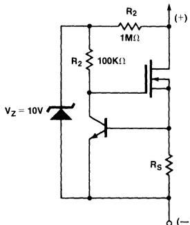
Figure 17. Two-Terminal Current Regulator
