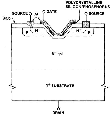
Figure 3. Flat-Bottomed Groove Silicon Gate VMOS
