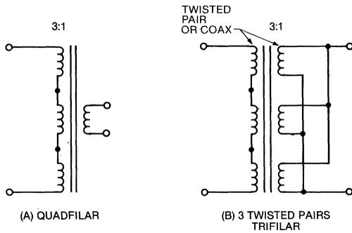
Figure 22. High Frequency Transformer Winding Techniques
