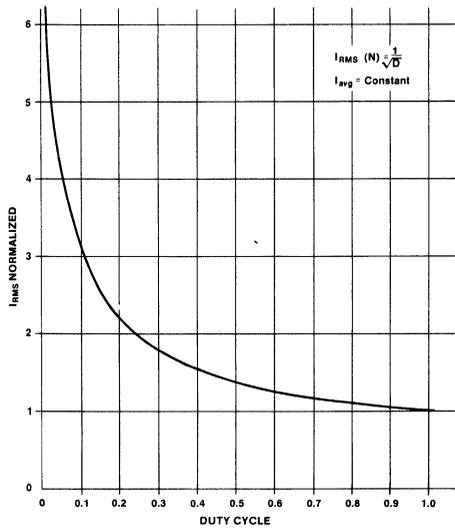
Figure 75: Variation of RMS Current with Duty Cycle.
