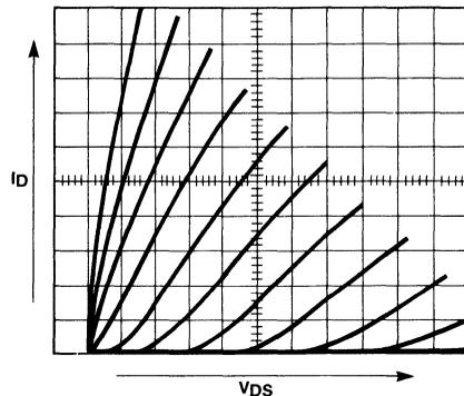
Figure 7. VFET Output Characteristics
