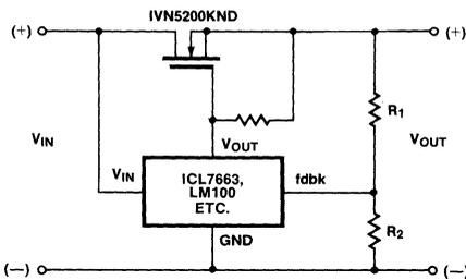
Figure 21. IC-Controlled Regulator
