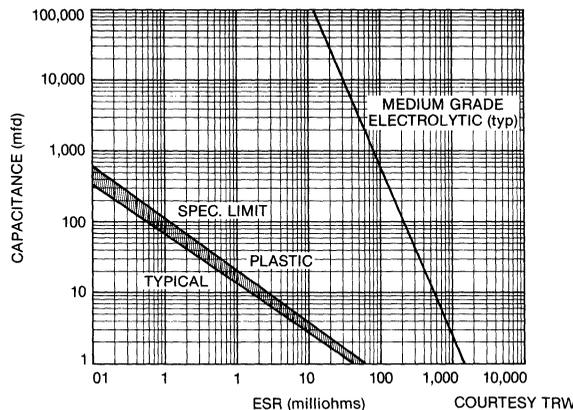
Figure 19. Plastic Film Versus Electrolytic
