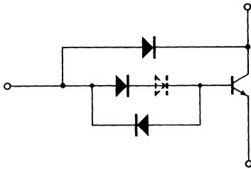
Figure 10. Storage Time Reduction Circuit (Baker Clamp)
