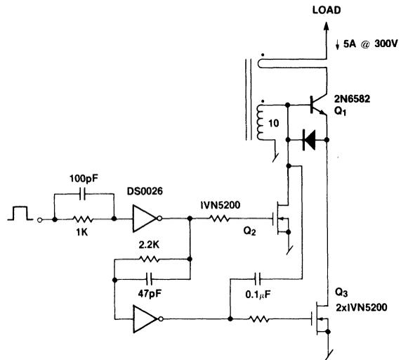
Figure 60. Proportionally Driven Cascode BJT/MOSFET
