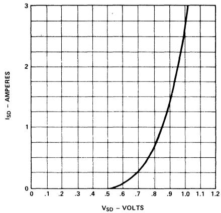
**Figure 4.** Diode Forward Voltage Characteristics
