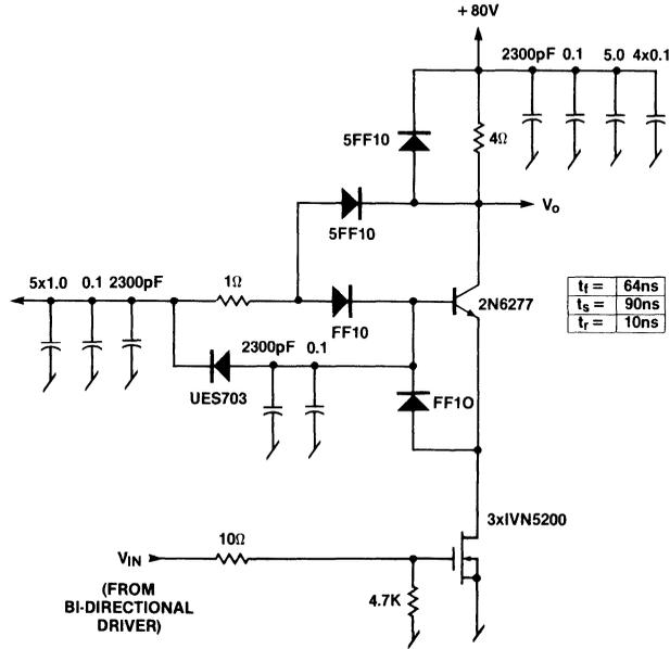
Figure 59. Cascode BJT/MOSFET Circuit
