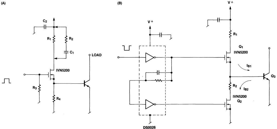
Figure 56. Bipolar Base Drive Using MOSFET
