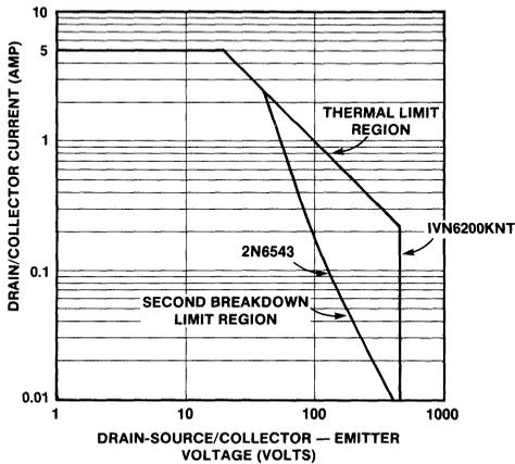
Figure 12. MOSFETs have Extended Safe Operating Area (SOA)
