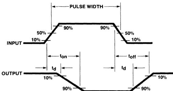
Figure 22. Switching Time Test Waveforms
