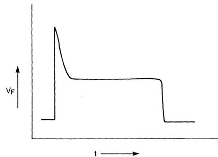
Figure 15. Silicon Junction Diode Forward Recovery Spike
