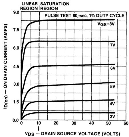
Figure 8. Output Characteristics IVN5200
