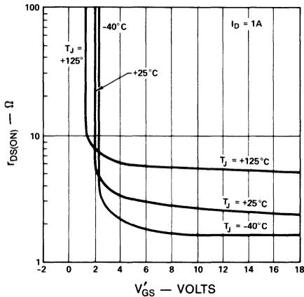
**ON RESISTANCE vs.  $V_{GS}^*$  AS A FUNCTION OF  $I_D$**
