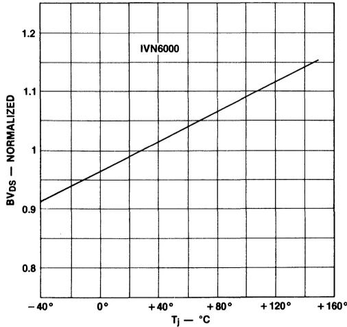
Figure 34. Breakdown Voltage Variation with Temperature
