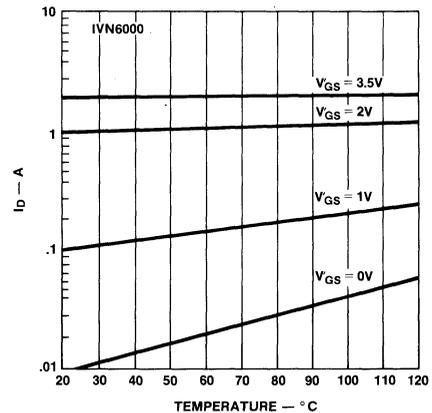
Figure 11. Drain Current
