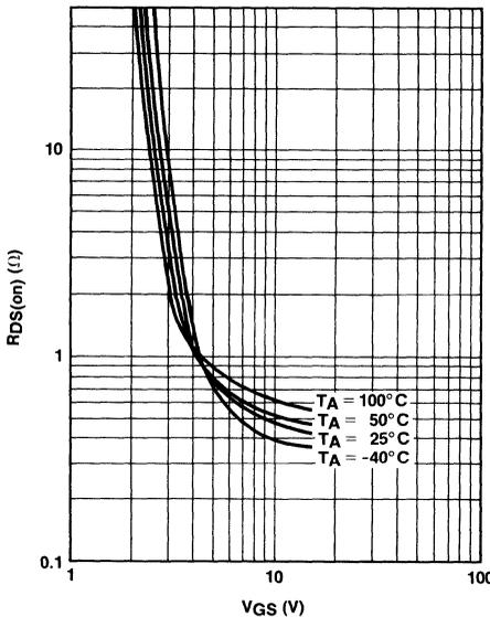
Figure 15. IVN5200  $R_{DS(on)}$  vs.  $V_{GS}$
