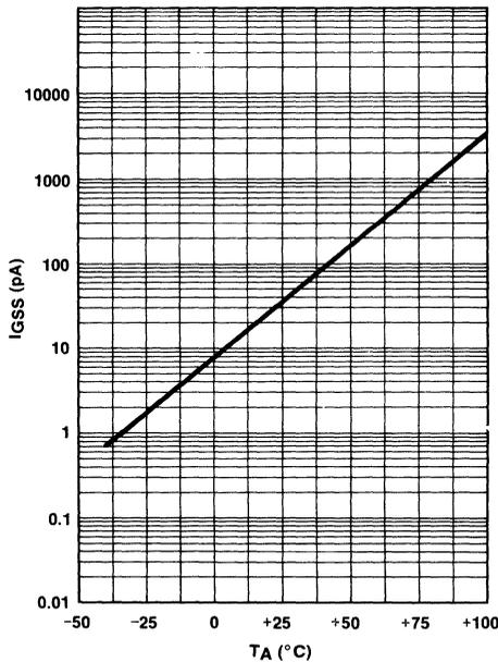
Figure 19. IVN5200 I<sub>GSS</sub> vs. T<sub>A</sub>
