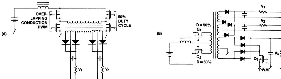
Figure 41. Boost Derived Power Converters
