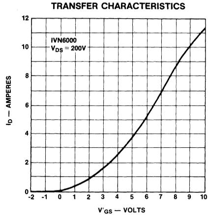
Figure 5. Drain Current vs. Gate-Source Voltage
