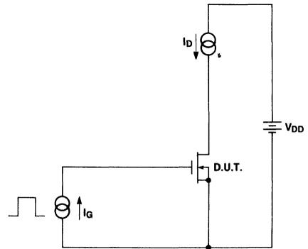
**Figure 7.** Simplified Test Circuit
