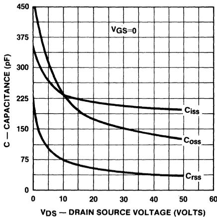
Figure 18. Capacitance vs. Drain-Source Voltage
