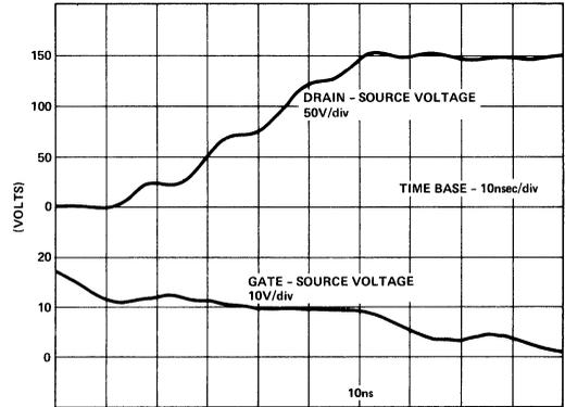
Figure 9. FET Switching Waveforms (5V/25A Load)
