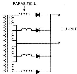
Figure 16. Parallel Diodes
