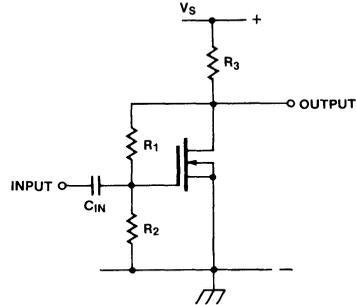
Figure 10. Feedback Bias Configuration
