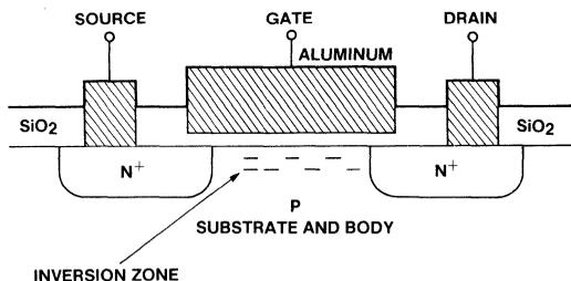
Figure 1. The Cross Section of a Conventional MOSFET
