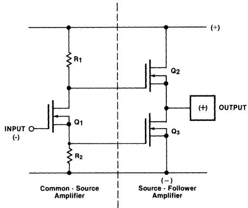
Figure 23. Linear Amplification
