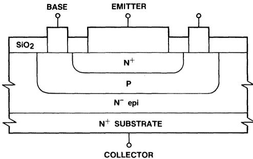
Figure 2B. Typical Double Diffused NPN Transistor
