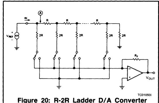
**Figure 20: R-2R Ladder D/A Converter**
