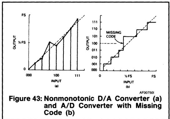
Figure 43: Nonmonotonic D/A Converter (a) and A/D Converter with Missing Code (b)
