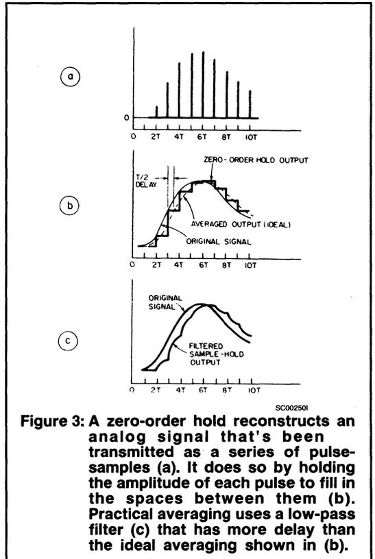
**Figure 3: A zero-order hold reconstructs an analog signal that's been transmitted as a series of pulse-samples (a). It does so by holding the amplitude of each pulse to fill in the spaces between them (b). Practical averaging uses a low-pass filter (c) that has more delay than the ideal averaging shown in (b).**
