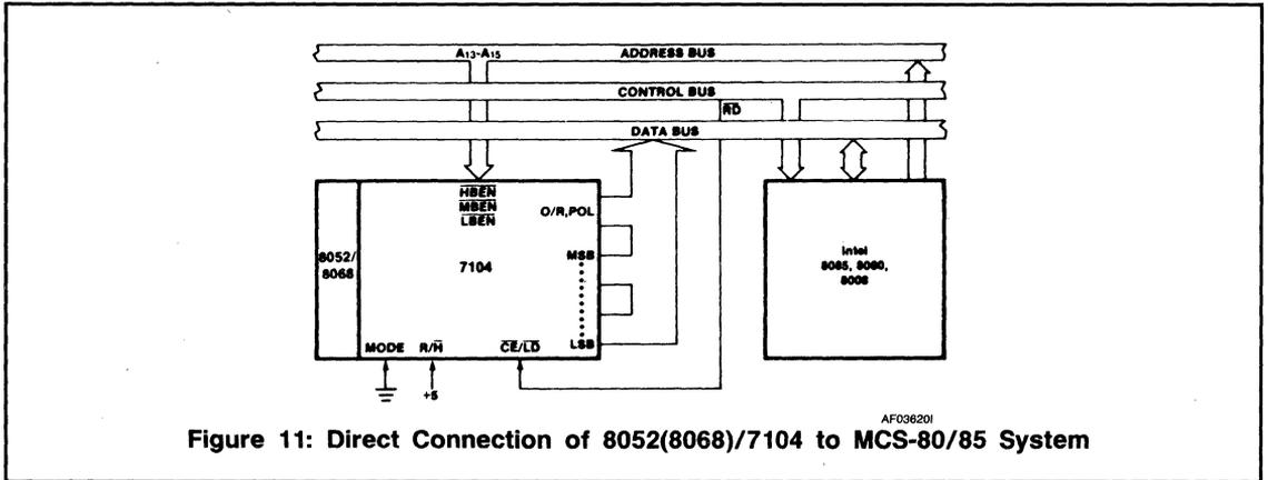
Figure 11: Direct Connection of 8052(8068)/7104 to MCS-80/85 System
