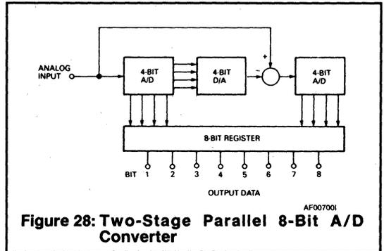
Figure 28: Two-Stage Parallel 8-Bit A/D Converter
