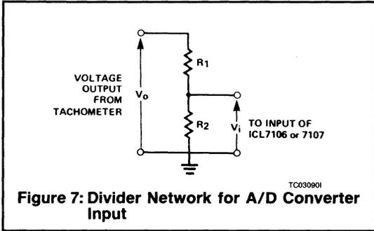
**Figure 7: Divider Network for A/D Converter Input**
