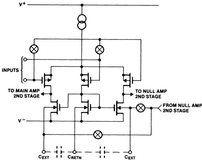
Figure 11: Three-Legged Input Stage (Simplified)
