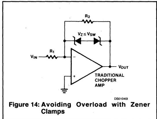
**Figure 14: Avoiding Overload with Zener Clamps**
