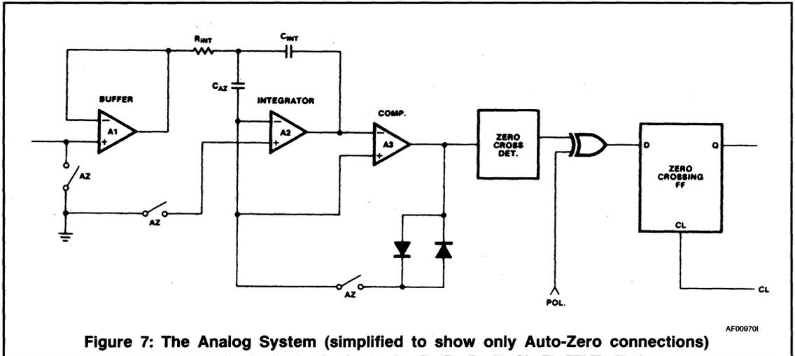
Figure 7: The Analog System (simplified to show only Auto-Zero connections)
