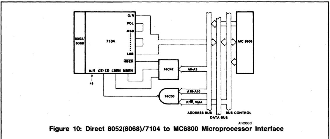
Figure 10: Direct 8052(8068)/7104 to MC6800 Microprocessor Interface
