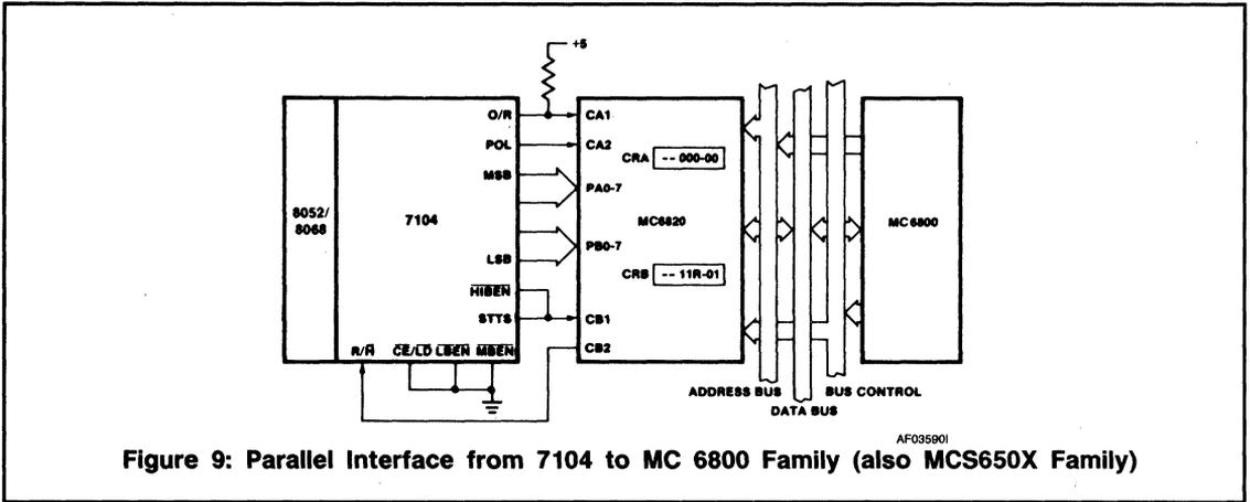
Figure 9: Parallel Interface from 7104 to MC 6800 Family (also MCS650X Family)
