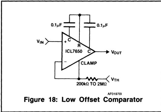
Figure 18: Low Offset Comparator
