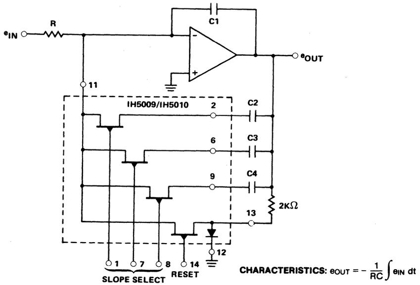
Figure 12: Programmable Slope Integrator
