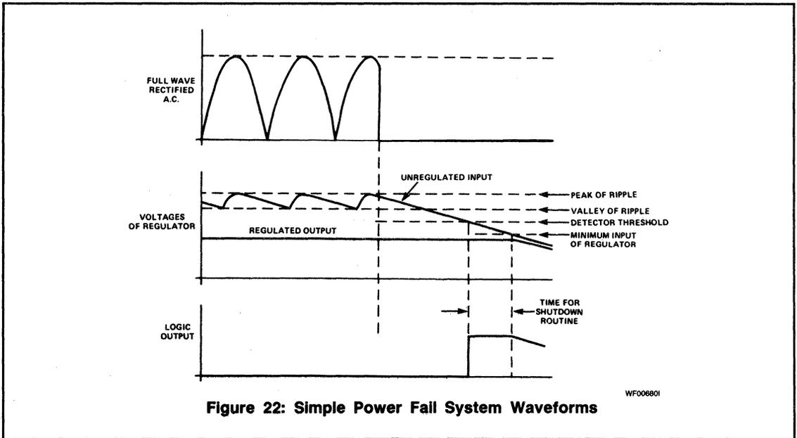
Figure 22: Simple Power Fail System Waveforms
