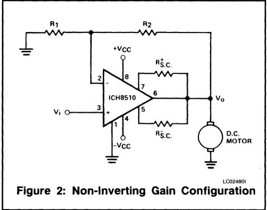
Figure 2: Non-Inverting Gain Configuration
