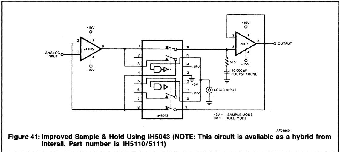
**Figure 41: Improved Sample & Hold Using IH5043 (NOTE: This circuit is available as a hybrid from Intersil. Part number is IH5110/5111)**
