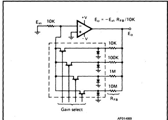
**Figure 4: Programmable gain op-amp has 16 levels of gain, from 1 to 1,000**
