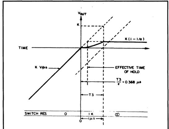
**Figure 9: The effective time at which hold commences occurs before the switch is fully opened.**
