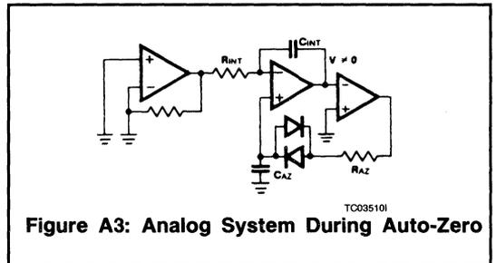
Figure A3: Analog System During Auto-Zero
