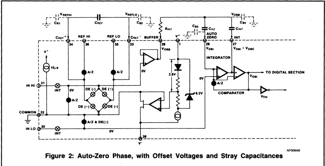
Figure 2: Auto-Zero Phase, with Offset Voltages and Stray Capacitances
