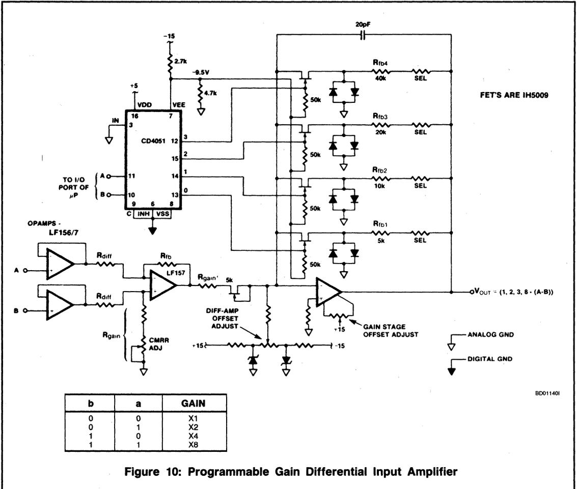
Figure 10: Programmable Gain Differential Input Amplifier
