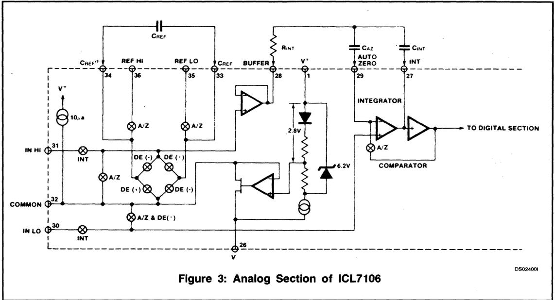
Figure 3: Analog Section of ICL7106
