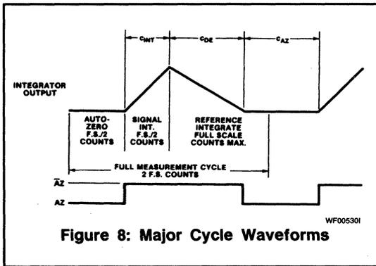
Figure 8: Major Cycle Waveforms
