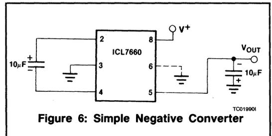
**Figure 6: Simple Negative Converter**
