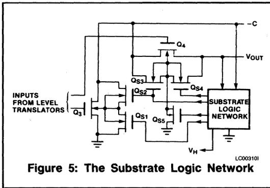
**Figure 5: The Substrate Logic Network**
