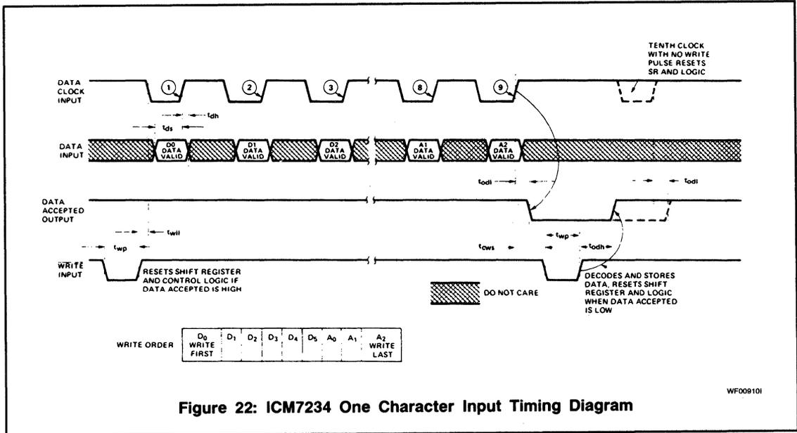
Figure 22: ICM7234 One Character Input Timing Diagram
