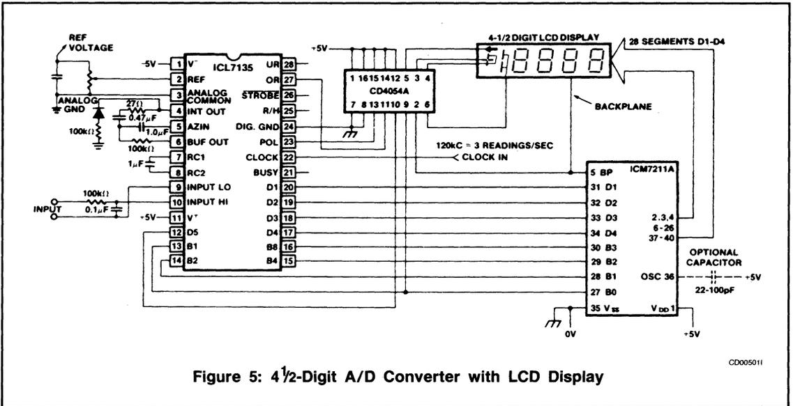
Figure 5: 4 1/2-Digit A/D Converter with LCD Display
