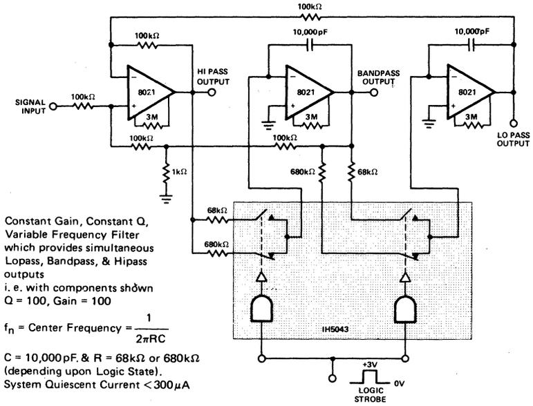
Figure 43: Digitally Tuned Low Power Active Filter
