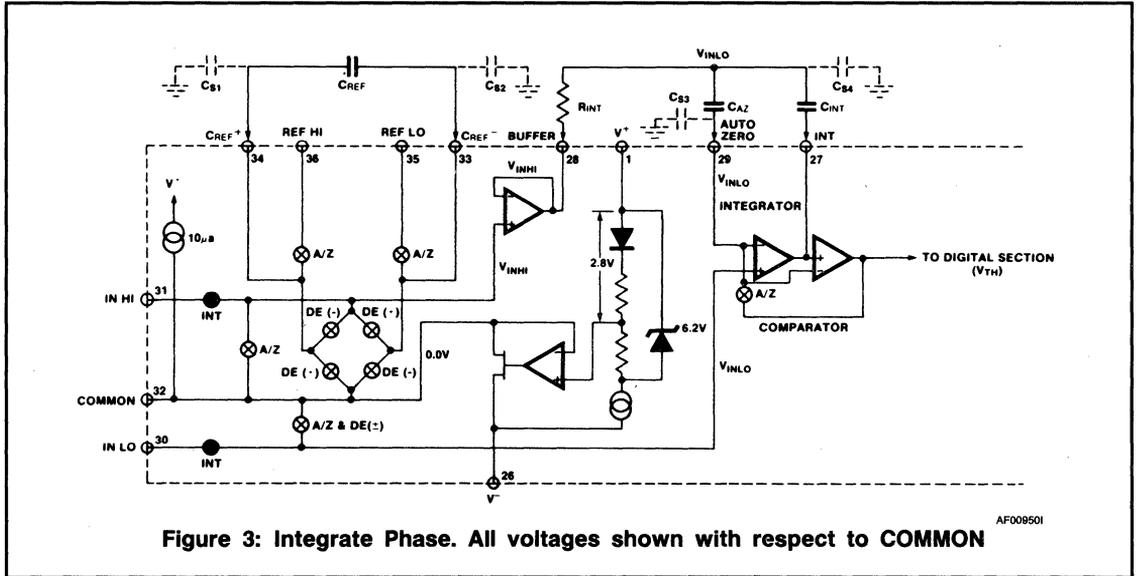
**Figure 3: Integrate Phase. All voltages shown with respect to COMMON**
