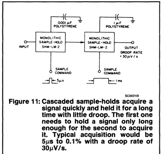
**Figure 11: Cascaded sample-holds acquire a signal quickly and held it for a long time with little droop. The first one needs to hold a signal only long enough for the second to acquire it. Typical acquisition would be 5μs to 0.1% with a droop rate of 30μV/s.**
