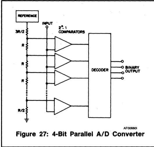
Figure 27: 4-Bit Parallel A/D Converter
