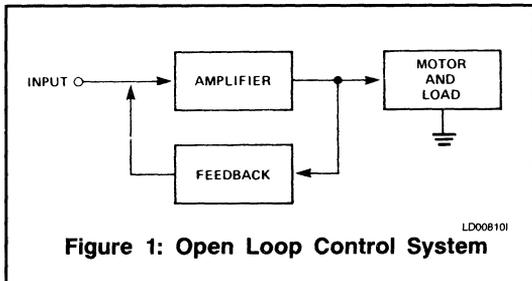
Figure 1: Open Loop Control System
