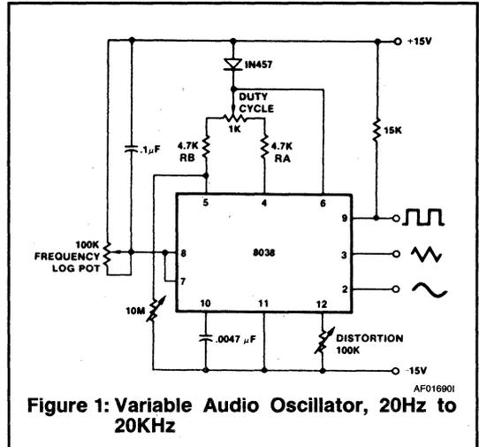
Figure 1: Variable Audio Oscillator, 20Hz to 20KHz
