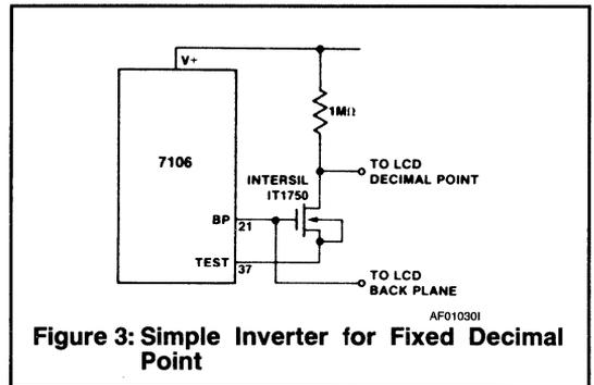
**Figure 3: Simple Inverter for Fixed Decimal Point**
