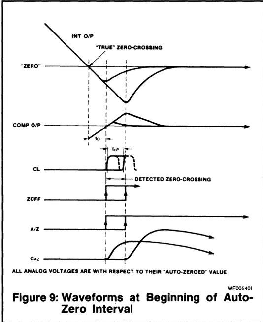
**Figure 9: Waveforms at Beginning of Auto-Zero Interval**
