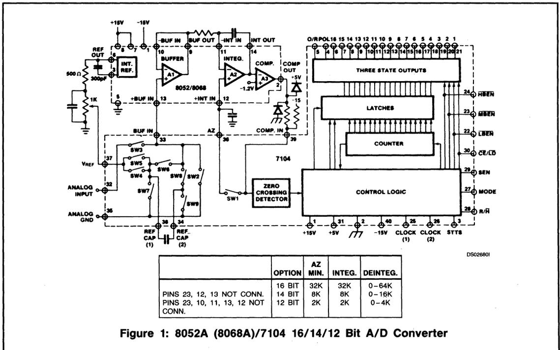
Figure 1: 8052A (8068A)/7104 16/14/12 Bit A/D Converter
