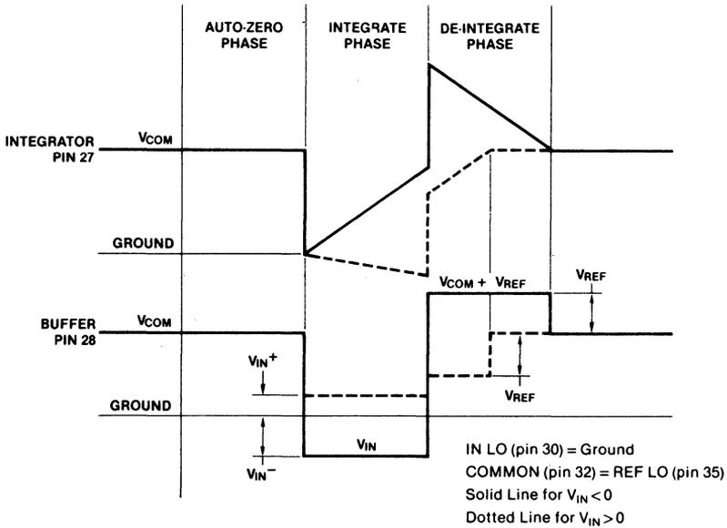
Figure 7: Integrator and Buffer Waveforms for ICL7106, ICL7126 Connected as in Figure 1, or ICL7107 Connected as in Figure 4
