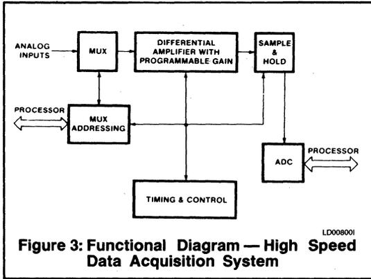
Figure 3: Functional Diagram — High Speed Data Acquisition System
