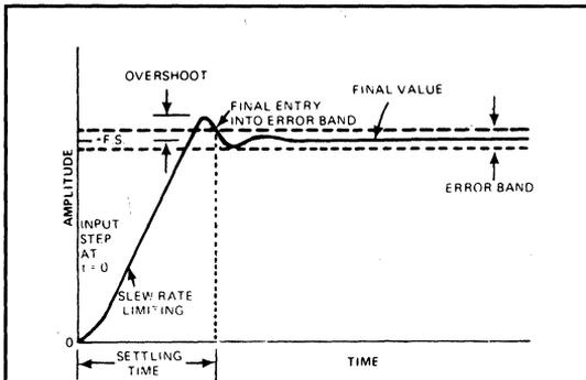
**Figure 2: Slewing time must be included in settling-time measurements.**
