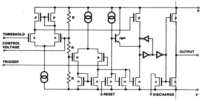
Figure 5: ICM7555/7558 CMOS Single and Dual Timers
