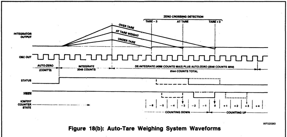
Figure 18(b): Auto-Tare Weighing System Waveforms
