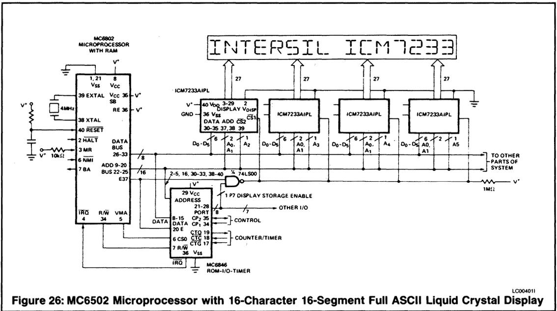
Figure 26: MC6502 Microprocessor with 16-Character 16-Segment Full ASCII Liquid Crystal Display
