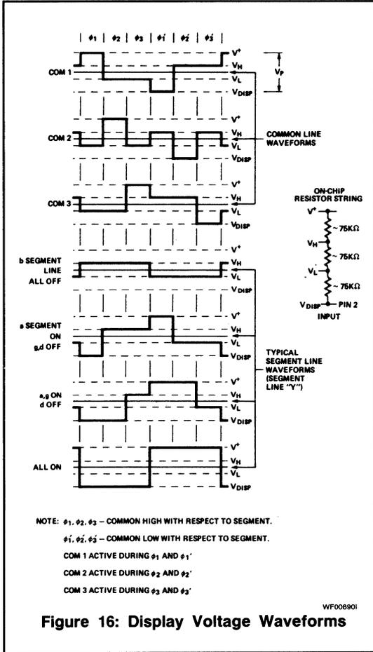
Figure 16: Display Voltage Waveforms
