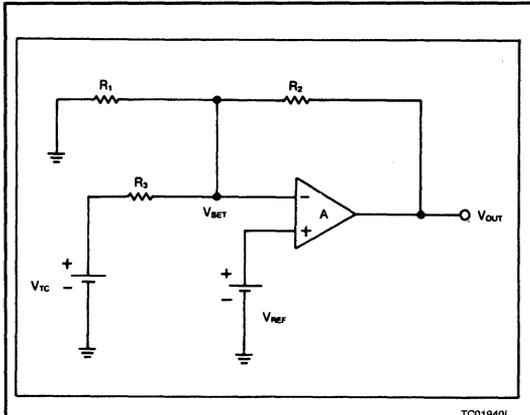
**Figure 2: The negative temperature coefficient required by a multiplexed liquid-crystal display is scaled by adjusting the  $V_{TC}$  output terminal of an ICL7663 positive-voltage regulator relative to the  $V_{SET}$  input.**
