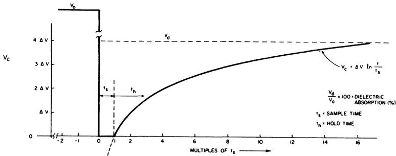
**Figure 2:** A natural log function of time is an accurate approximation to the voltage creep caused by dielectric absorption. Before sampling, the capacitor has been holding a voltage  $V_0$ . A new sample charges the capacitor to a new voltage (zero, in this case, for simplicity), for period  $t_s$ . Once in hold mode, the capacitor reaches a voltage  $\Delta V$  at time  $2t$ , and continues to creep toward  $V_0$  according to the logarithmic expression.
