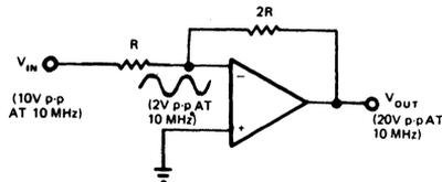
**Figure 3: The summing junction is NOT a virtual ground in high speed op-amp applications. Thus the amplifier must be designed with a large input dynamic range (IDR), or distortion, limiting or clipping will result.**
