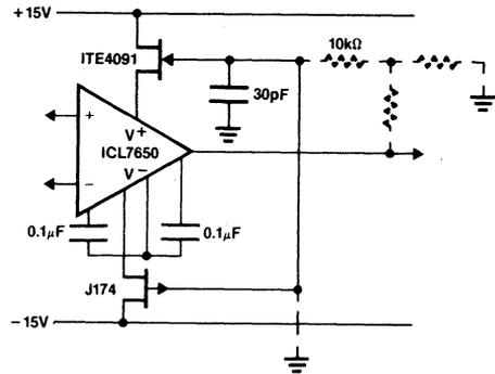
Figure 23: Operating with  $\pm 15V$  Supplies
