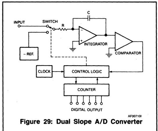
Figure 29: Dual Slope A/D Converter
