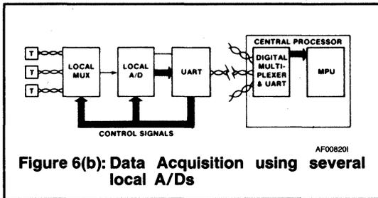
**Figure 6(b): Data Acquisition using several local A/Ds**
