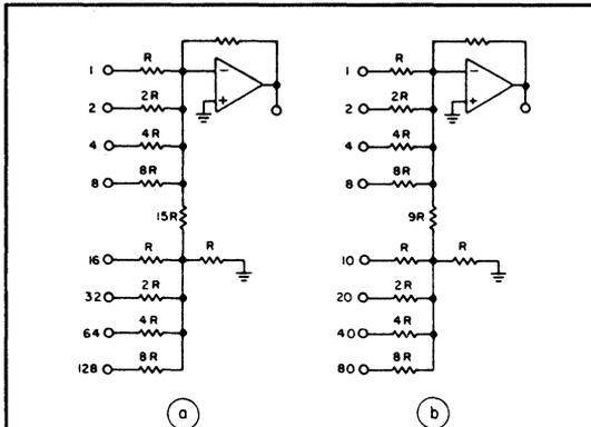
Figure 2: Binary (a) and BCD (b) ladder networks in D/A converters use the same weighting in the resistor quads but different divider ratios.
