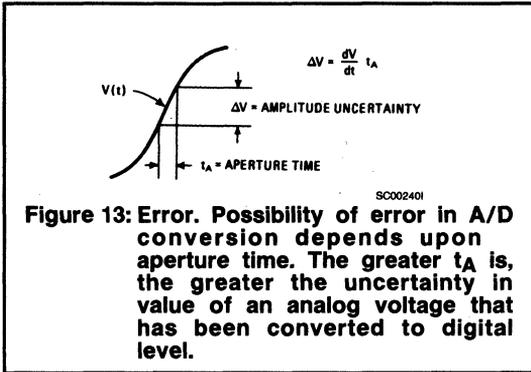
**Figure 13: Error. Possibility of error in A/D conversion depends upon aperture time. The greater  $t_A$  is, the greater the uncertainty in value of an analog voltage that has been converted to digital level.**
