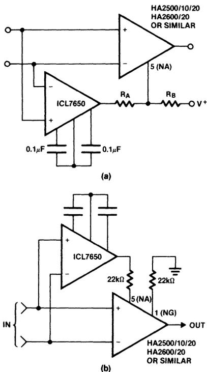
**Figure 26: HA2500 or 2600 Offset Nulled by ICL7650**
