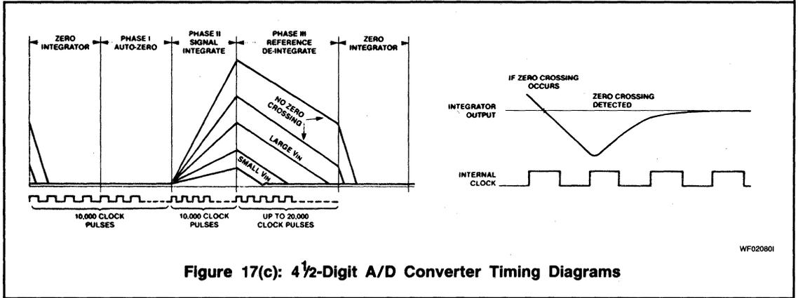
Figure 17(c): 4 1/2-Digit A/D Converter Timing Diagrams
