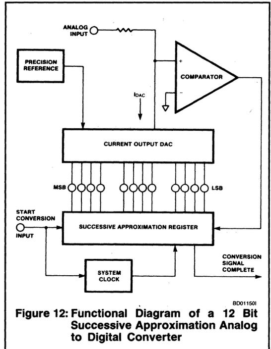
Figure 12: Functional Diagram of a 12 Bit Successive Approximation Analog to Digital Converter
