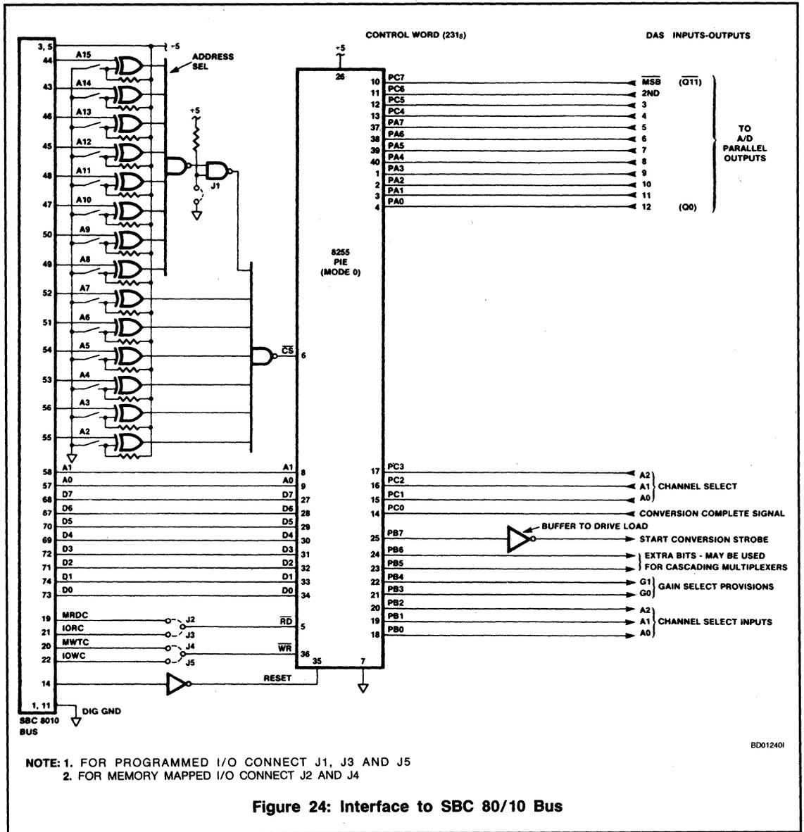
Figure 24: Interface to SBC 80/10 Bus
