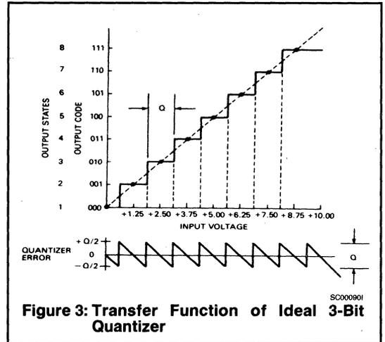
Figure 3: Transfer Function of Ideal 3-Bit Quantizer
