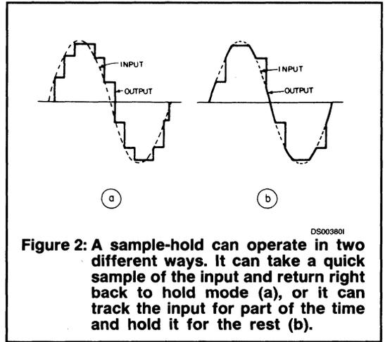
**Figure 2: A sample-hold can operate in two different ways. It can take a quick sample of the input and return right back to hold mode (a), or it can track the input for part of the time and hold it for the rest (b).**
