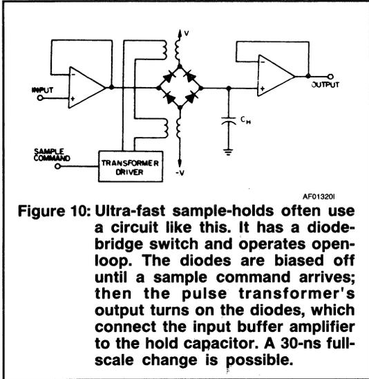
**Figure 10: Ultra-fast sample-holds often use a circuit like this. It has a diode-bridge switch and operates open-loop. The diodes are biased off until a sample command arrives; then the pulse transformer's output turns on the diodes, which connect the input buffer amplifier to the hold capacitor. A 30-ns full-scale change is possible.**
