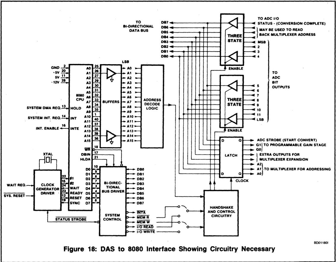
Figure 18: DAS to 8080 Interface Showing Circuitry Necessary
