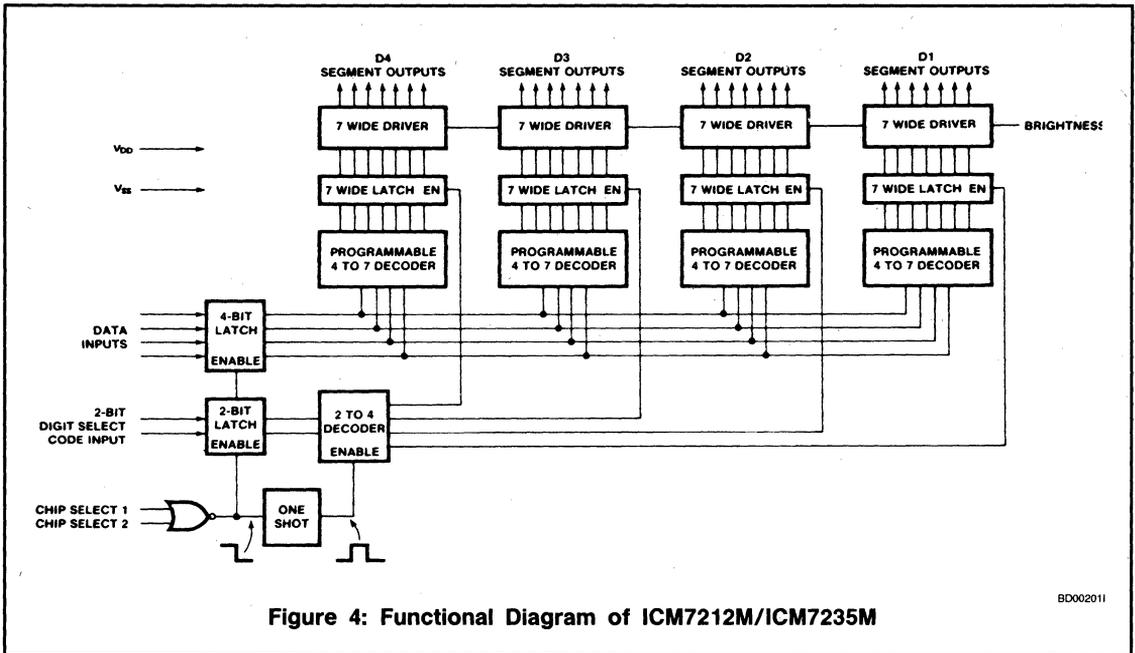
Figure 4: Functional Diagram of ICM7212M/ICM7235M
