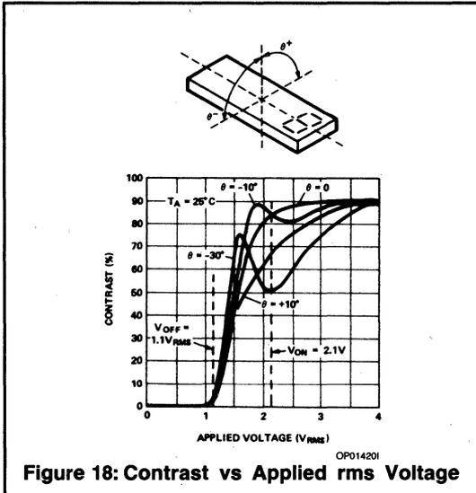
Figure 18: Contrast vs Applied rms Voltage
