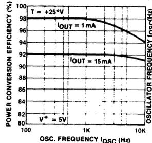
Figure 10: Efficiency Change with Oscillator Frequency
