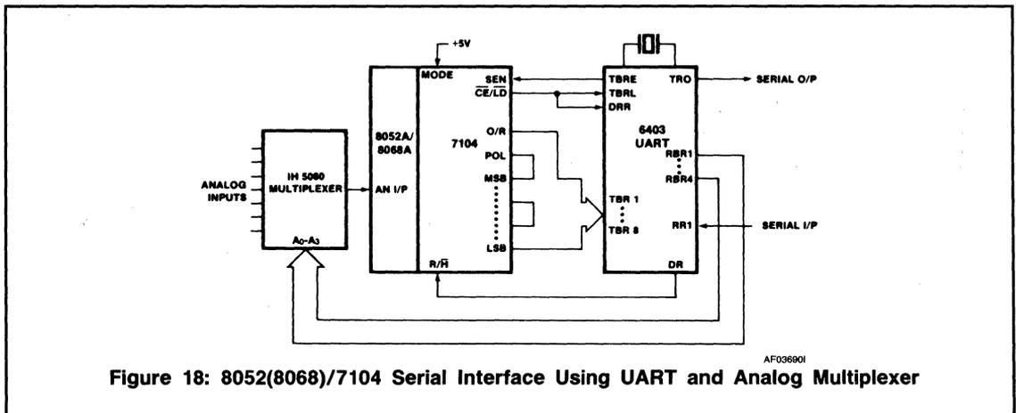
Figure 18: 8052(8068)/7104 Serial Interface Using UART and Analog Multiplexer
