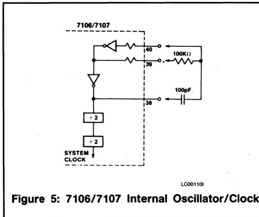
Figure 5: 7106/7107 Internal Oscillator/Clock
