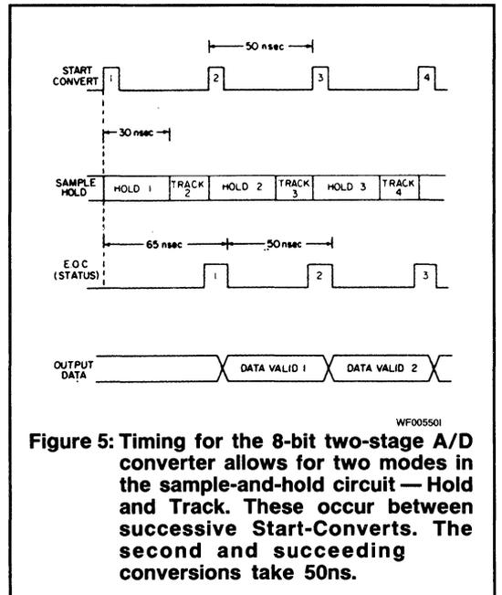
Figure 5: Timing for the 8-bit two-stage A/D converter allows for two modes in the sample-and-hold circuit — Hold and Track. These occur between successive Start-Converts. The second and succeeding conversions take 50ns.
