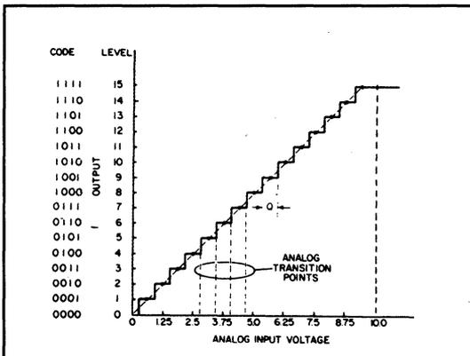
**Figure 2: The quantizer transfer function for a 4-bit parallel-type converter shows how the analog input is broken into 16 different levels. Each word of digitally coded output signals represents a range, Q, of input voltage.**
