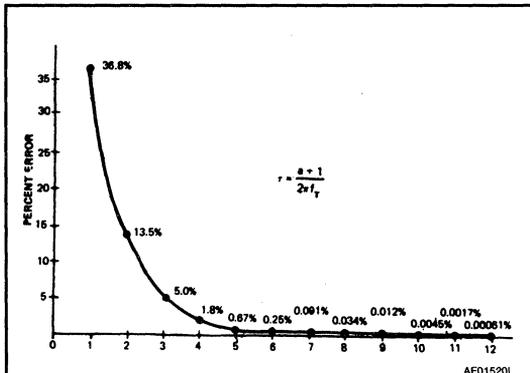
**Figure 9:** Output error decreases predictably as a function of the number of time constants when the op-amp circuit exhibits a single-pole response.
