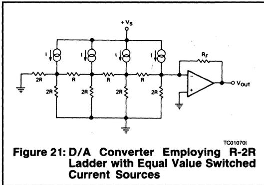
**Figure 21: D/A Converter Employing R-2R Ladder with Equal Value Switched Current Sources**
