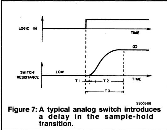
**Figure 7: A typical analog switch introduces a delay in the sample-hold transition.**
