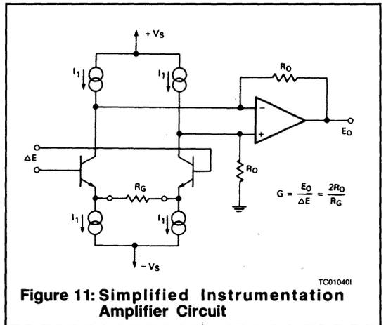
Figure 11: Simplified Instrumentation Amplifier Circuit
