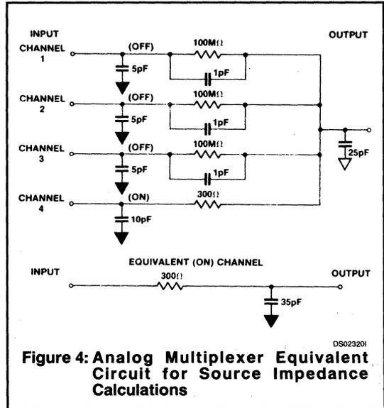
Figure 4: Analog Multiplexer Equivalent Circuit for Source Impedance Calculations
