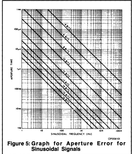
**Figure 5: Graph for Aperture Error for Sinusoidal Signals**
