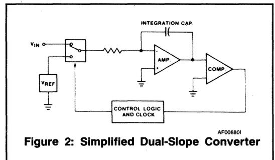
**Figure 2: Simplified Dual-Slope Converter**
