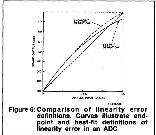
**Figure 6: Comparison of linearity error definitions. Curves illustrate end-point and best-fit definitions of linearity error in an ADC**
