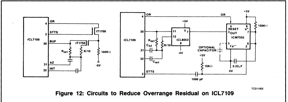
Figure 12: Circuits to Reduce Overage Residual on ICL7109
