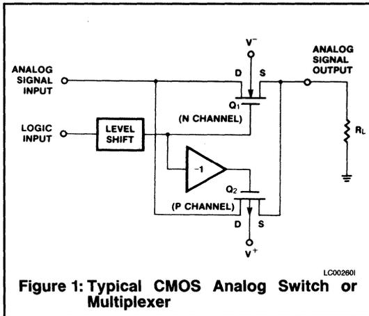
Figure 1: Typical CMOS Analog Switch or Multiplexer
