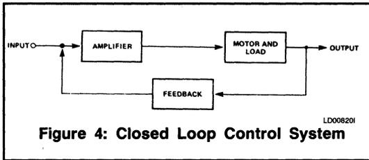
Figure 4: Closed Loop Control System
