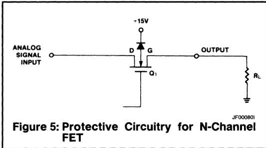
**Figure 5: Protective Circuitry for N-Channel FET**
