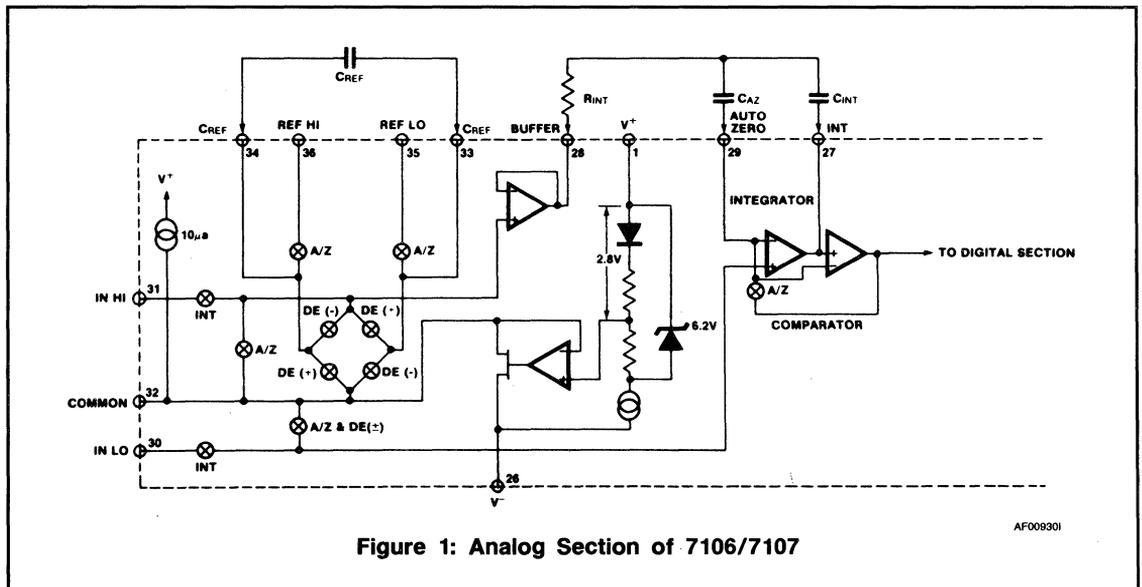
Figure 1: Analog Section of 7106/7107
