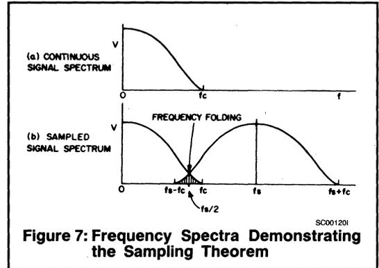
Figure 7: Frequency Spectra Demonstrating the Sampling Theorem
