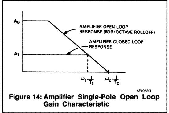
Figure 14: Amplifier Single-Pole Open Loop Gain Characteristic
