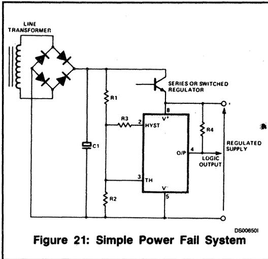
Figure 21: Simple Power Fail System
