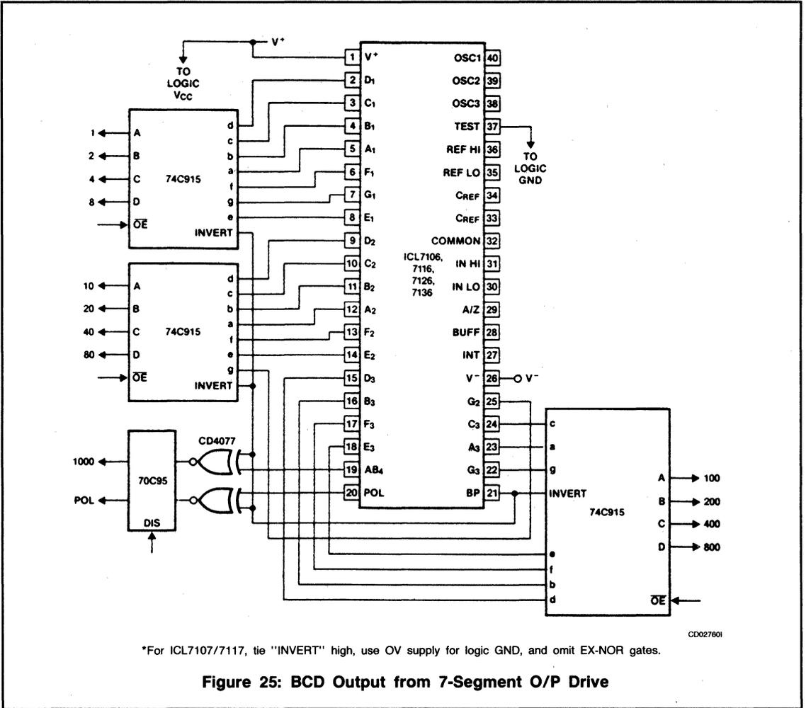
\*For ICL7107/7117, tie "INVERT" high, use OV supply for logic GND, and omit EX-NOR gates.
