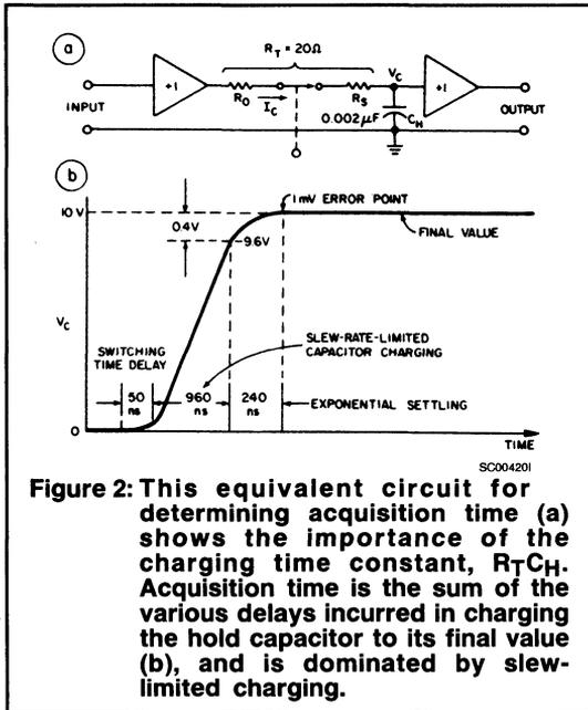
**Figure 2: This equivalent circuit for determining acquisition time (a) shows the importance of the charging time constant,  $R_T C_H$ . Acquisition time is the sum of the various delays incurred in charging the hold capacitor to its final value (b), and is dominated by slew-limited charging.**
