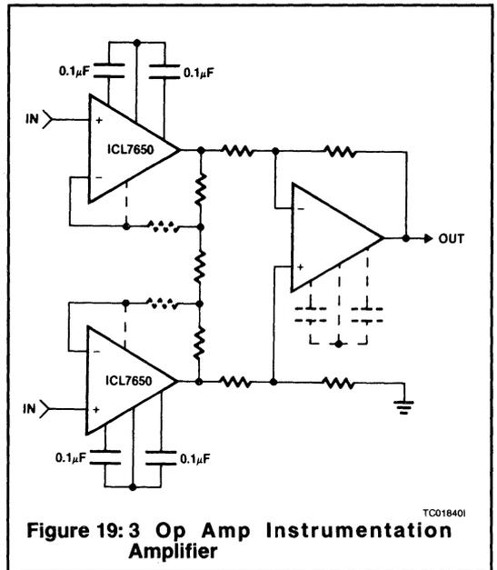
Figure 19: 3 Op Amp Instrumentation Amplifier
