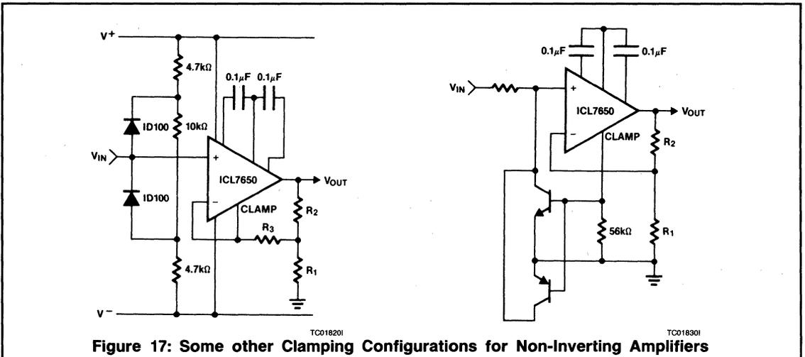
**Figure 17: Some other Clamping Configurations for Non-Inverting Amplifiers**
