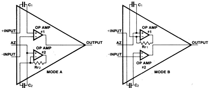
Figure 7: ICL7600/ICL7601 Commutating Auto-Zero (CAZ) Operational Amplifier Showing Two-Cycle Operation
