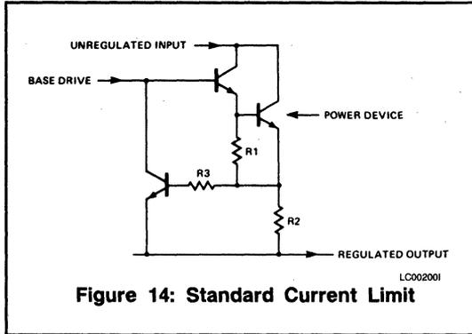
**Figure 14: Standard Current Limit**
