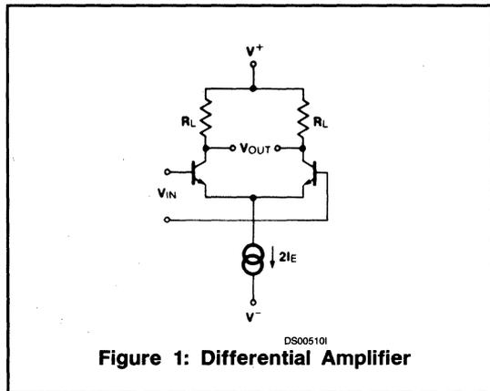
The small differential voltage gain on this circuit is given by
