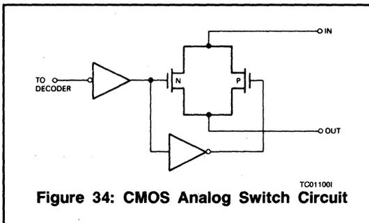
**Figure 34: CMOS Analog Switch Circuit**
