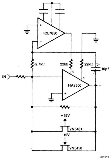
**Figure 27: Nulled HA2500 with Dynamic Correction and Overload Clamp**
