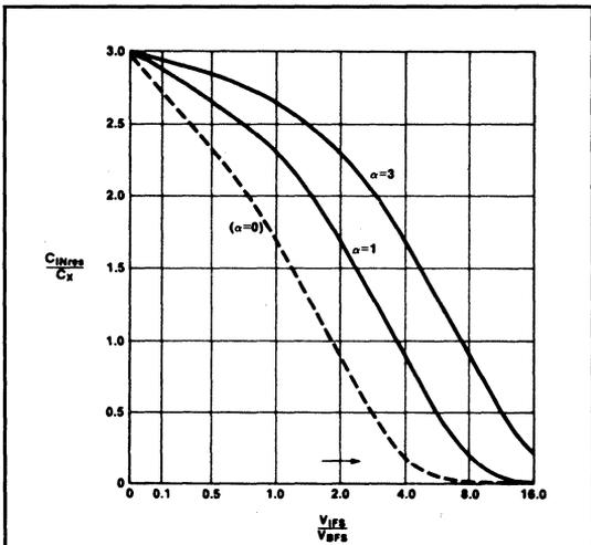
**Figure 10: Auto-Zero Loop Residual vs. Integrator/Buffer Swing and Capacitor Ratios (worst case)**
