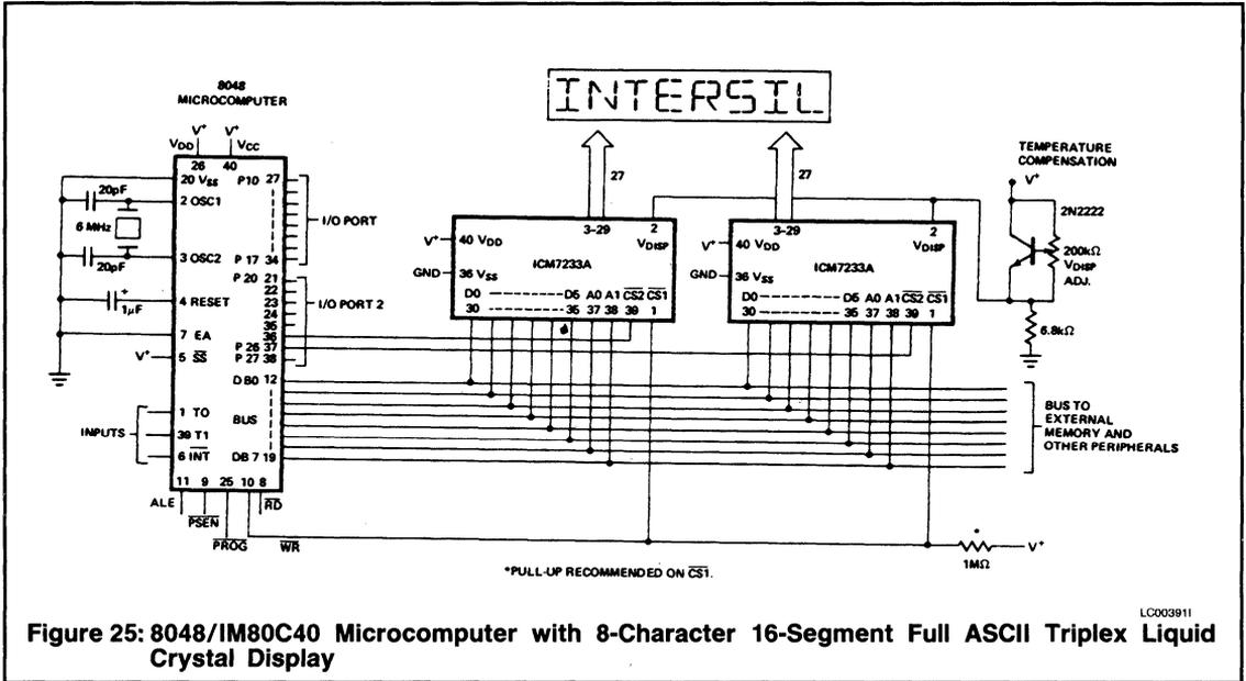
Figure 25: 8048/IM80C40 Microcomputer with 8-Character 16-Segment Full ASCII Triplex Liquid Crystal Display
