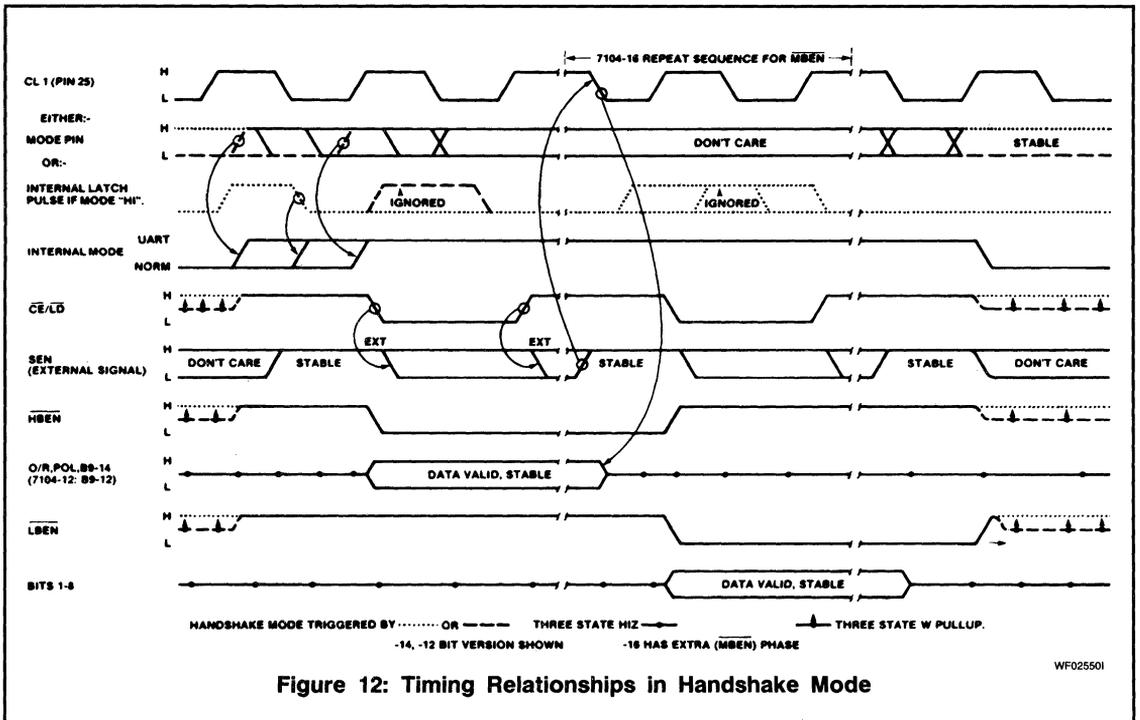
Figure 12: Timing Relationships in Handshake Mode
