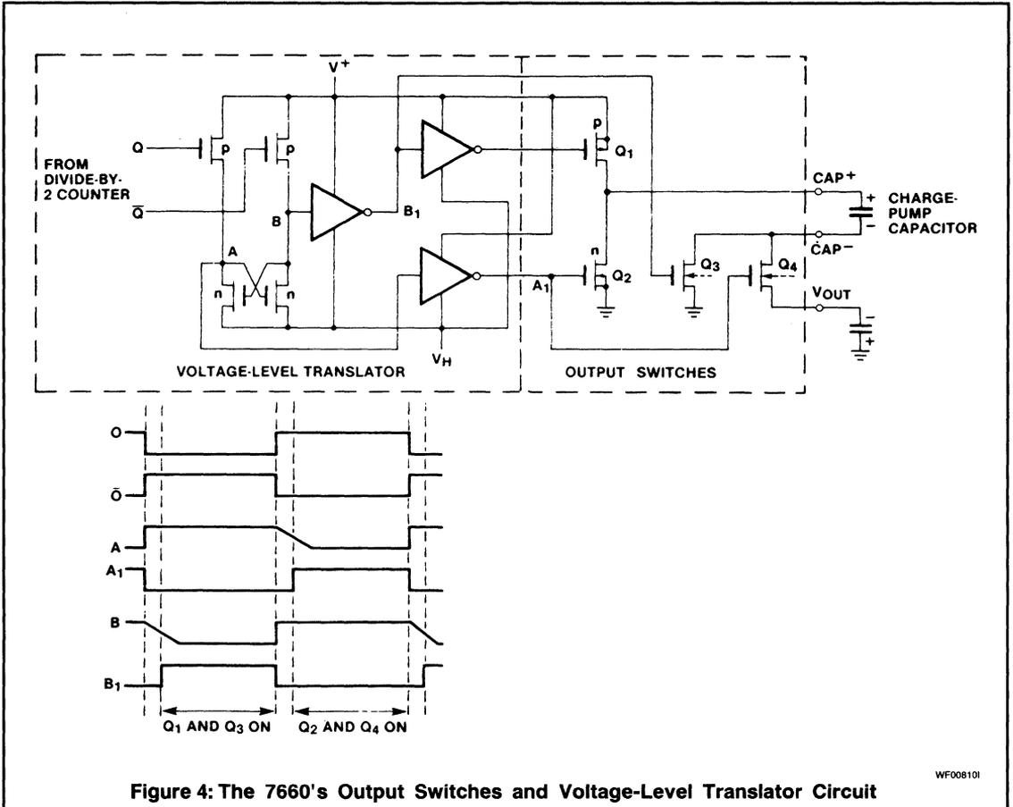
**Figure 4: The 7660's Output Switches and Voltage-Level Translator Circuit**
