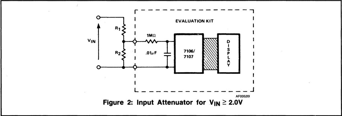
Figure 2: Input Attenuator for  $V_{IN} \geq 2.0V$
