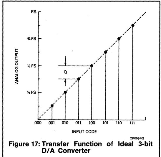
**Figure 17: Transfer Function of Ideal 3-bit D/A Converter**
