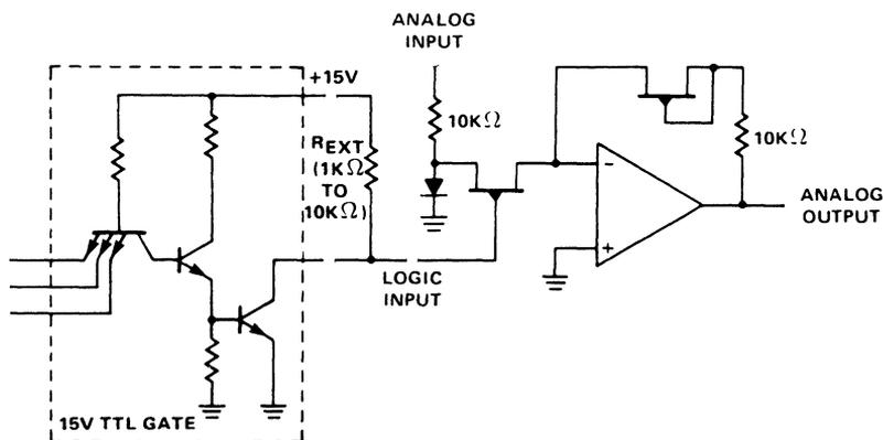
Figure 5: Interfacing With +15V Open Collector Logic
