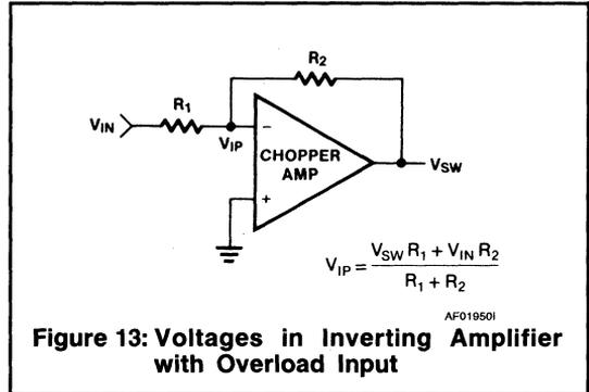
**Figure 13: Voltages in Inverting Amplifier with Overload Input**
