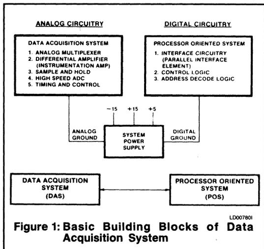
Figure 1: Basic Building Blocks of Data Acquisition System
