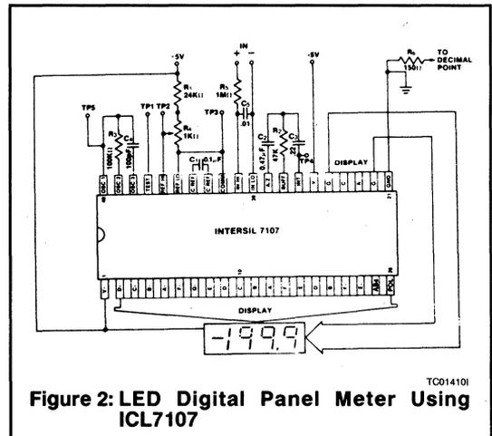
Figure 2: LED Digital Panel Meter Using ICL7107
