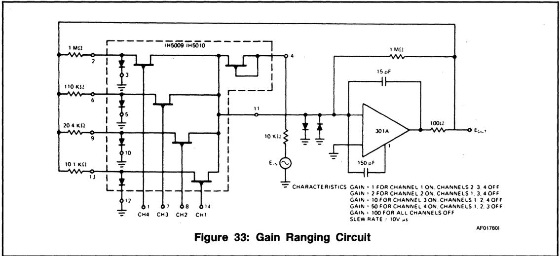
Figure 33: Gain Ranging Circuit
