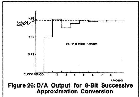
Figure 26: D/A Output for 8-Bit Successive Approximation Conversion
