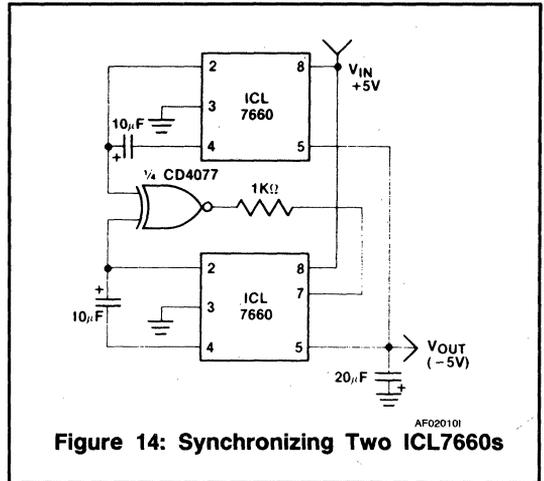
Figure 14: Synchronizing Two ICL7660s
