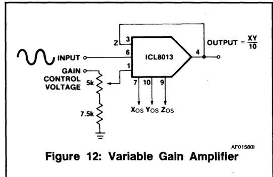
Figure 12: Variable Gain Amplifier
