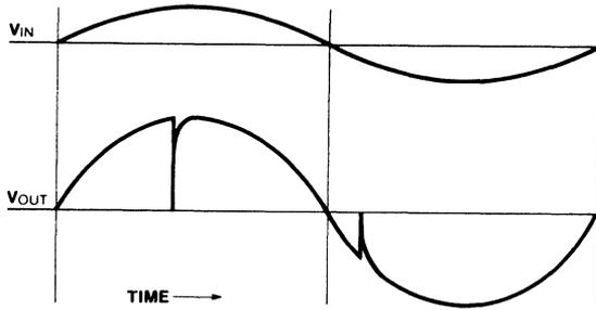
Figure 8: Output Spikes Due to Commutating Operation
