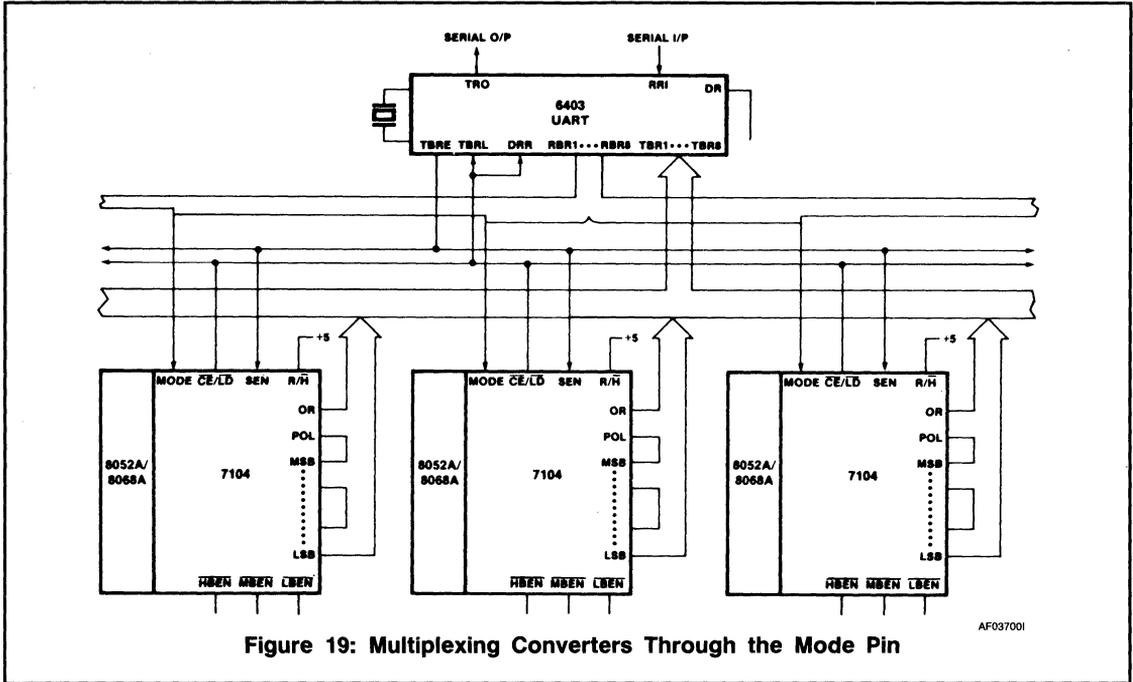
Figure 19: Multiplexing Converters Through the Mode Pin
