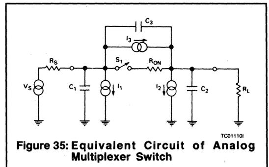
**Figure 35: Equivalent Circuit of Analog Multiplexer Switch**
