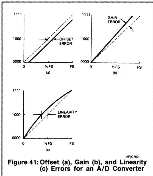
Figure 41: Offset (a), Gain (b), and Linearity (c) Errors for an A/D Converter
