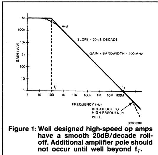
Figure 1: Well designed high-speed op amps have a smooth 20dB/decade roll-off. Additional amplifier pole does not occur until well beyond  $f_T$ .
