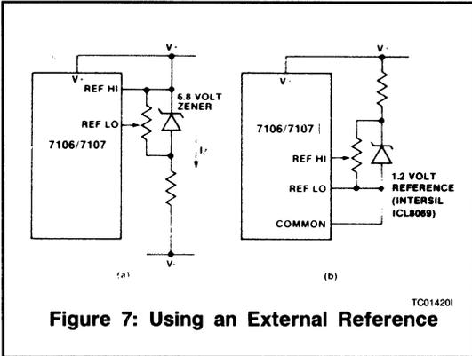
Figure 7: Using an External Reference
