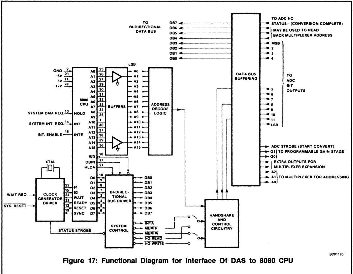
Figure 17: Functional Diagram for Interface Of DAS to 8080 CPU
