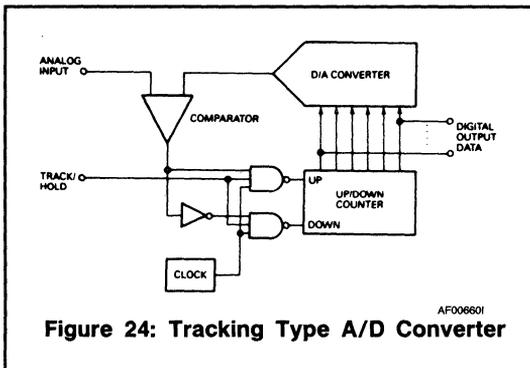
Figure 24: Tracking Type A/D Converter
