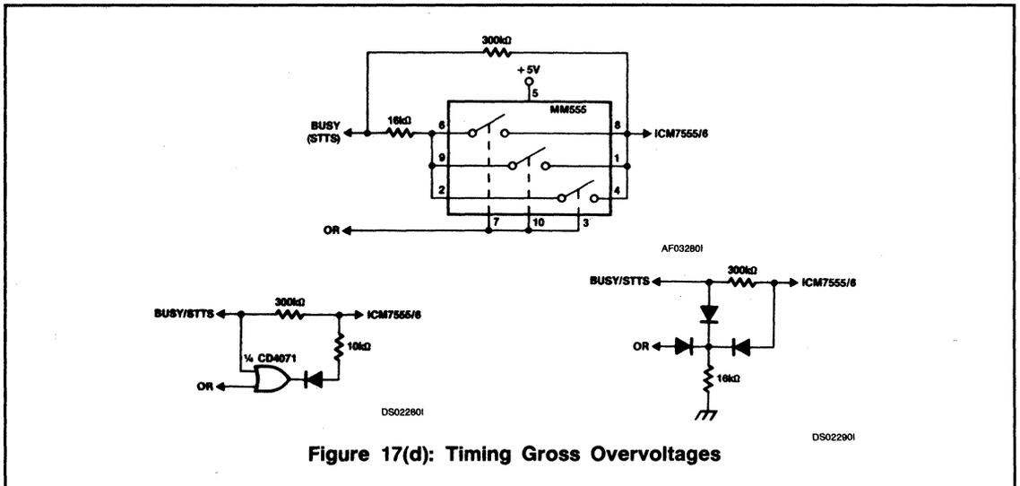
Figure 17(d): Timing Gross Overvoltages
