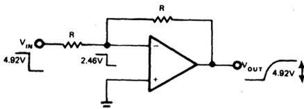
**Figure 4: Staying within an amplifier's IDR avoids slew-rate limitation problems and produces a smooth output response.**
