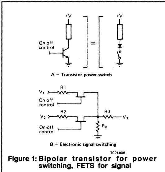
**Figure 1: Bipolar transistor for power switching, FETS for signal**
