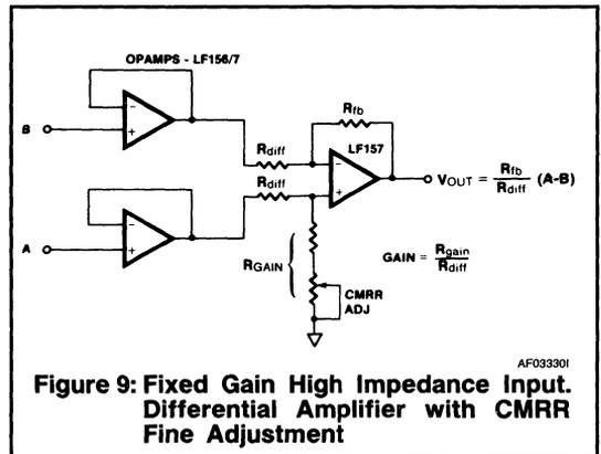
**Figure 9: Fixed Gain High Impedance Input. Differential Amplifier with CMRR Fine Adjustment**
