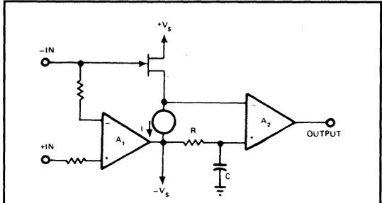
**Figure 6: Fast-feedforward amplifier design combines a low-drift bipolar IC op amp with an FET feedforward stage to produce excellent dc and ac characteristics.**
