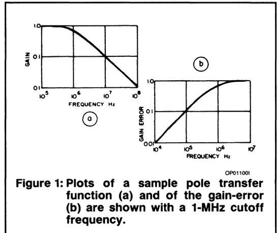
Figure 1: Plots of a sample pole transfer function (a) and of the gain-error (b) are shown with a 1-MHz cutoff frequency.
