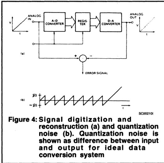
**Figure 4: Signal digitization and reconstruction (a) and quantization noise (b). Quantization noise is shown as difference between input and output for ideal data conversion system**
