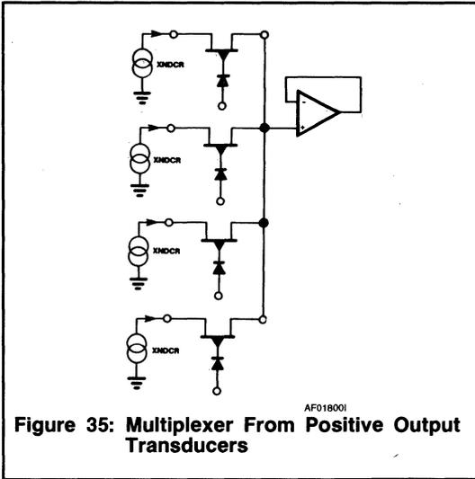
**Figure 35: Multiplexer From Positive Output Transducers**
