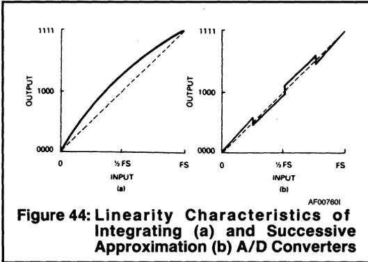
**Figure 44: Linearity Characteristics of Integrating (a) and Successive Approximation (b) A/D Converters**
