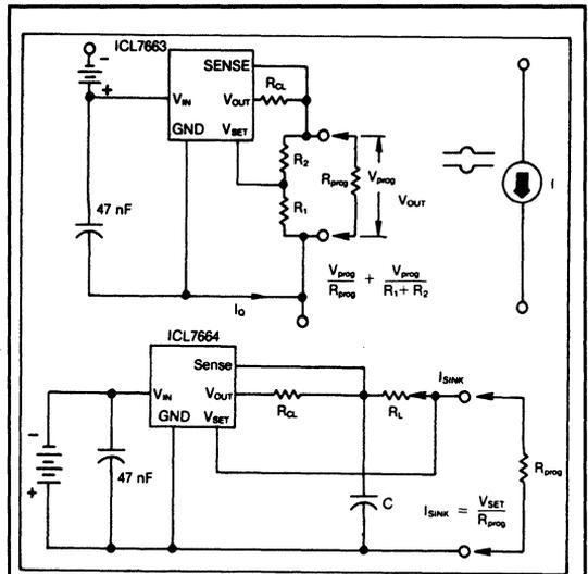
**Figure 3: With the proper regulator and polarities, the two-terminal current source (top), and the precision current sink (bottom) can serve as either sink or source. In either capacity, however, the bottom circuit can be set more accurately for small currents.**
