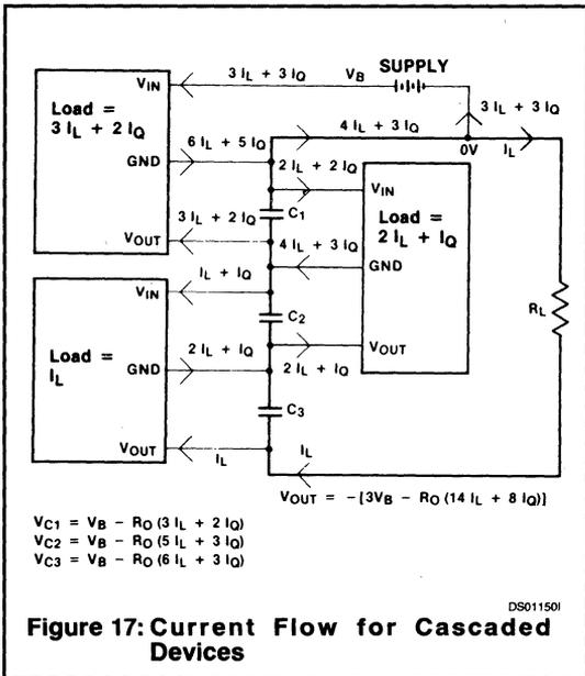
Thus the load current is rapidly multiplied down the chain, as shown in Figure 17. Note also that the quiescent current increases the load current on each stage, though not as fast as the ultimate load itself.
