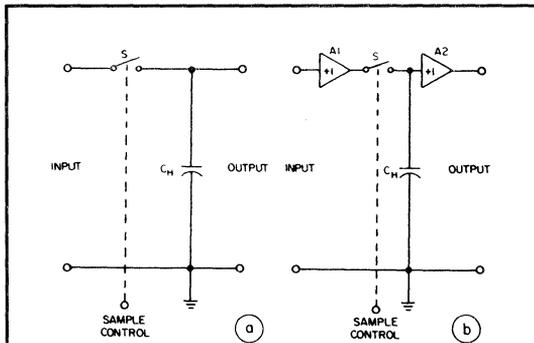
**Figure 1: In a basic sample-hold circuit (a), the switch closes to sample the input voltage. When the switch opens, the capacitor holds the voltage. A practical circuit (b) has unity-gain buffers to charge the capacitor without loading the source and to drive normal loads without changing the voltage stored by the capacitor.**
