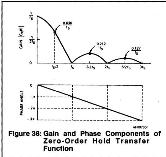
As with other filter circuits, the gain and phase components of the transfer function are of interest. By an analysis based on the impulse response of a sample-and-hold and use of the Laplace transform, the transfer function is found to be
