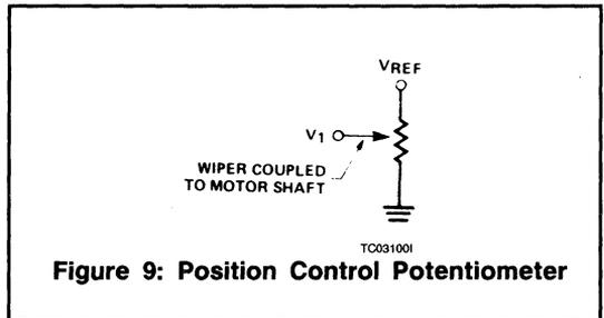
**Figure 9: Position Control Potentiometer**
