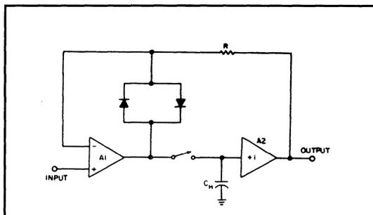
**Figure 7:** Closed-loop sample-holds can also be noninverting. In this configuration,  $A_1$  is both an input buffer and an error-correcting amplifier. When the switch closes, current from  $A_1$  charges the hold capacitor until the output equals the input. The pair of diodes clamps  $A_1$ 's output to keep it stable when the switch is open.
