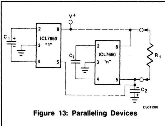
Figure 13: Paralleling Devices
