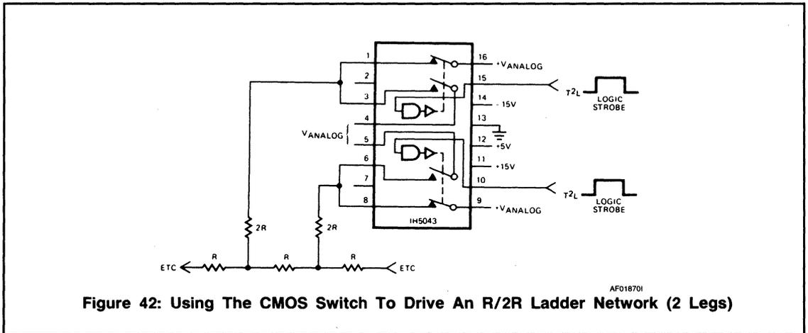
**Figure 42: Using The CMOS Switch To Drive An R/2R Ladder Network (2 Legs)**
