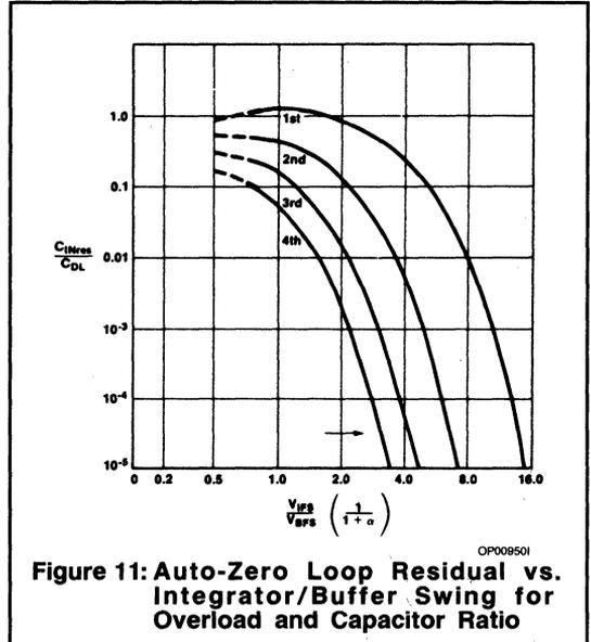
**Figure 11: Auto-Zero Loop Residual vs. Integrator/Buffer Swing for Overload and Capacitor Ratio**
