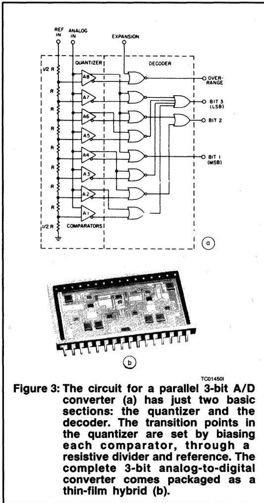
**Figure 3: The circuit for a parallel 3-bit A/D converter (a) has just two basic sections: the quantizer and the decoder. The transition points in the quantizer are set by biasing each comparator, through a resistive divider and reference. The complete 3-bit analog-to-digital converter comes packaged as a thin-film hybrid (b).**
