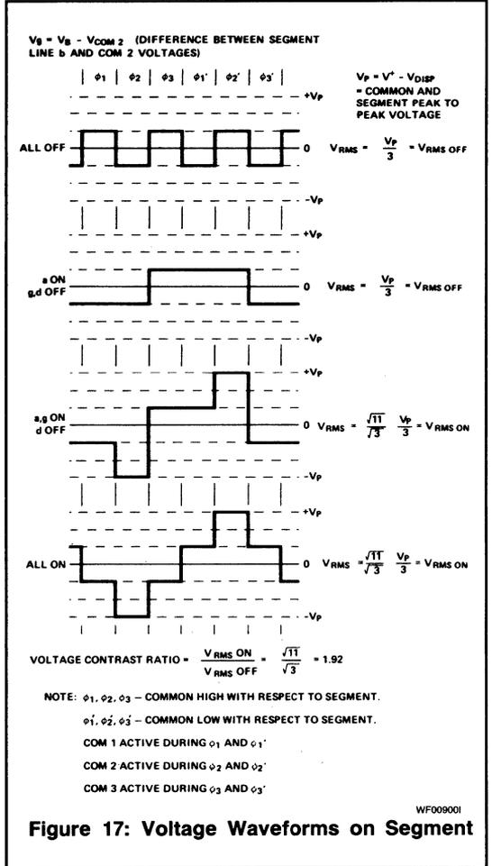
Figure 17: Voltage Waveforms on Segment
