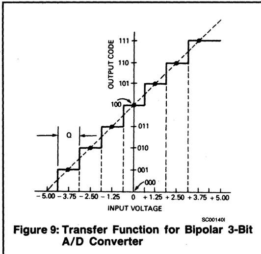
**Figure 9: Transfer Function for Bipolar 3-bit A/D Converter**
