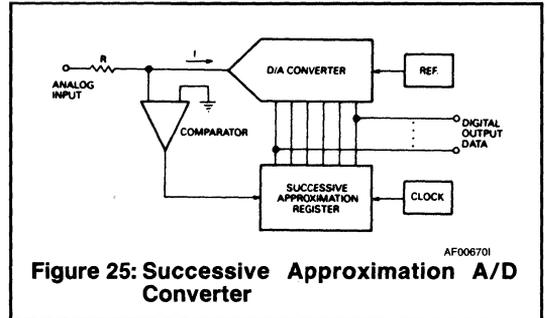
Figure 25: Successive Approximation A/D Converter
