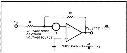
**Figure 7: Noise gain and signal gain differ. In an inverting circuit the noise gain equals the signal gain plus one.**
