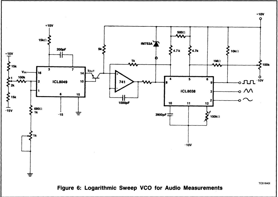
Figure 6: Logarithmic Sweep VCO for Audio Measurements
