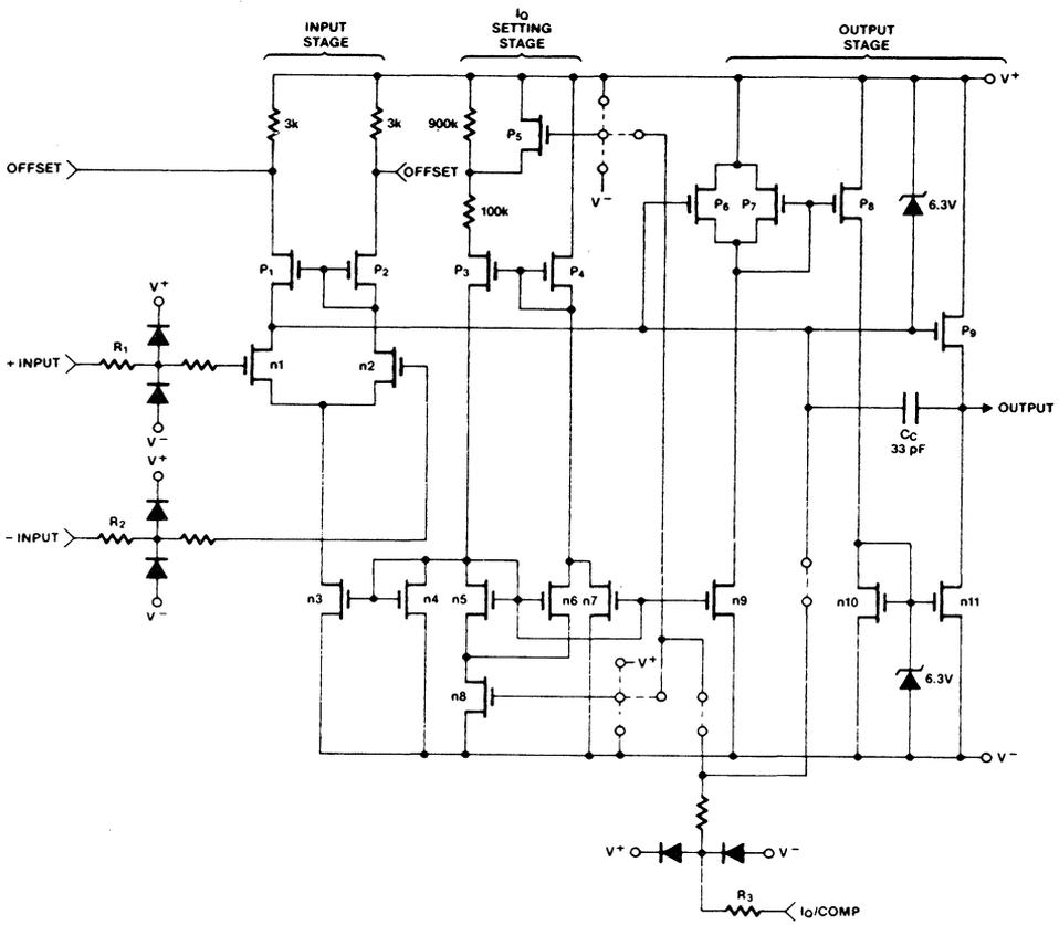
Figure 4: CMOS Op Amp Schematic (ICL7611 Family)
