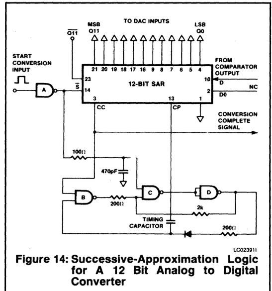
Figure 14: Successive-Approximation Logic for A 12 Bit Analog to Digital Converter
