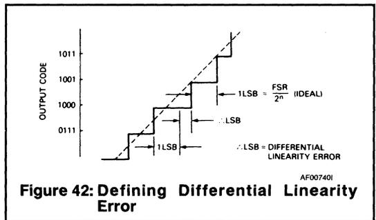
Figure 42: Defining Differential Linearity Error
