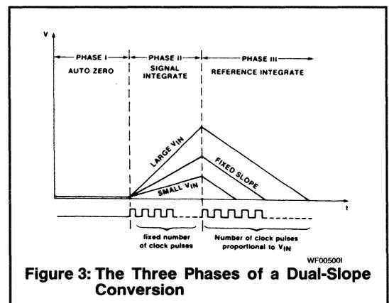
**Figure 3: The Three Phases of a Dual-Slope Conversion**
