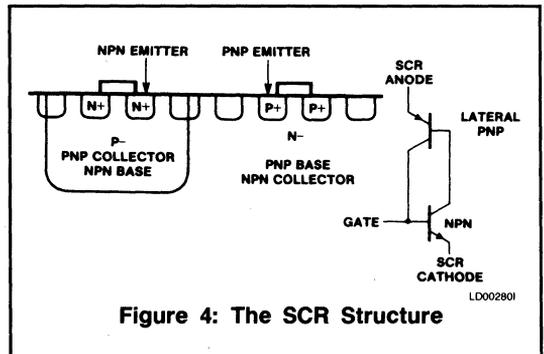
Figure 4: The SCR Structure
