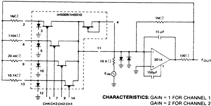
**CHARACTERISTICS:** GAIN = 1 FOR CHANNEL 1 ON; CHANNELS 2, 3, 4 OFF
