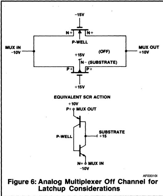
The best way to eliminate this problem is to select a device which has no latchup problems. See Intersil Application Bulletin A006 for a description of some latchup proof analog multiplexers and switches.
