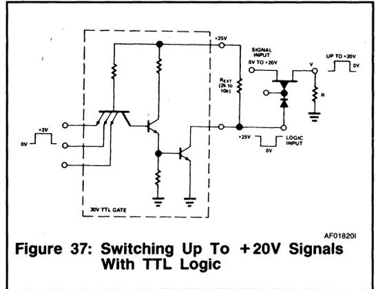
**Figure 37: Switching Up To +20V Signals With TTL Logic**
