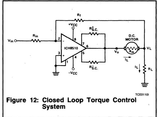
Figure 12: Closed Loop Torque Control System
