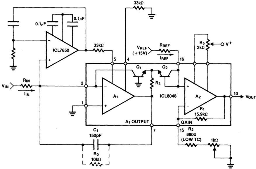
Figure 22: ICL8048 Offset Nulled by ICL7650
