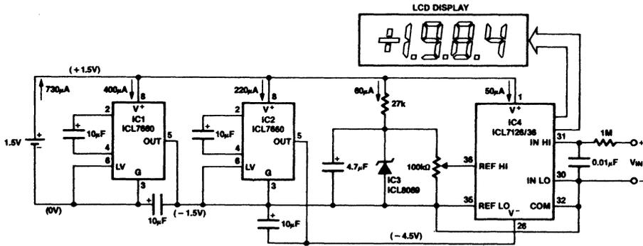
Figure 13: Using ICL7660 to Run ICL7126/36 from 1.5V Battery
