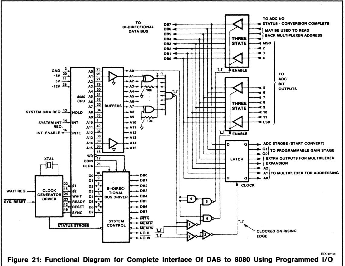
Figure 21: Functional Diagram for Complete Interface Of DAS to 8080 Using Programmed I/O BD012101
