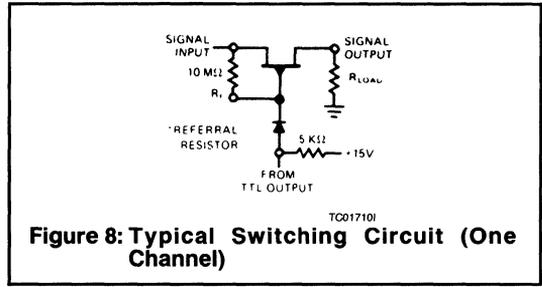
**Figure 8: Typical Switching Circuit (One Channel)**
