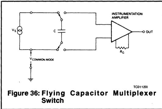
**Figure 36: Flying Capacitor Multiplexer Switch**
