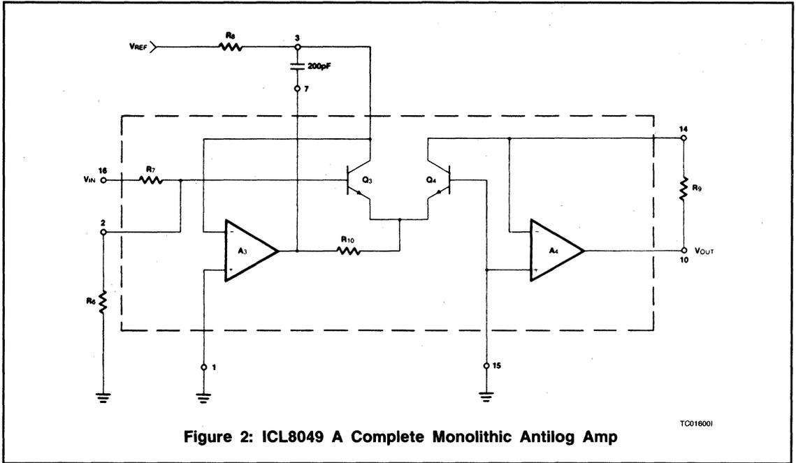
Figure 2: ICL8049 A Complete Monolithic Antilog Amp
