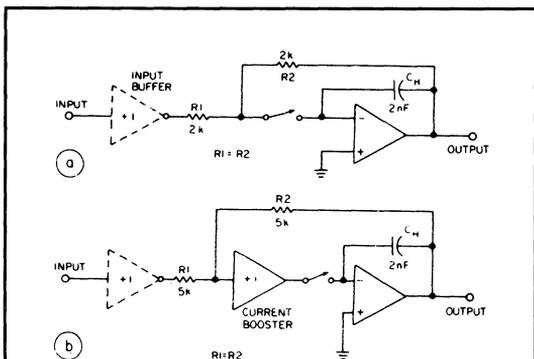
**Figure 6:** This type of inverting, closed-loop circuit is both accurate and simple. The charge time constant,  $R_2C_H$ , of the basic circuit (a) is much too long for some applications. The current booster in (b) speeds up charging considerably. The input resistance,  $R_1$ , may be too low for some sources; the buffer raises it a great deal.
