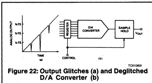
**Figure 22: Output Glitches (a) and Deglitched D/A Converter (b)**
