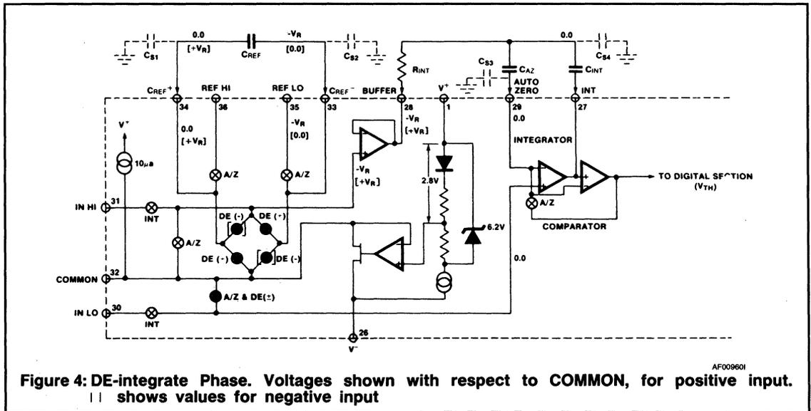
**Figure 4: DE-integrate Phase. Voltages shown with respect to COMMON, for positive input. | | shows values for negative input**
