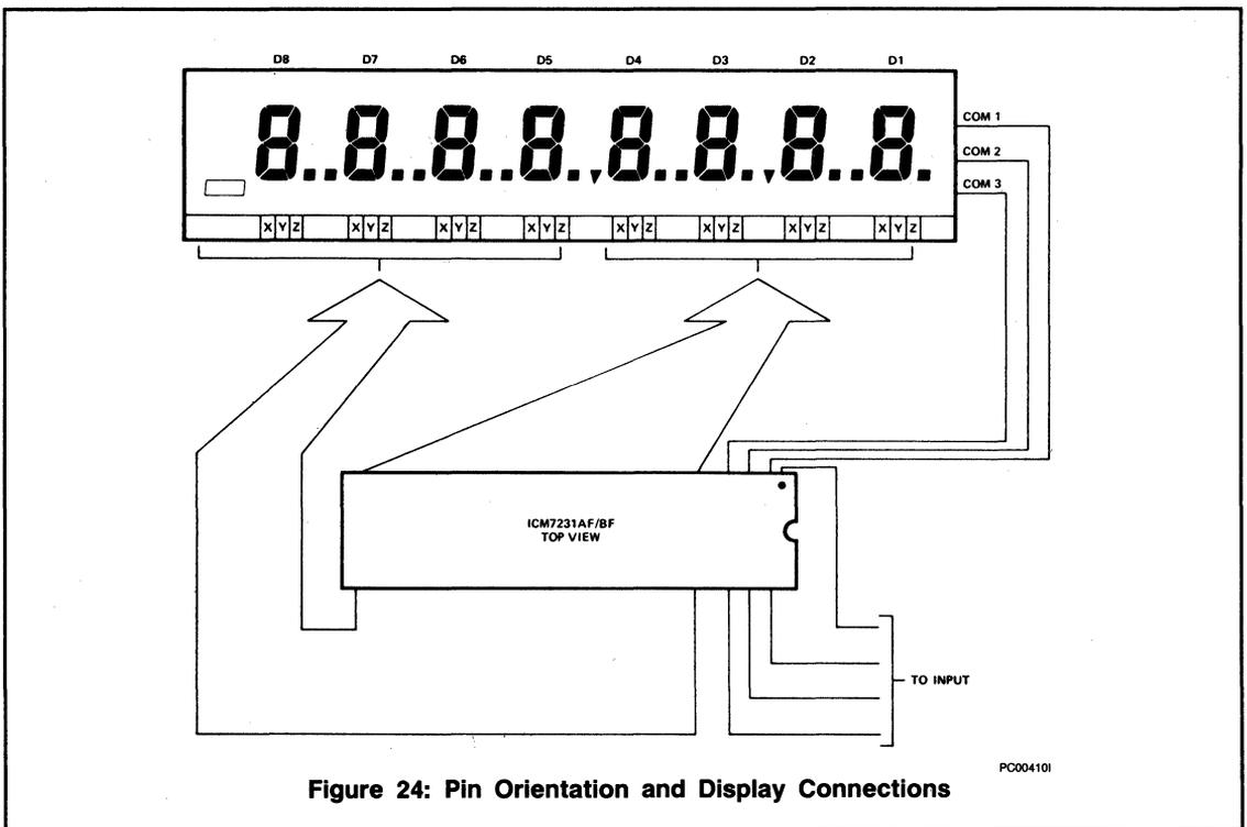
Figure 24: Pin Orientation and Display Connections
