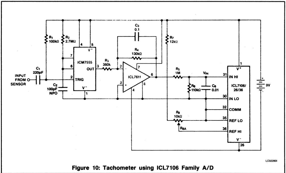
**Figure 10: Tachometer using ICL7106 Family A/D**
