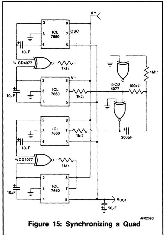
Figure 15: Synchronizing a Quad
