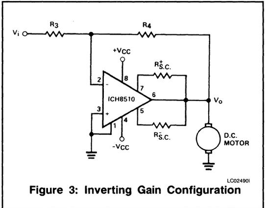
Figure 3: Inverting Gain Configuration
