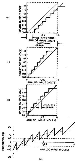
**Figure 5: Errors in nonideal A/D converters. Transfer functions are shown for ADCs with offset error (a), gain error (b), and linearity error (c). ADC with all three errors present will have quantization error as shown in (d)**
