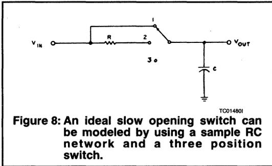
**Figure 8: An ideal slow opening switch can be modeled by using a sample RC network and a three position switch.**
