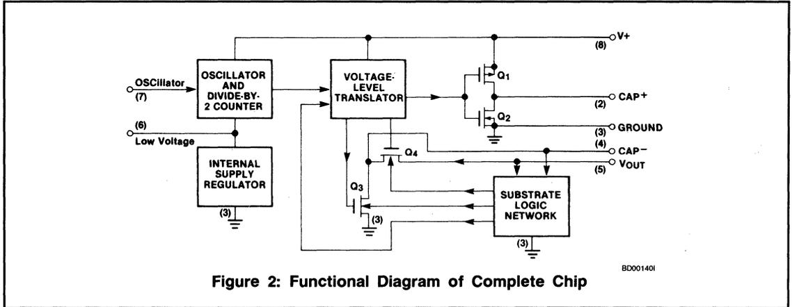
**Figure 2: Functional Diagram of Complete Chip**
