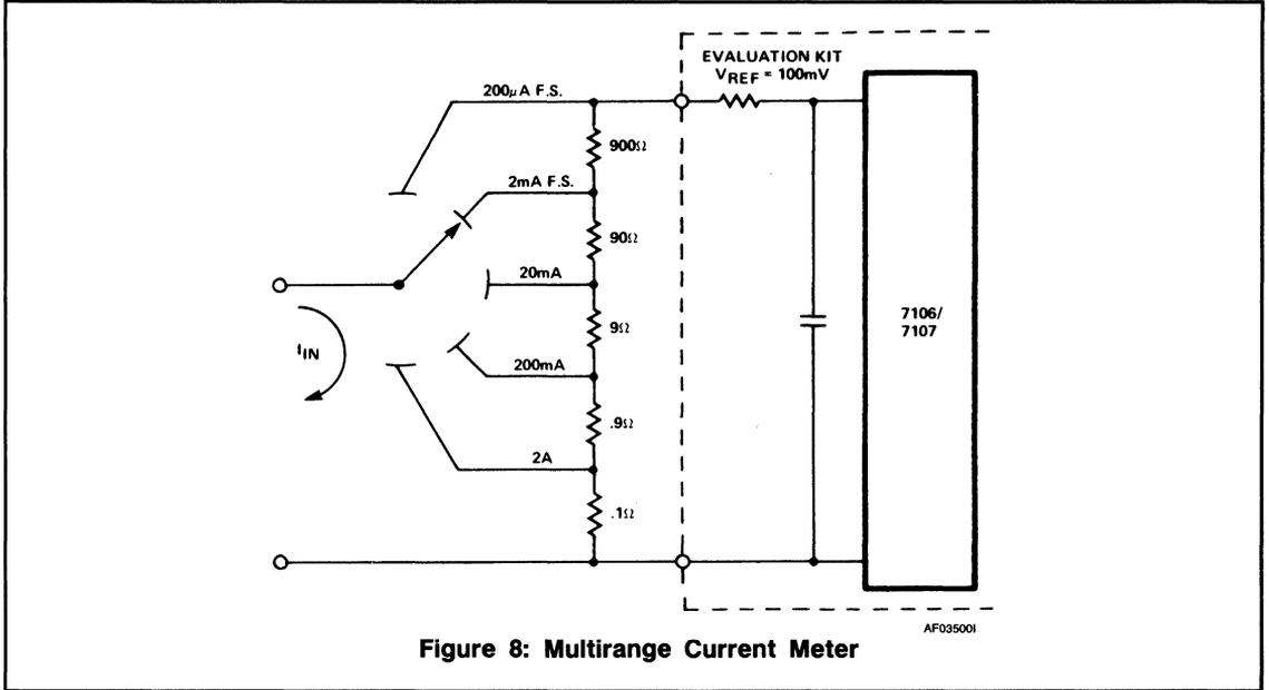
Figure 8: Multirange Current Meter
