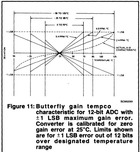
With a 12-bit ADC for example,  $1/2$  LSB is equal to 120ppm. If the operating temperature range is 0 to 70°C and the converter is calibrated at 25°C, the maximum temperature change is 70°C - 25°C, or 45°C. To guarantee
