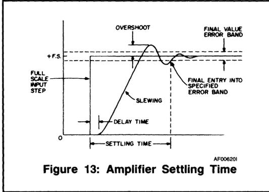
Figure 13: Amplifier Settling Time
