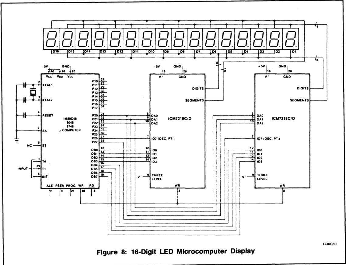
Figure 8: 16-Digit LED Microcomputer Display
