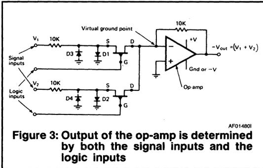
**Figure 3: Output of the op-amp is determined by both the signal inputs and the logic inputs**
