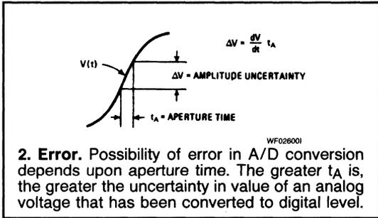
The two graphs are derived with reference to Fig. 2, which shows a time-varying signal and the amplitude uncertainty  $\Delta V$  associated with an aperture time  $t_A$
