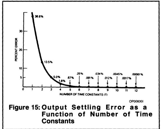
Figure 15: Output Settling Error as a Function of Number of Time Constants
