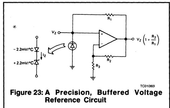
**Figure 23: A Precision, Buffered Voltage Reference Circuit**
