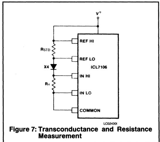
For transconductance measurement, merely switch  $R_{STD}$  and  $R_X$ . This scheme makes the measurement of large resistors, in conductance form, convenient and easy. This is also convenient for leakage measurements.
