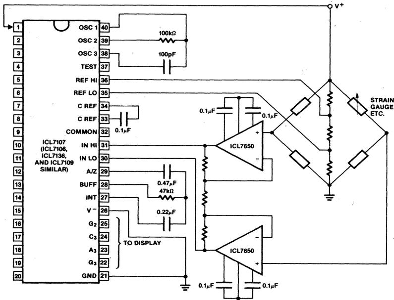
Figure 20: 2 Op Amp Differential Preamp for ICL7106/7/9 Families
