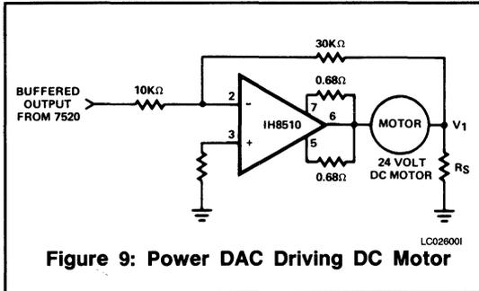
**Figure 9: Power DAC Driving DC Motor**
