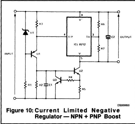
**Figure 10: Current Limited Negative Regulator — NPN + PNP Boost**
