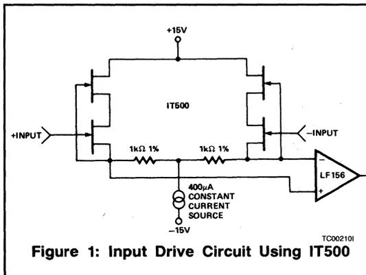
Figure 1: Input Drive Circuit Using IT500
