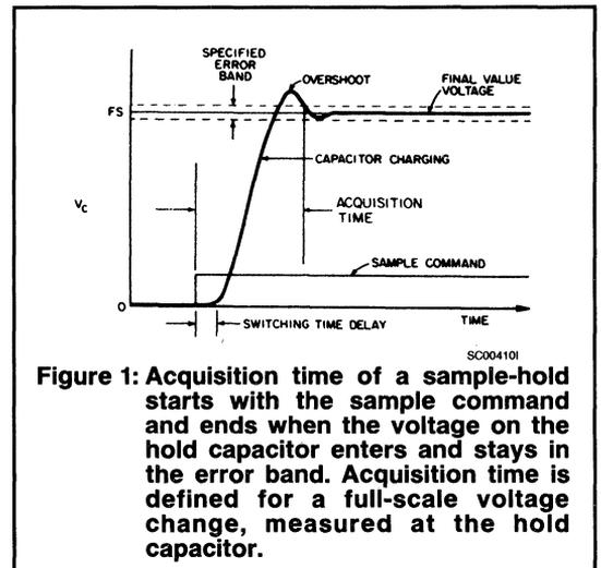
**Figure 1: Acquisition time of a sample-hold starts with the sample command and ends when the voltage on the hold capacitor enters and stays in the error band. Acquisition time is defined for a full-scale voltage change, measured at the hold capacitor.**
