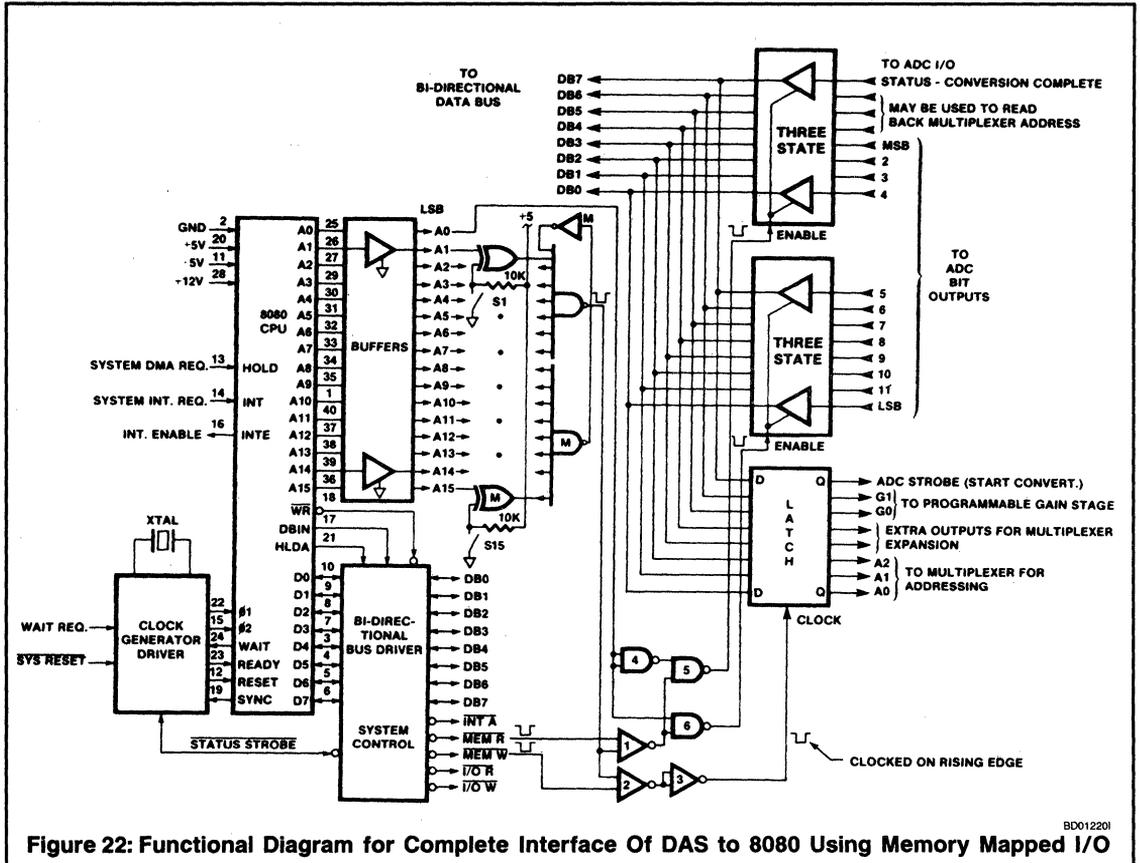
Figure 22: Functional Diagram for Complete Interface Of DAS to 8080 Using Memory Mapped I/O
