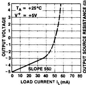
Figure 7: Output Characteristics
