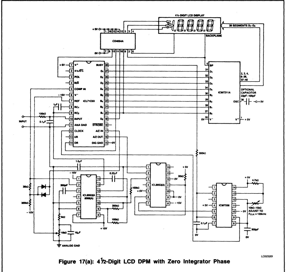
Figure 17(a): 4 1/2-Digit LCD DPM with Zero Integrator Phase
