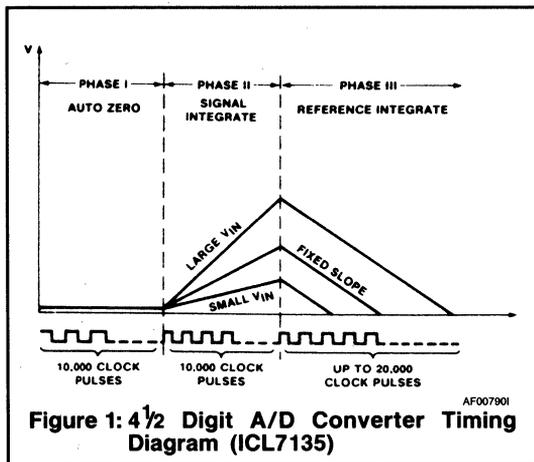
These timing characteristics give the dual slope circuit both its strengths and its weaknesses. By making the signal integrate period an integral number of line frequency periods, excellent 60Hz noise rejection can be obtained. And of course integrating the input signal for several milliseconds smoothes out the effect of high frequency noise.
