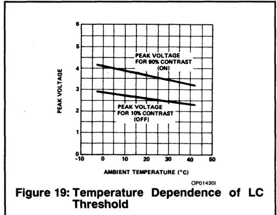
Figure 19: Temperature Dependence of LC Threshold
