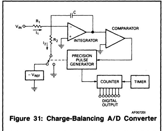
**Figure 31: Charge-Balancing A/D Converter**
