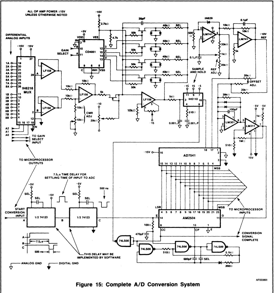
Figure 15: Complete A/D Conversion System
