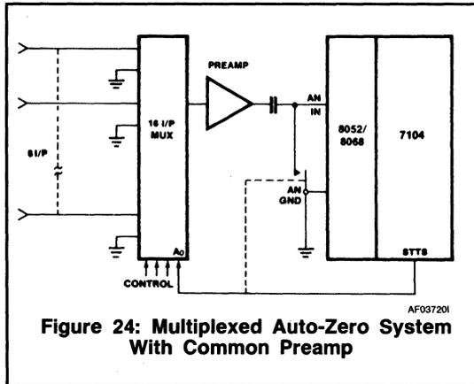
Figure 24: Multiplexed Auto-Zero System With Common Preamp
