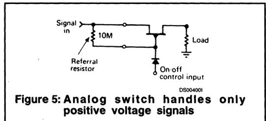
**Figure 5: Analog switch handles only positive voltage signals**
