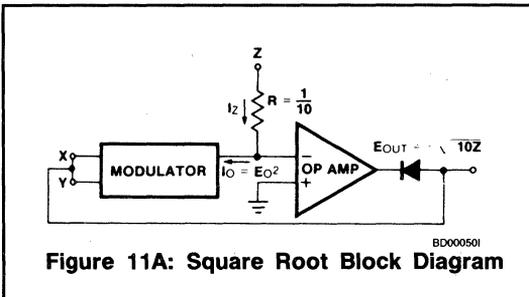
Figure 11A: Square Root Block Diagram
