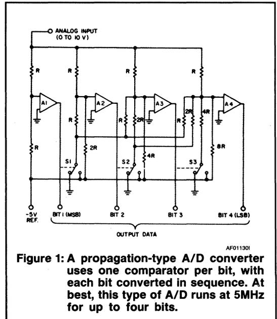
**Figure 1: A propagation-type A/D converter uses one comparator per bit, with each bit converted in sequence. At best, this type of A/D runs at 5MHz for up to four bits.**
