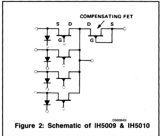
Figure 2: Schematic of IH5009 & IH5010
