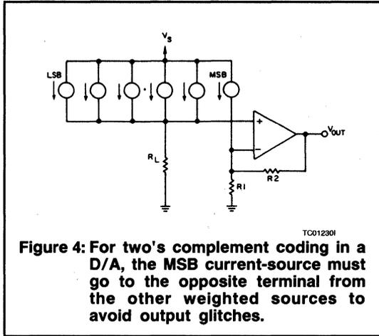
Figure 4: For two's complement coding in a D/A, the MSB current-source must go to the opposite terminal from the other weighted sources to avoid output glitches.
