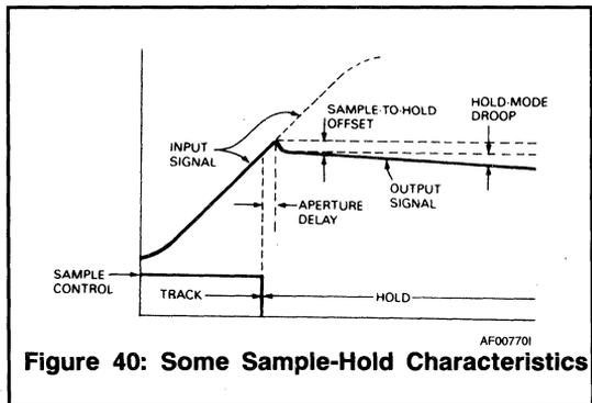
The most critical phase of sample-and-hold operation is the transition from the sample mode to the hold mode. Several important parameters characterize this transition. *Sample-to-hold offset* (or step) error is the change in output voltage from the sample mode to the hold mode, with a constant input voltage. It is caused by the switch transferring charge onto the hold capacitor as it turns off.
