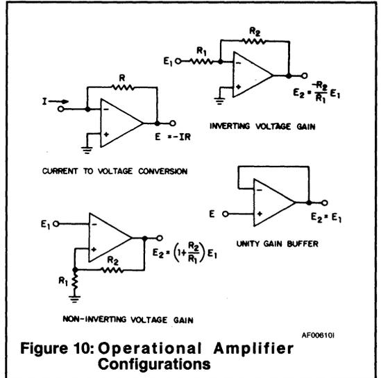
Figure 10: Operational Amplifier Configurations
