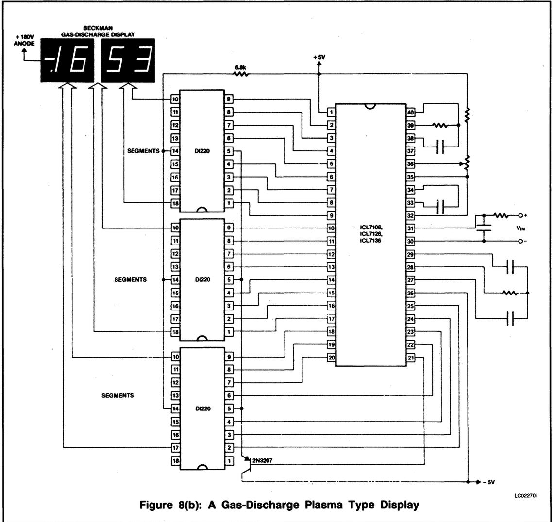
Figure 8(b): A Gas-Discharge Plasma Type Display
