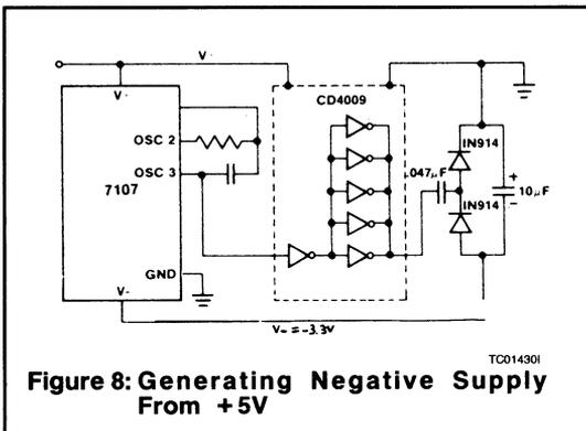
Figure 8: Generating Negative Supply From +5V
