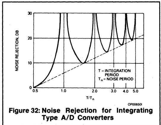
**Figure 32: Noise Rejection for Integrating Type A/D Converters**
