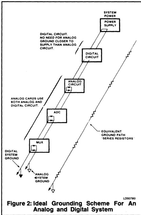
Figure 2: Ideal Grounding Scheme For An Analog and Digital System
