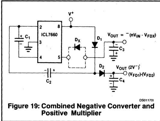
Figure 19: Combined Negative Converter and Positive Multiplier
