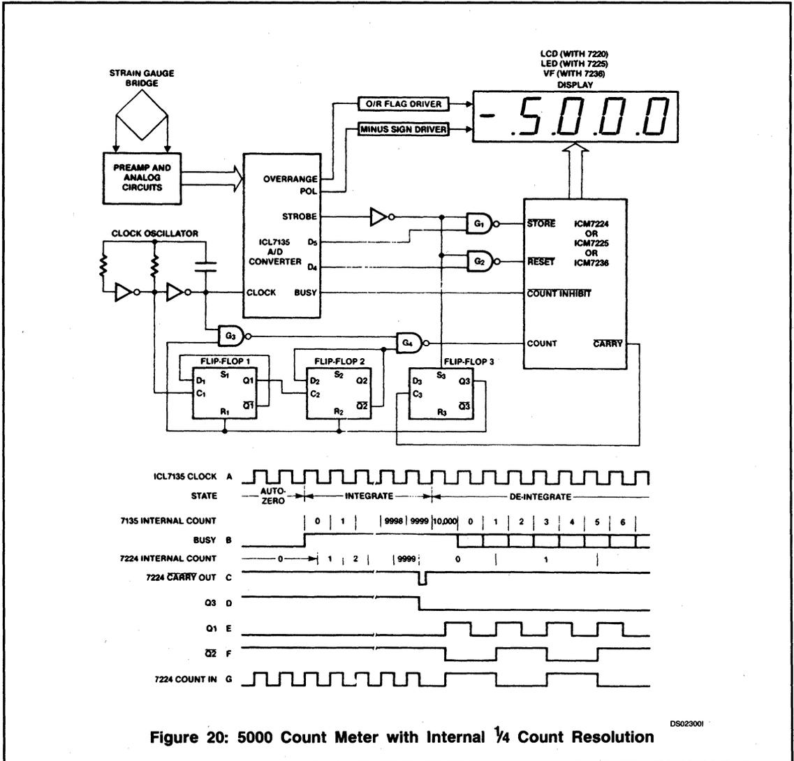
Figure 20: 5000 Count Meter with Internal  $\frac{1}{4}$  Count Resolution
