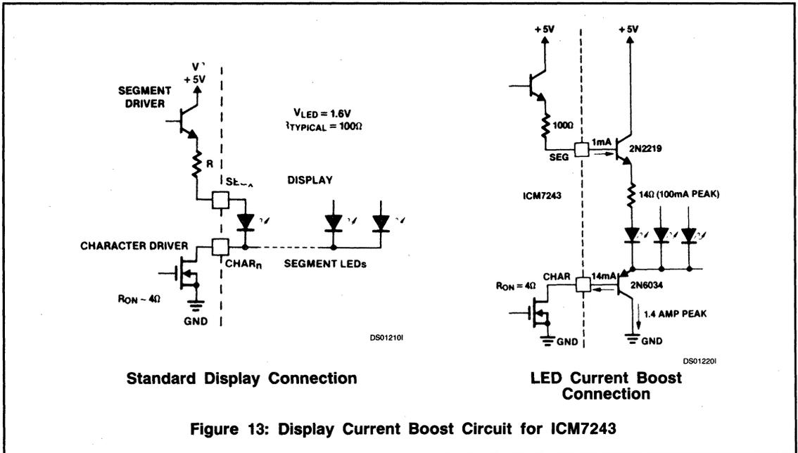
The average segment current of the ICM7243 is 3mA maximum (24mA/8 digits). This is quite enough current to give good contrast to the 0.375 or 0.4 inch high displays. If larger displays are to be driven it is an easy task to add a simple transistor current boost circuit to each character and
