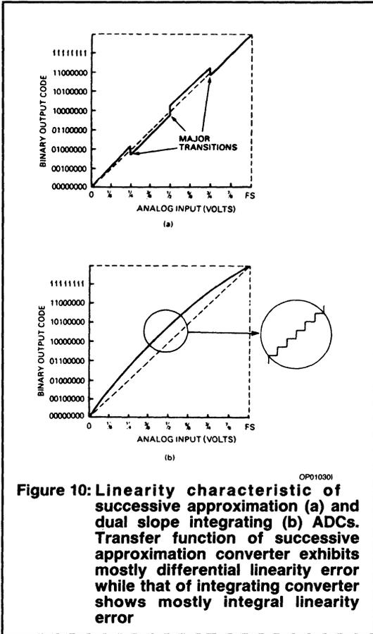
Figure 10(b) shows a dual-slope integrating ADC transfer function. In this case, the predominant nonlinearity is the integral linearity error; differential linearity error is almost nonexistent in integrating type ADCs, which also includes charge balancing ADCs. The curvature of the transfer function is caused by a nonideal integrator circuit. Differential linearity is determined by the time between clock pulses in the converter, and this is constant within any conversion cycle.
