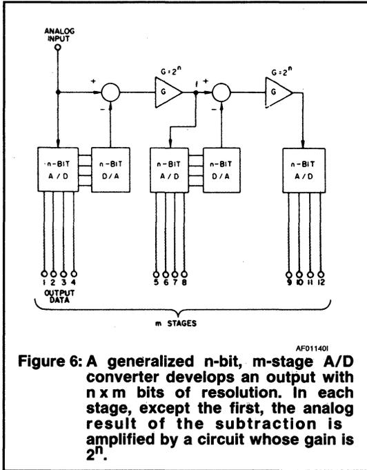
**Figure 6: A generalized n-bit, m-stage A/D converter develops an output with  $n \times m$  bits of resolution. In each stage, except the first, the analog result of the subtraction is amplified by a circuit whose gain is  $2^n$ .**
