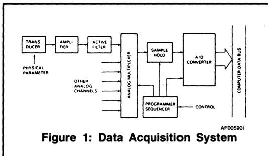
Figure 1: Data Acquisition System
