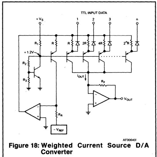
**Figure 18: Weighted Current Source D/A Converter**
