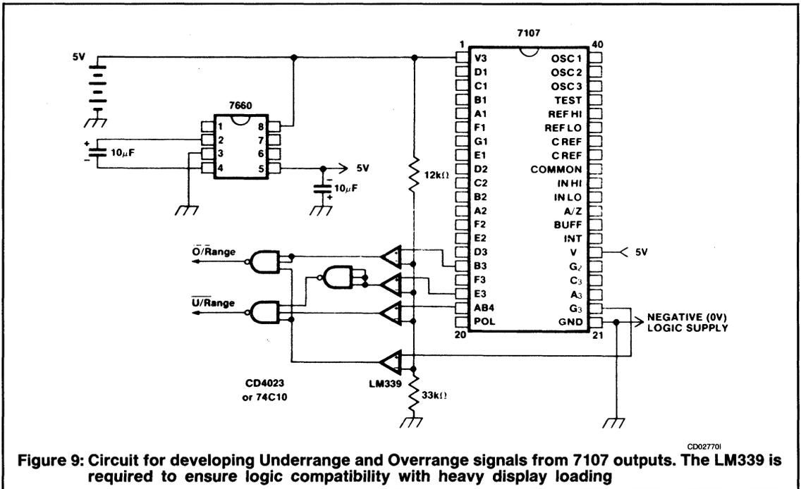
Figure 9: Circuit for developing Underrange and Overrange signals from 7107 outputs. The LM339 is required to ensure logic compatibility with heavy display loading
