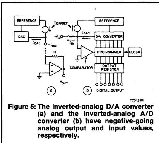
Figure 5: The inverted-analog D/A converter (a) and the inverted-analog A/D converter (b) have negative-going analog output and input values, respectively.
