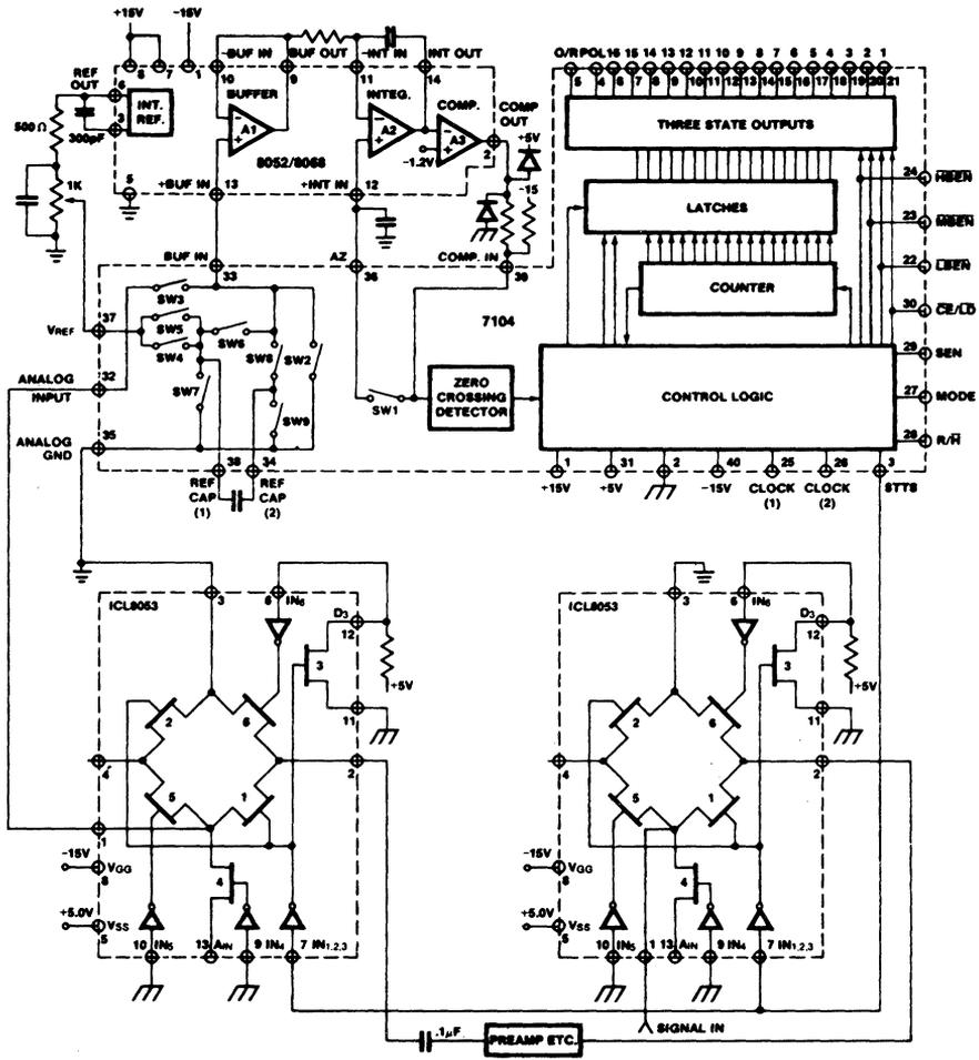
Figure 21: External Auto-Zero System Using 8053 Switches
