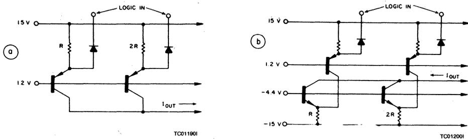
**Figure 1: Weighted current-source configurations for straight binary (a) and complementary binary (b) coding generate output current in different directions. The resistor weighting determines the output code.**
