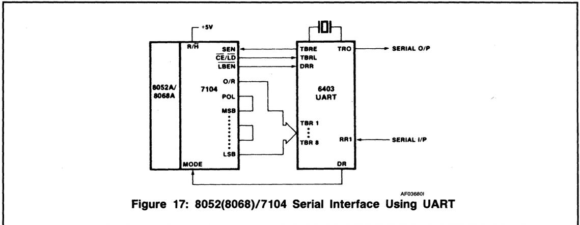
Figure 17: 8052(8068)/7104 Serial Interface Using UART
