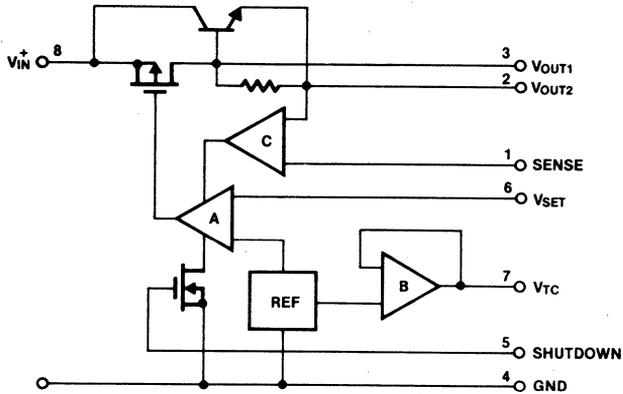
Figure 6: Functional Diagram of the ICL7663 CMOS Regulator
