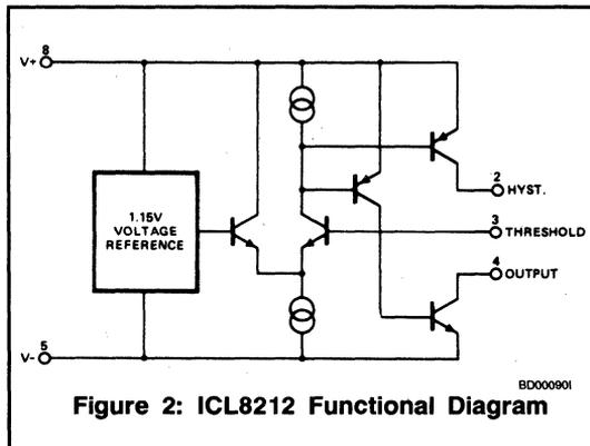
Figure 2: ICL8212 Functional Diagram
