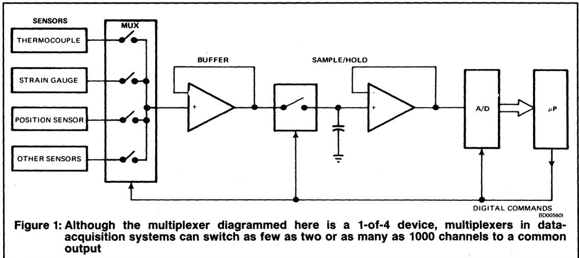
Figure 1: Although the multiplexer diagrammed here is a 1-of-4 device, multiplexers in data-acquisition systems can switch as few as two or as many as 1000 channels to a common output
