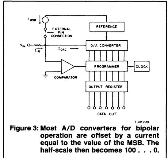
Figure 3: Most A/D converters for bipolar operation are offset by a current equal to the value of the MSB. The half-scale then becomes 100 . . . 0.
