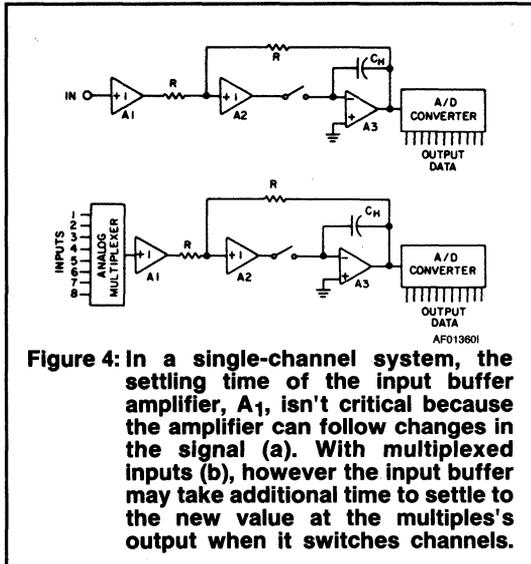
**Figure 4:** In a single-channel system, the settling time of the input buffer amplifier, A<sub>1</sub>, isn't critical because the amplifier can follow changes in the signal (a). With multiplexed inputs (b), however the input buffer may take additional time to settle to the new value at the multiplexer's output when it switches channels.
