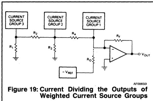
**Figure 19: Current Dividing the Outputs of Weighted Current Source Groups**
