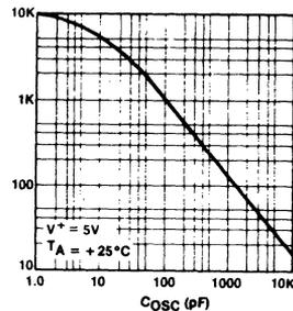
Figure 11: Frequency Variation with Oscillator Capacitance
