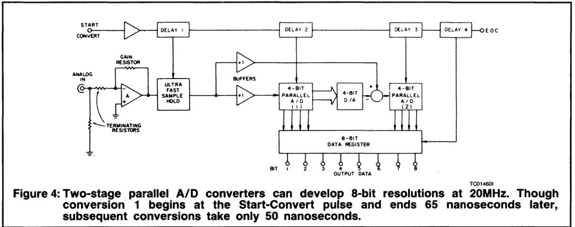
Figure 4: Two-stage parallel A/D converters can develop 8-bit resolutions at 20MHz. Though conversion 1 begins at the Start-Convert pulse and ends 65 nanoseconds later, subsequent conversions take only 50 nanoseconds.
