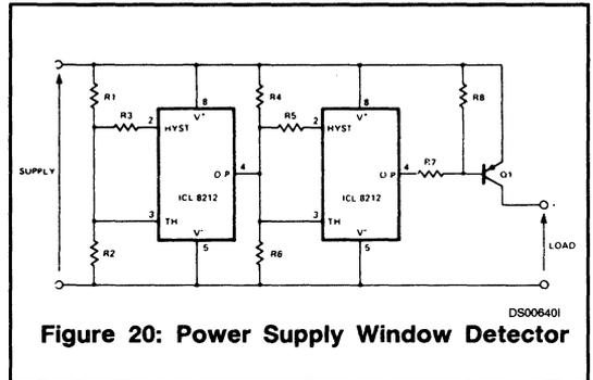
Figure 20: Power Supply Window Detector
