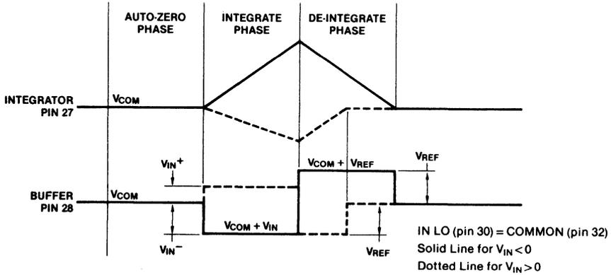
Figure 6: Integrator and Buffer Waveforms for Circuit of Figure 5
