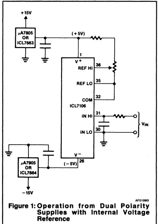
**Figure 1: Operation from Dual Polarity Supplies with Internal Voltage Reference**
