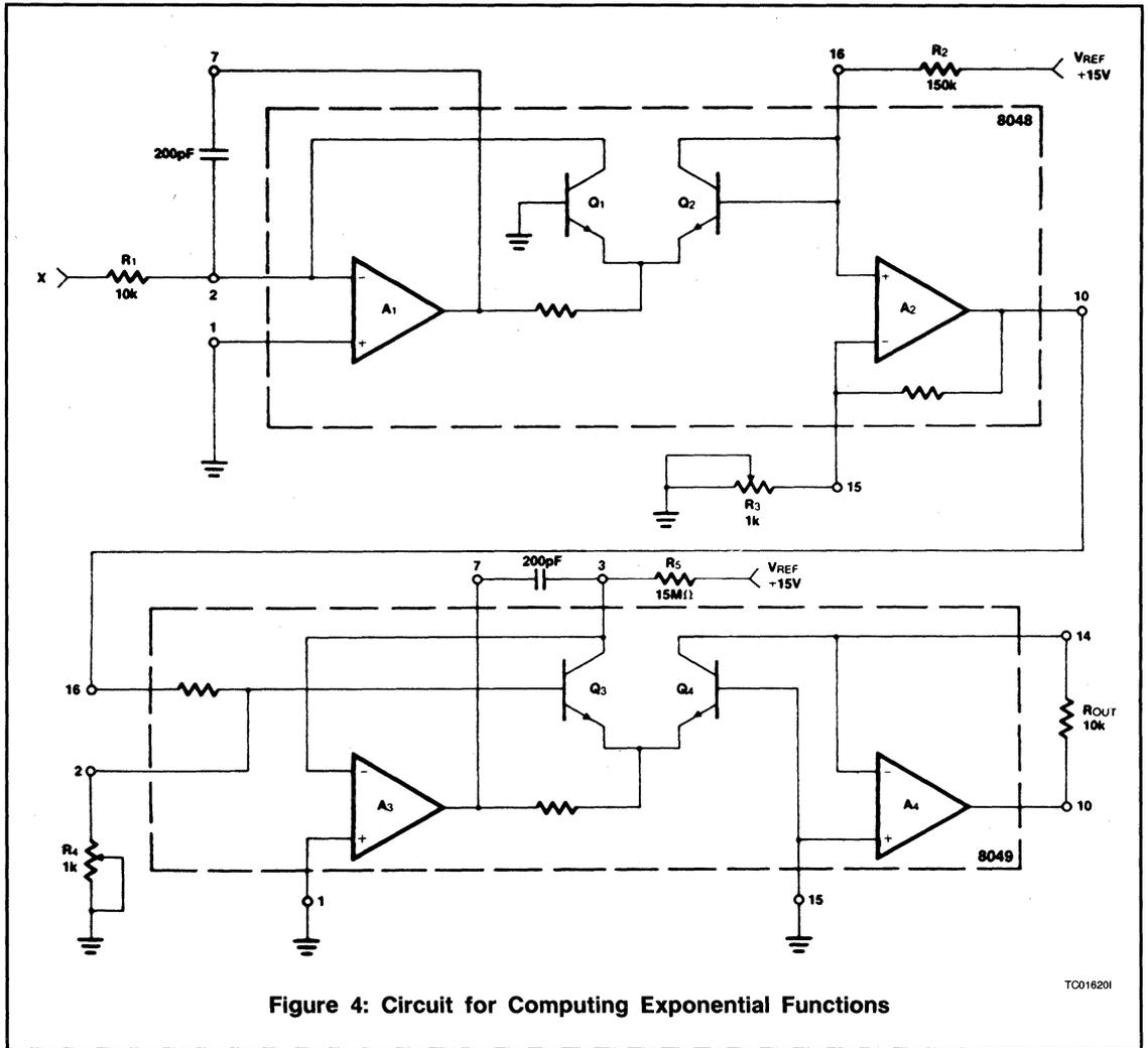
Figure 4: Circuit for Computing Exponential Functions
