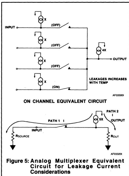
**Figure 5: Analog Multiplexer Equivalent Circuit for Leakage Current Considerations**
