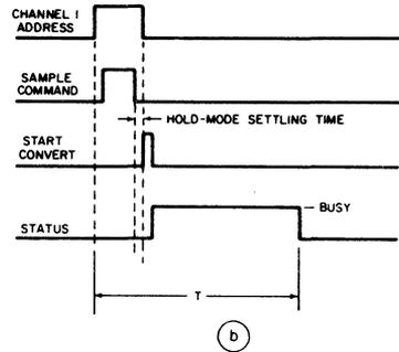
**Figure 3:** A data-acquisition system scans a number of analog inputs and converts them, one at a time, to digital form (a). The sample-hold provides an unchanging input to the converter until its conversion is complete. When it's finished, the STATUS line goes low to permit the next input in sequence to be converted (b).
