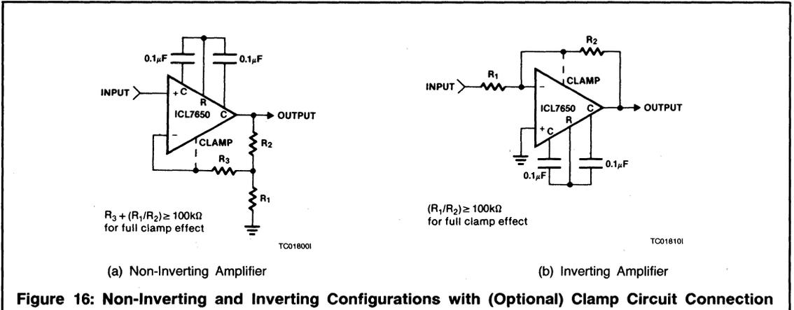
**Figure 16: Non-Inverting and Inverting Configurations with (Optional) Clamp Circuit Connection**
