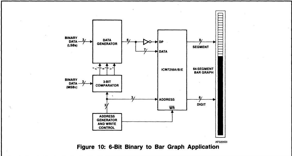
Figure 10: 6-Bit Binary to Bar Graph Application
