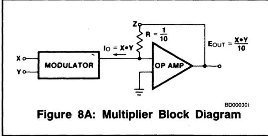
**Figure 8A: Multiplier Block Diagram**
