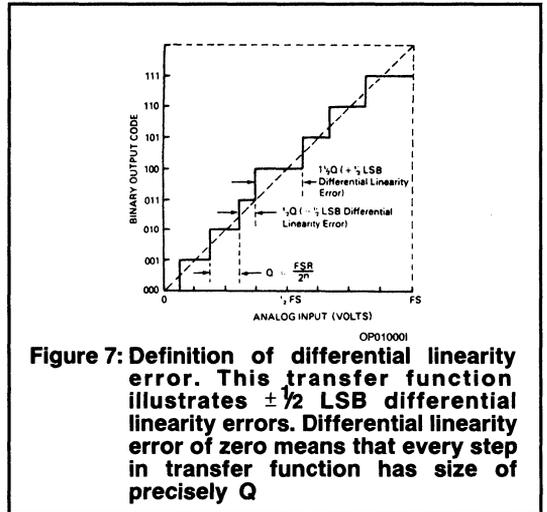
**Figure 7: Definition of differential linearity error. This transfer function illustrates  $\pm 1/2$  LSB differential linearity errors. Differential linearity error of zero means that every step in transfer function has size of precisely Q**
