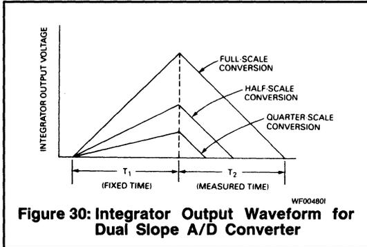
**Figure 30: Integrator Output Waveform for Dual Slope A/D Converter**
