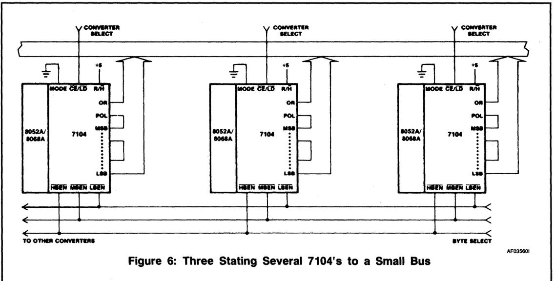
Figure 6: Three Stating Several 7104's to a Small Bus
