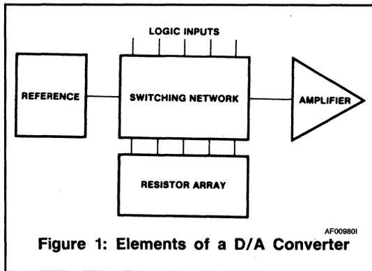
Figure 1: Elements of a D/A Converter
