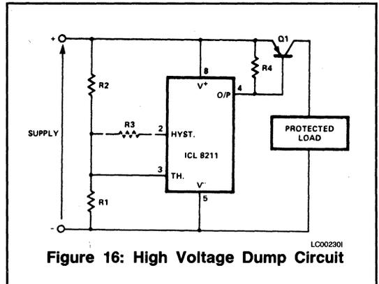
**Figure 16: High Voltage Dump Circuit**
