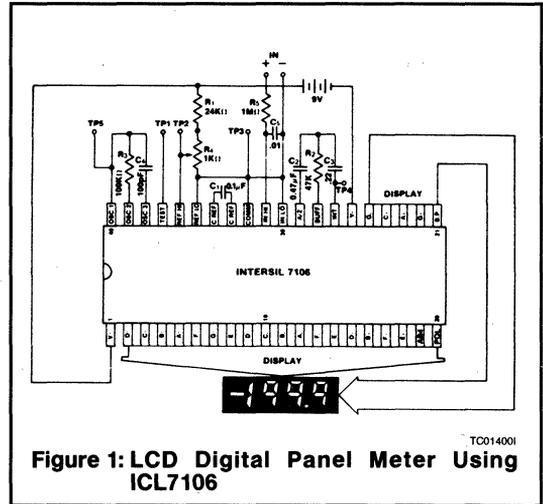
Figure 1: LCD Digital Panel Meter Using ICL7106
