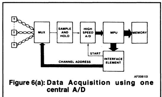
**Figure 6(a): Data Acquisition using one central A/D**
