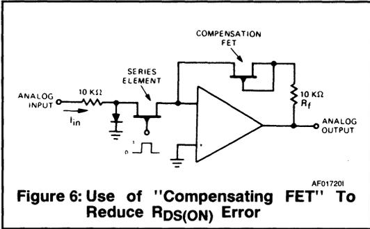
**Figure 6: Use of "Compensating FET" To Reduce  $R_{DS(ON)}$  Error**
