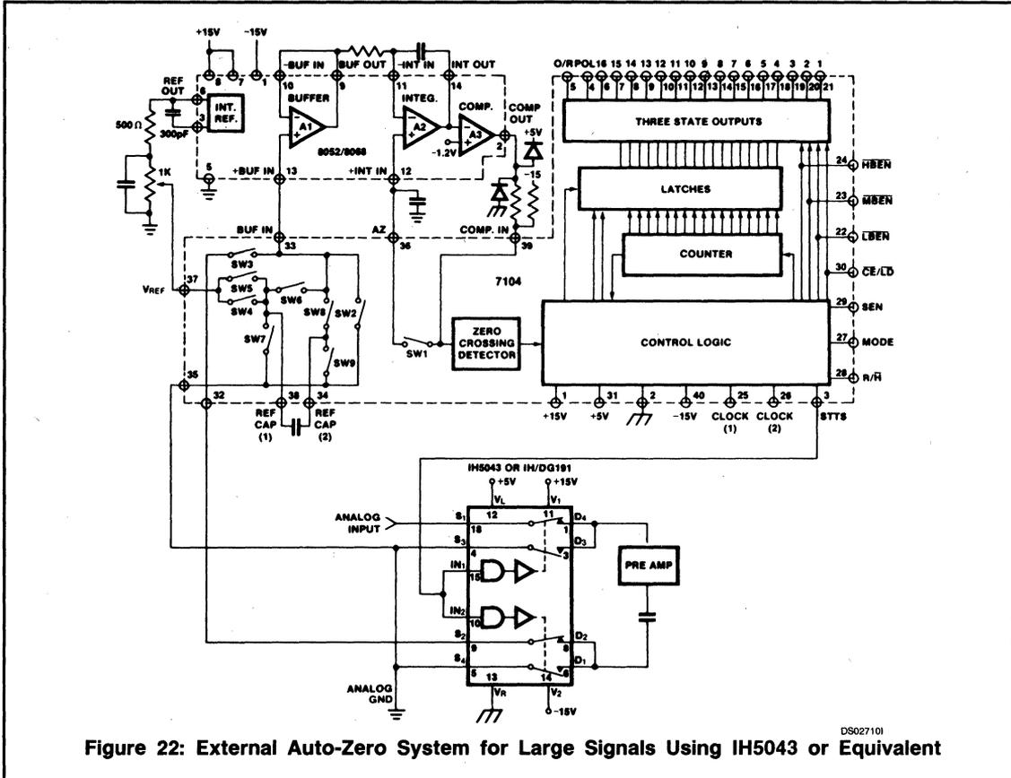
Figure 22: External Auto-Zero System for Large Signals Using IH5043 or Equivalent
