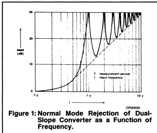
**Figure 1: Normal Mode Rejection of Dual-Slope Converter as a Function of Frequency.**
