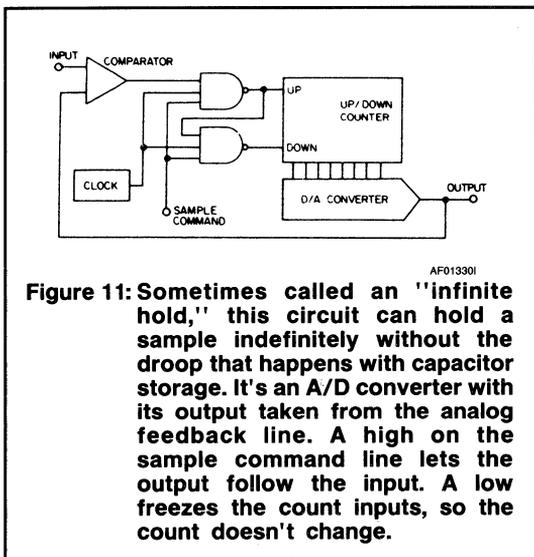
**Figure 11: Sometimes called an "infinite hold," this circuit can hold a sample indefinitely without the droop that happens with capacitor storage. It's an A/D converter with its output taken from the analog feedback line. A high on the sample command line lets the output follow the input. A low freezes the count inputs, so the count doesn't change.**
