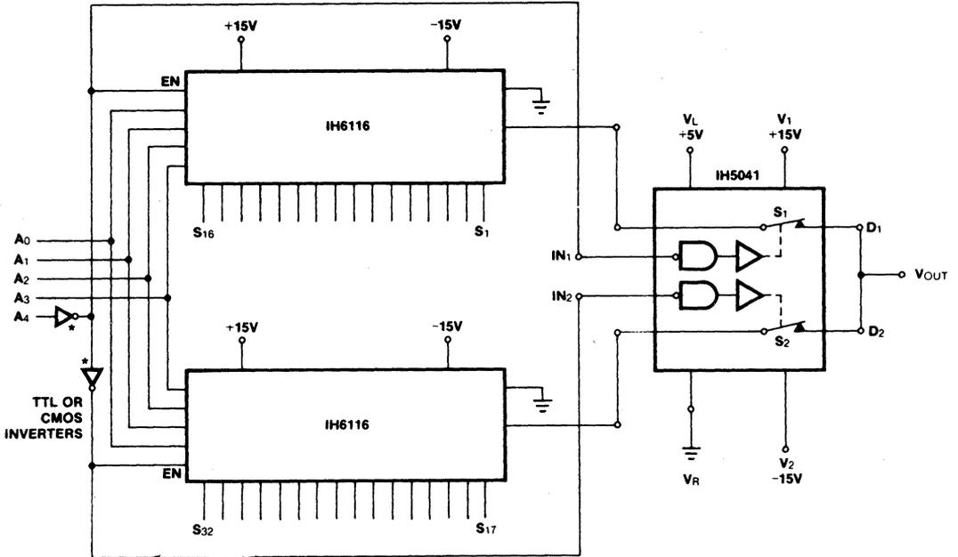
\*TTL gate must have resistor pullup to +5V to drive "EN" input.
