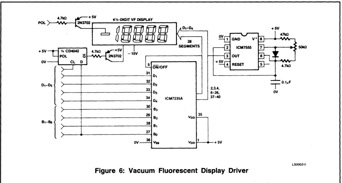
Figure 6: Vacuum Fluorescent Display Driver
