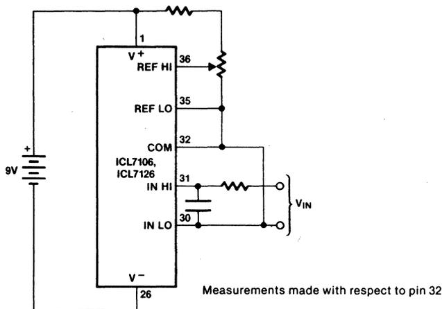
**Figure 5: Operation from 9 Volt Battery with Internal Voltage Reference**
