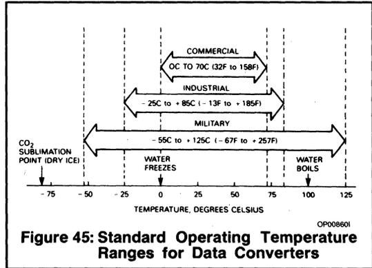
**Figure 45: Standard Operating Temperature Ranges for Data Converters**
