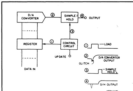
**Figure 9: An output developed by many D/A converters for certain input-code transitions temporarily goes the wrong way. This transient, or "glitch", is undesirable in some applications and can be removed by sampling the converter's output after the glitch has gone by.**
