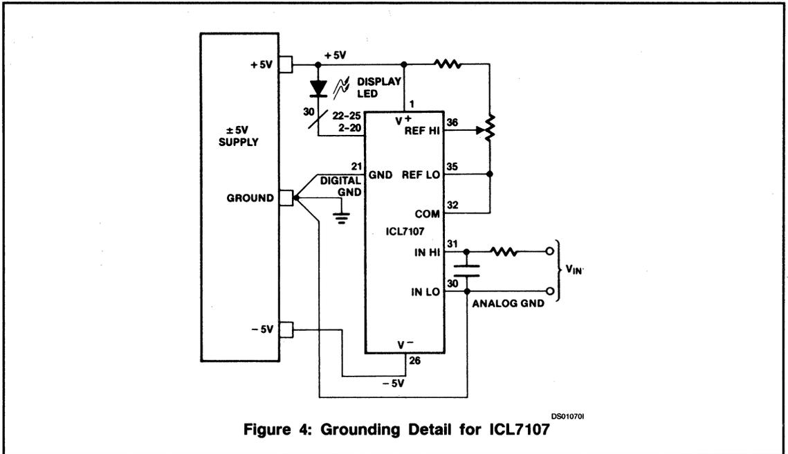
Figure 4: Grounding Detail for ICL7107
