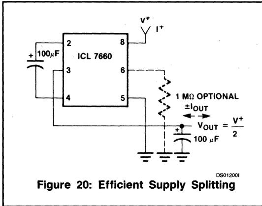
Figure 20: Efficient Supply Splitting
