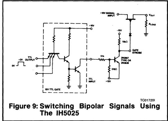
**Figure 9: Switching Bipolar Signals Using The IH5025**
