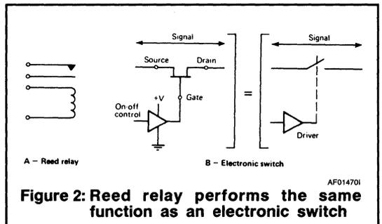
**Figure 2: Reed relay performs the same function as an electronic switch**
