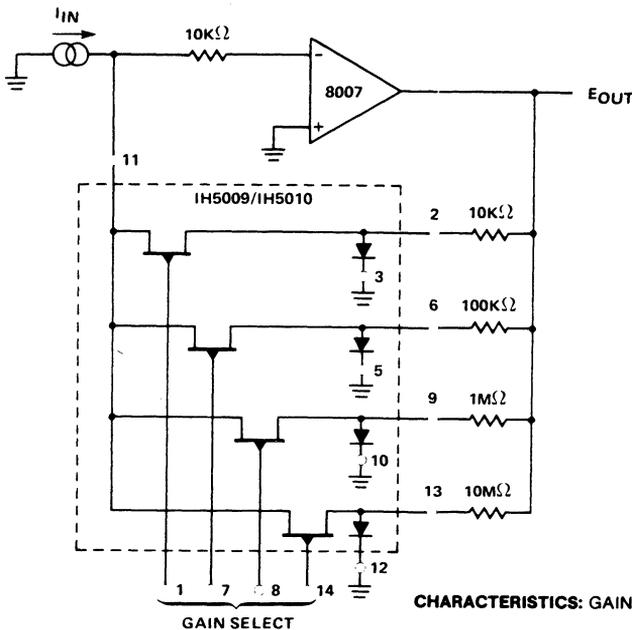
**CHARACTERISTICS:** GAIN =  $\frac{-E_{OUT}}{I_{IN}} = R_{FB}$
