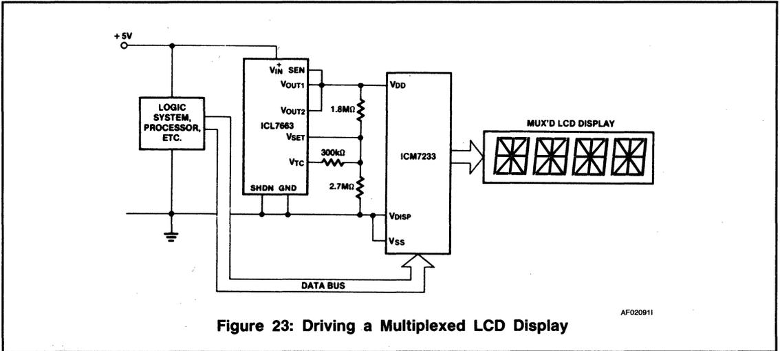
Figure 23: Driving a Multiplexed LCD Display
