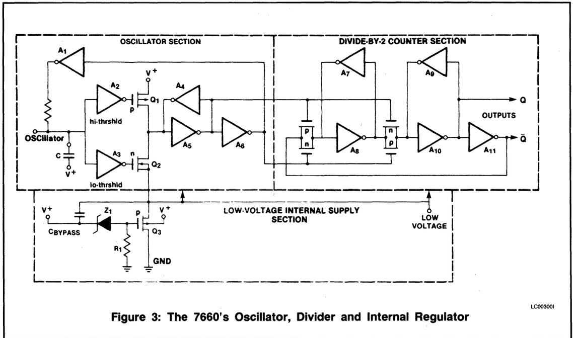
**Figure 3: The 7660's Oscillator, Divider and Internal Regulator**
