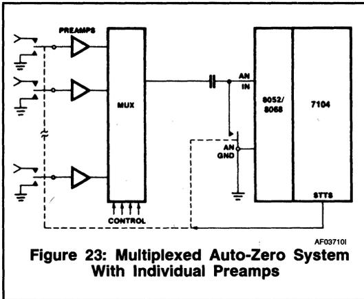
Figure 23: Multiplexed Auto-Zero System With Individual Preamps
