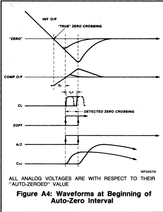
**Figure A4: Waveforms at Beginning of Auto-Zero Interval**
