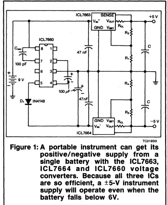
**Figure 1: A portable instrument can get its positive/negative supply from a single battery with the ICL7663, ICL7664 and ICL7660 voltage converters. Because all three ICs are so efficient, a  $\pm 5\text{-V}$  instrument supply will operate even when the battery falls below 6V.**
