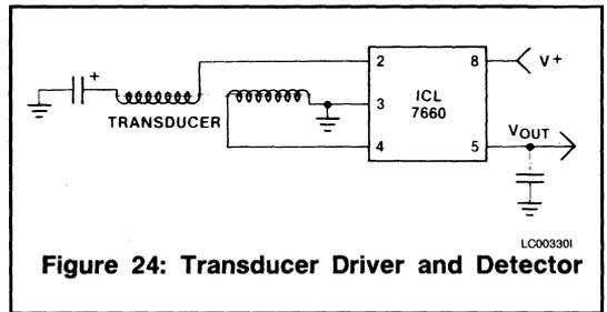
**Figure 24: Transducer Driver and Detector**
