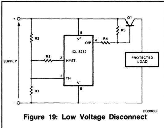
Figure 19: Low Voltage Disconnect
