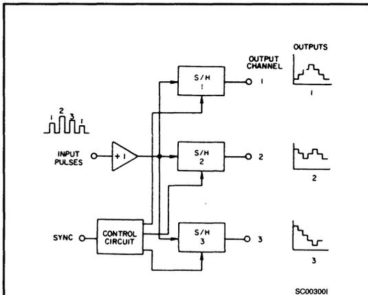
**Figure 10: When analog signals are encoded by pulse-amplitude modulation and then multiplexed, they can be sorted out and reconstructed by a set of sample-holds with properly timed sample commands. The time scale of the input is shorter than that of the outputs.**
