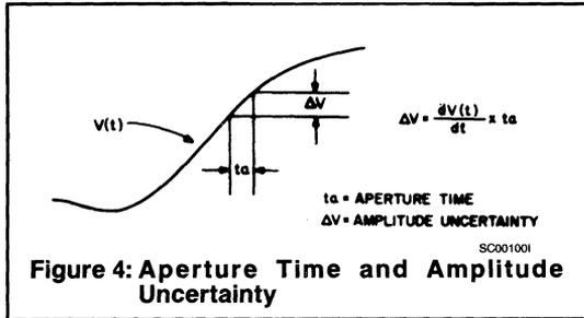
As shown in Figure 4, the input signal to the A/D converter changes by  $\Delta V$  during the aperture time  $t_a$  in which the conversion is performed. The error can be considered an amplitude error or a time error; the two are related as follows
