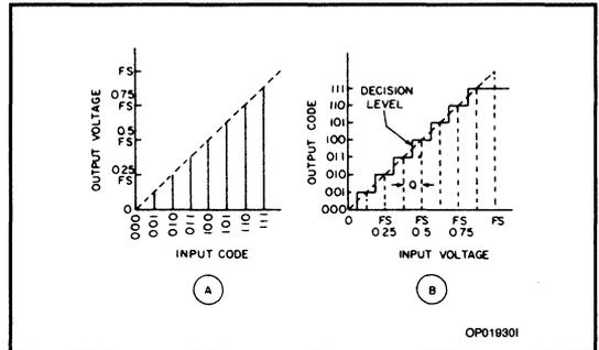
Complementary-binary, positive-true coding is also used in D/A converters. This scheme is used because of the weighted current source configuration employed in many converter designs.
