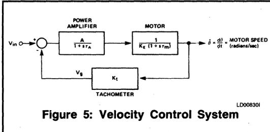
Figure 5: Velocity Control System
