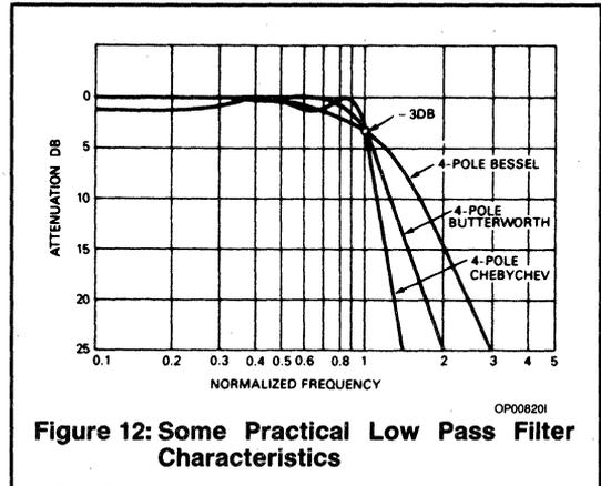
Figure 12: Some Practical Low Pass Filter Characteristics
