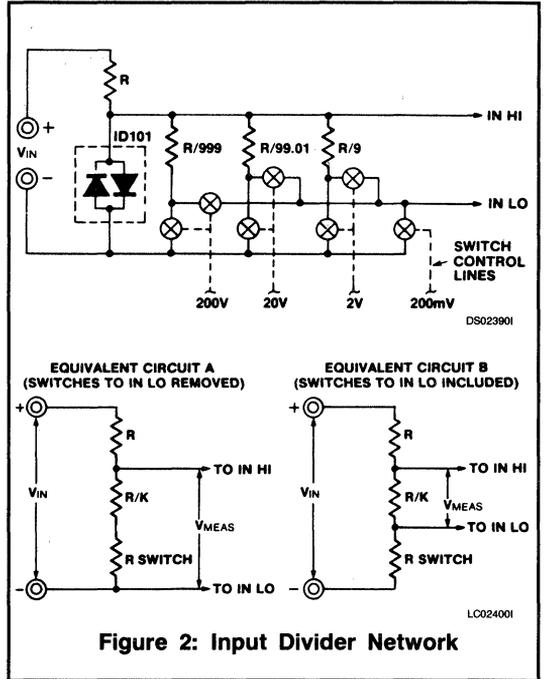
Figure 2: Input Divider Network
