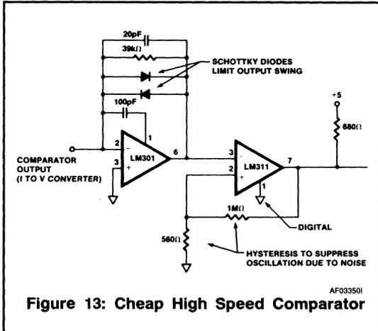
Figure 13: Cheap High Speed Comparator
