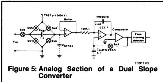
**Figure 5: Analog Section of a Dual Slope Converter**
