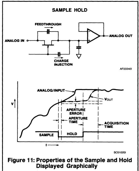
Figure 11: Properties of the Sample and Hold Displayed Graphically
