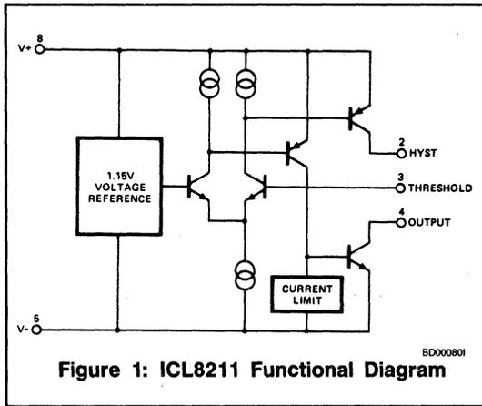
Figure 1: ICL8211 Functional Diagram
