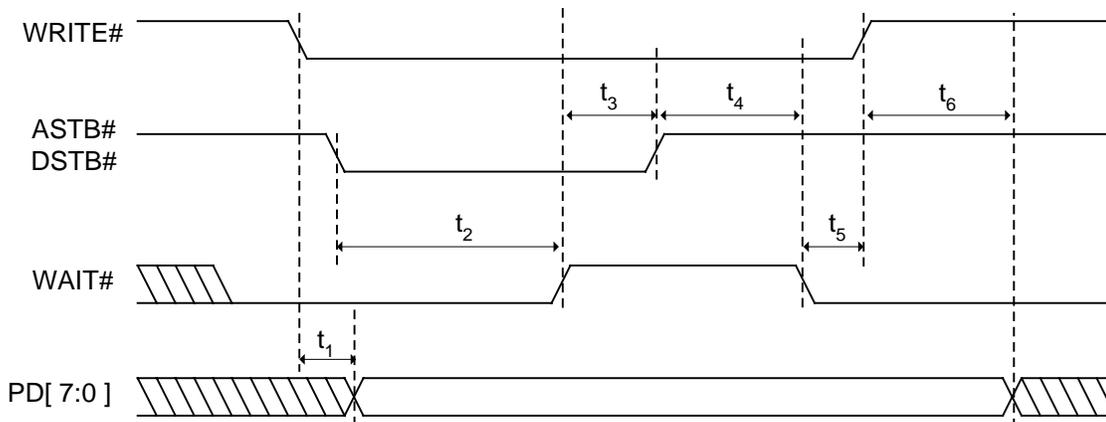
Figure 11-7. EPP Address or Data Write Cycle
