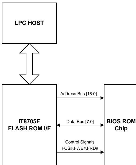
Figure 9-8. FLASH ROM Interface Diagram
