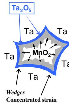
In the tantalum anode pellet, areas of constriction exist where tantalum particles form a closed loop around an open channel. The MnO<sub>2</sub> filling this enclosure is a hard, crystalline material. The impregnation process involves dip at +25°C and conversion at +270°C. Stresses might be the root of cracks created in the dielectric.
