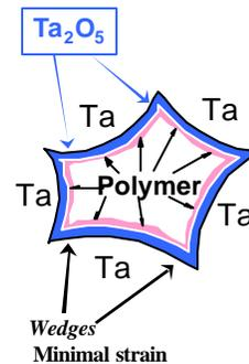
The polymer material is soft and elastic. The forces generated because of mismatches in CTEs are insignificant when compared to MnO<sub>2</sub>. The process involves conversion at room temperature after each dip cycle -- not at any elevated temperatures.
