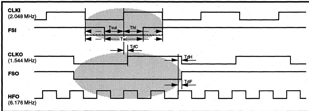
**Figure 4: LXP604 High to Low Frequency Conversion Frame Sync Alignment**
