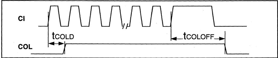
Figure 24: Mode 4 COL/CI Output Timing
