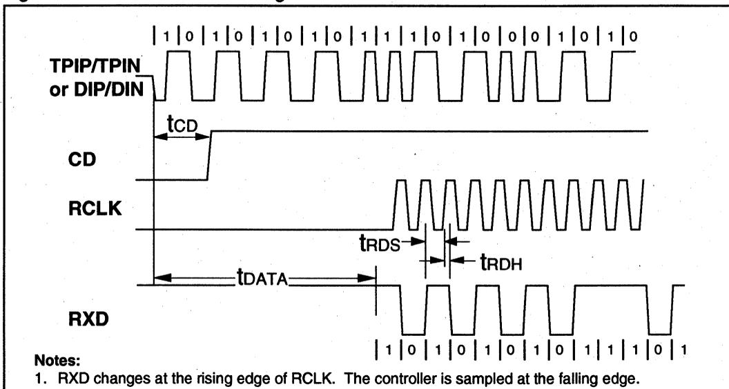
Figure 3: Mode 1 RCLK/EoF Timing
