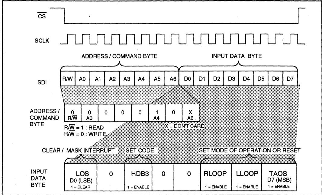
**Figure 10: LXT318 SIO Output Data Structure**
