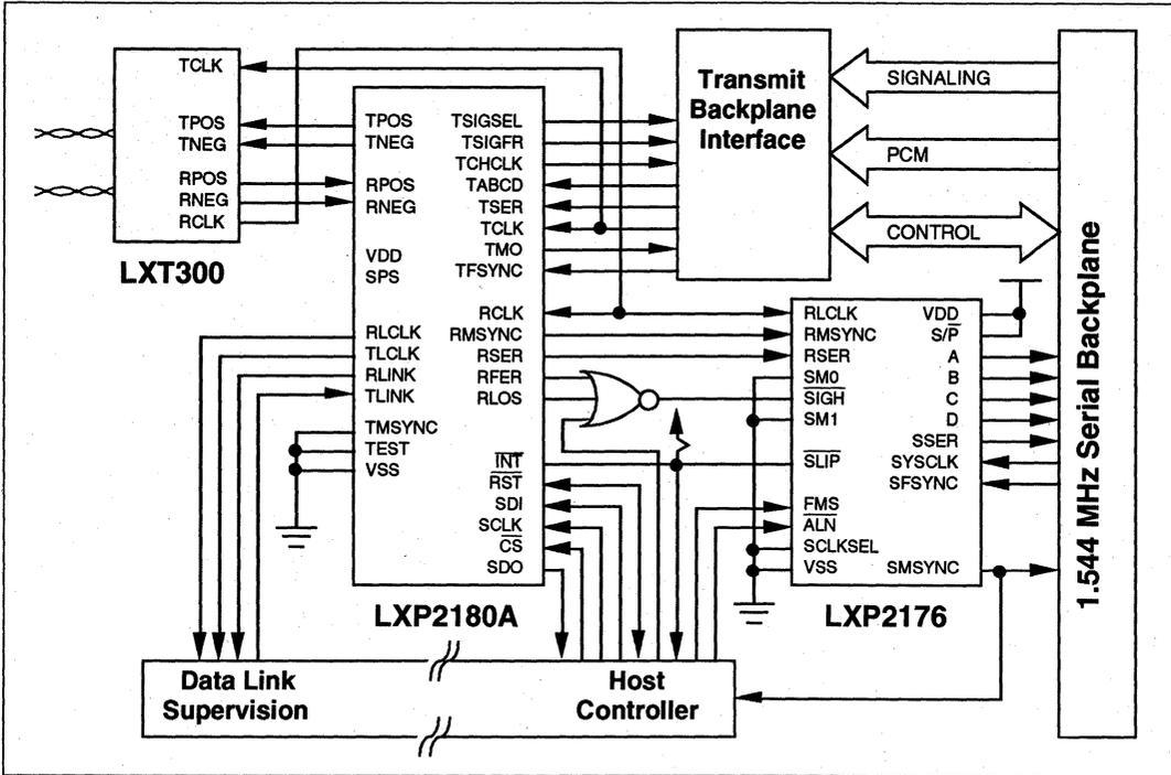
Figure 23: Processor-Based Transmit Signaling Insertion Application
