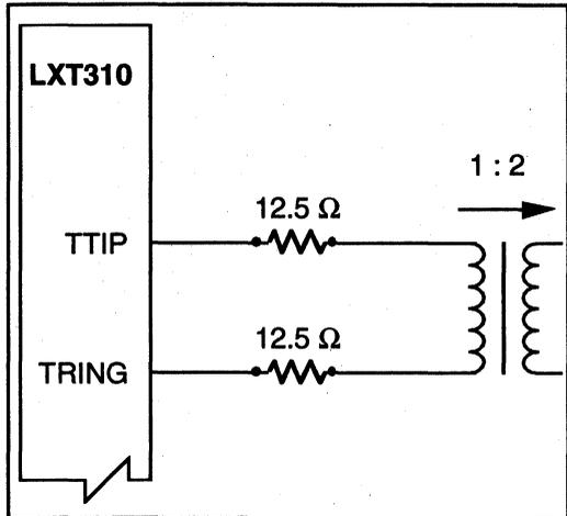
**Figure 1b: LXT310 Transmit Line Interface**
