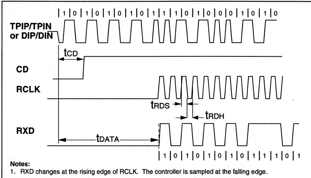
**Figure 15: Mode 3 RCLK/End-of-Frame Timing**
