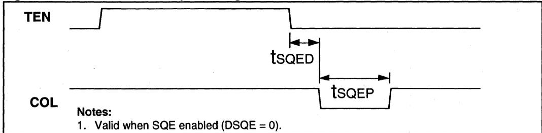
Figure 19: Mode 3 Loopback Timing
