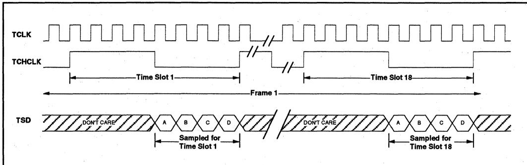
**Figure 9: CAS Output Format in Time Slot 16**
