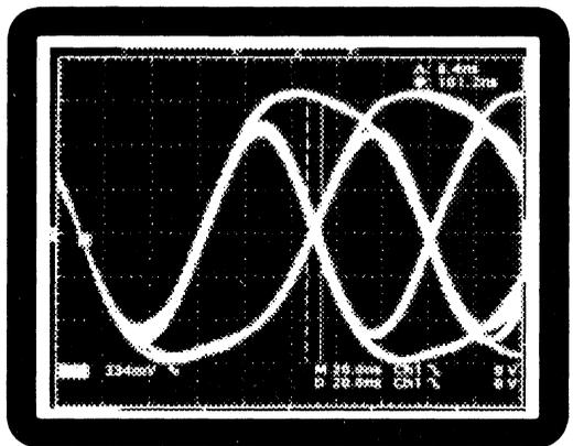
Figure 21: LXT902 Random Data Output Jitter (After Line Model - Falling Edge Trigger)
