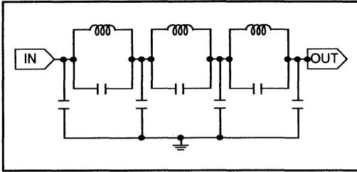
Figure 12: Receive Filter Diagram
