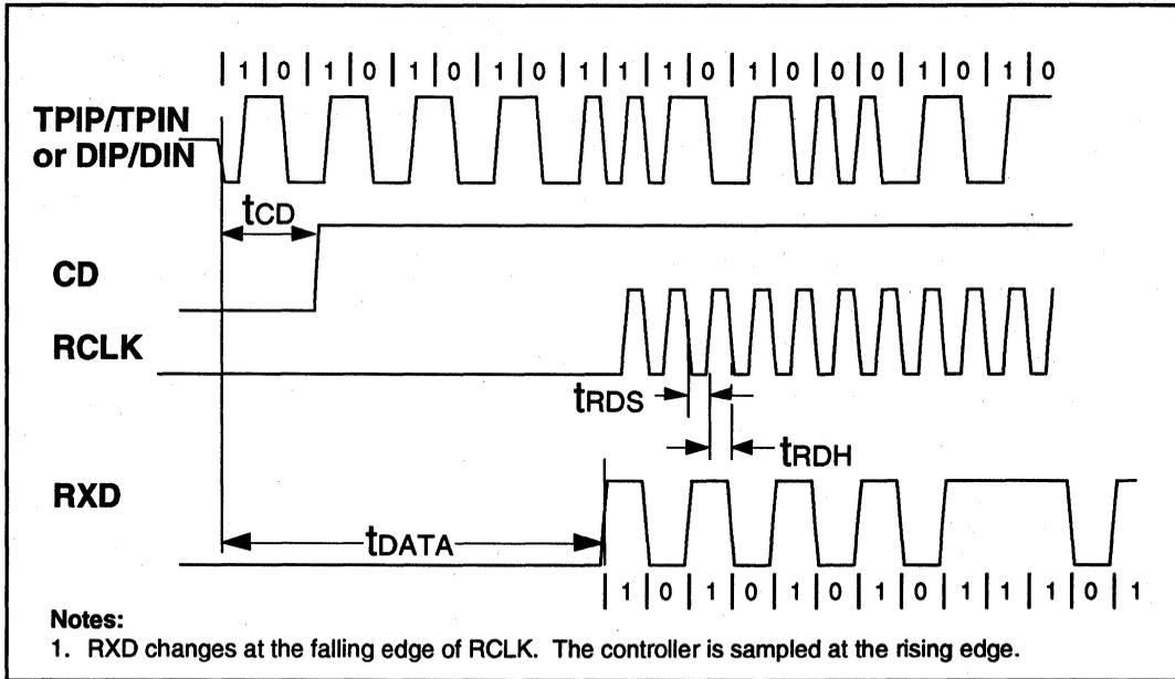
**Figure 21: Mode 4 RCLK/EoF Timing**
