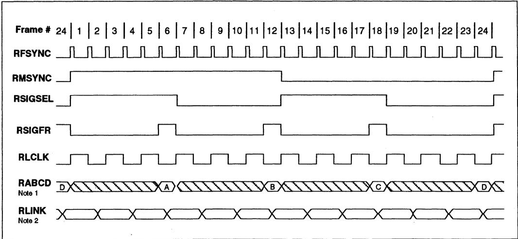
1. Signaling data is updated during signaling frames on channel boundaries. RABCD is the LSB of each channel word in non-signaling frames.
