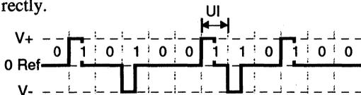
Jitter is measured in Unit Intervals (UIs). A UI is equal to the bit rate period. A UI is, therefore, the reciprocal of the frequency. For T1 service, a UI equals 648 ns, while the "1" pulse duration is 324 ns. Jitter amplitude is measured in UI pp (peak-to-peak). Jitter specifications have both an amplitude component and a frequency component; that is, for a given jitter parameter, performance will be specified at a particular amplitude (in UI pp) within a particular frequency band.
