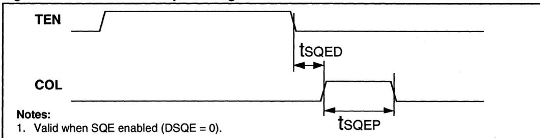
Figure 7: Mode 1 Loopback Timing
