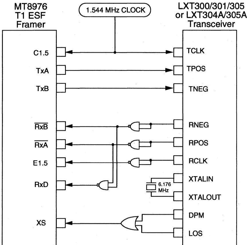
Figure 2: LXT300 interface to MT8979 E1 CRC Framing
