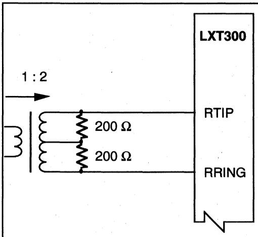
**Figure 2a: LXT300 Receive Line Interface**
