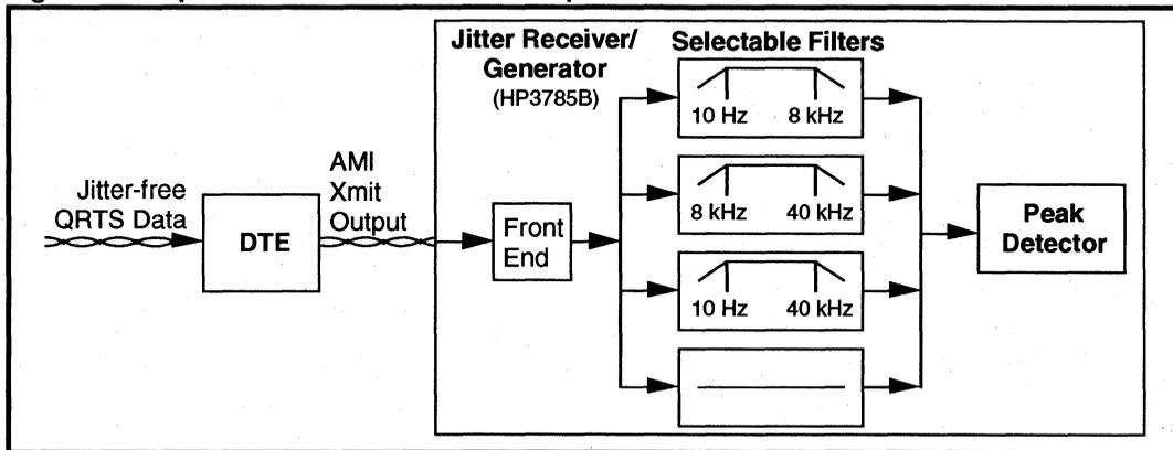
**Figure 5: Output Jitter Generation Specification**
