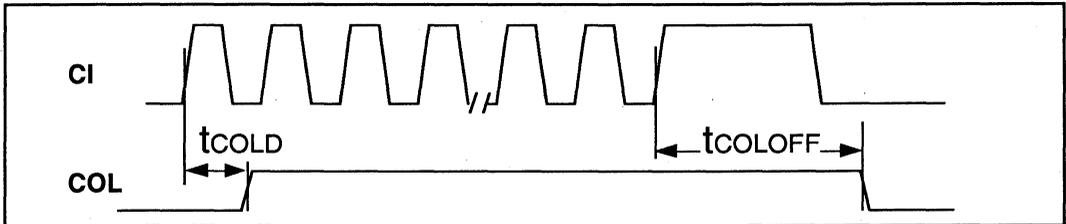
Figure 24: Mode 4 COL/CI Output Timing
