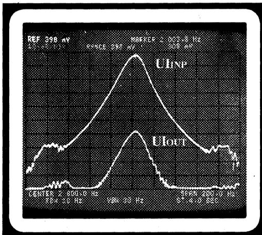
**Figure 9: Typical LXT304A JA Performance**
