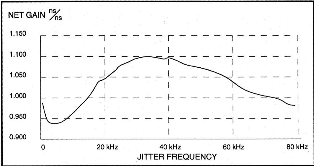
Figure 9: Nominal Jitter Transfer - 1.544 MHz CLKI to 2.048 MHz CLKO (Input Jitter = 0.25 UI)
