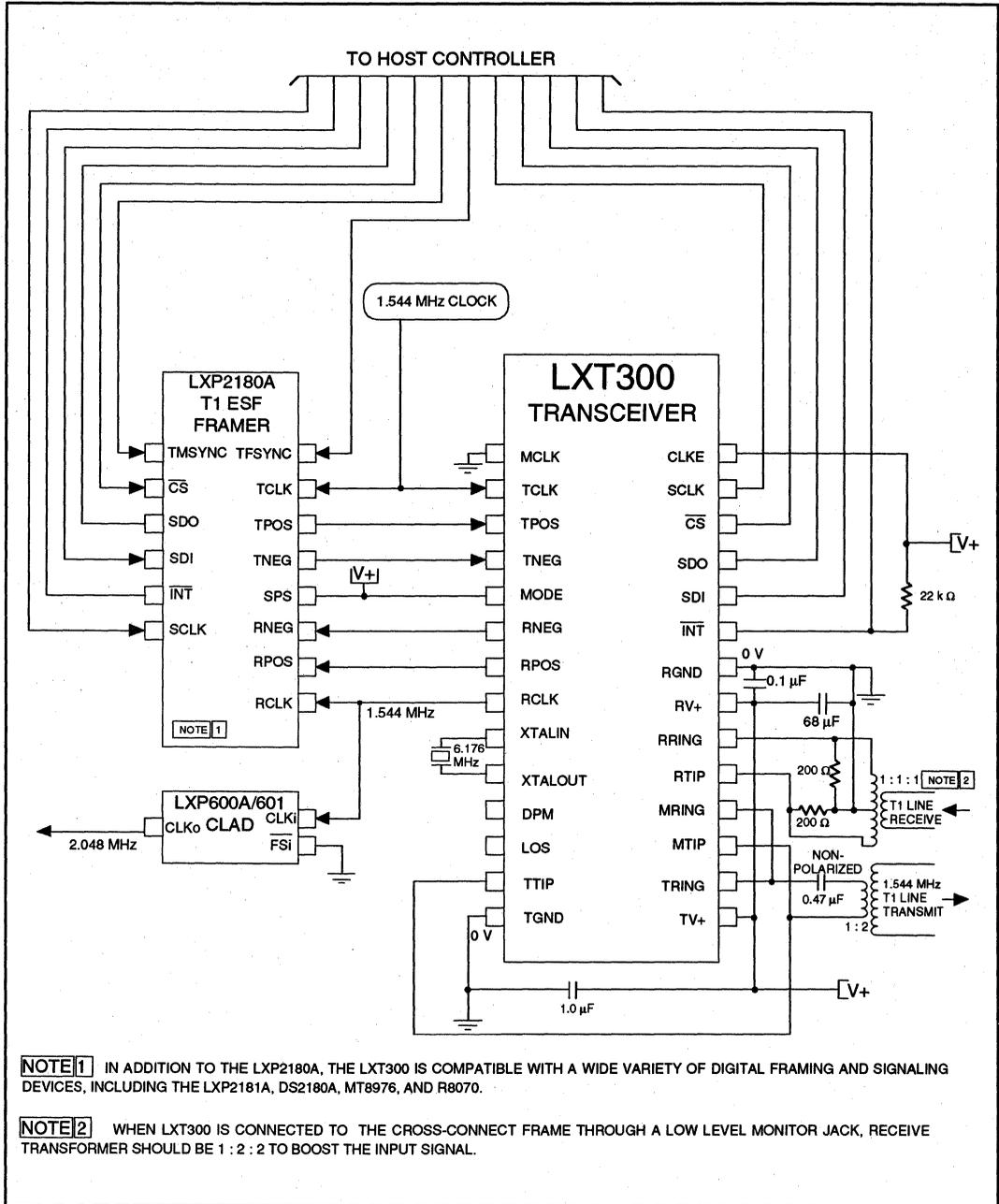
Figure 11: Typical LXT300 2.048 MHz E1 Application (Hardware Mode)
