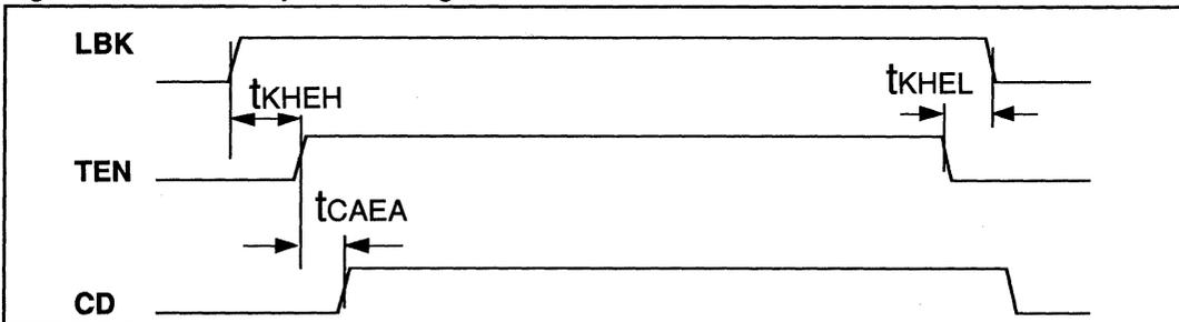
**Figures 8 through 13 - Timing Diagrams for Mode 2 (MD1 = 0, MD0 = 1)**
