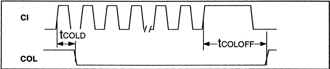
Figure 12: Mode 2 COL/CI Output Timing
