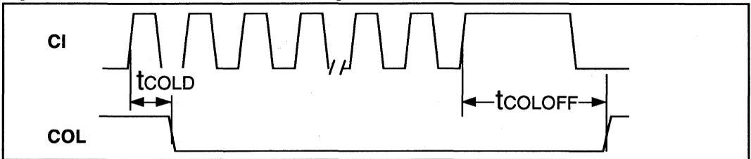
Figure 12: Mode 2 COL/CI Output Timing
