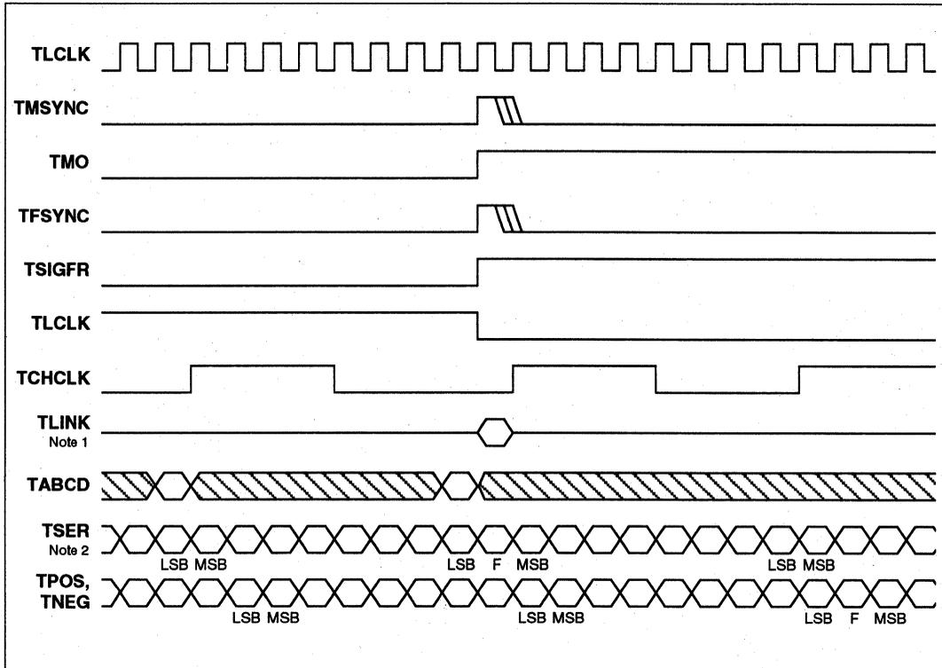
1. TLINK timing shown is for 193E framing. In 193E framing, TLINK is sampled as indicated for insertion into F-bit position of odd frames. When S-bit insertion is enabled in 193S framing, TLINK is sampled during even frames.
