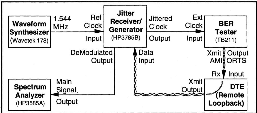
**NOTE:** The test setup shown in Figure 7 is used to measure jitter amplitudes less than 10 UI (the limit of the HP3785B). Alternate test setups should be used for other jitter amplitudes or amplitude/frequency combinations.
