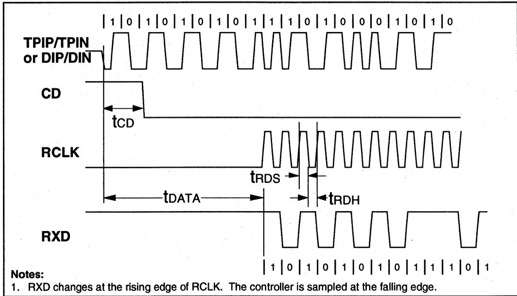
**Figure 9: Mode 2 RCLK/End-of-Frame Timing**
