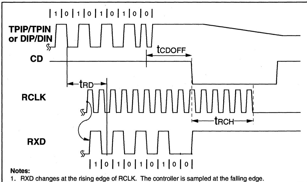
Figure 4: Mode 1 Transmit Timing
