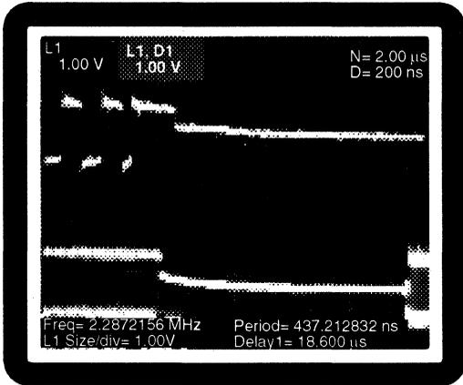
**Figure 7A: DI (AUI) End of Frame with Test Load (Transformer Coupling)**
