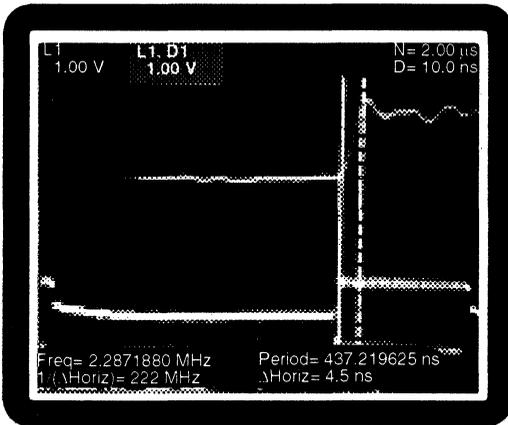
**Figure 6A: DI (AUI) Rise time < 5 ns with Test Load (Transformer Coupling)**
