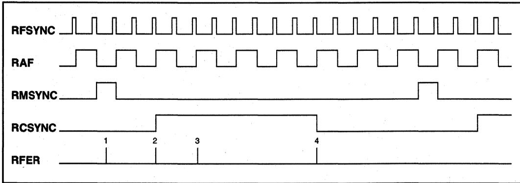
Figure 25: CAS Multiframe Alignment Error
