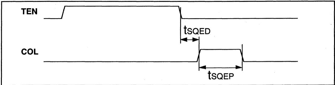
Figure 25: Mode 4 Loopback Timing
