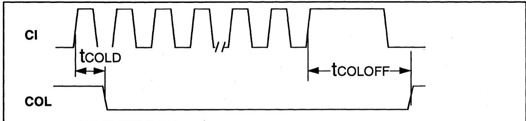
Figure 18: Mode 3 COL/CI Output Timing
