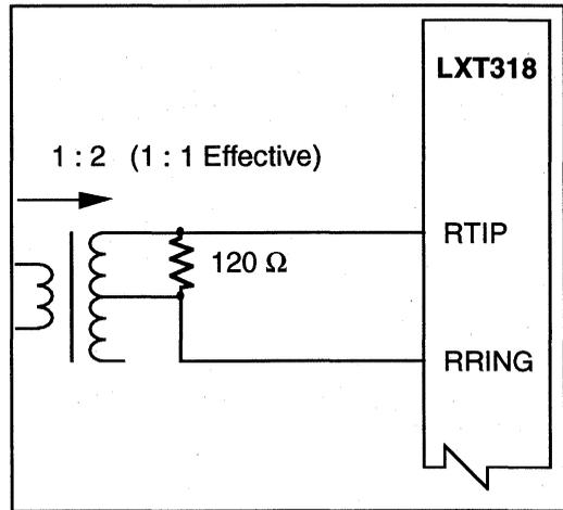
**Figure 2b: LXT318 Receive Line Interface**
