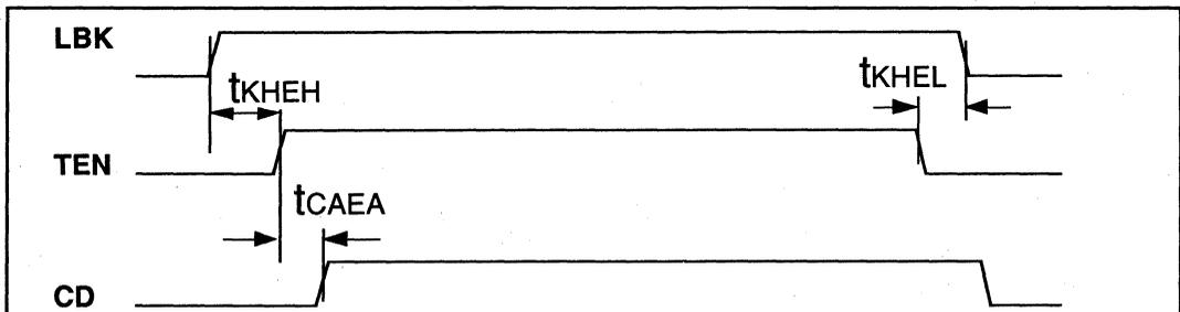
**Figures 20 through 25 - Timing Diagrams for Mode 4 (MD1 = 1, MD0 = 1)**
