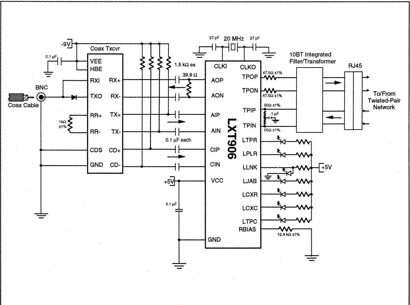
Figure 5: Typical TP to Coax Adapter Application Circuit
