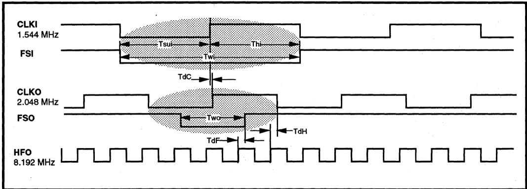
Figure 7: LXP604 Low to High Frequency Conversion Frame Sync Alignment
