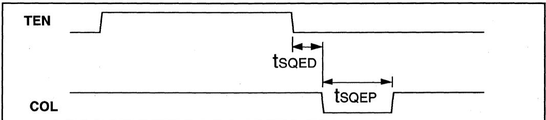
Figure 19: Mode 3 Loopback Timing
