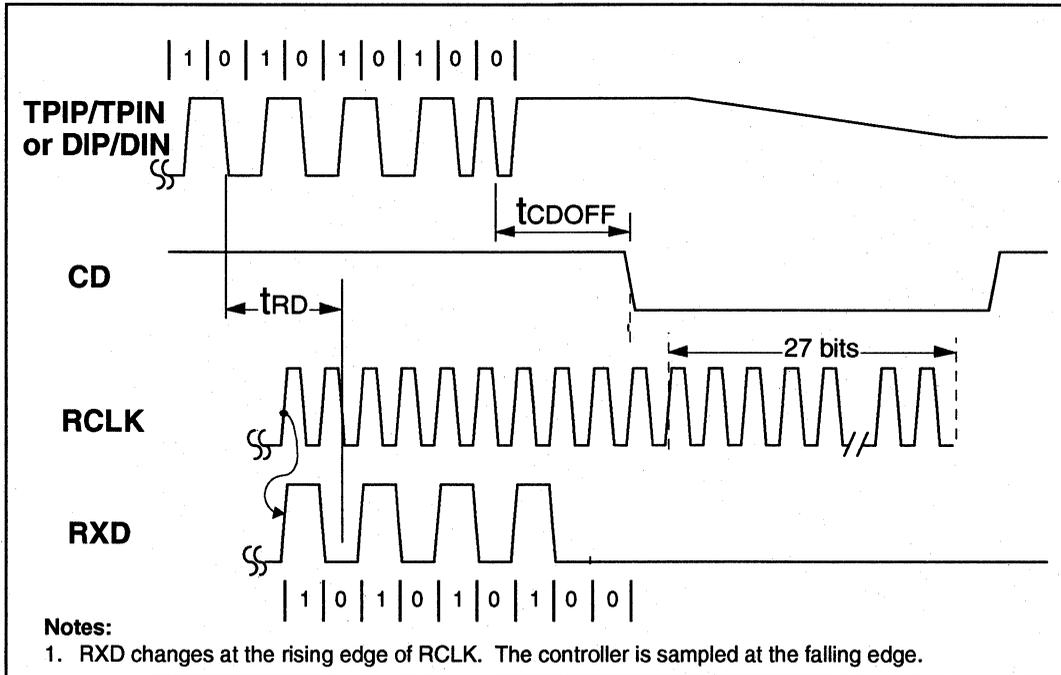
Figure 16: Mode 3 Transmit Timing
