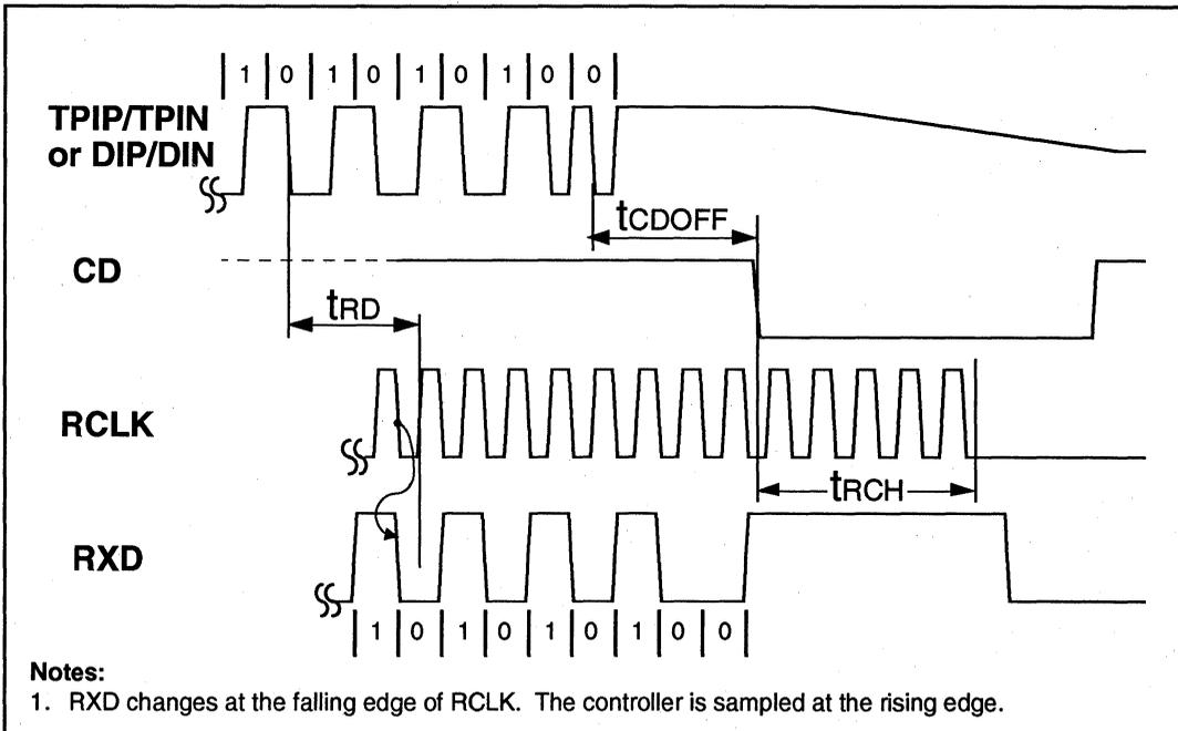
Figure 22: Mode 4 Transmit Timing
