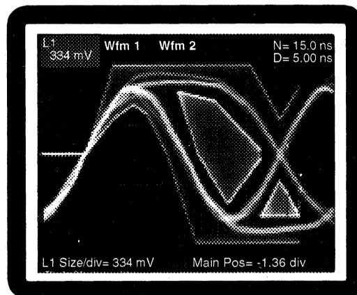
Figure 5A: TP Idle Pulse before Line Model with Test Load
