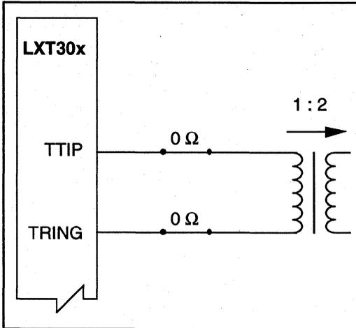
**Figure 1a: LXT30x Transmit Line Interface**
