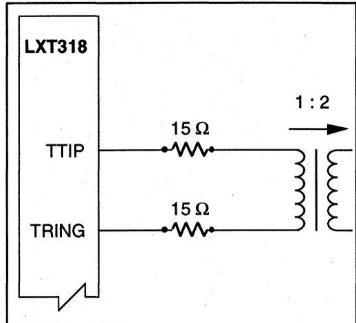
**Figure 1b: LXT318 Transmit Line Interface**
