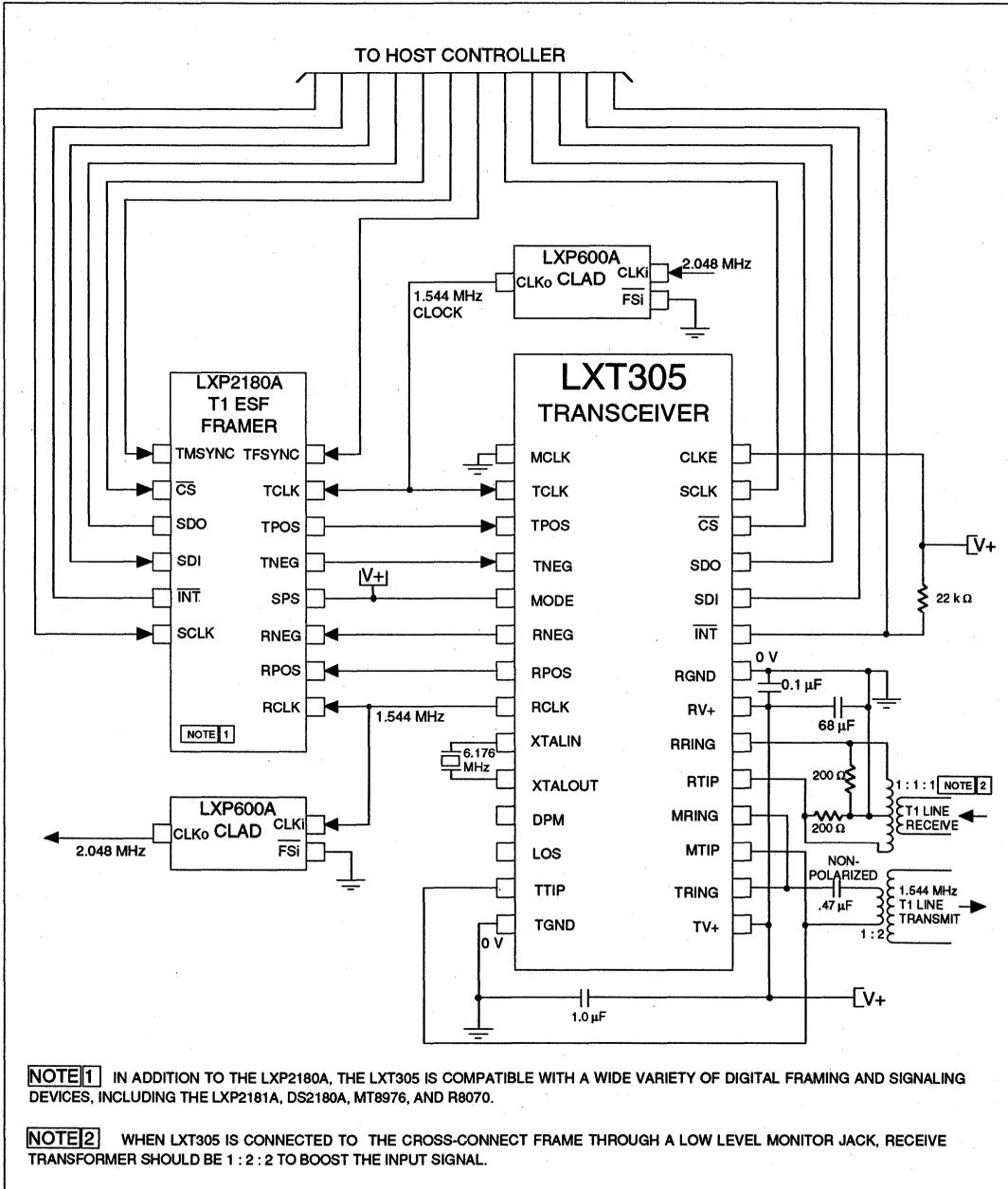
Figure 9: Typical LXT305 2.048 MHz E1 Application (Hardware Mode)
