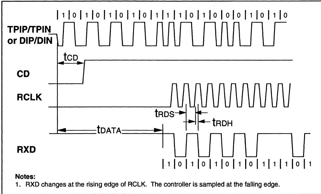
**Figure 3: Mode 1 RCLK/End-of-Frame Timing**
