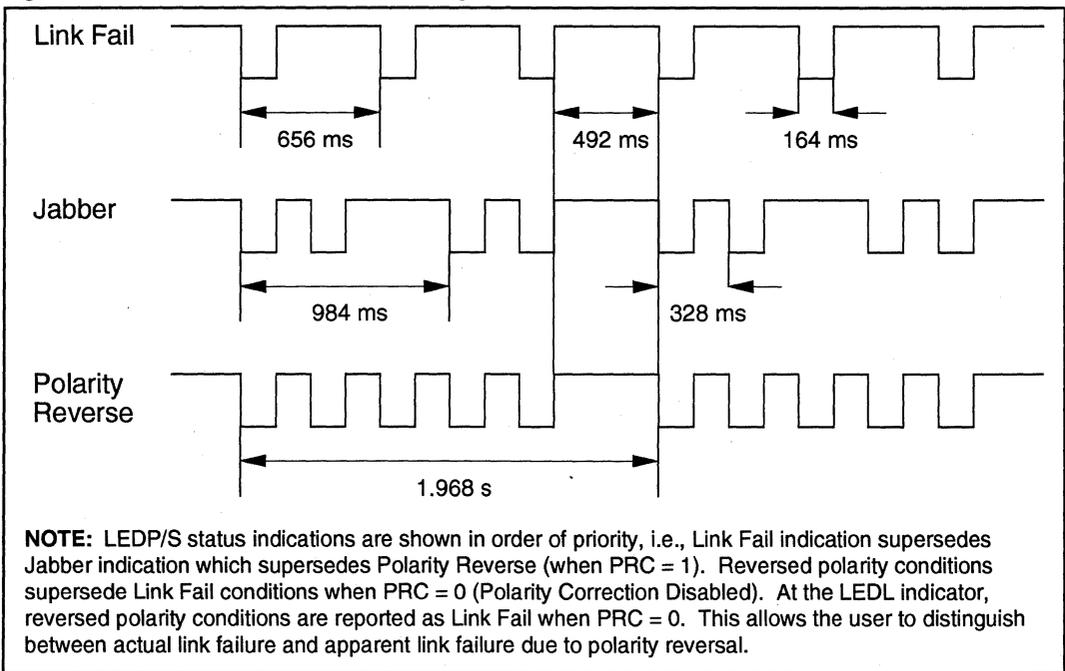
**NOTE:** LEDP/S status indications are shown in order of priority, i.e., Link Fail indication supersedes Jabber indication which supersedes Polarity Reverse (when PRC = 1). Reversed polarity conditions supersede Link Fail conditions when PRC = 0 (Polarity Correction Disabled). At the LEDL indicator, reversed polarity conditions are reported as Link Fail when PRC = 0. This allows the user to distinguish between actual link failure and apparent link failure due to polarity reversal.
