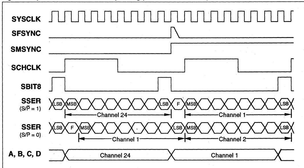
applications the F-bit is passed through the receive buffer and presented at SSER immediately after a rising edge on SFSYNC. The F-bit is dropped in 2.048 MHz applications and the MSB of channel 1 appears at SSER one bit period after a rising edge at SFSYNC. SSER is forced to 1 in all channels greater than 24. See Figures 3 and 4.
