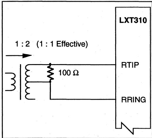
**Figure 2b: LXT310 Receive Line Interface**
