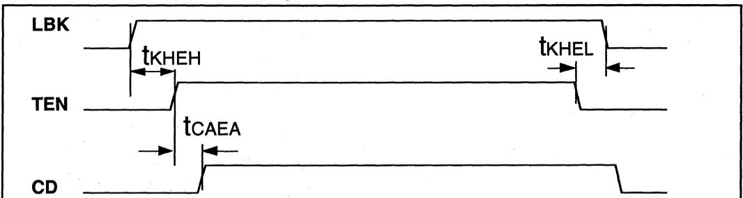
**Figures 20 through 25 - Timing Diagrams for Mode 4 (MD1 = 1, MD0 = 1)**
