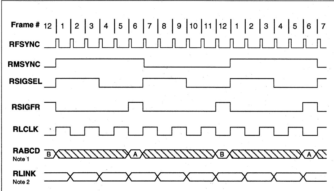
1. Signaling data is updated during signaling frames on channel boundaries. RABCD is the LSB of each channel word in non-signaling frames.
