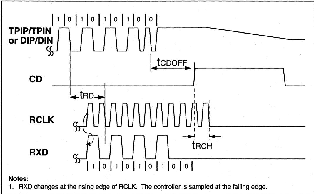
Figure 10: Mode 2 Transmit Timing
