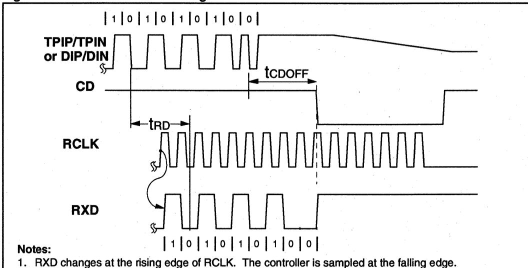
Figure 4: Mode 1 Transmit Timing
