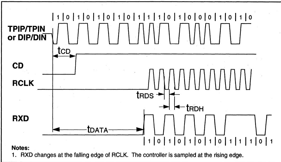
**Figure 21: Mode 4 RCLK/End-of-Frame Timing**
