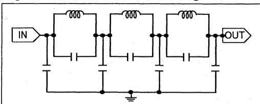
Figure 10: Receive Filter Diagram
