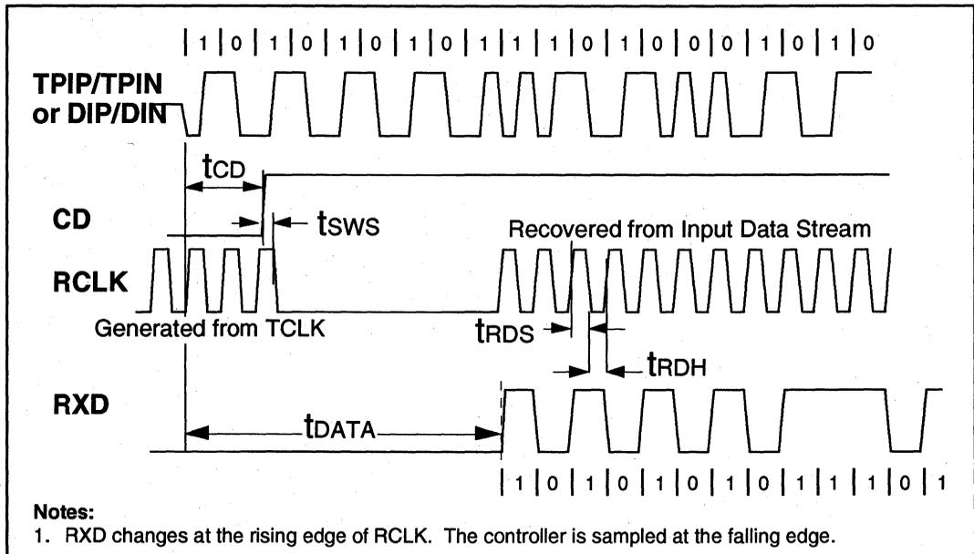
**Figure 15: Mode 3 RCLK/End-of-Frame Timing**
