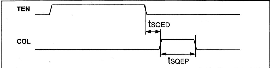
Figure 7: Mode 1 Loopback Timing
