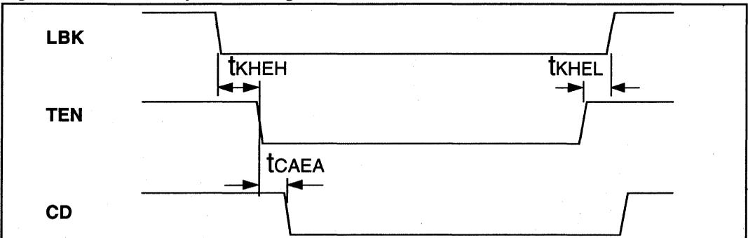
**Figures 14 through 19 - Timing Diagrams for Mode 3 (MD1 = 1, MD0 = 0)**
