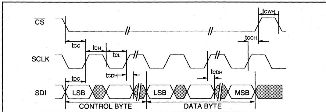
**Figure 8: LXT305A Serial Data Output Timing Diagram**
