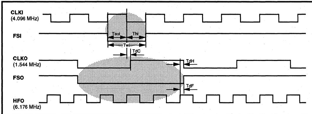
Figure 5: LXP600A Low to High Frequency Conversion Frame Sync Alignment
