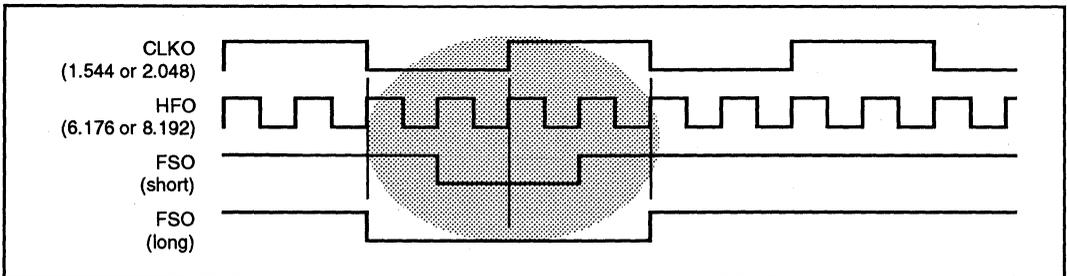
Figure 7: Output Frame Sync Alignment when HFO = 5 x CLKO
