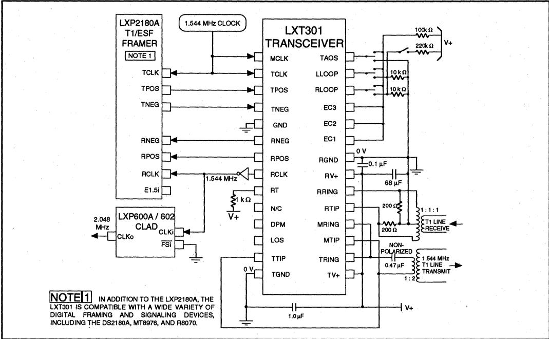
Figure 13: Typical LXT301 2.048 MHz E1 Application
