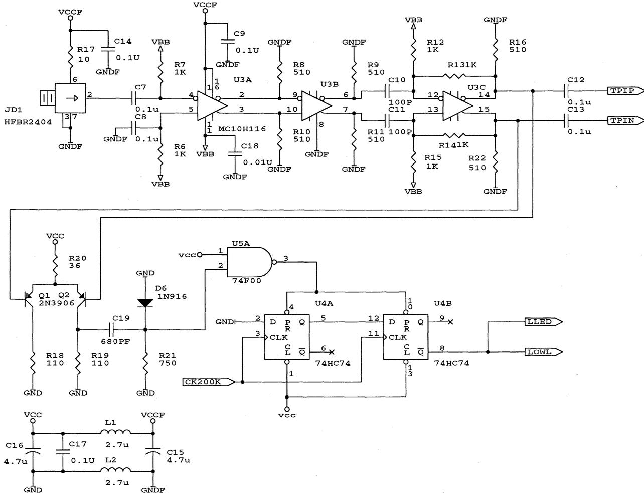
Figure 4: Fiber Output Port Schematic
