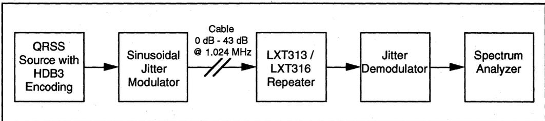
**Figure 7: Receiver Noise Interference Margin Test Setup**
