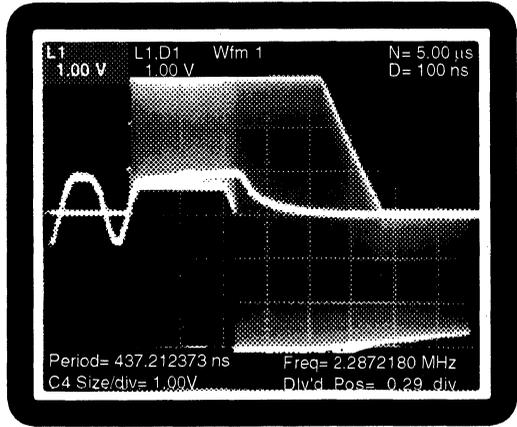
Figure 6A: Link Test Pulse before Line Model
