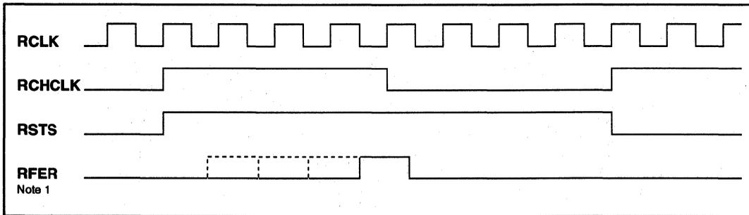
Figure 26: CRC4 Sub-Multiframe 2 Errored
