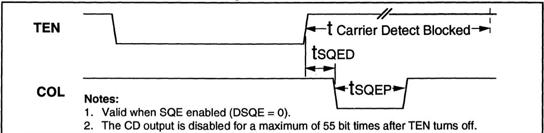
Figure 13: Mode 2 Loopback Timing
