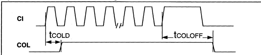
Figure 6: Mode 1 COL/CI Output Timing
