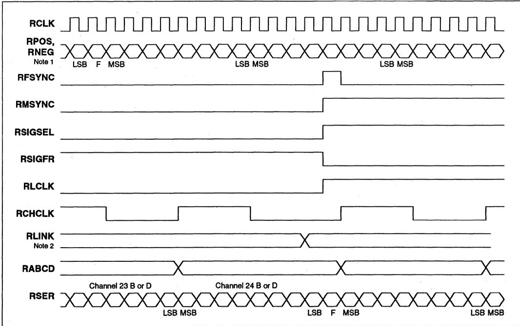
1. Total delay from RPOS and RNEG to RSER output is 13 RCLK periods.
