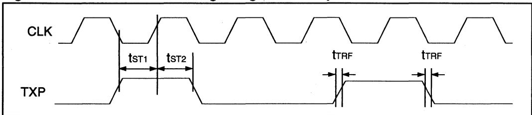
Figure 4: LXT903 Transmit Timing - Differential Input Mode
