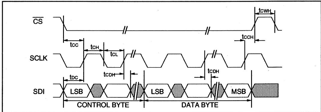
**Figure 8: LXT304A Serial Data Output Timing Diagram**
