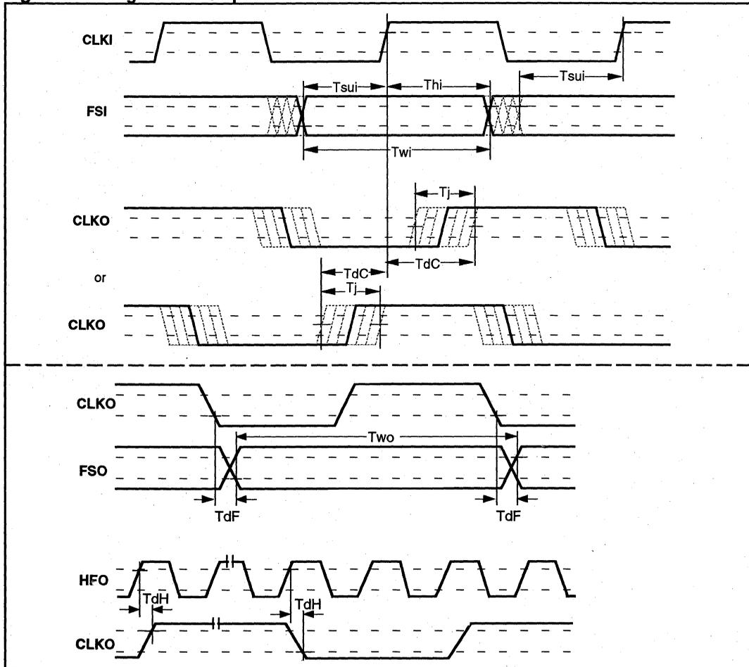
Figure 4: Output Frame Sync Alignment when HFO = 2 x CLKO
