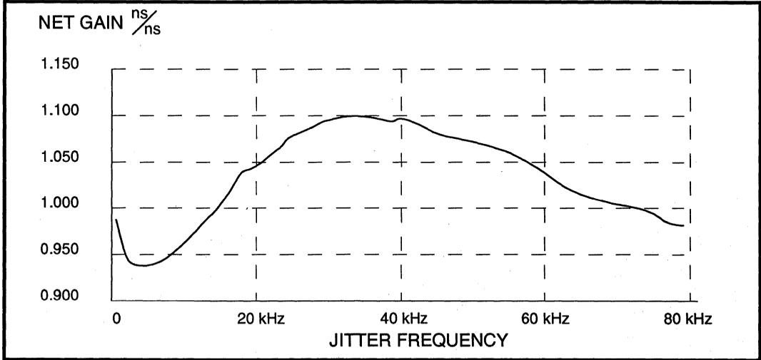
**Figure 9: Nominal Jitter Transfer - 1.544 MHz CLKI to 2.048 MHz CLKO (Input Jitter = 0.25 UI)**
