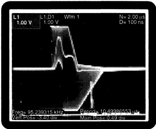
**Figure 5A: Link Test Pulse before Line Model**
