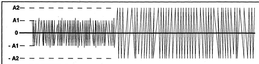
different length. These changes trigger the RLOS report and automatic re-initialization. Any remote changes in line length or transceiver configuration are beyond the local user's control. Remote changes in baud rate are not detected.
