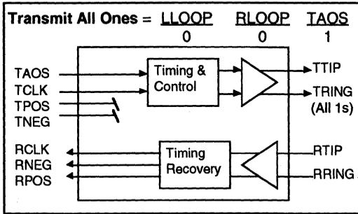
Figure 15: TAOS with LOOP Data Path
