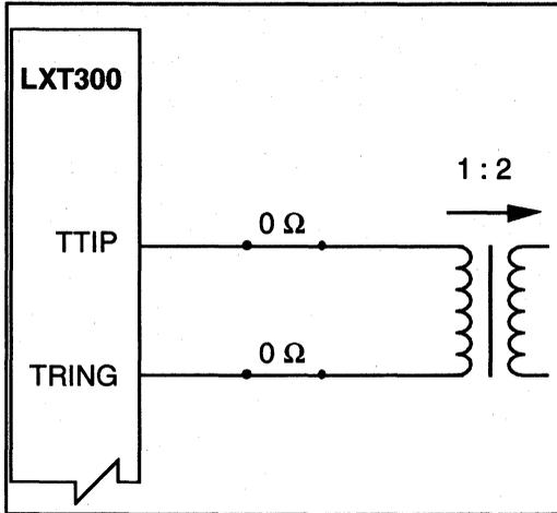
**Figure 1a: LXT300 Transmit Line Interface**
