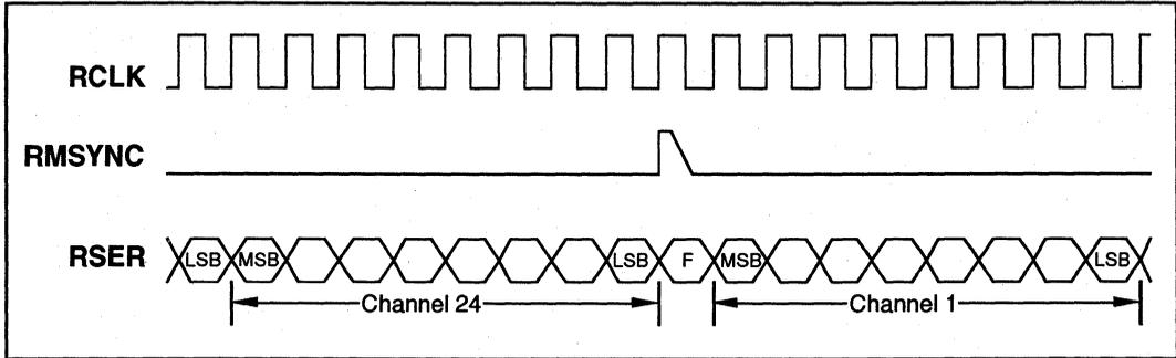
**Figure 3: Receive Side Timing (RCLK = 2.048 MHz)**
