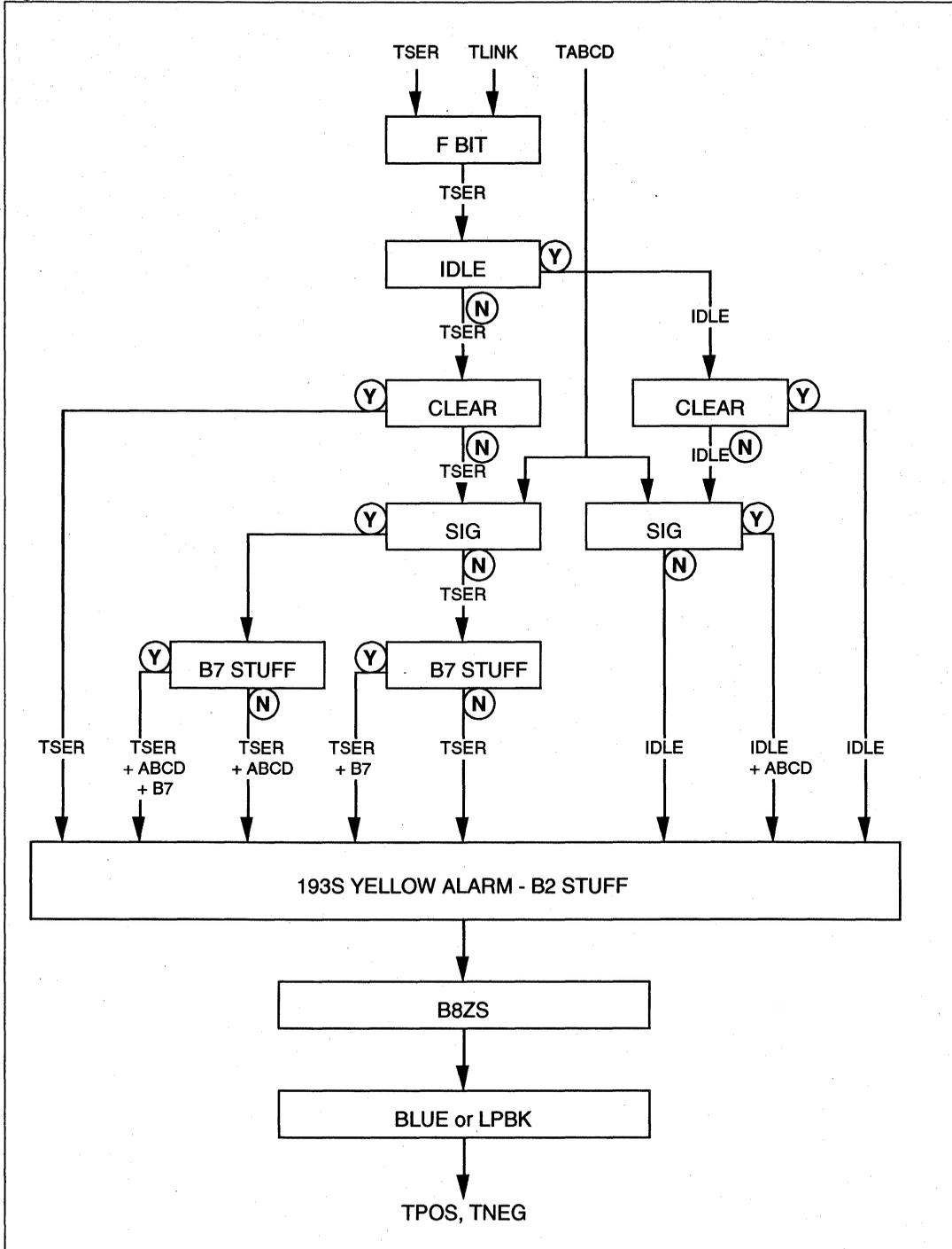
Figure 9: 193S Transmit Multiframe Timing
