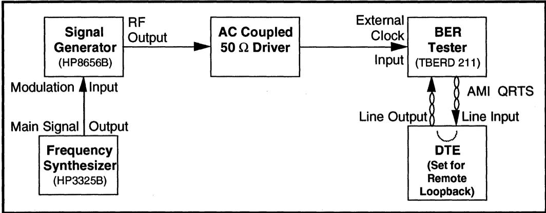
**Figure 3: Charting Input Jitter Tolerance Test Results**
