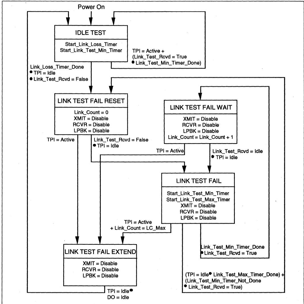
are transmitted in the absence of receive traffic. If no serial data stream or link integrity pulses are detected within 50 - 150 ms, the chip enters a link fail state and disables the transmit and normal loopback functions. The LXT901 ignores any link integrity pulse with interval less than 2 - 7 ms. The LXT901 will remain in the link fail state until it detects either a serial data packet or two or more link integrity pulses.
