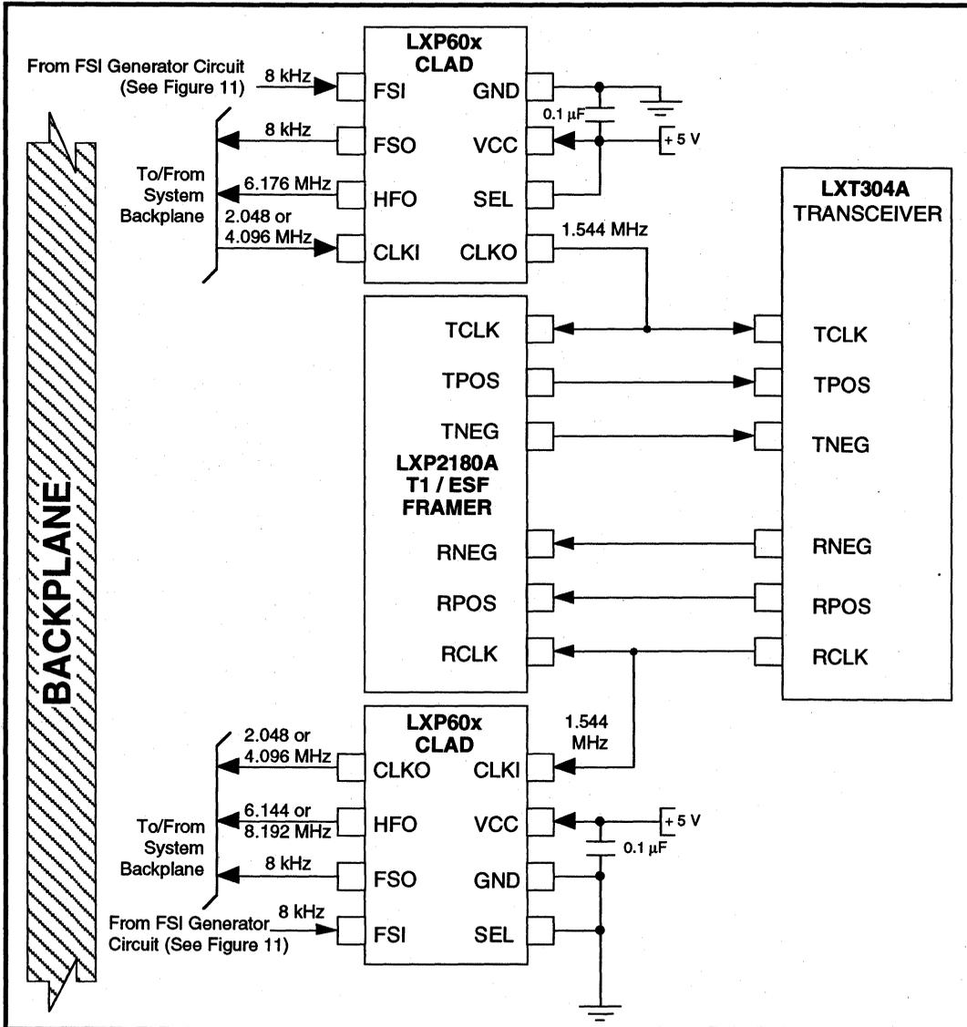
The CLADs are monolithic silicon devices which incorporates both analog and digital circuits. CLAD application circuit design may require closer attention to power supply filtering and bypassing than required for strictly digital devices.
