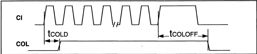
Figure 6: Mode 1 COL/CI Output Timing
