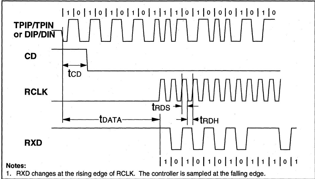
**Figure 9: Mode 2 RCLK/End-of-Frame Timing**
