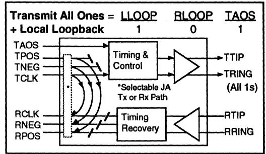
Figure 16: Local Loopback Data Path
