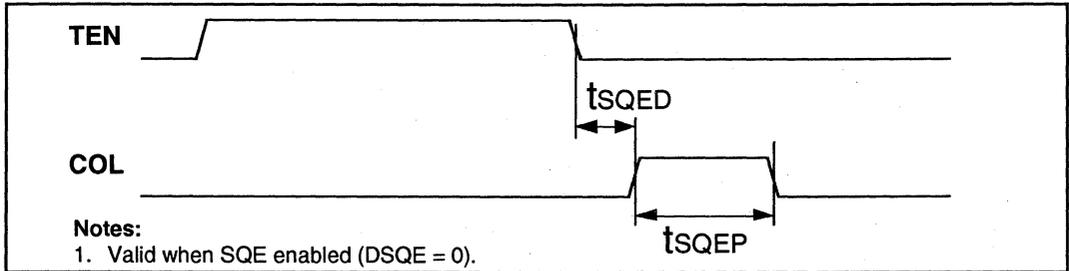
Figure 25: Mode 4 Loopback Timing
