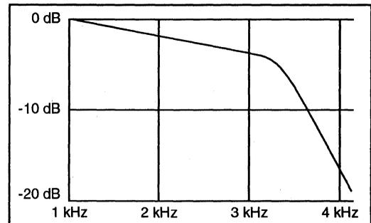
Depending on the data rate, the frequency template extends to different limits as shown in Table 9. (An alternate notch filter is used for data rates of 3.5 and 7.0 kbps.) The single pole, low-pass filter would maintain the frequency within  $\pm 5\%$ . The notch filter attenuation is added to this.
