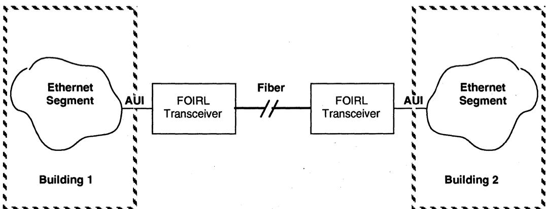
Figure 2: Application Schematic
