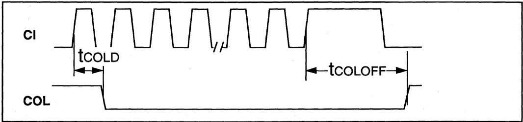
Figure 18: Mode 3 COL/CI Output Timing
