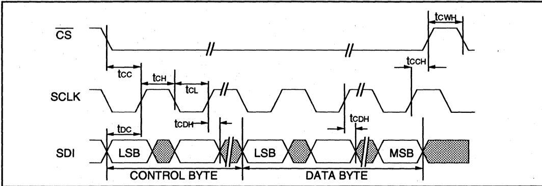
**Figure 7: LXT305 Serial Data Output Timing Diagram**
