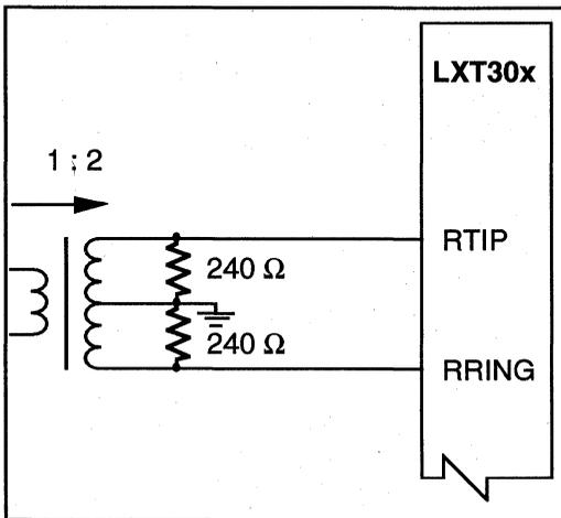
**Figure 2a: LXT30x Receive Line Interface**
