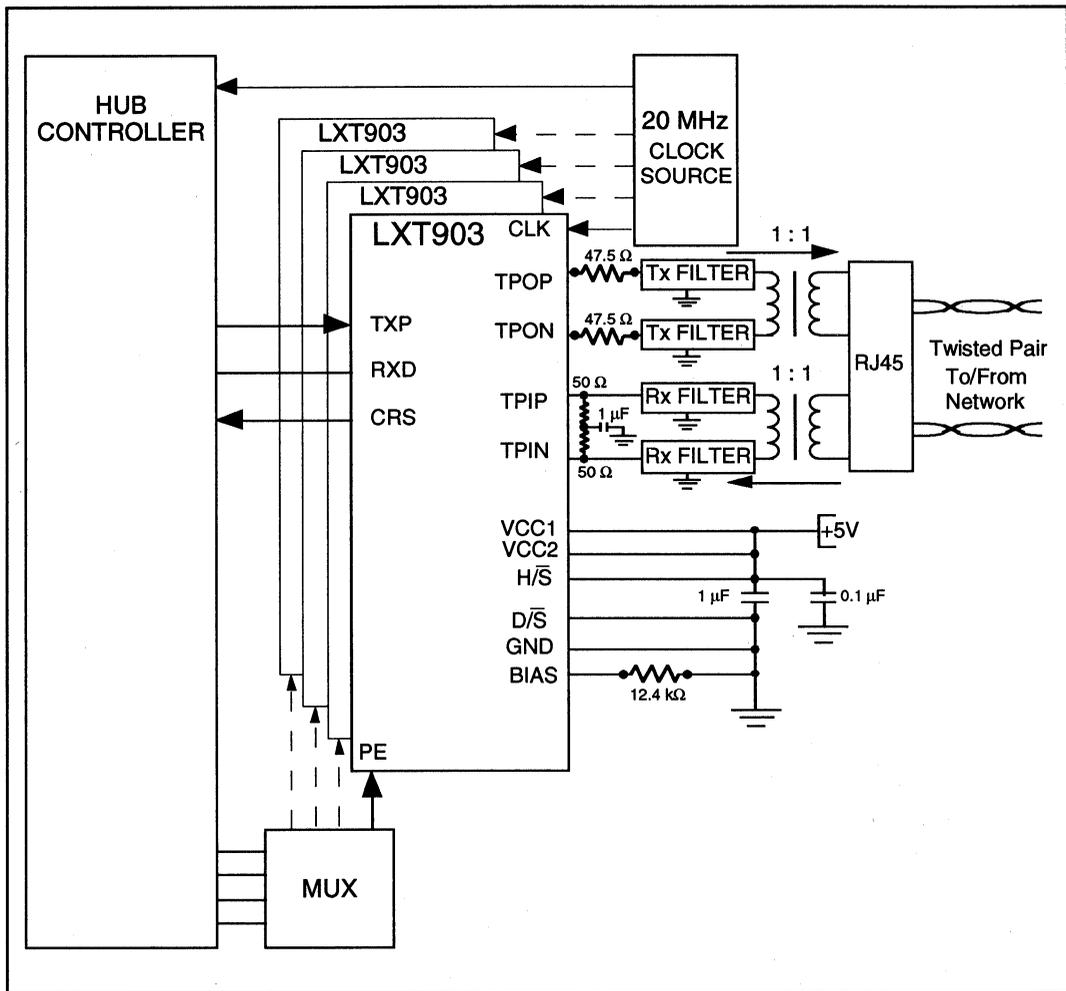
Figure 11: Transmit Filter Diagram
