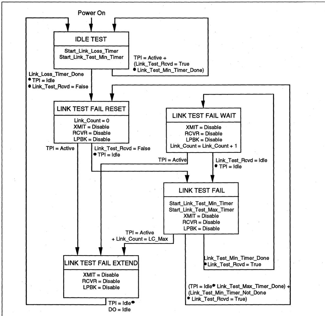
data stream or link integrity pulses are detected within 50 - 150 ms, the chip enters a link fail state and disables the transmit and normal loopback functions. The LXT907 ignores any link integrity pulse with interval less than 2 - 7 ms. The LXT907 will remain in the link fail state until it detects either a serial data packet or two or more link integrity pulses.
