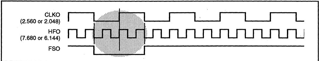
Figure 6: Output Frame Sync Alignment when HFO = 4 x CLKO
