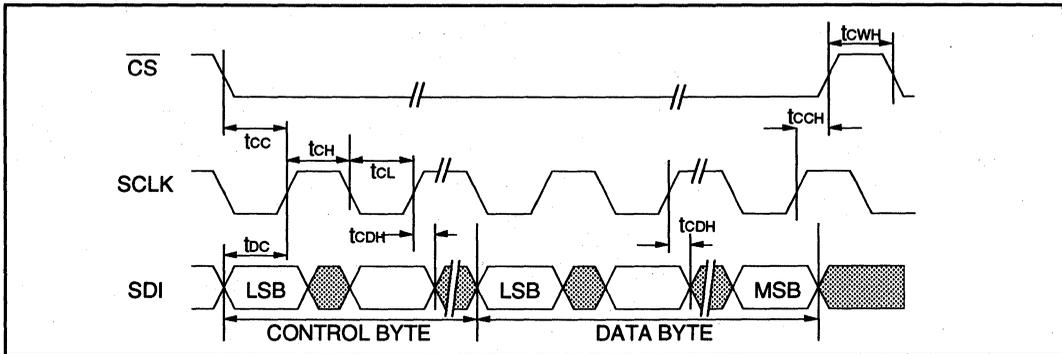
**Figure 12: LXT318 Serial Data Output Timing Diagram**
