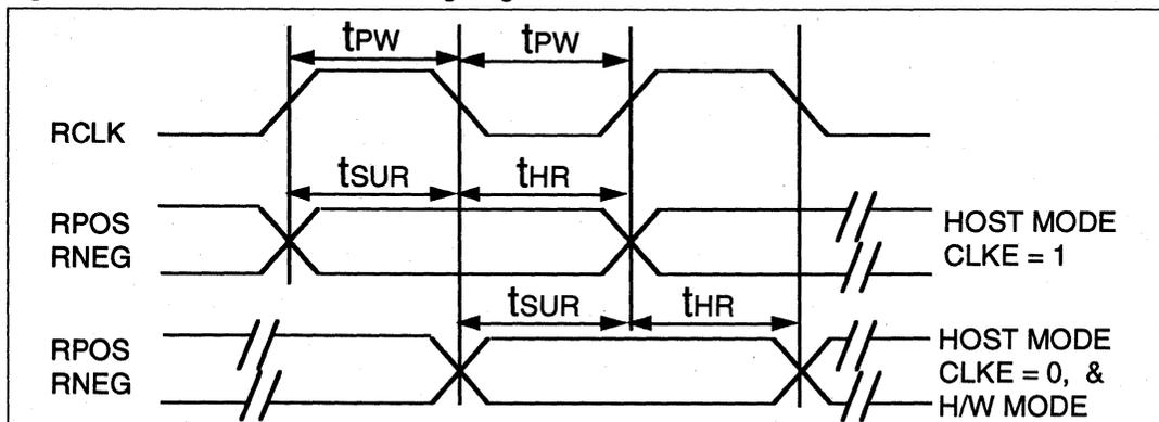
(spaces). The receiver monitor loads a digital counter at the RCLK frequency. The count is incremented each time a zero is received, and reset to zero each time a one (mark) is received. Upon receipt of 175 consecutive zeros the LOS pin goes high, and the RCLK output is replaced with the MCLK.
