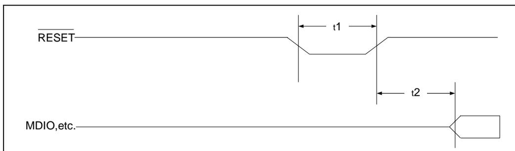
Table 51. RESET Pulse Width and Recovery Timing Parameters
