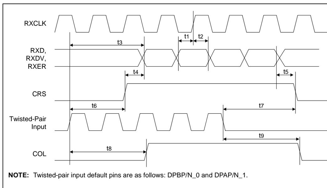
Table 45. MII - 10BASE-T Receive Timing Parameters (Parallel Mode)
