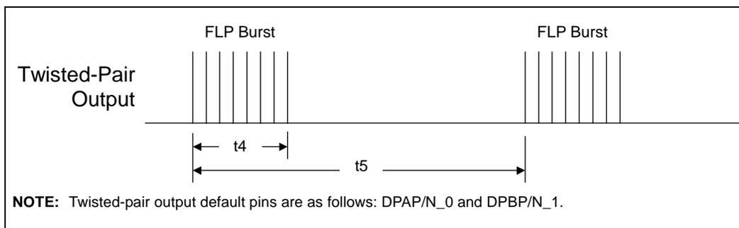
Table 48. Fast Link Pulse Timing Parameters
