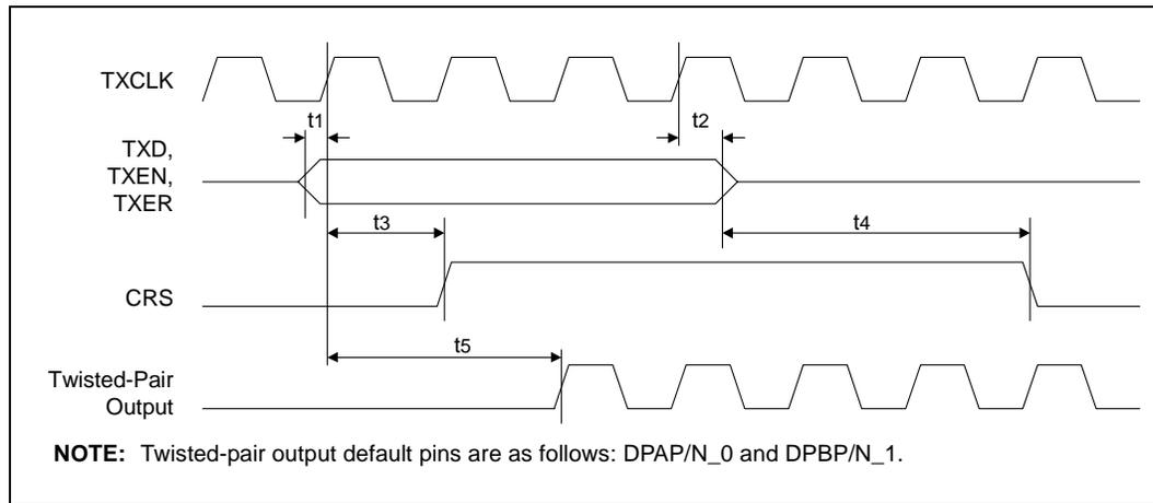
Table 44. MII - 10BASE-T Transmit Timing Parameters (Parallel Mode)
