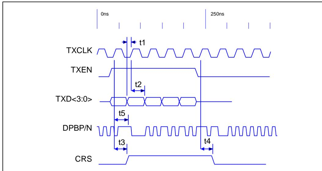
Table 42. 100BASE-FX Transmit Timing Parameters
