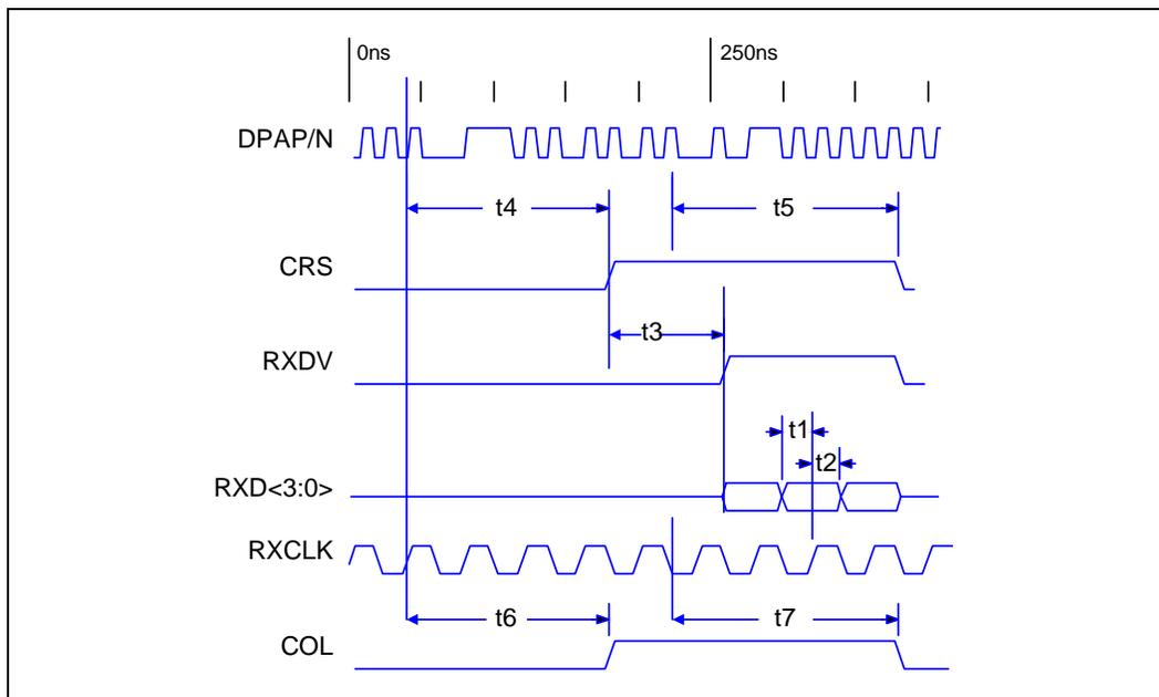
Table 43. 100BASE-FX Receive Timing Parameters
