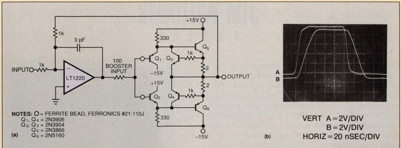
**Fig F**—This circuit (a) produces more pleasing results than Fig Ea's circuit. The 45-MHz LT1220 replaces the 100-MHz LT1223. The slower amplifier now works well with the booster stage in its loop. The circuit is well controlled, with no sign of oscillation (b).
