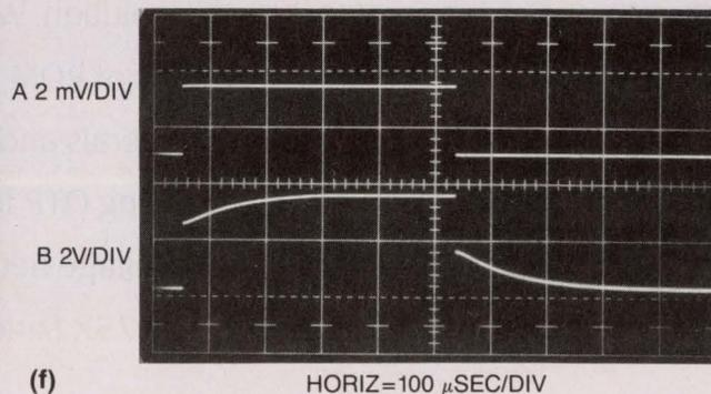
(c) as a slight peak near 6 MHz. In the other three photos, (d, e, and f), you see, respectively, the effects of correctly matching the ac and dc gains, setting the ac gain too high, and setting the dc gain too high.
