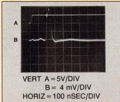
**Fig C**—The 280-nsec settling time shown here was measured using the Fig B circuit. The sampling switch closes just before the third vertical division, which lets you observe the settling detail without overdriving the oscilloscope.
