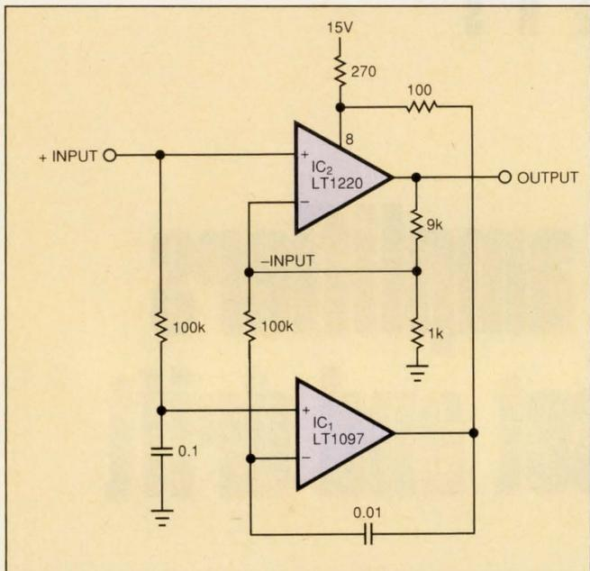
**Fig 2**—You can also stabilize the offset of a wideband amplifier ( $IC_2$ , in this case) by using a precision dc amplifier ( $IC_1$ ) to apply correcting signals to the wideband amplifier's offset-trim adjustment pin.
