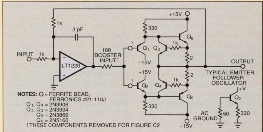
**Fig A**—In this booster circuit, the 100Ω resistor and the ferrite beads at the inputs of Q<sub>1</sub> and Q<sub>2</sub> play a critical role in maintaining stability.
