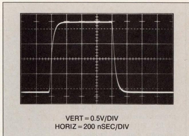
**Fig 8**—Excessive source impedance produced this serene—but undesired—result.
