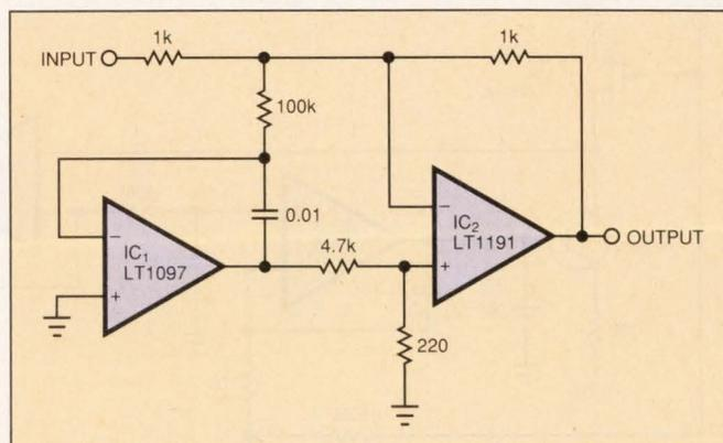
**Fig 1**—An integrator ( $IC_1$ ) reduces the drift of a wideband amplifier ( $IC_2$ ) by applying a signal to the wideband amplifier's noninverting input. That signal holds the wideband amplifier's summing junction at ground.
