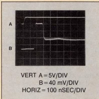
**Fig E**—Harvey's method was used to obtain this 280-nsec settling-time measurement. After subtracting this method's inherent 30-nsec delay, the settling time and waveform are identical to that of Figs C and D.
