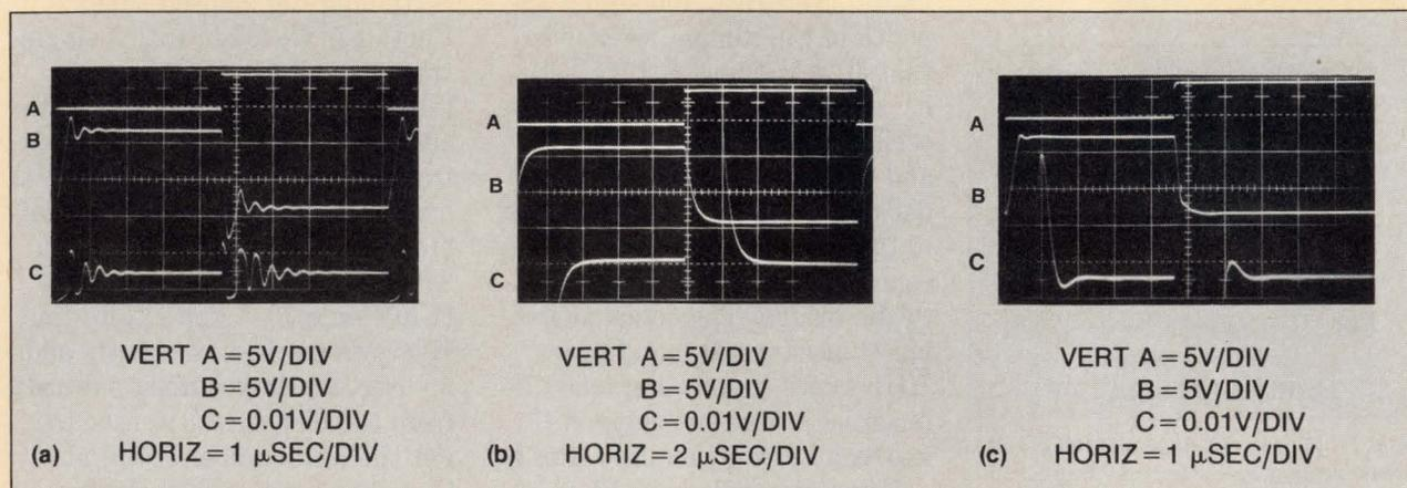
**Fig F**—These three scope traces show the effects of different values of feedback capacitors on DAC-amplifier combinations. The values for the three photos are no capacitance (a), 82 pF (b), and 22 pF (c).
