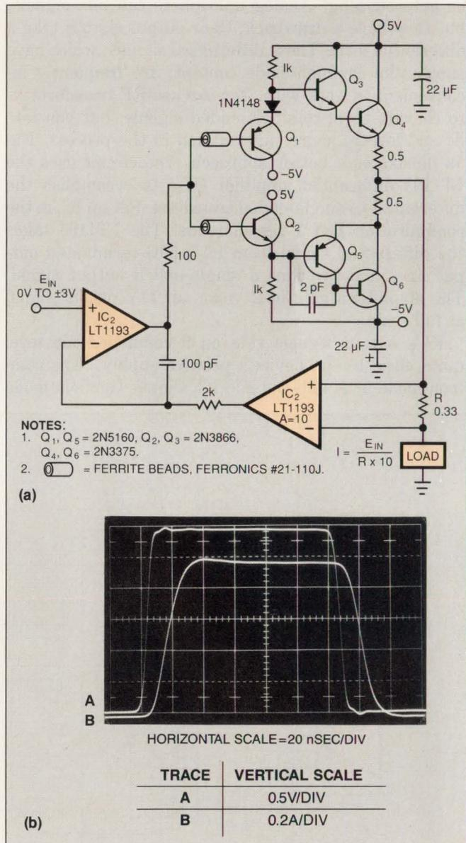
**Fig 8**—A booster circuit in the middle of this voltage-to-current converter (a) provides more power to your load than does the current source of **Fig 7**. Trace A (b) represents voltage; trace B represents current.
