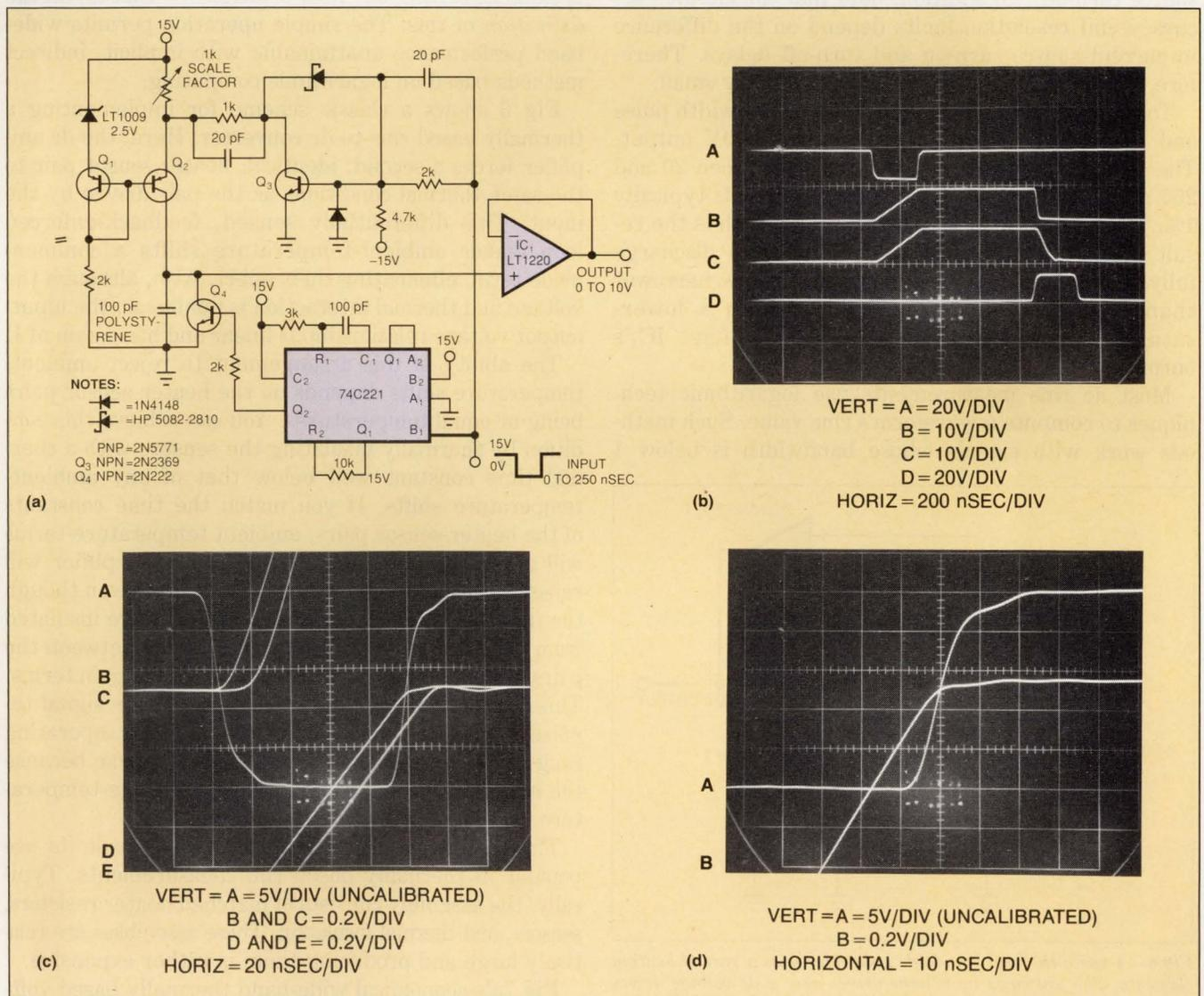
**Fig 5—Changing pulse widths to voltages** provides a convenient way to monitor changes in time intervals that occur as a function of time. The circuit in **a** performs this function. In **b** you see circuit waveforms. These waveforms appear in expanded form in **c**. The current-source turn-off appears in **d**.
