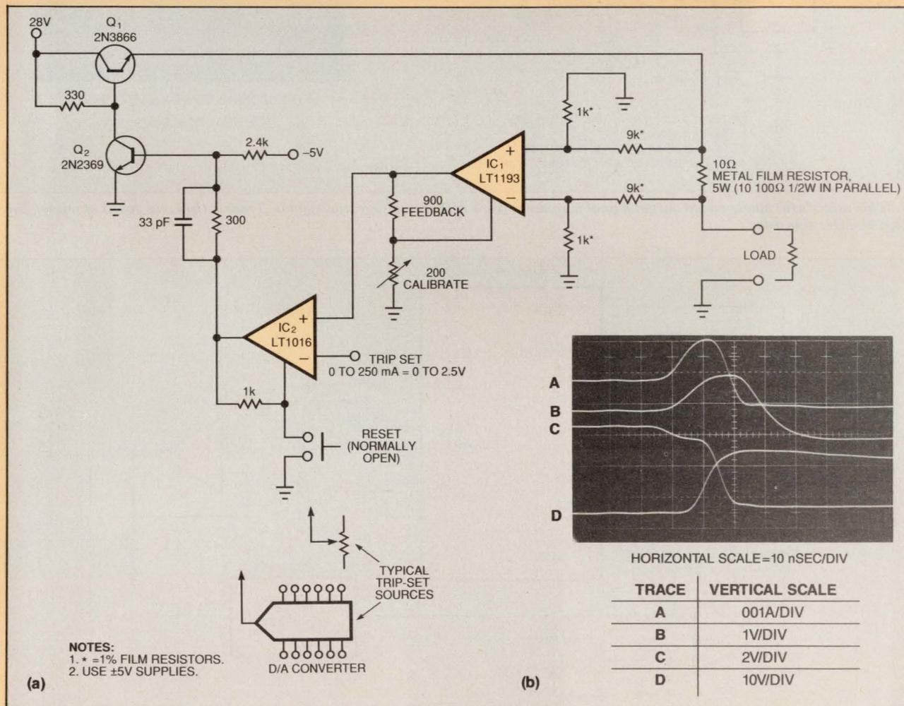
Fig A—This circuit breaker (a) trips in as little as 18 nsec. The circuit shuts down the load (b, trace C) when the load current (trace A) exceeds the trip point. Trace B represents IC<sub>1</sub>'s output voltage; trace D represents IC<sub>2</sub>'s output voltage.
