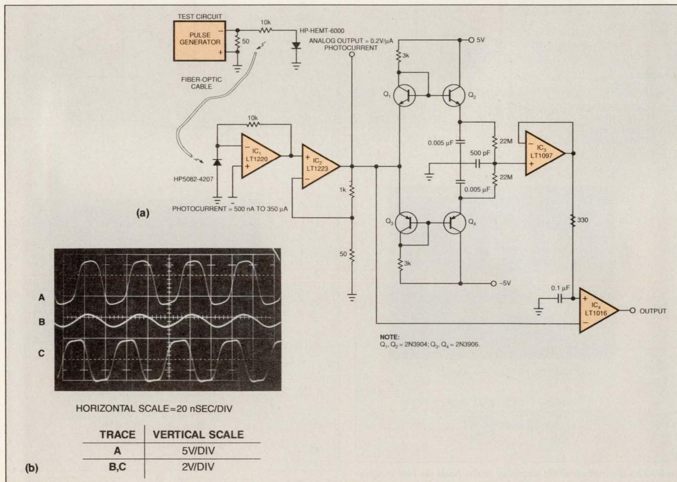
**Fig 4—A self-adapting threshold** is the hallmark of this optical receiver (a). Driven by a test signal (b, trace A), the circuit lets you monitor the detector's current (trace B) in addition to producing a final output (trace C).
