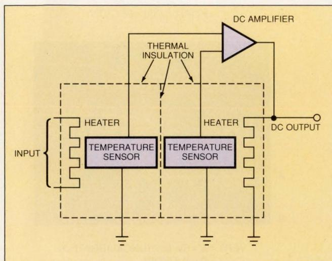
**Fig 6**—A basic thermal rms-to-dc converter uses a pair of heating elements. The unknown ac voltage drives one; a dc voltage drives the other. By using a high-gain amplifier to provide the dc voltage, you force the heating effect of the dc to equal that of the ac. Hence the rms value of the dc and ac are equal. Thus, when you measure the dc voltage, you are measuring the rms ac voltage.
