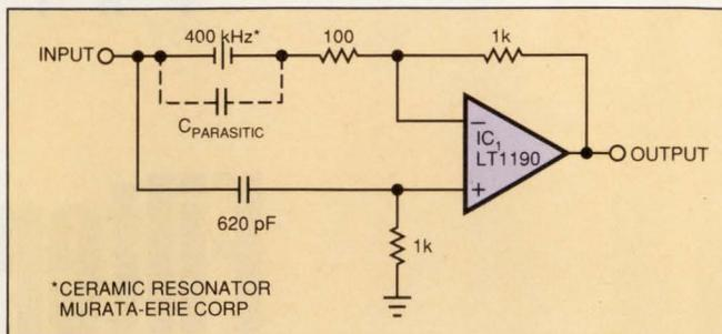
**Fig 2**—A slight modification of the circuit in Fig 1a allows you to cancel out the effects of the resonator's parasitic capacitance. The dashed curve of Fig 1b shows the effects on the filter response. Below resonance, the modified circuit attenuates by an extra 20 dB. Above approximately 525 kHz, the improvement is even more dramatic.
