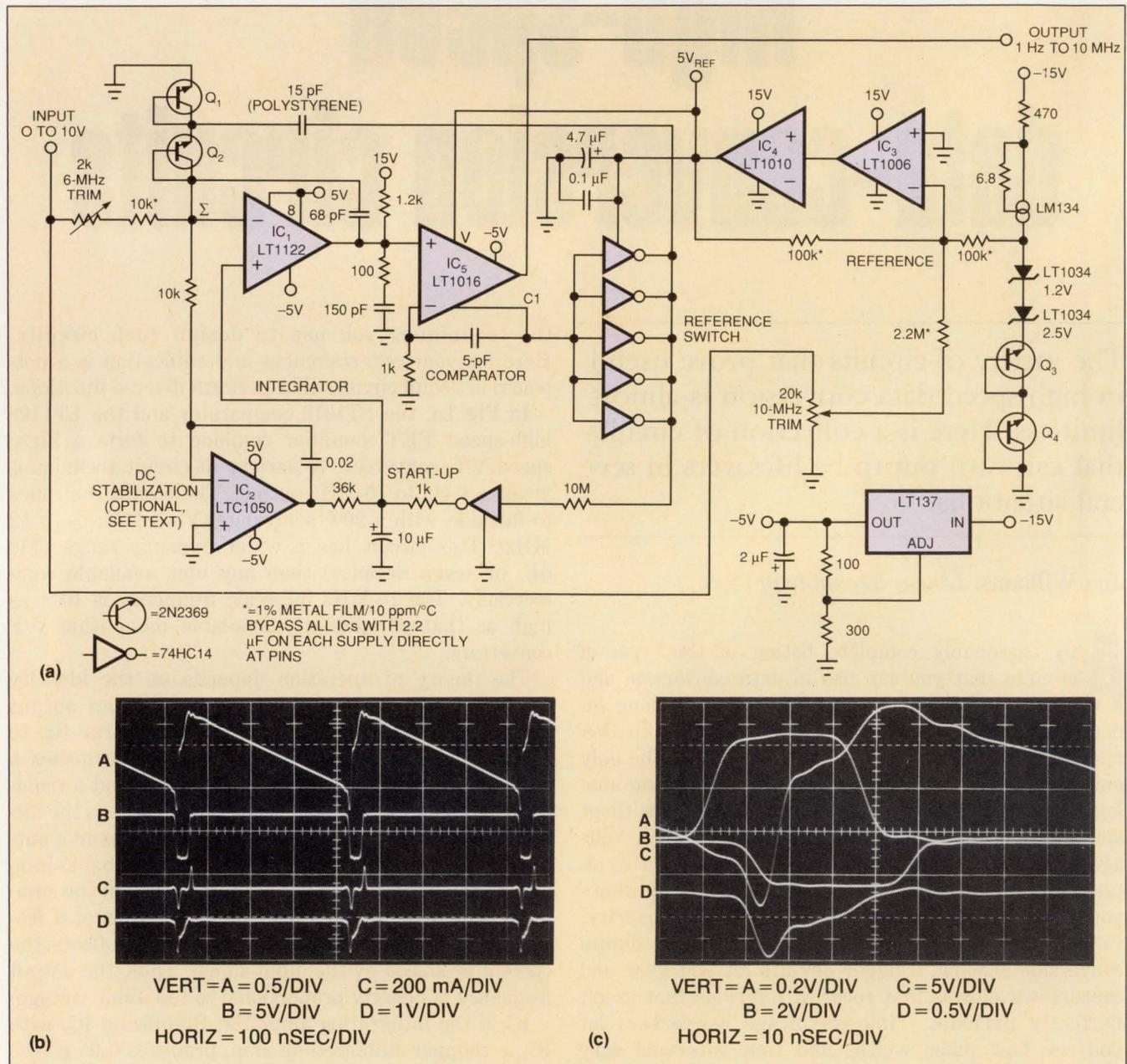
**Fig 1—A voltage-to-frequency converter** with a maximum output frequency of 10 MHz and a 140-dB dynamic range is only moderately complex (a). In b, you see the circuit waveforms; c is an expanded view of the discharge-reset sequence upon which the circuit performance depends.
