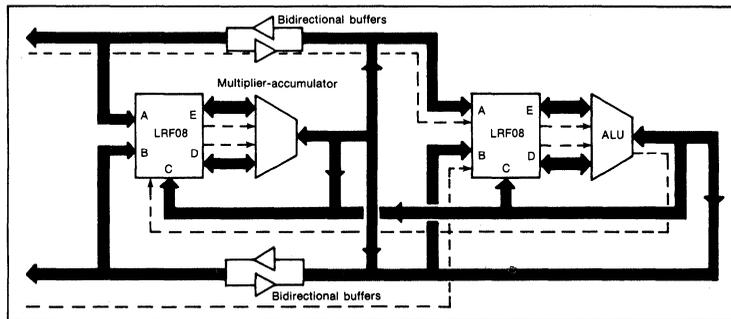
3. Used in a pipeline processor, the multiport register file makes reconfiguration easy. The large number of independent ports allows data routing through the system to be software controlled. The dotted lines show system data flow for a finite-impulse-response filter algorithm.
