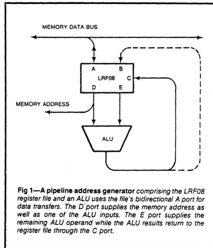
Fig 1—A pipeline address generator comprising the LRF08 register file and an ALU uses the file's bidirectional A port for data transfers. The D port supplies the memory address as well as one of the ALU inputs. The E port supplies the remaining ALU operand while the ALU results return to the register file through the C port.
