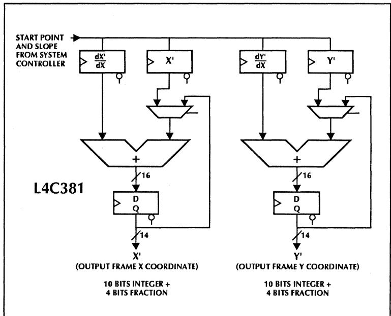
Frame Store outputs the values of the *four stored pixel values closest to the addressed point*. In order to accomplish this, only the integer part of the  $X', Y'$  address need be considered. If  $I(X')$  is taken to mean the integer part of  $X'$ , and similarly with  $Y'$ , then for an input address  $X', Y'$  the desired four pixel locations are:
