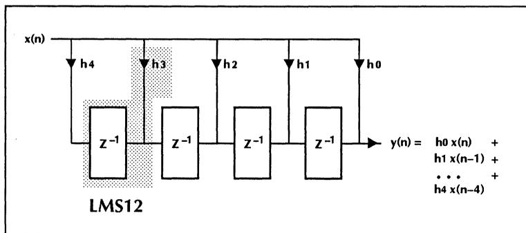
Figure 12. Horizontal Anti-aliasing Filter.
