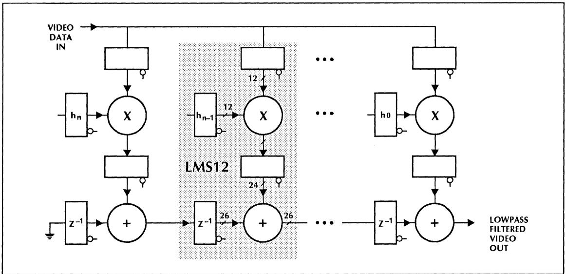
Figure 13. Vertical Anti-aliasing Filter.
