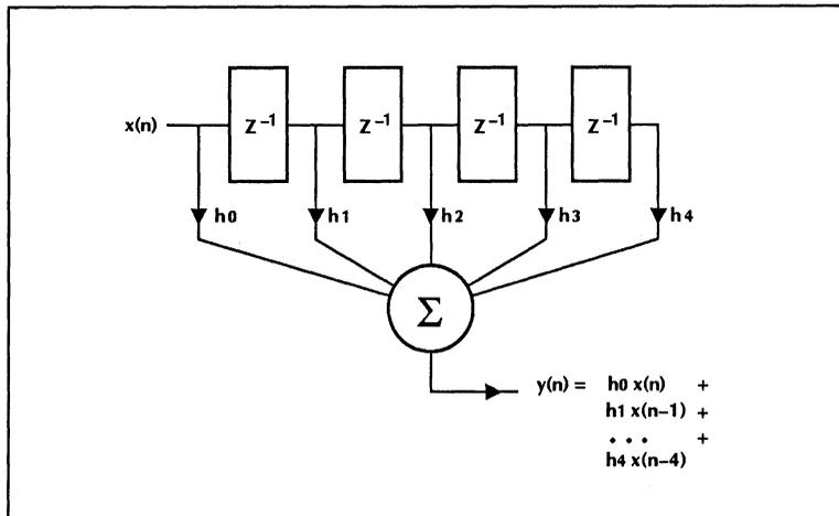
Figure 11. F.I.R. Filter (Transpose Form).
