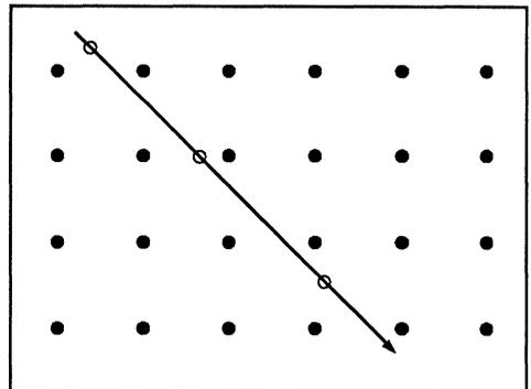
to calculate the value of a point which does not fall exactly on a pixel location. For the system under discussion, bilinear interpolation is used for this calculation.
