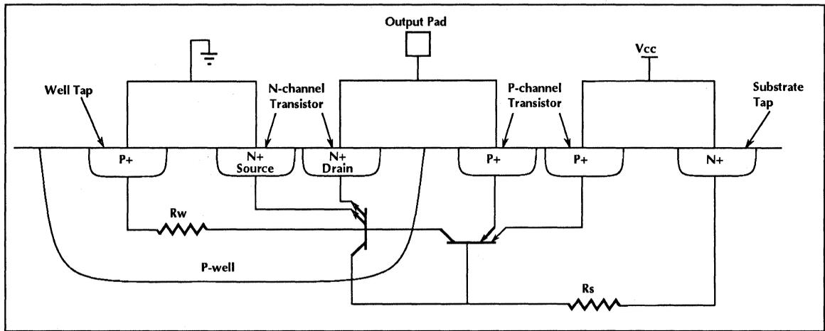
Figure 2. Equivalent circuit for Latchup path.
