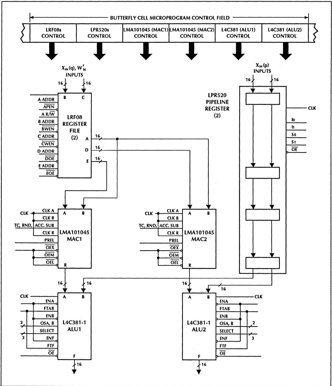
Devices' LRF08 multiport register file and L4C381 16-bit ALU. Because of their ability to be controlled by microcode, these two high-speed CMOS LSI devices provide the flexibility required of the FFT Address Sequencer. Also, the overhead time required to pre-sort the complex data sequence prior to the computation phase is reduced.
