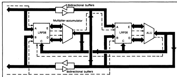
5. The LRF08 multiport register file allows reconfiguration of the pipeline architecture for a different algorithm, in this case, the complex decimation-in-time FFT butterfly (Fig. 4).
