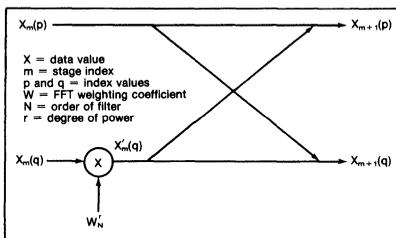
4. In a radix-two decimation-in-time butterfly, the basic unit of the fast Fourier transform, four real multiplications and six real additions take place.
