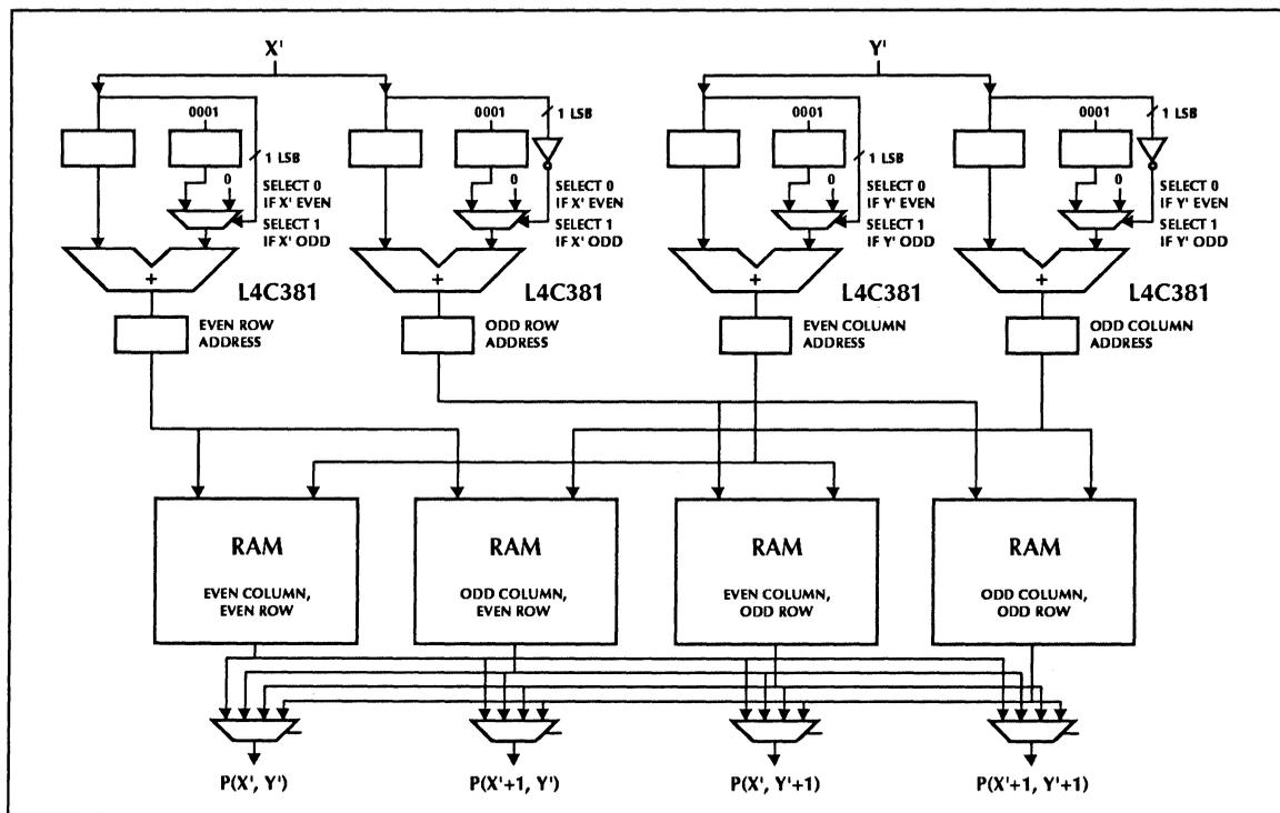
to address a RAM bank, i.e., the internal plane sizes are integral powers of 2. Once these addresses are formed, four memory accesses are executed in parallel. Finally, multiplexers route the appropriate data to the four output ports, with selection of these muxes again determined by whether X' and Y' are even or odd.
