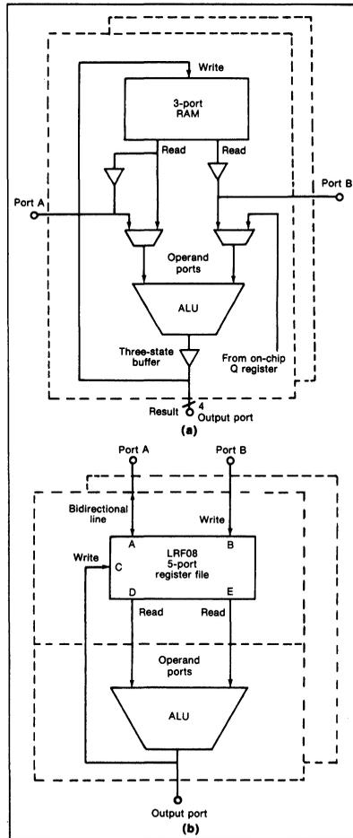
2. The bit-slice architecture of processors like the Am2903 (a) limits the memory-to-ALU bandwidth and leads to delays when outside data is introduced, because the ALU's operation may have to be suspended while the external data is written into the three-port RAM. Using the LRF08 allows complete overlap of an ALU operand and result transfers with external read/write of the register set (b).
