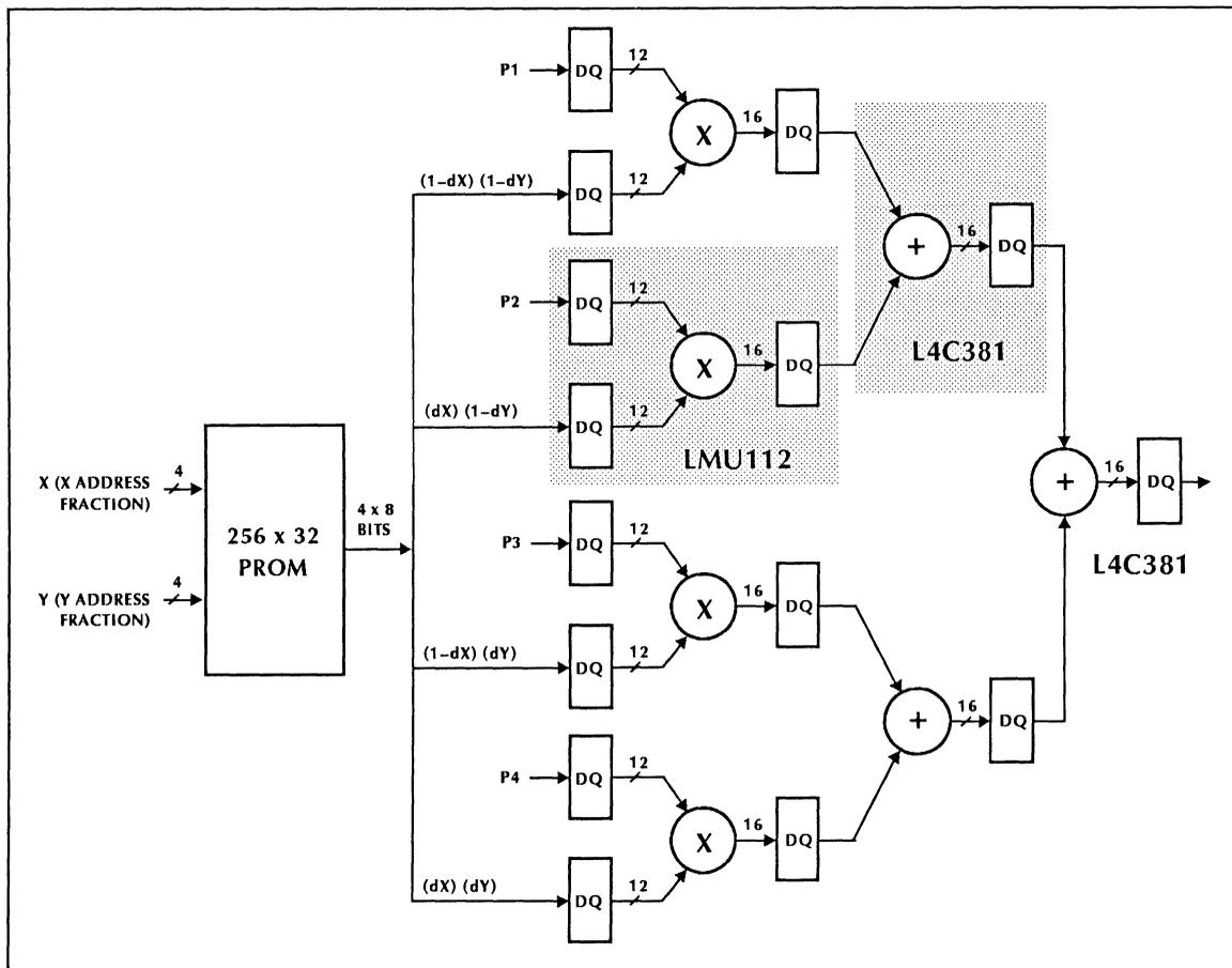
setting the function control lines of the last ALU stage to 000 (force-to-zero instruction) when writing the nonimage areas of the display memory, the pixel data stored in these locations is blanked. This instruction control is provided by the system controller.
