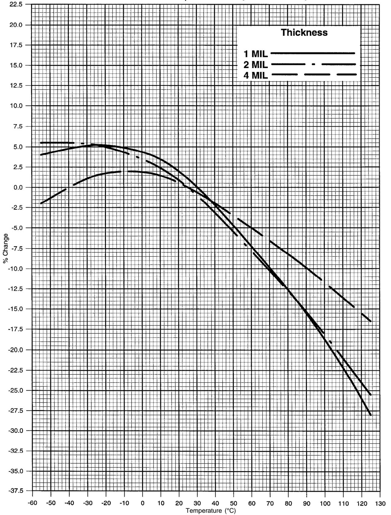
Curve #8: Variation of  $\Delta H_1$  of Permalloy 80 with temperature
