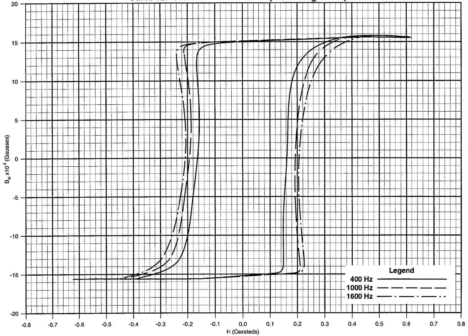
Curve #3: Permalloy 80 -- 0.001" thick (sine voltage drive)
