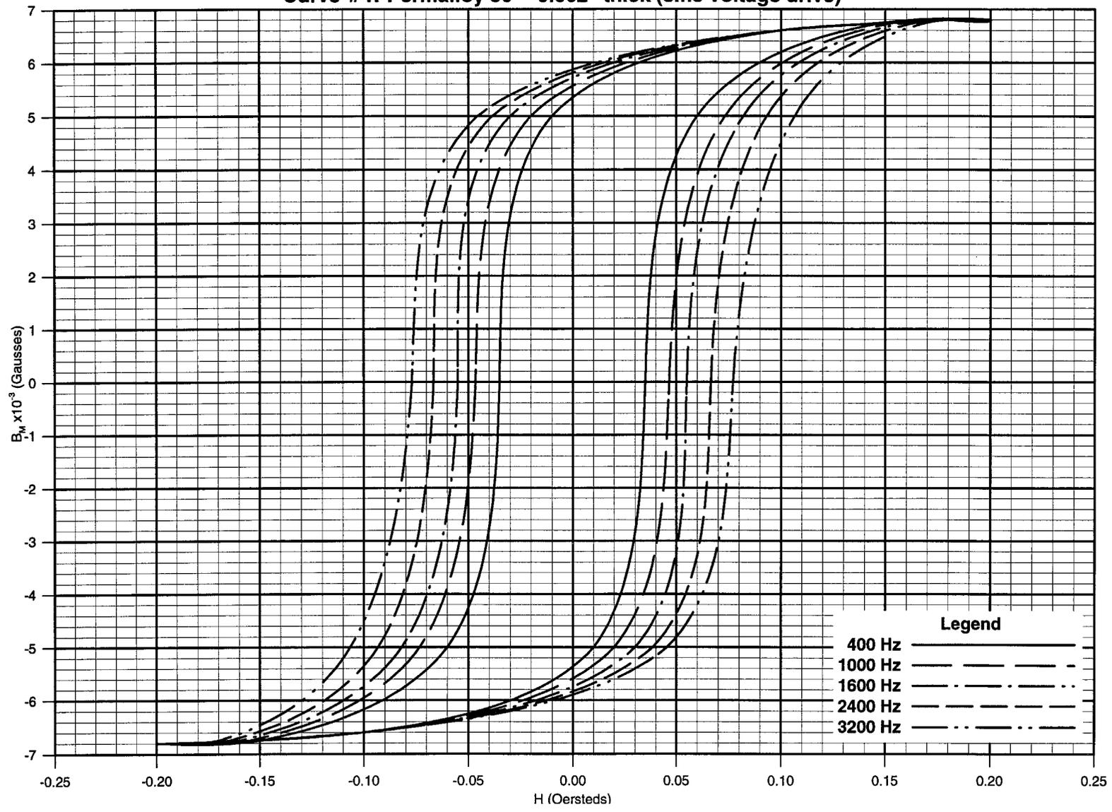
Curve #5: Average M.M.F. required to saturate Orthonol versus frequency (current drive)
