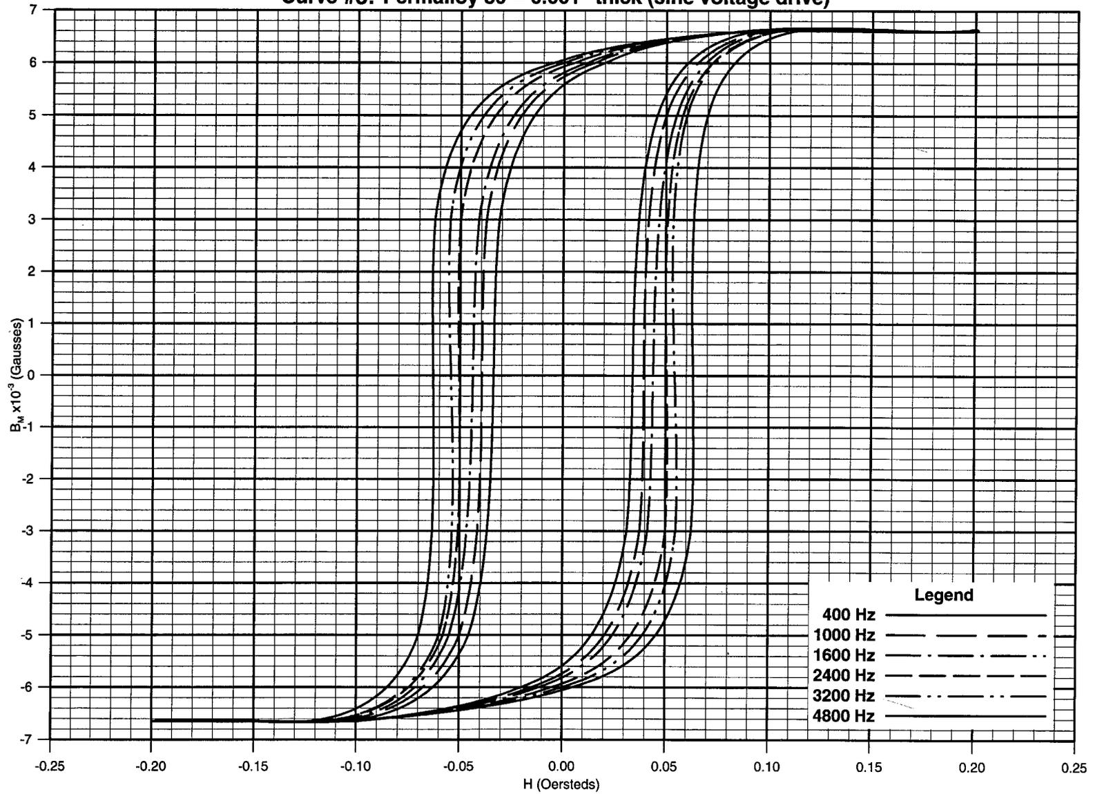
Curve #4: Permalloy 80 -- 0.002" thick (sine voltage drive)
