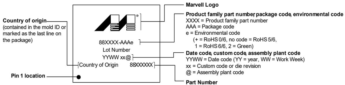
**Note:** The above drawing is not drawn to scale. The location of markings is approximate. Add-on marks are not represented. Flip chips vary widely in their markings and flip chip examples are not shown here. For flip chips, the markings may be omitted per customer requirement.
