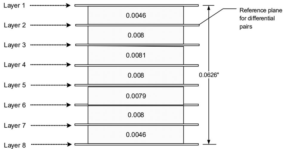
Table 4-2 details the stack-up parameters for the board shown in Figure 4-3.
